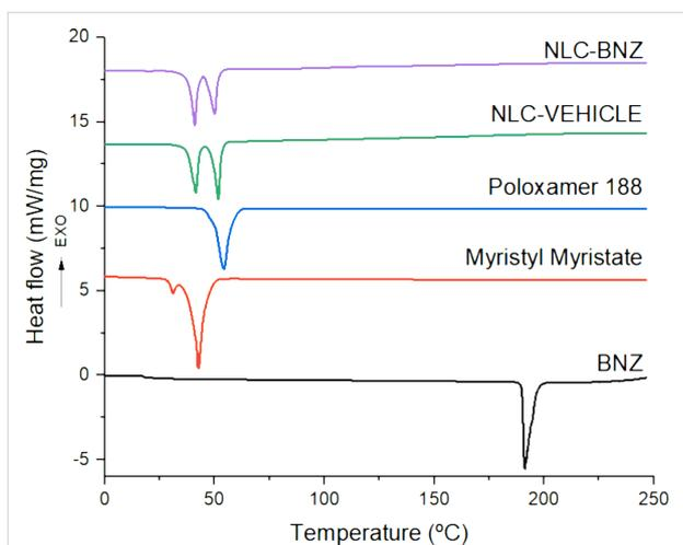
**Figure 2:** DSC thermograms of BNZ, myristyl myristate, poloxamer 188, NLC VEHICLE, and NLC-BNZ.
