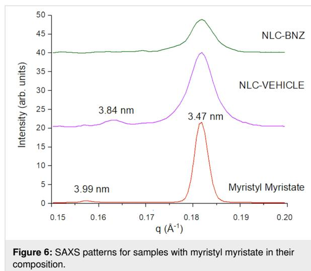
**Figure 6:** SAXS patterns for samples with myristyl myristate in their composition.
