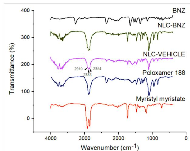
**Figure 4:** ATR-FTIR spectra of BNZ, myristyl myristate, poloxamer 188, NLC VEHICLE, and NLC-BNZ.
