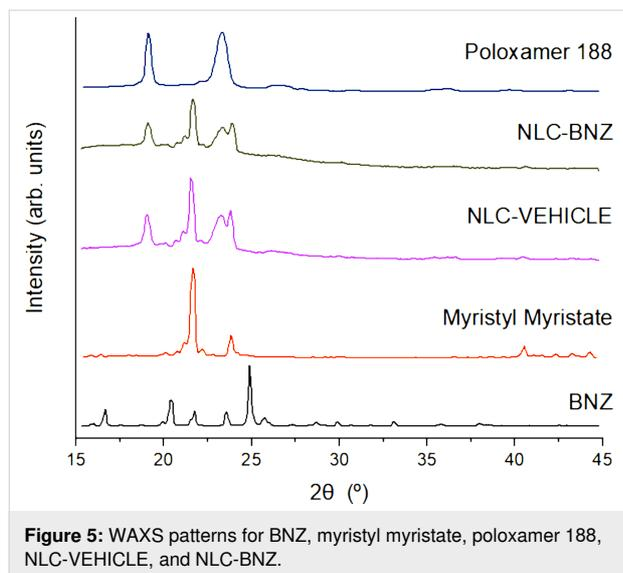
**Figure 5:** WAXS patterns for BNZ, myristyl myristate, poloxamer 188, NLC-VEHICLE, and NLC-BNZ.
