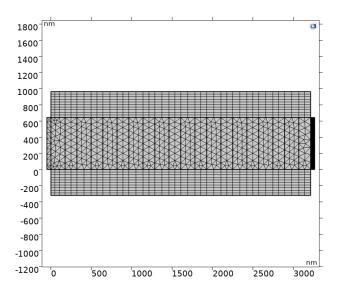
**Figure S2:** The customized triangular and rectangular mesh discretization on the PhC geometry built in COMSOL.
