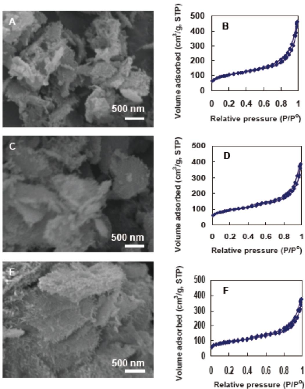
**Figure S1:** SEM images (A, C and E) and N<sub>2</sub> adsorption/desorption isotherms (B, D and F) of silica nanotubes synthesized with silicification times of 5 min (A and B), 60 min (C and D) and 240 min (E and F). The synthetic conditions for LPEI aggregates and silica deposition are the same as those used for Figure 3.
