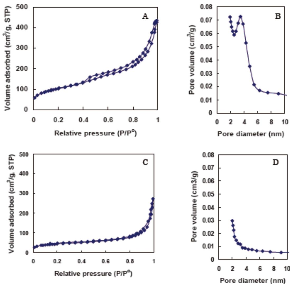
**Figure S2:** N<sub>2</sub> adsorption/desorption isotherms (A and C) and BJH pore-size distribution curve obtained from the adsorption branch (B and D) of silica nanotube (A and B) and silica nanoribbon (C and D). The synthesis conditions are the same as those of the samples shown in Figure 4. The sample was calcined at 800°C in air for 3h with at heating rate of 2.5°C per min.
