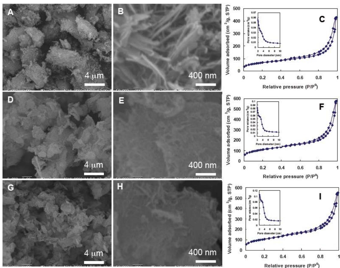
**Figure S5:** SEM images (A, B, E, F, H and I) and BET results (C, G and J) of nanostructured silicas synthesized by using bases of Et<sub>4</sub>NOH ([OH]/[EI] = 1.6) (A–C), LiOH ([OH]/[EI] = 2.7) (D–F) and KOH ([OH]/[EI] = 3.2) (H–J). 0.5 g of LPEI-HCl was dissolved into 6 mL of water for LPEI self-assembly induced with various bases. The silica deposition was performed by stirring a mixture of 1.5 mL of MS51 and 15 mL of aqueous dispersion of LPEI aggregates for 4 h at room temperature.
