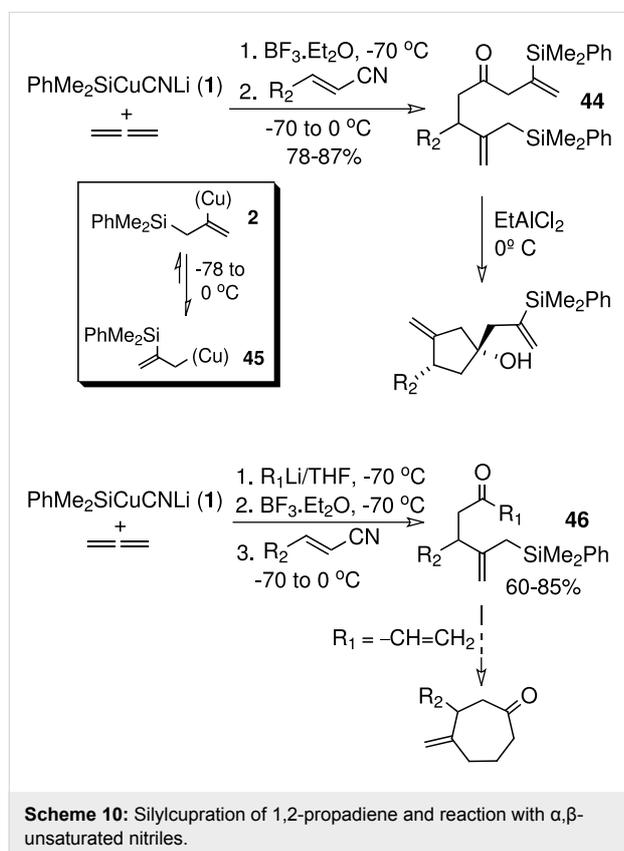
When  $\text{R}_1\text{Li}$  is an alkenyllithium this reaction opens new alternatives for preparation of 7-membered rings by intramolecular Michael addition of the allylsilane group to the enone (Scheme 10).
