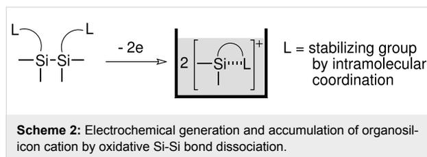
Symmetrical disilanes having coordinating groups on both silicon atoms were used as starting materials for electrochemical generation and accumulation of organosilicon cations, because oxidative dissociation of the Si-Si bond leads to the formation of two equivalents of organosilicon cations and no other product is formed.
