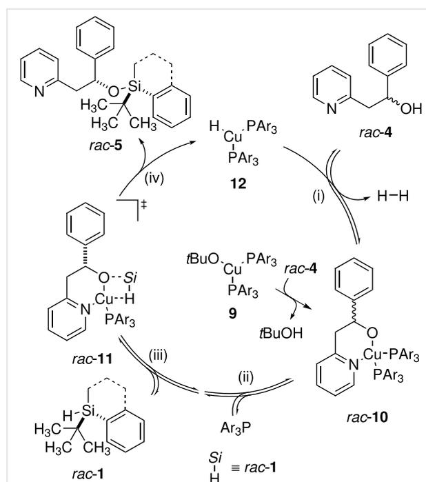
**Scheme 4:** Postulated catalytic cycle for dehydrogenative coupling.
