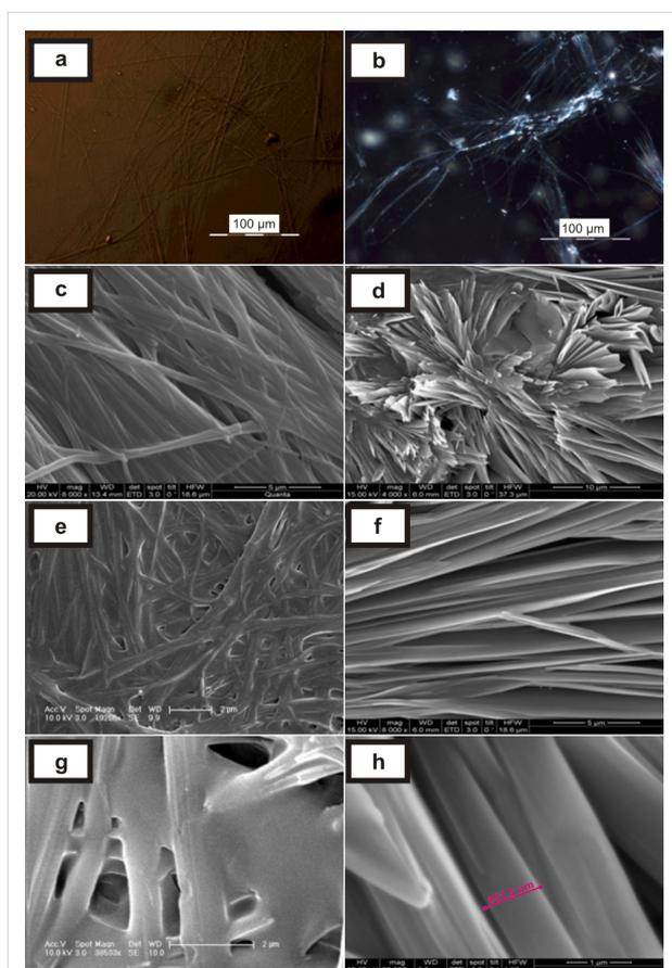
**Figure 5:** (a) and (b) POM images of bis(2-hydroxyethyl)aminodeoxycholate **2** gel in 1:1 DMSO/water (normally-cooled gel); (c), (e) and (g) SEM images of the xerogels (normally cooled gels); (d), (f) and (h) SEM images of the xerogels (heated and sonicated).
