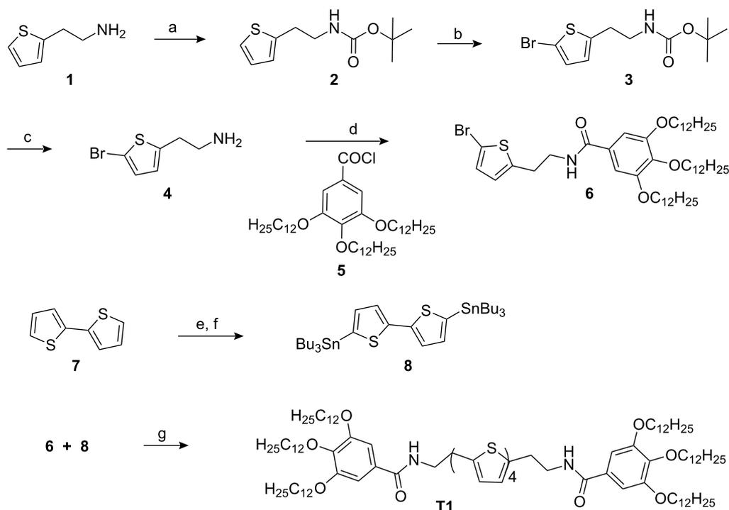
**Scheme 2:** Synthetic route to **T1**. Reagent and conditions: a) Boc anhydride,  $\text{CH}_2\text{Cl}_2$ , 6 h,  $0^\circ\text{C}$ –rt, 97%; b) NBS, DMF, rt, 12 h, 89%; c) TFA,  $\text{CH}_2\text{Cl}_2$ , rt, 4 h, 99%; d)  $\text{Et}_3\text{N}$ ,  $\text{CH}_2\text{Cl}_2$ ,  $0^\circ\text{C}$ –rt, 78%; e) BuLi, THF,  $0^\circ\text{C}$ , 1 h; f)  $\text{Bu}_3\text{SnCl}$ , rt, 12 h; g)  $\text{Pd}(\text{PPh}_3)_2\text{Cl}_2$ , DMF,  $80^\circ\text{C}$ , 8 h, 82%.
