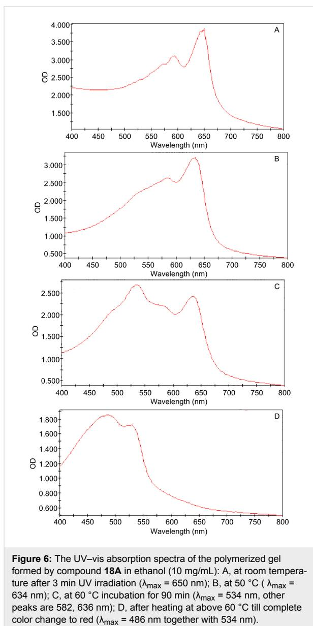
**Figure 6:** The UV–vis absorption spectra of the polymerized gel formed by compound **18A** in ethanol (10 mg/mL): A, at room temperature after 3 min UV irradiation ( $\lambda_{\text{max}} = 650$  nm); B, at 50 °C ( $\lambda_{\text{max}} = 634$  nm); C, at 60 °C incubation for 90 min ( $\lambda_{\text{max}} = 534$  nm, other peaks are 582, 636 nm); D, after heating at above 60 °C till complete color change to red ( $\lambda_{\text{max}} = 486$  nm together with 534 nm).
