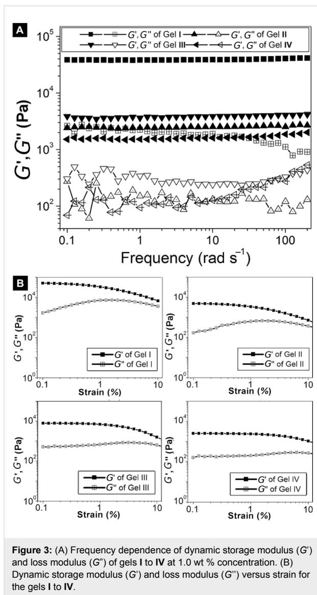
**Figure 3:** (A) Frequency dependence of dynamic storage modulus ( $G'$ ) and loss modulus ( $G''$ ) of gels I to IV at 1.0 wt % concentration. (B) Dynamic storage modulus ( $G'$ ) and loss modulus ( $G''$ ) versus strain for the gels I to IV.
