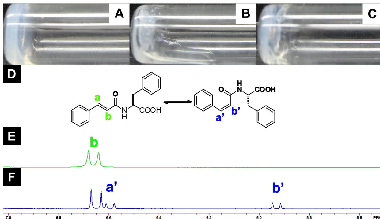
**Figure 1:** Optical images of (A) gel **IV** (1.5 wt %, pH = 4.6), (B) gel **IV** after UV irradiation (no aging), (C) gel **IV** after UV irradiation (aging 2 hours), (D) the structure of compound **6** in *trans*- and *cis*-isomers, (E) the NMR spectra of compound **6** before and (F) after UV irradiation for 2 hours.
