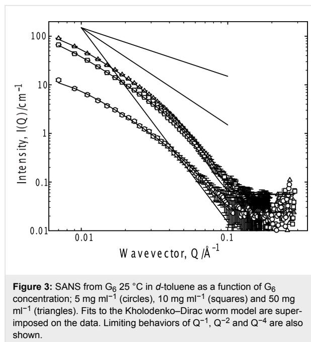
systems show a smooth transition from a simple  $Q^{-1}$  dependence indicative of rodlike structures, into the  $Q^{-4}$  expected for well-defined objects. This latter dependence ( $Q^{-4}$ ) is most evident in  $75\%$   $D_2O/d$ -ethanol, implying the structure in this case is more particle-like, consistent with the fragility (and appearance) of this gel. Clearly, existing frameworks for analyzing such data are not appropriate here.
