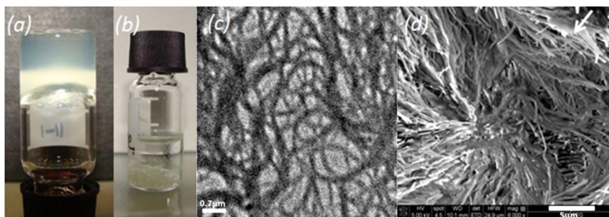
**Figure 2:** a) **R-3** gel in octane (5 mM); b) octane solution containing a mixture of **R-3** (2.5 mM) and **S-3** (2.5 mM) after cooling from 80 °C to room temperature; c) TEM image of the xerogel of **R-3** in octane; d) the surface morphology of the dried gel obtained from **R-3** in octane (15 mM) observed by FESEM.
