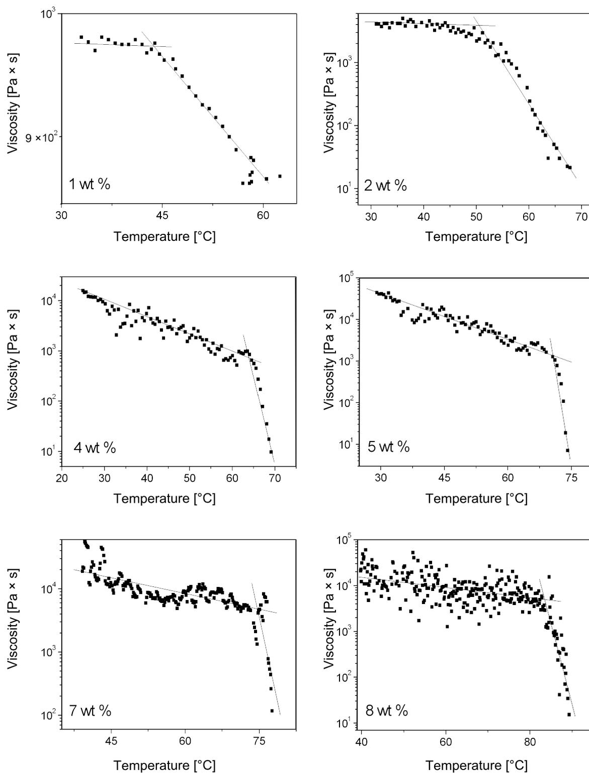
**Figure 3:** Dependence of viscosity of ODA-C/silicone oil gels on temperature at a shear stress of 1 Pa. From top left to bottom right: [ODA] = 1, 2, 4, 5, 7, and 8 wt %. Note that the viscosities of the 1 wt % sample have been plotted linearly and those at the other concentrations are plotted semi-logarithmically.
