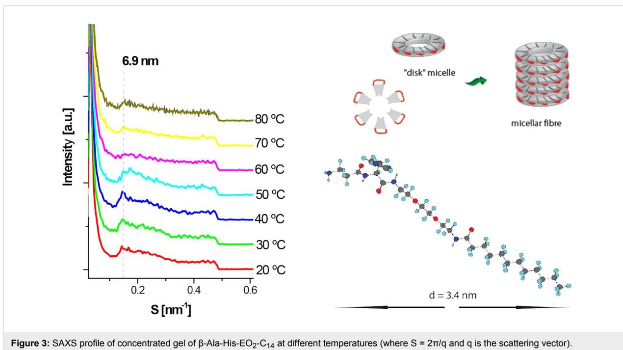
**Figure 3:** SAXS profile of concentrated gel of  $\beta$ -Ala-His-EO<sub>2</sub>-C<sub>14</sub> at different temperatures (where  $S = 2\pi/q$  and  $q$  is the scattering vector).
