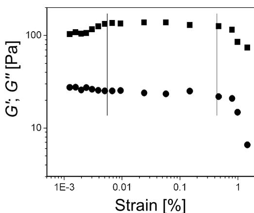
**Figure 5:** Amplitude sweep test of a 2 wt % **ODA-C**/silicone oil gel showing  $G'$  (■) and  $G''$  (●). The vertical lines mark the range of the linear viscoelastic region.
