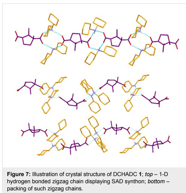
**Figure 7:** Illustration of crystal structure of DCHADC **1**; *top* – 1-D hydrogen bonded zigzag chain displaying SAD synthon; *bottom* – packing of such zigzag chains.
