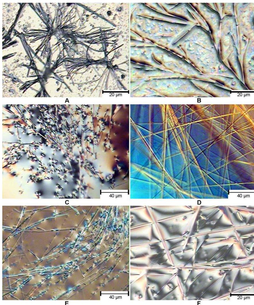
**Figure 3:** Optical micrographs of the gels formed by compound **9A** in hexane at 15 mg/mL (**A**, **B**), **9B** in DMSO/water (1:2) at 20 mg/mL (**C**, **D**), and **15B** in EtOH/H<sub>2</sub>O (1:2) at 4 mg/mL (**E**, **F**). The images were taken with gels containing solvents (not dried gels).
