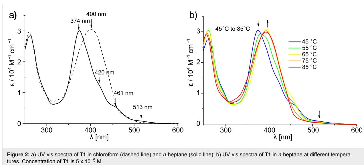
**Figure 2:** a) UV-vis spectra of **T1** in chloroform (dashed line) and *n*-heptane (solid line); b) UV-vis spectra of **T1** in *n*-heptane at different temperatures. Concentration of **T1** is  $5 \times 10^{-5}$  M.
