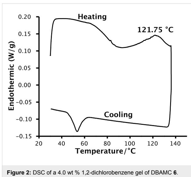
Figure 2: DSC of a 4.0 wt % 1,2-dichlorobenzene gel of DBAMC 6.
