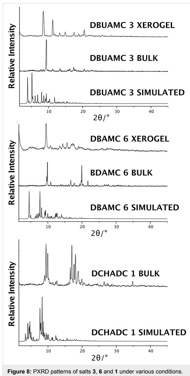
Figure 8: PXRD patterns of salts **3**, **6** and **1** under various conditions.
