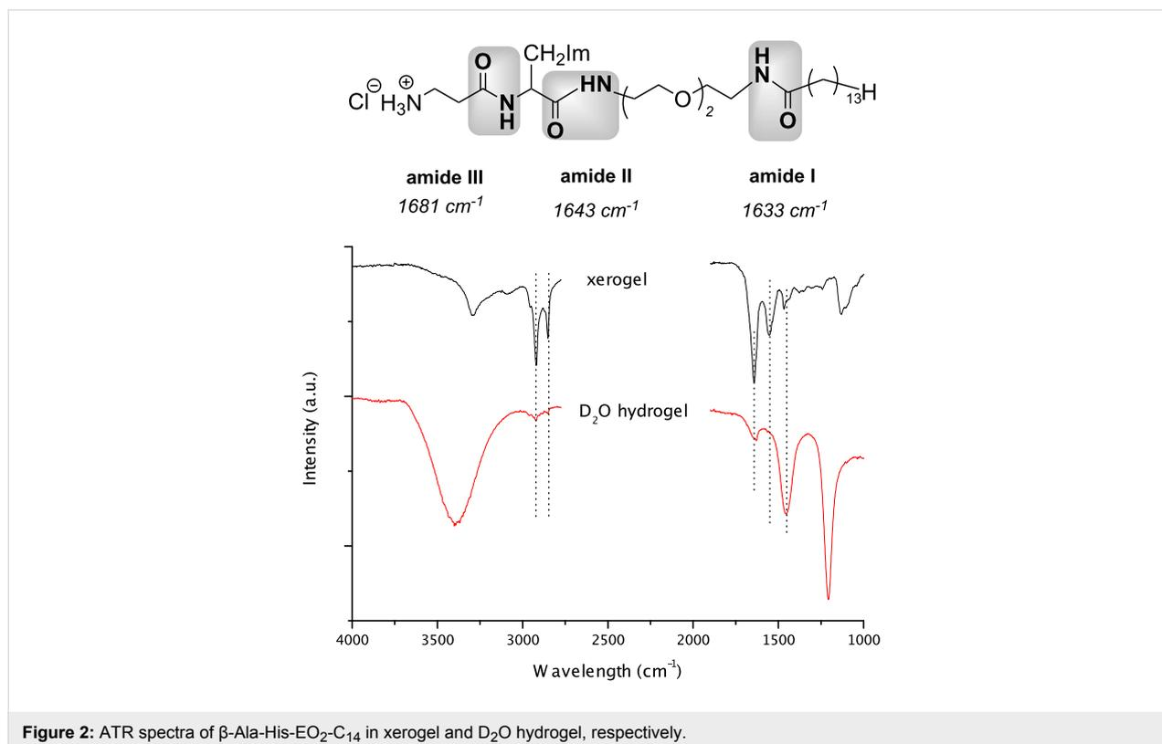
**Figure 2:** ATR spectra of  $\beta$ -Ala-His-EO<sub>2</sub>-C<sub>14</sub> in xerogel and D<sub>2</sub>O hydrogel, respectively.
