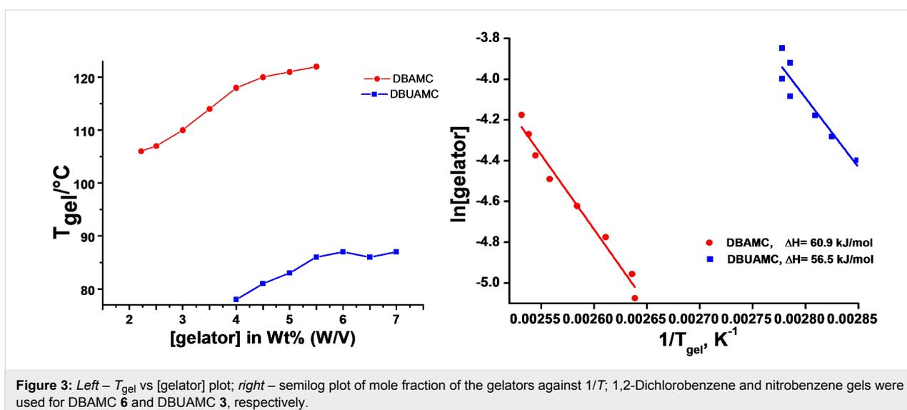
Figure 3: Left –  $T_{\text{gel}}$  vs [gelator] plot; right – semilog plot of mole fraction of the gelators against  $1/T$ ; 1,2-Dichlorobenzene and nitrobenzene gels were used for DBAMC 6 and DBUAMC 3, respectively.
