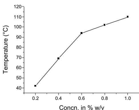
**Figure 6:** Gel melting profile of diethylaminolithocholyl iodide **1** gel in 1,2-dichlorobenzene.
