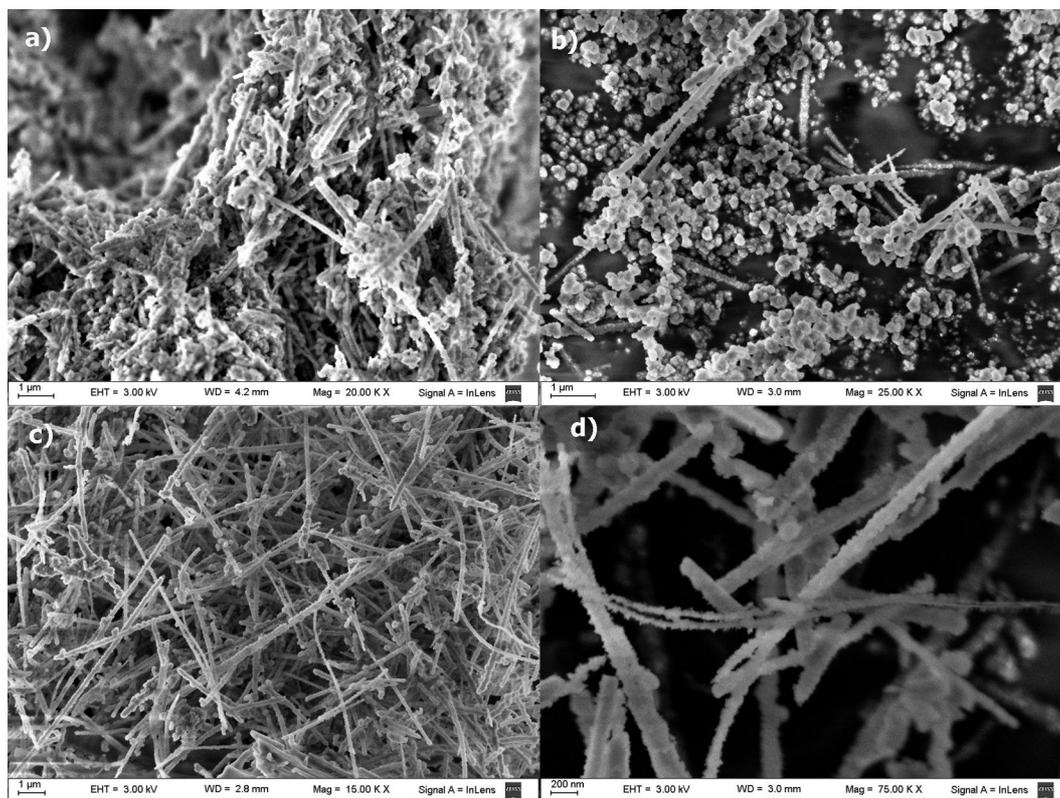
**Figure 7:** SEM images of nanostructured silica obtained from gels of LMOG **1** under the following conditions: 0.5 mL of dioxane, 0.1 mL TEOS, 35 mg of **1**, and (a) 3  $\mu\text{L}$  of benzylamine and 15  $\mu\text{L}$  of water, (b) 3  $\mu\text{L}$  of benzylamine and 3  $\mu\text{L}$  of water (c,d) 1  $\mu\text{L}$  of benzylamine and 15  $\mu\text{L}$  of water.
