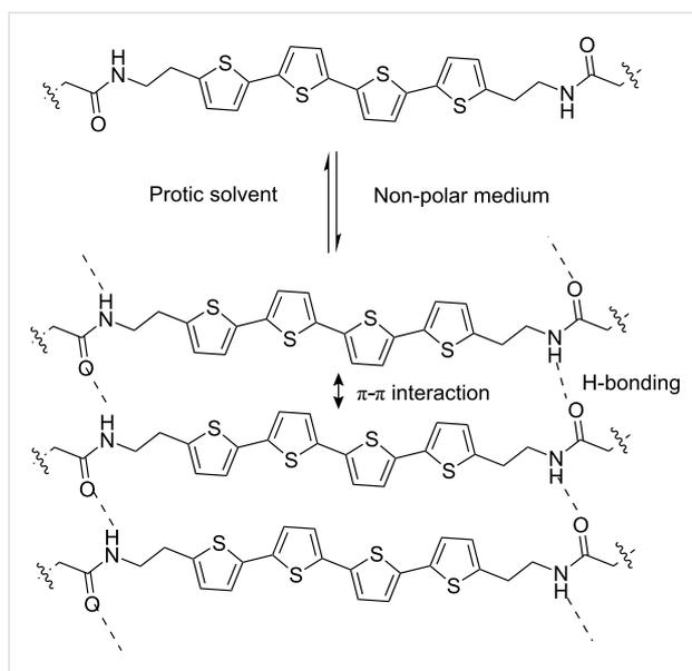
**Scheme 3:** Proposed mode of self-assembly of **T1**.
