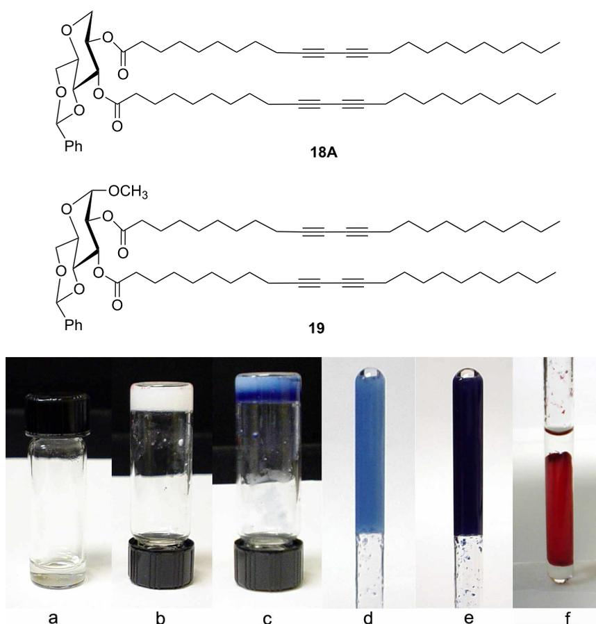
**Figure 4:** An ethanol gel formed by compound **18A** at <10 mg/mL. a) A clear solution when heated above 70 °C; b) a stable gel after cooling to room temperature; c) a blue gel after illuminating with UV lamp from the top of the vial in b; d) a light blue gel inside quartz tube after UV treatment for 1 min; e) a dark blue gel in quartz tube after UV treatment for 3 min; f) the blue gel in e) turned red after heating.
