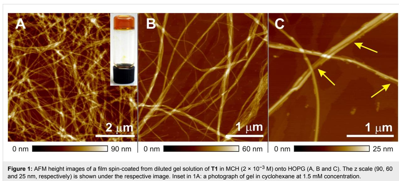
**Figure 1:** AFM height images of a film spin-coated from diluted gel solution of **T1** in MCH ( $2 \times 10^{-3}$  M) onto HOPG (A, B and C). The z scale (90, 60 and 25 nm, respectively) is shown under the respective image. Inset in 1A: a photograph of gel in cyclohexane at 1.5 mM concentration.
