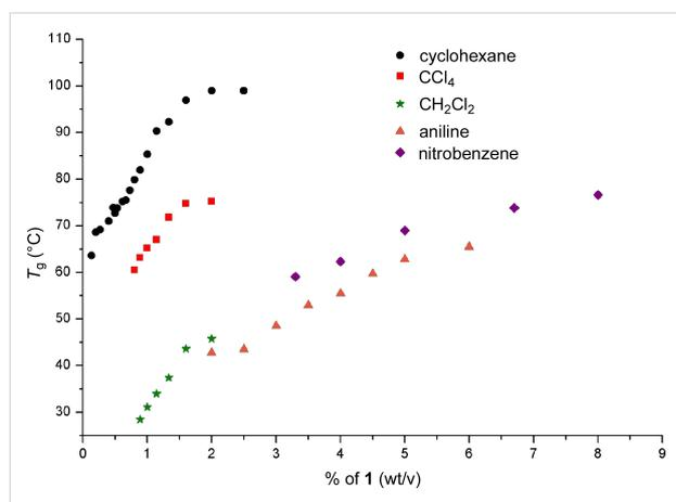
**Figure 3:**  $T_g$ -vs-concentration plots for gels of **1**.
