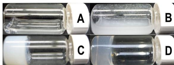
**Figure 2:** The optical images of (A) solution of **6** (2 wt %, pH = 9.0), (B) suspension of **6** (2 wt %, pH = 6.5), (C) opaque gel of **6** (2 wt %, pH = 4.6), (D) transparent gel of **6** (2 wt %, pH = 4.6, aging for 10 days).
