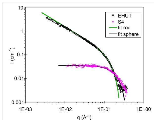
**Figure 4:** SANS intensity versus scattering vector for 12 mM solutions of **EHUT** or **S4** in  $d_8$ -toluene, at 22 °C. The plain curves are fits according to a model for infinitely long rigid rods of diameter 26 Å (green), or for spheres of diameter 22 Å (black).
