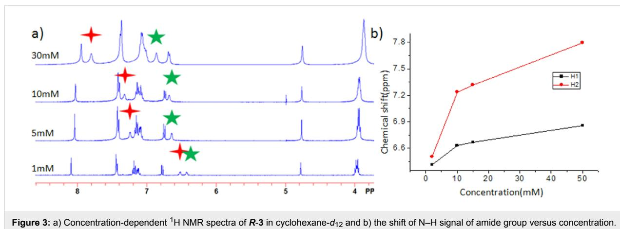
**Figure 3:** a) Concentration-dependent <sup>1</sup>H NMR spectra of **R-3** in cyclohexane-*d*<sub>12</sub> and b) the shift of N-H signal of amide group versus concentration.
