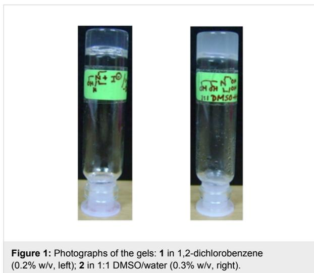
Figure 1: Photographs of the gels: **1** in 1,2-dichlorobenzene (0.2% w/v, left); **2** in 1:1 DMSO/water (0.3% w/v, right).
