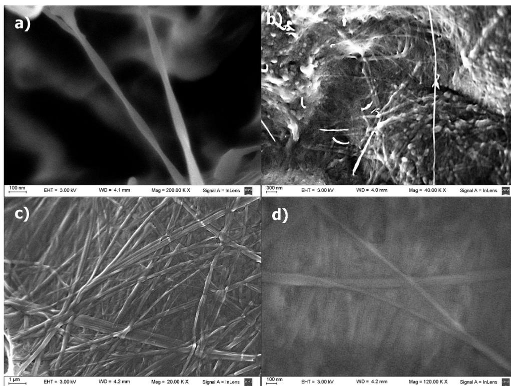
Figure 4: SEM images of xerogels from a,b) dichloromethane, and c,d) from dioxane.
