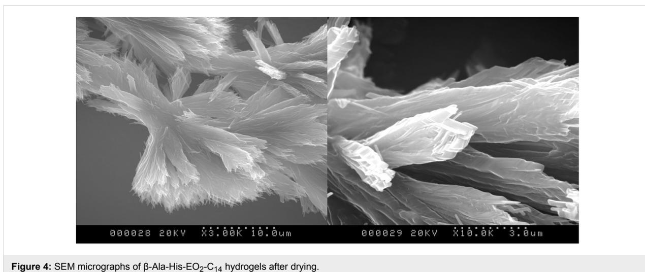
**Figure 4:** SEM micrographs of  $\beta$ -Ala-His-EO<sub>2</sub>-C<sub>14</sub> hydrogels after drying.
