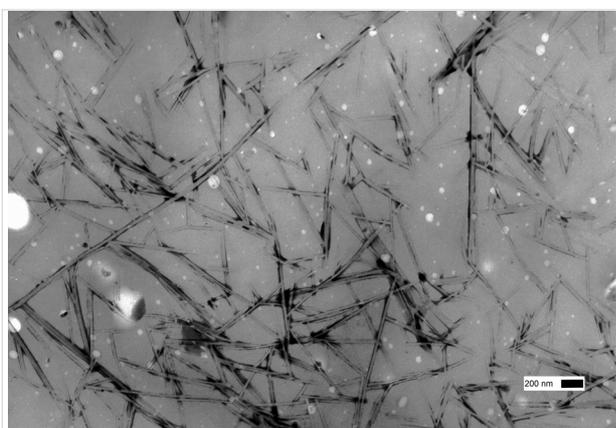
**Figure 3:** TEM images (PWK staining) of: *(S,R)*-**1a** H<sub>2</sub>O/DMSO gel.
