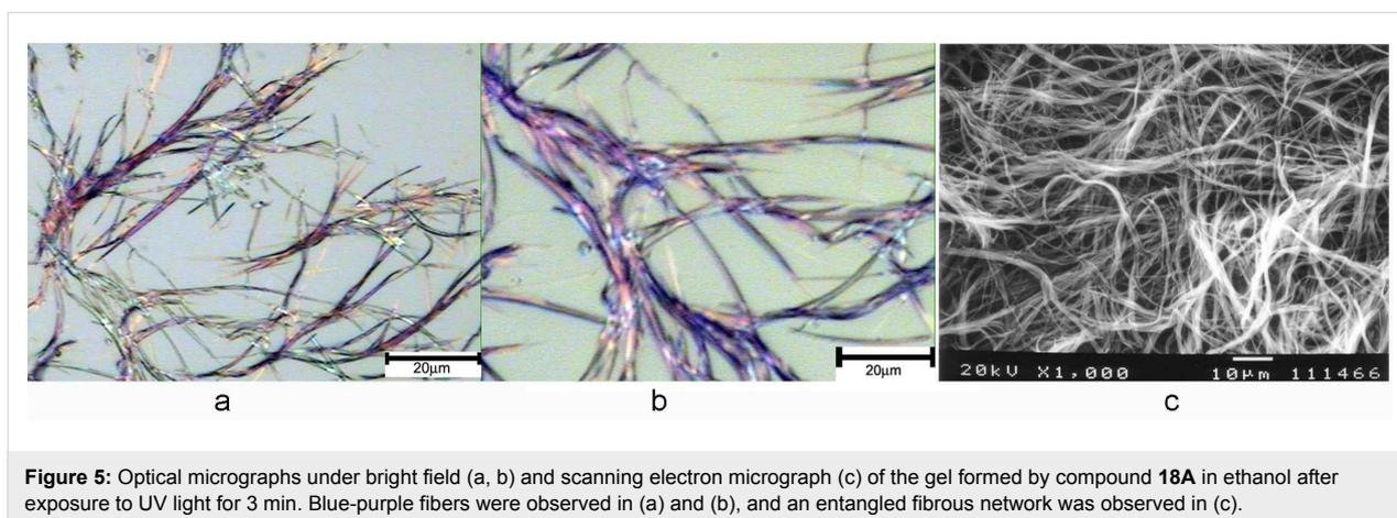
**Figure 5:** Optical micrographs under bright field (a, b) and scanning electron micrograph (c) of the gel formed by compound **18A** in ethanol after exposure to UV light for 3 min. Blue-purple fibers were observed in (a) and (b), and an entangled fibrous network was observed in (c).
