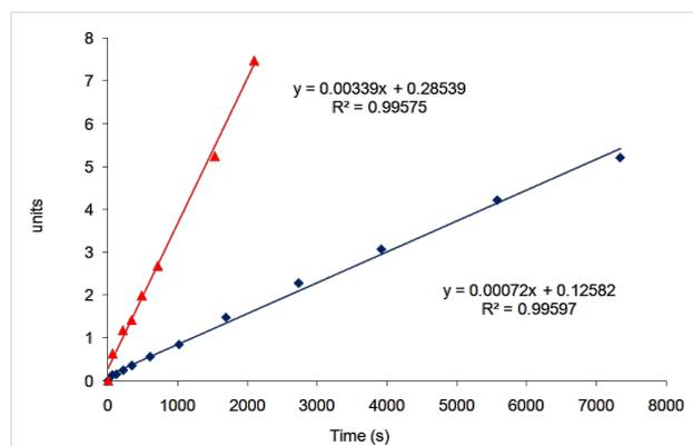
**Figure 2:** Second-order kinetics plot for the addition of TMSCN to benzaldehyde at 0 °C catalysed by complex **2** in dichloromethane (red) and propylene carbonate (blue). The units for the vertical scale are  $\ln[(B_0A_t)/(B_tA_0)]/(A_0 - B_0)$ , where A = [PhCHO], B = [Me<sub>3</sub>SiCN], and the subscripts 0 and t refer to initial concentrations and concentrations at time t, respectively.
