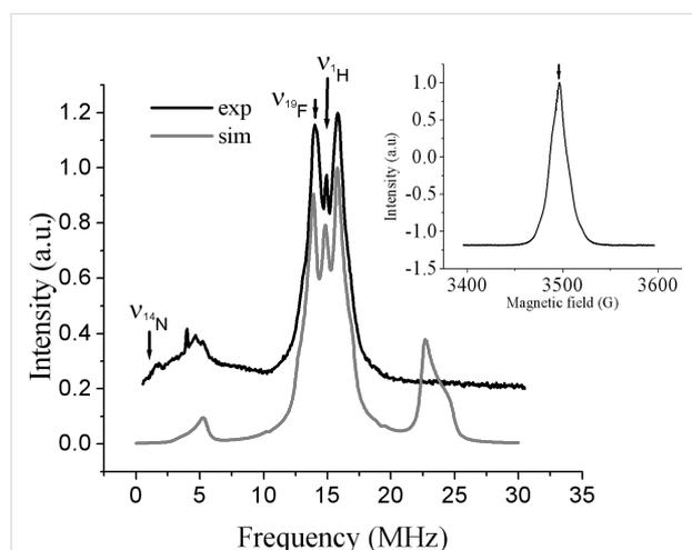
**Figure 7:** Experimental and simulated Davies ENDOR spectrum after the Ga-promoted reaction of azide **6** recorded at 50 K. The inset shows the field-swept EPR spectrum with an arrow indicating the magnetic field position of the ENDOR experiment.
