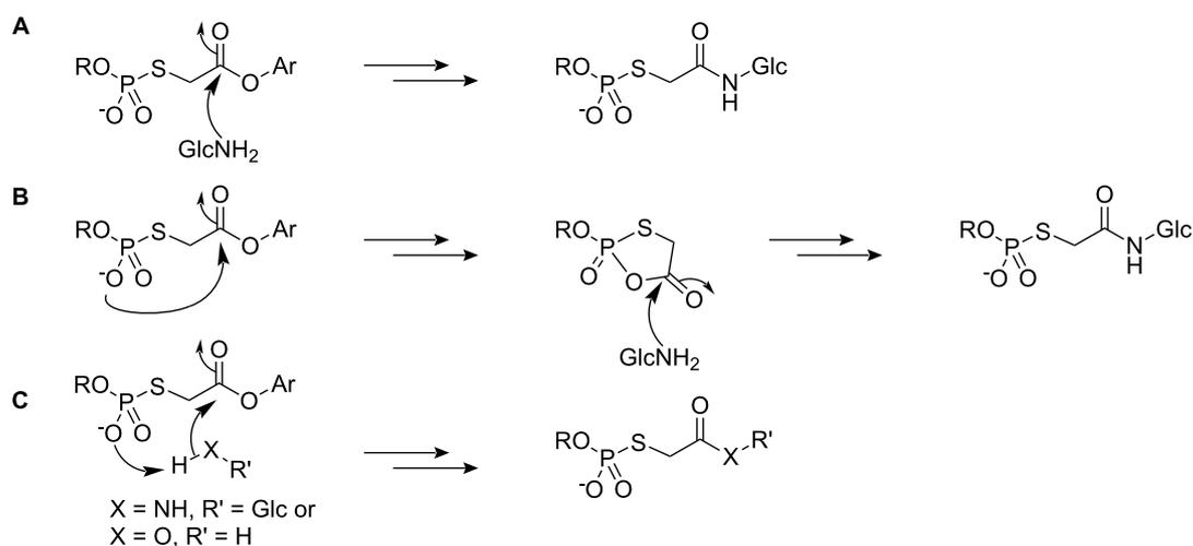
**Scheme 6:** (A) Direct aminolysis of the ester carbonyl group; (B) intramolecular nucleophilic catalysis of ester cleavage followed by aminolysis of the mixed phosphoric-carboxylic anhydride; (C) intramolecular general base-assisted attack by amine or water.
