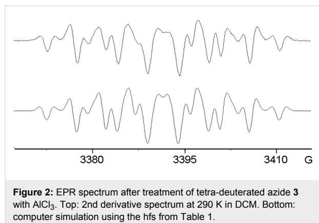
**Figure 2:** EPR spectrum after treatment of tetra-deuterated azide **3** with  $AlCl_3$ . Top: 2nd derivative spectrum at 290 K in DCM. Bottom: computer simulation using the hfs from Table 1.
