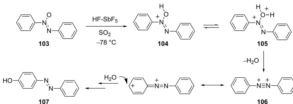
**Scheme 22:** Proposed mechanism for the Wallach rearrangement.
