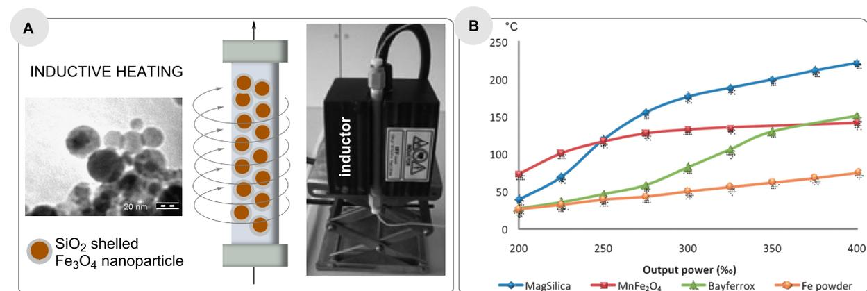
**Figure 4:** A. Flow reactor filled with magnetic nanostructured particles (MagSilica™) and packed bed reactor embedded in inductor (right); B. heating profile of different materials exposed to an electromagnetic field. Heating profiles of MagSilica™, MnFe<sub>2</sub>O<sub>4</sub>, Bayferrox™, and iron powder.
