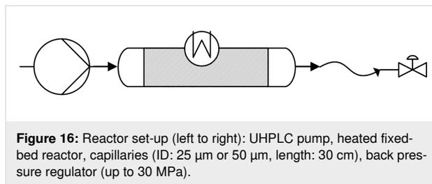
**Figure 16:** Reactor set-up (left to right): UHPLC pump, heated fixed-bed reactor, capillaries (ID: 25  $\mu\text{m}$  or 50  $\mu\text{m}$ , length: 30 cm), back pressure regulator (up to 30 MPa).
