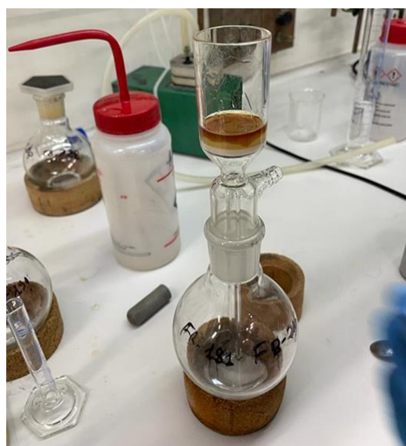
Figure 2: The purification process of a brownish isocyanide on a short silica pad.
