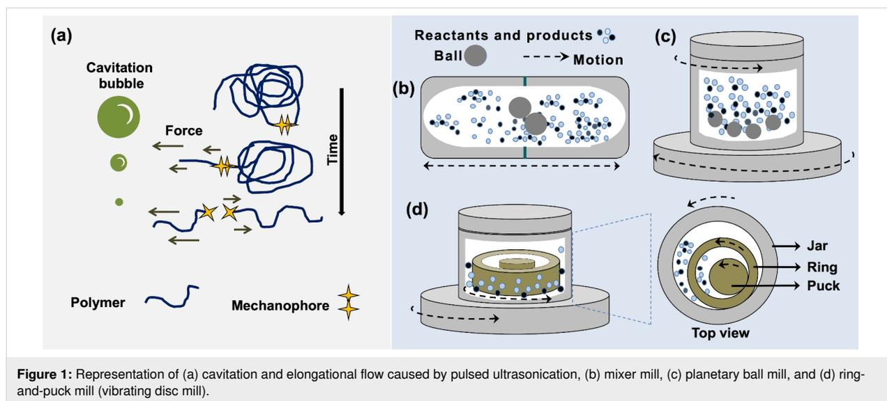
**Figure 1:** Representation of (a) cavitation and elongational flow caused by pulsed ultrasonication, (b) mixer mill, (c) planetary ball mill, and (d) ring-and-puck mill (vibrating disc mill).
