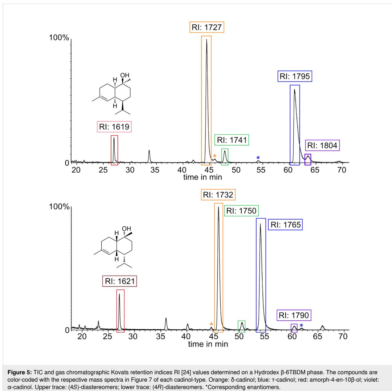
**Figure 5:** TIC and gas chromatographic Kovats retention indices RI [24] values determined on a Hydrodex  $\beta$ -6TBDM phase. The compounds are color-coded with the respective mass spectra in Figure 7 of each cadinol-type. Orange:  $\delta$ -cadinol; blue:  $\tau$ -cadinol; red: amorph-4-en-10 $\beta$ -ol; violet:  $\alpha$ -cadinol. Upper trace: (4*S*)-diastereomers; lower trace: (4*R*)-diastereomers. \*Corresponding enantiomers.
