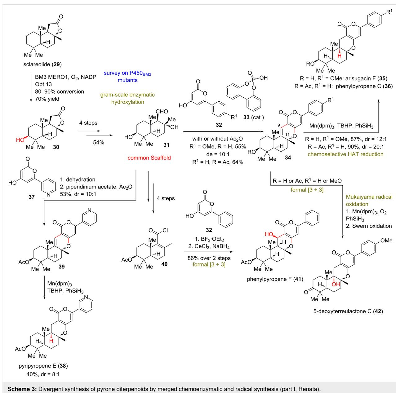
**Scheme 3:** Divergent synthesis of pyrone diterpenoids by merged chemoenzymatic and radical synthesis (part I, Renata).
