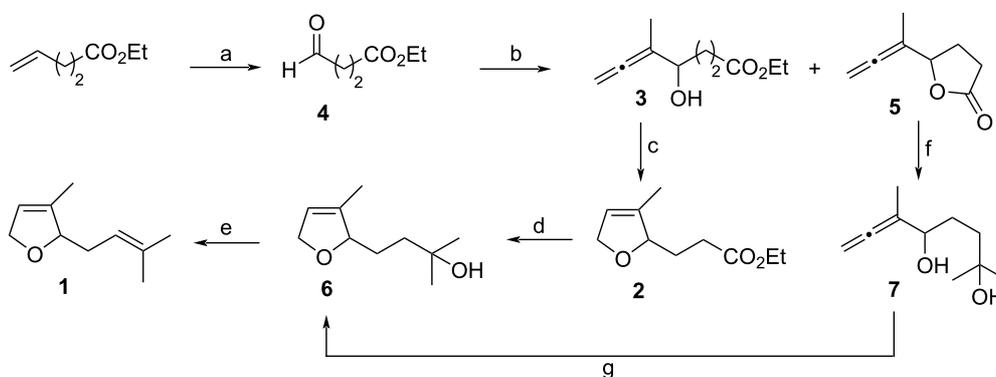
**Scheme 2:** Synthesis of dihydrofuran-monoterpene **1**. a) i. O<sub>3</sub>, –78 °C; ii. PPh<sub>3</sub>, rt, 76%; b) 1-bromobut-2-yne, CpTiCl<sub>3</sub>, Mn and THF (**3**: 71–81%, **5**: 0–10%); c) AgNO<sub>3</sub>, Me<sub>2</sub>CO, 88%; d) MeMgBr, Et<sub>2</sub>O, 90%; e) Amberlyst<sup>®</sup>-15, DCM, 74%; f) MeMgBr, Et<sub>2</sub>O, 83%; g) AgNO<sub>3</sub>, Me<sub>2</sub>CO, 75%.
