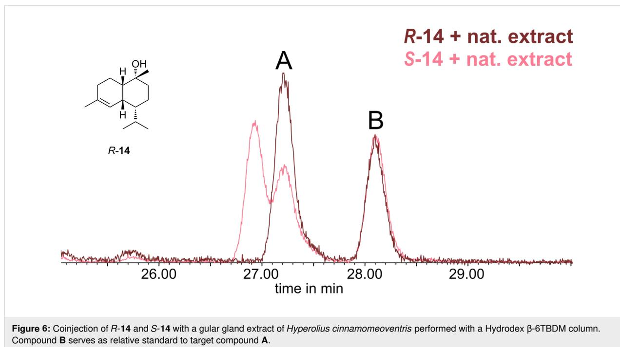
**Figure 6:** Coinjection of *R-14* and *S-14* with a gular gland extract of *Hyperolius cinnamomeoventris* performed with a Hydrodex  $\beta$ -6TBDM column. Compound **B** serves as relative standard to target compound **A**.
