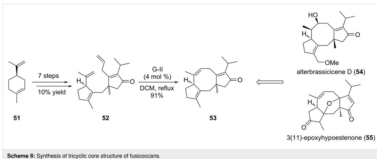
**Scheme 8:** Synthesis of tricyclic core structure of fusicoccans.
