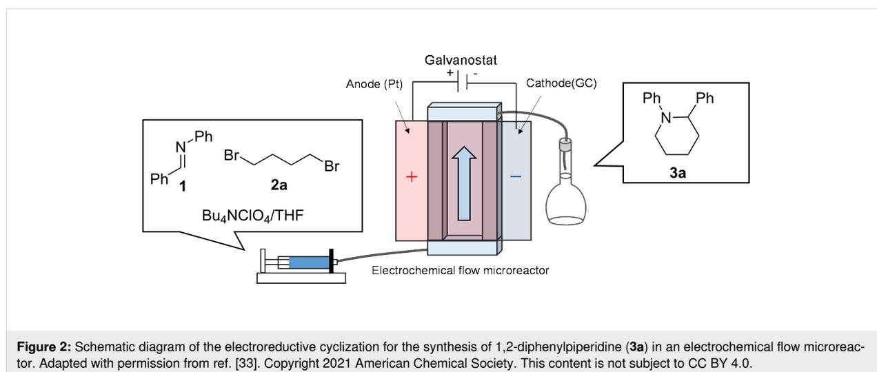
**Figure 2:** Schematic diagram of the electroreductive cyclization for the synthesis of 1,2-diphenylpiperidine (**3a**) in an electrochemical flow microreactor. Adapted with permission from ref. [33]. Copyright 2021 American Chemical Society. This content is not subject to CC BY 4.0.
