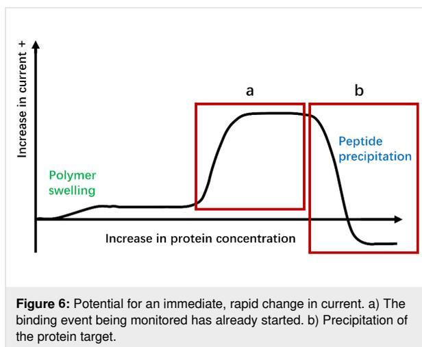
binding constant that is greater than either of the individual interactions. Alternatively, the surface-bound substrate could lead to avidity events where more than one of the ligands binds to the protein at the same time by taking advantage of allosteric binding sites.
