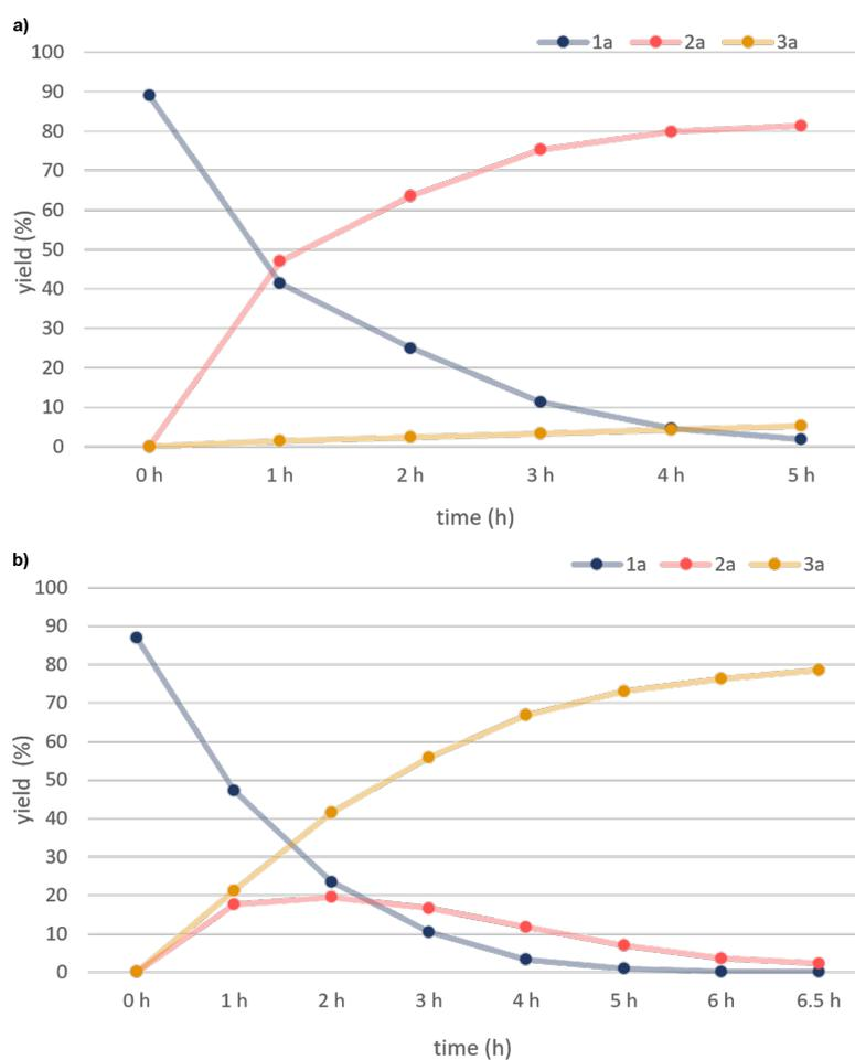
**Figure 2:** Reaction profile of the electrochemical hydrogenation of **1a** with a PEM reactor using a) Pd/C and b) Ir/C cathode catalyst. The yield of **2a** and **3a** and the recovery of **1a** are shown in red, brown, and blue, respectively.
