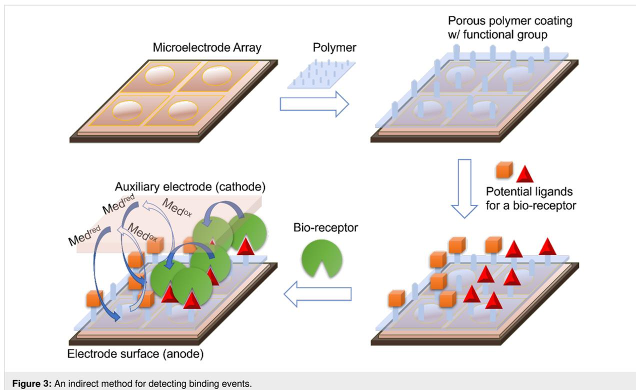
**Figure 3:** An indirect method for detecting binding events.
