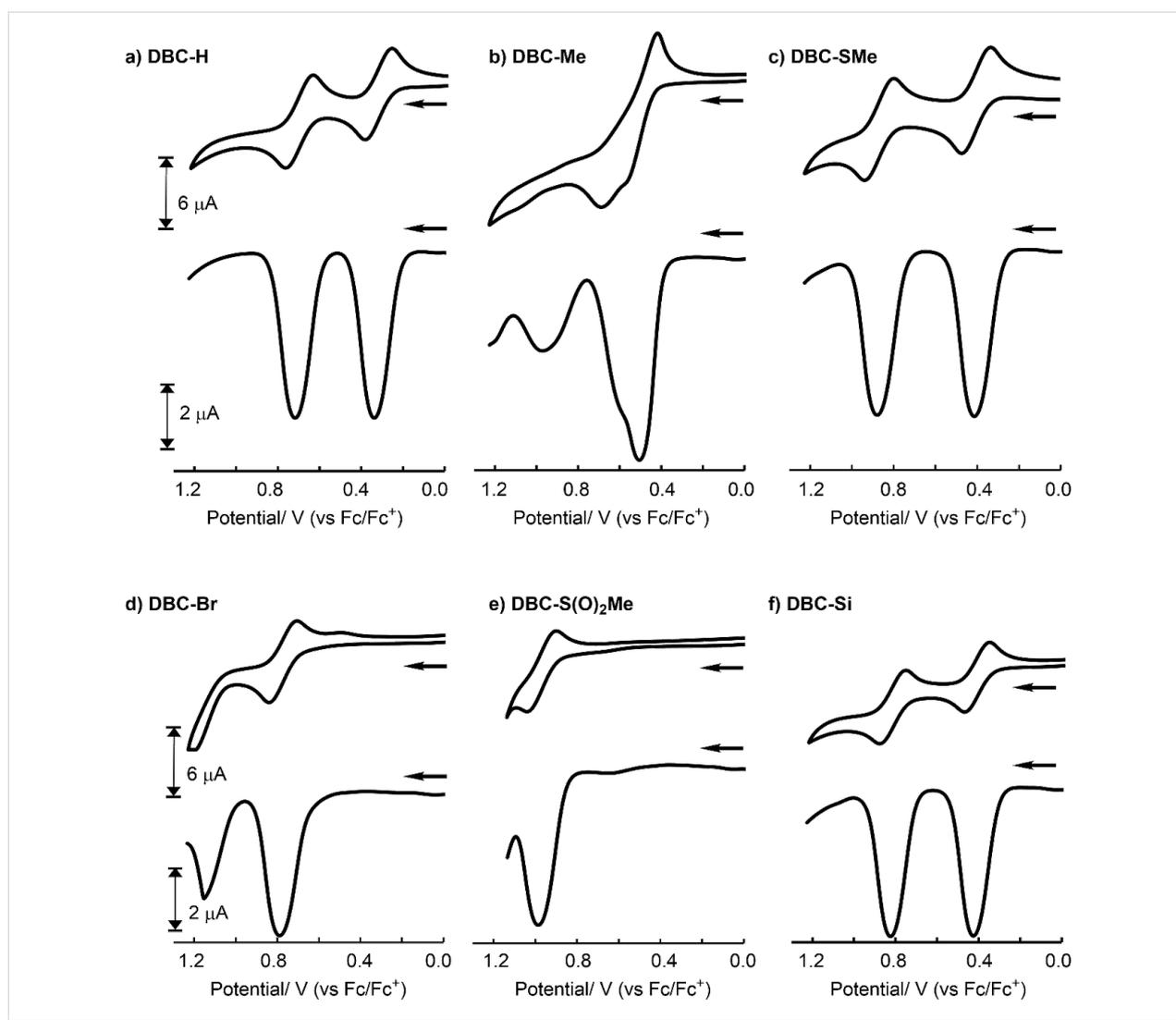
**Figure 2:** CVs and SWVs of DBC derivatives in  $\text{CH}_2\text{Cl}_2$  ( $\approx 1.0 \times 10^{-3}$  M, see Supporting Information File 1 for details) including  $5.0 \times 10^{-2}$  M  $\text{NBu}_4\text{BF}_4$  as a supporting electrolyte under Ar at 298 K (working electrode: Pt, scan rate: 100 mV/s and 40 mV/s for CV and SWV measurements, respectively).
