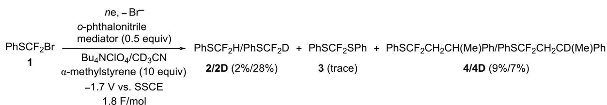
**Scheme 9:** Indirect cathodic reduction of compound **1** in  $\text{CD}_3\text{CN}$ .
