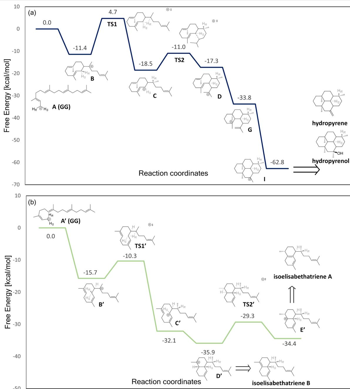
**Figure 2:** Free energy profile of hydroppyrene cation (a), and IE cation (b) formation in the gas phase. The free energy of cation **A** and **A'** is set to zero. Bonds breaking/forming in the transition states are marked by dotted lines. All calculations were performed in the gas phase at the M06-2X/6-31G+(d,p) level of theory.
