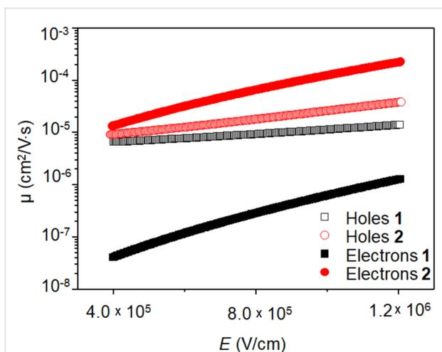
**Figure 7:** Charge carrier mobility as a function of the applied electric field obtained for the hole-only and electron-only devices of compounds **1** and **2**.
