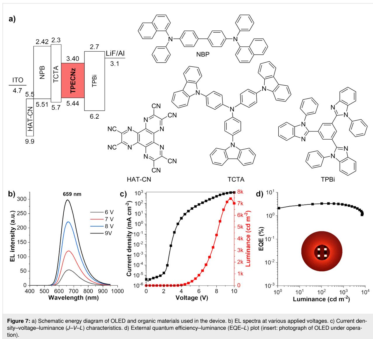
**Figure 7:** a) Schematic energy diagram of OLED and organic materials used in the device. b) EL spectra at various applied voltages. c) Current density–voltage–luminance ( $J$ – $V$ – $L$ ) characteristics. d) External quantum efficiency–luminance (EQE– $L$ ) plot (insert: photograph of OLED under operation).
