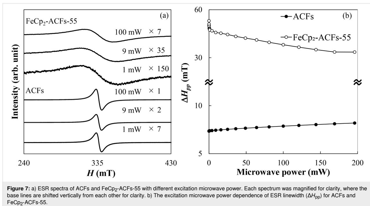
**Figure 7:** a) ESR spectra of ACFs and  $\text{FeCp}_2$ -ACFs-55 with different excitation microwave power. Each spectrum was magnified for clarity, where the base lines are shifted vertically from each other for clarity. b) The excitation microwave power dependence of ESR linewidth ( $\Delta H_{pp}$ ) for ACFs and  $\text{FeCp}_2$ -ACFs-55.
