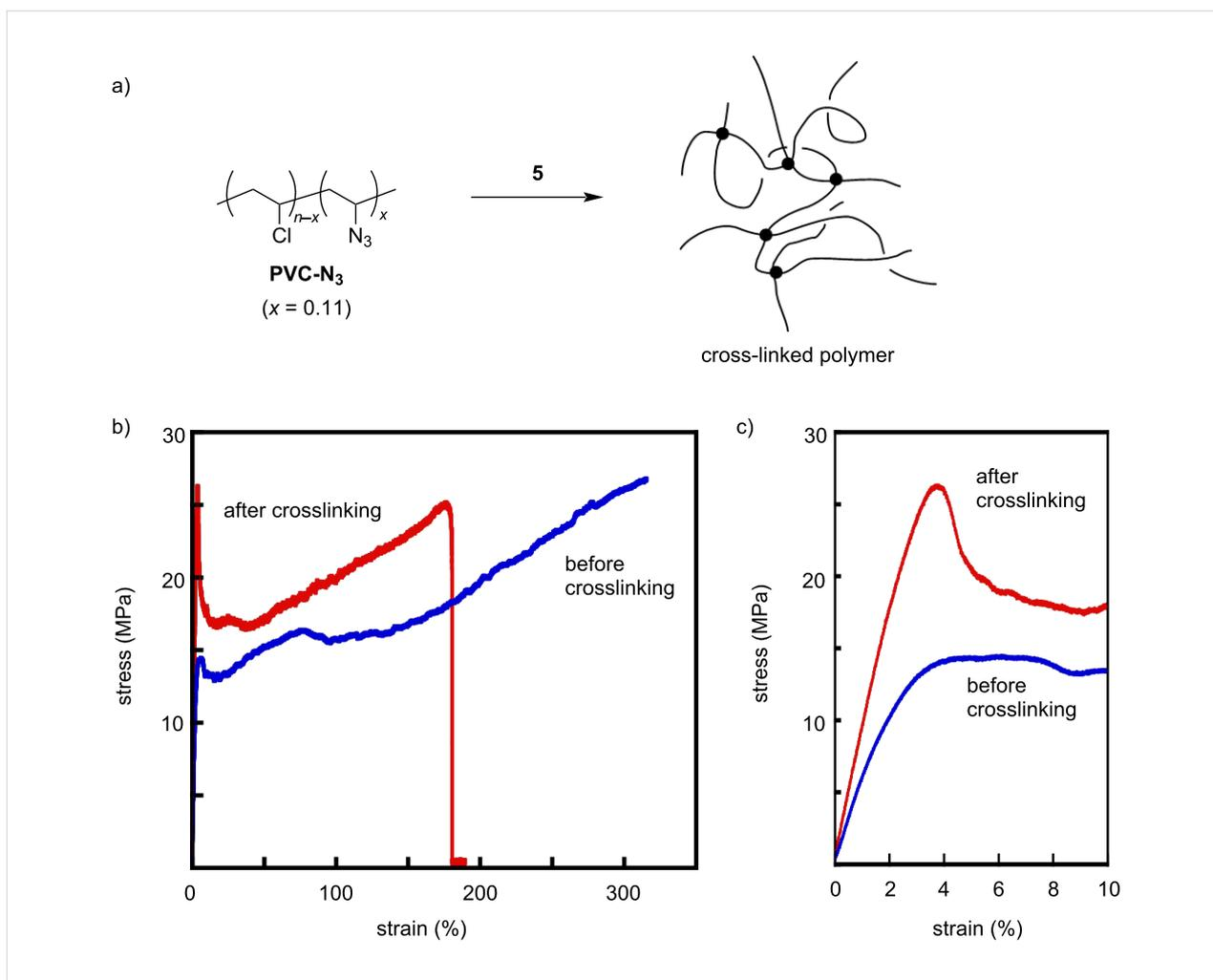
**Figure 6:** (a) Crosslinking reaction of PVC-N<sub>3</sub> ( $x = 0.11$ ) with compound 5. (b,c) Strain-stress curves of PVC-N<sub>3</sub> before (blue) and after (red) crosslinking.
