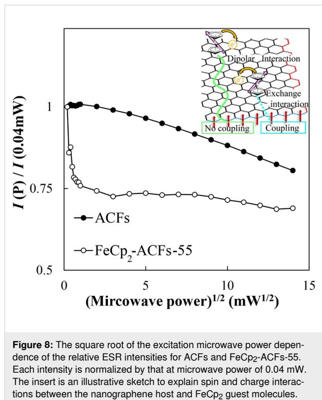
**Figure 8:** The square root of the excitation microwave power dependence of the relative ESR intensities for ACFs and FeCp<sub>2</sub>-ACFs-55. Each intensity is normalized by that at microwave power of 0.04 mW. The insert is an illustrative sketch to explain spin and charge interactions between the nanographene host and FeCp<sub>2</sub> guest molecules.
