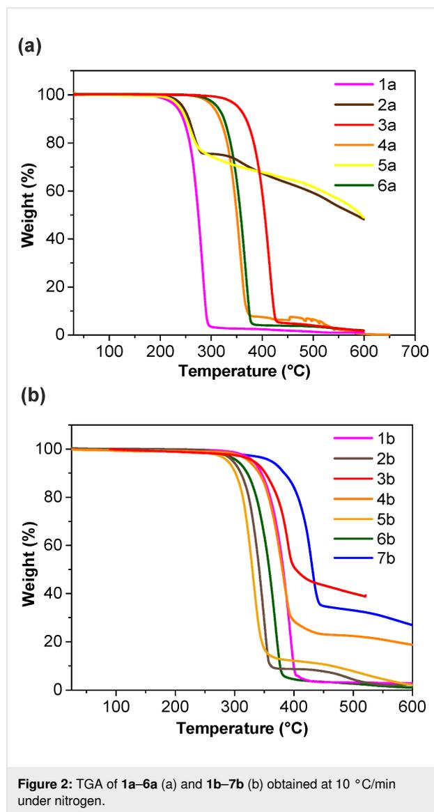
**Figure 2:** TGA of **1a–6a** (a) and **1b–7b** (b) obtained at 10 °C/min under nitrogen.
