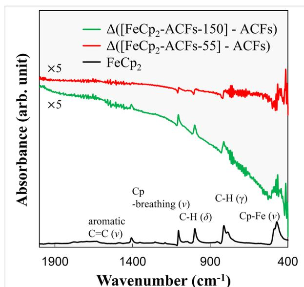
**Figure 5:** The raw infrared spectrum for FeCp<sub>2</sub> (black) and differential absorbance spectra for FeCp<sub>2</sub>-ACFs-55 (red) and FeCp<sub>2</sub>-ACFs-150 (green) after subtracting the ACFs spectrum as a background signal. The subtracted spectra are magnified five times, where the base lines are shifted vertically from each other for clarity. Raw spectra for FeCp<sub>2</sub>-ACFs-55 and FeCp<sub>2</sub>-ACFs-150 are shown in Supporting Information File 1.
