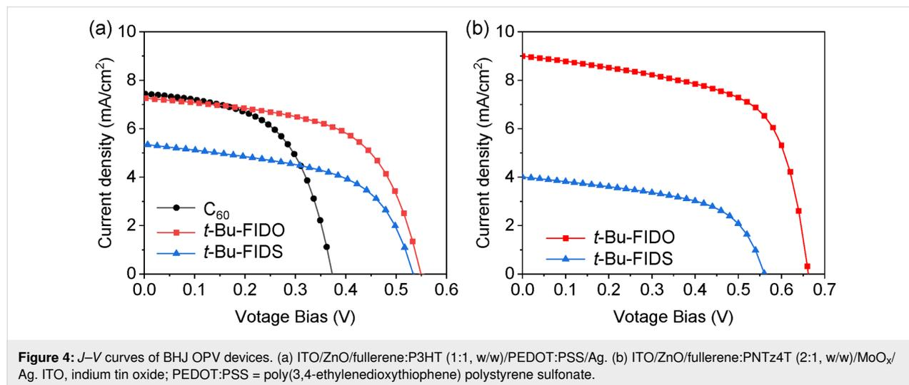
**Figure 4:**  $J$ – $V$  curves of BHJ OPV devices. (a) ITO/ZnO/fullerene:P3HT (1:1, w/w)/PEDOT:PSS/Ag. (b) ITO/ZnO/fullerene:PNTz4T (2:1, w/w)/MoO<sub>x</sub>/Ag. ITO, indium tin oxide; PEDOT:PSS = poly(3,4-ethylenedioxythiophene) polystyrene sulfonate.
