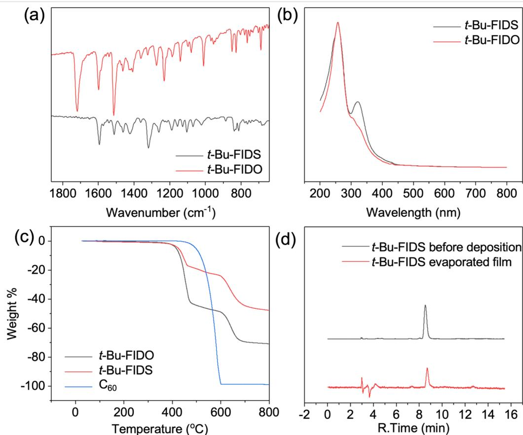
**Figure 1:** Characterization data. (a) FTIR spectra of *t*-Bu-FIDO and *t*-Bu-FIDS. (b) UV-vis spectra of fullerene derivatives normalized at 270 nm. (c) Vacuum TGA curves of *t*-Bu-FIDO (black), *t*-Bu-FIDS (red), and C<sub>60</sub> (blue). The measurements were conducted under 0.1 Pa. (d) HPLC analyses before deposition of *t*-Bu-FIDS (black) and of toluene used to rinse the evaporated film of *t*-Bu-FIDS (red).
