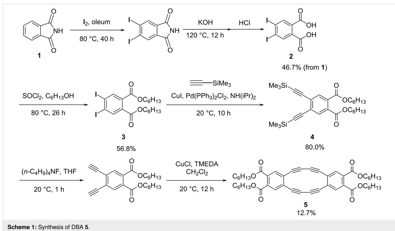
1-hexanol yielded compound **3** in 56.8% yield and the subsequent Sonogashira coupling with trimethylsilylacetylene provided compound **4** in 80.0%. Silyl deprotection with (*n*-C<sub>4</sub>H<sub>9</sub>)<sub>4</sub>NF in THF followed by acetylenic oxidative dimerization under Hay conditions produced the desired DBA **5** in 12.7% yield. It should be noted that a thermodynamically more stable trimeric macrocycle was also formed in 17.7%, but it was
