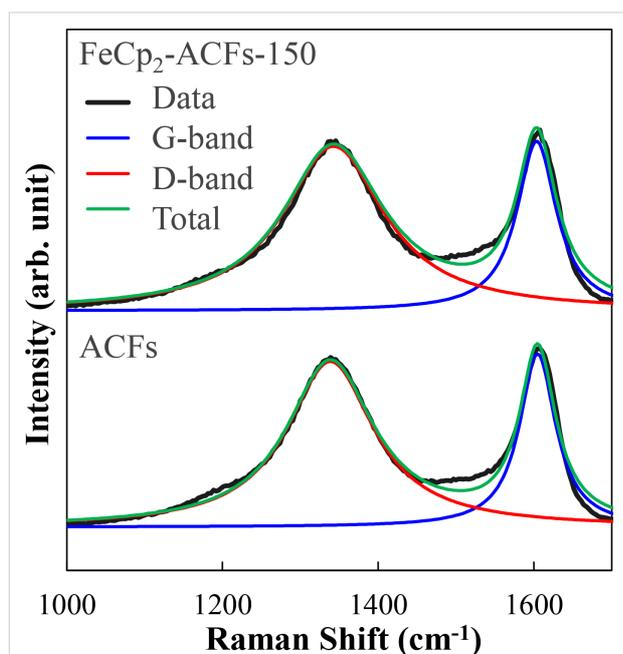
**Figure 4:** Raman spectra for ACFs and FeCp<sub>2</sub>-ACFs-150. Each raw data (black) was fitted to the G-band (blue) and D-band (red) components, resulting in the total curve (green). The base lines of the spectra are shifted vertically from each other for clarity.
