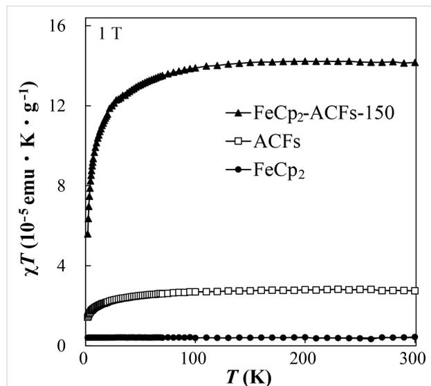
**Figure 6:** The temperature ( $T$ ) dependence of the magnetic susceptibility  $\chi$  for FeCp<sub>2</sub>-ACFs-150, ACFs, and FeCp<sub>2</sub> measured at 1 T, where the vertical axis denotes the  $\chi$  multiplied by  $T$ . The temperature-independent diamagnetic contribution to the magnetic susceptibility is subtracted.
