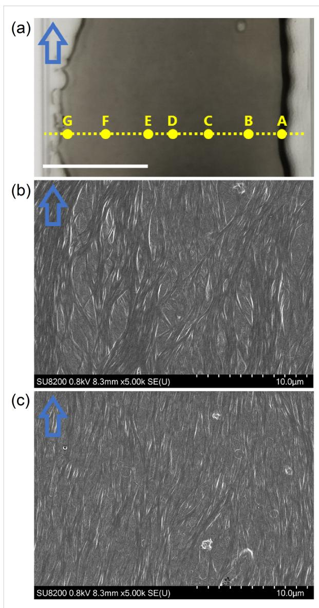
**Figure 5:** (a) Photograph of the DWCNT film. Thicknesses were measured at 7 spots along the yellow dashed line. Scale bar is 1 cm. SEM image at spot (b) A and (c) D. Blue outlined arrows indicate the shear direction of bar-coating.
