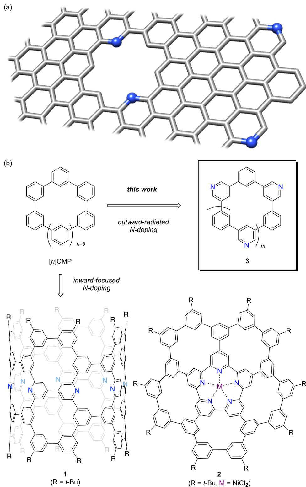
**Figure 1:** Nitrogen-doped nanocarbons. (a) Schematic illustration of pyridinic nitrogen atoms installed at the interior and periphery of a graphene sheet. (b) Phenine nanocarbon molecules with nitrogen dopants.
