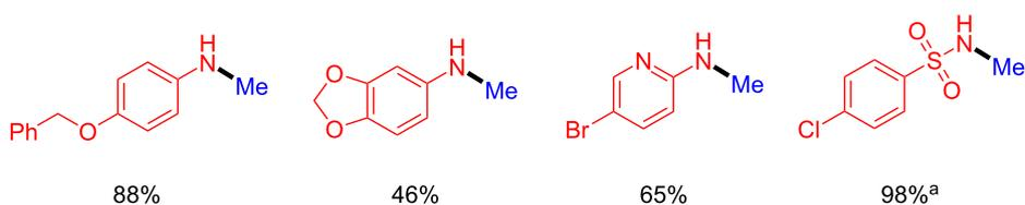
**Scheme 5:** C–N-Bond formation with amines and methanol using PN<sup>3</sup>P–Mn complex **Mn3** reported by Sortais et al. [36]. <sup>a</sup>1.2 Equiv *t*-BuOK, 60 h.
