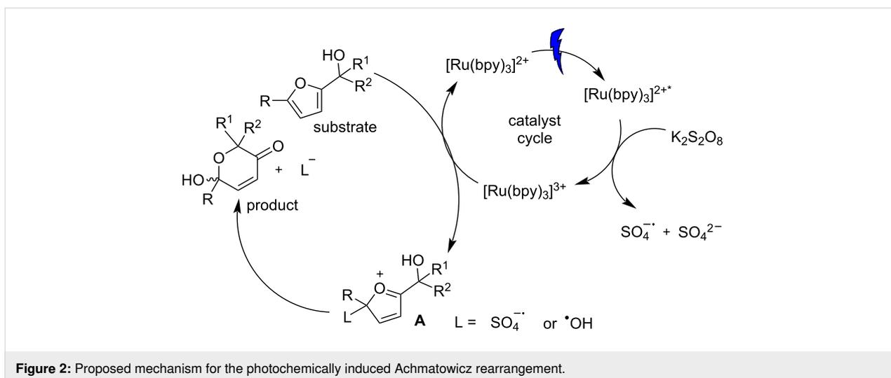
of sulfate and a sulfate radical. SET from furfuryl alcohol closes the catalytic cycle of the PC and an intermediate A is generated with L (L =  $\text{SO}_4^{\cdot-}$  or  $\text{OH}$ ). The Achmatowicz product is formed by addition of water to oxocarbenium intermediate A followed by elimination of L.
