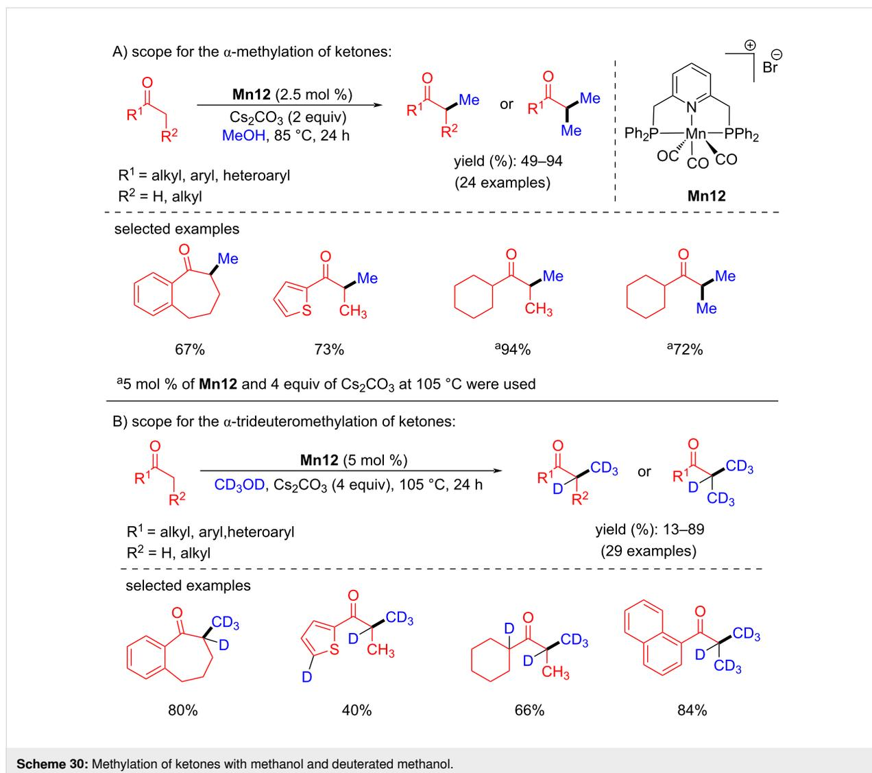
Scheme 30: Methylation of ketones with methanol and deuterated methanol.
