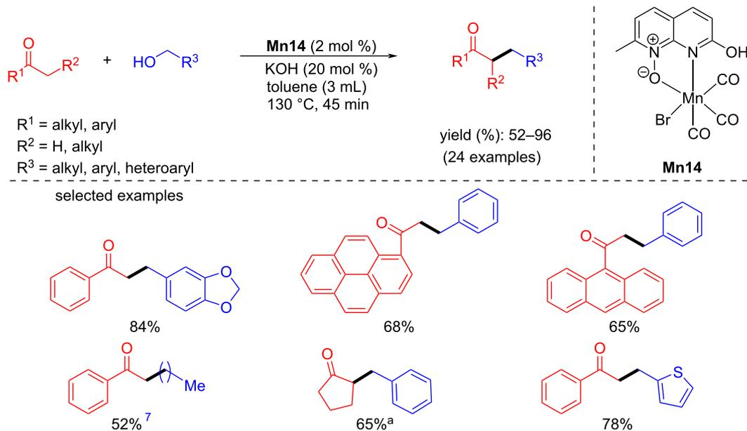
**Scheme 38:** Naphthyridine-*N*-oxide manganese complex **Mn14** applied for the alkylation of ketones with alcohols. <sup>a</sup>Reaction time was 6 h.
