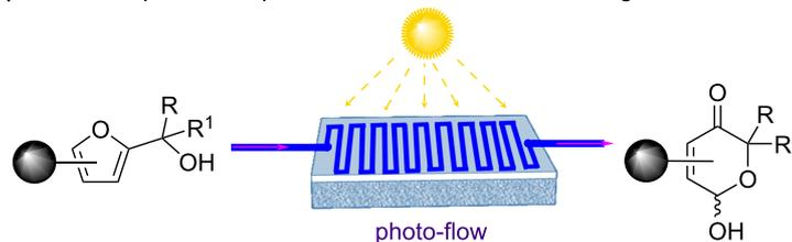
novel photo-flow reactor, safe and green process, sunlight as a green energy source, broad substrate scope, 16 examples with good to excellent yields (51–85%).
