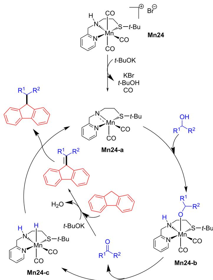
**Scheme 80:** Proposed mechanism for the C-alkylation of fluorene with alcohols catalyzed by **Mn24**.
