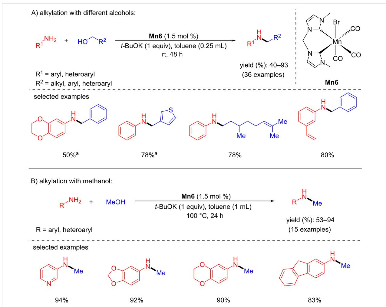
Scheme 11: Mn–NHC catalyst **Mn6** applied for the N-alkylation of amines with alcohols. <sup>a</sup>3 mol % of **Mn6** were used.
