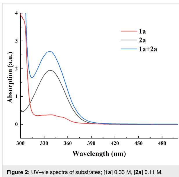
Figure 2: UV–vis spectra of substrates; [1a] 0.33 M, [2a] 0.11 M.
