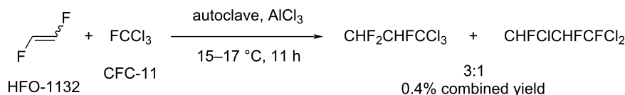
Scheme 17: Reaction of trichlorofluoromethane with 1,2-difluoroethylene.
