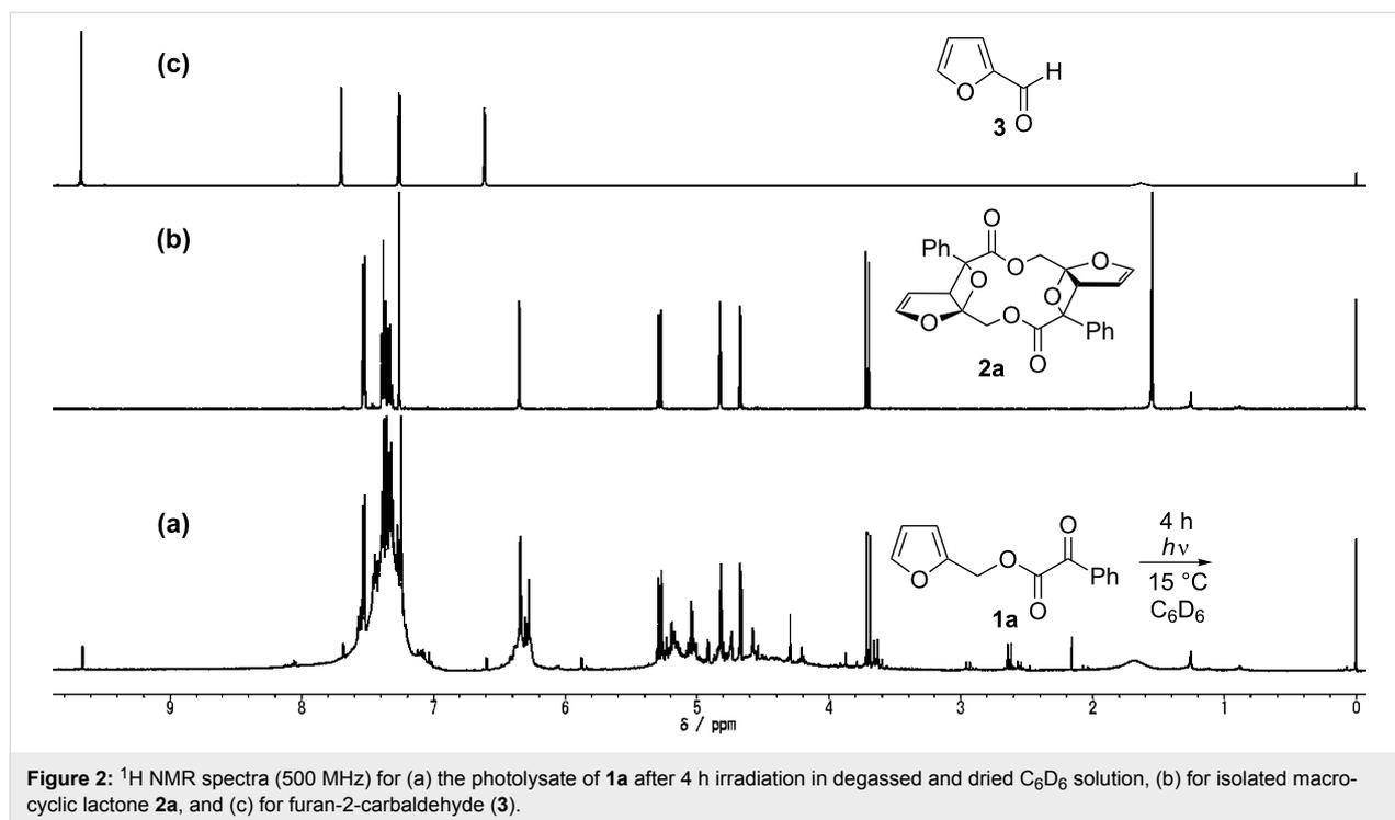
**Figure 2:** <sup>1</sup>H NMR spectra (500 MHz) for (a) the photolysate of **1a** after 4 h irradiation in degassed and dried C<sub>6</sub>D<sub>6</sub> solution, (b) for isolated macrocyclic lactone **2a**, and (c) for furan-2-carbaldehyde (**3**).
