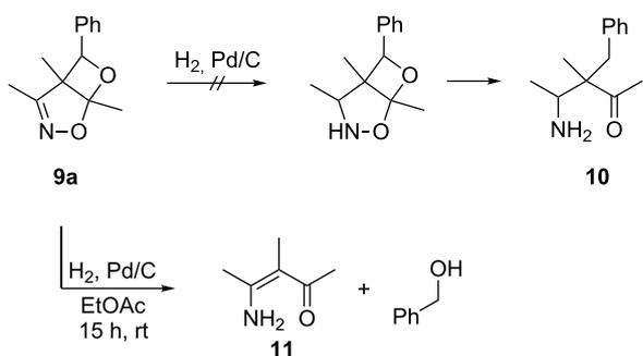
Scheme 8: Reductive cleavage of the trimethylisoxazole adduct **9a**.
