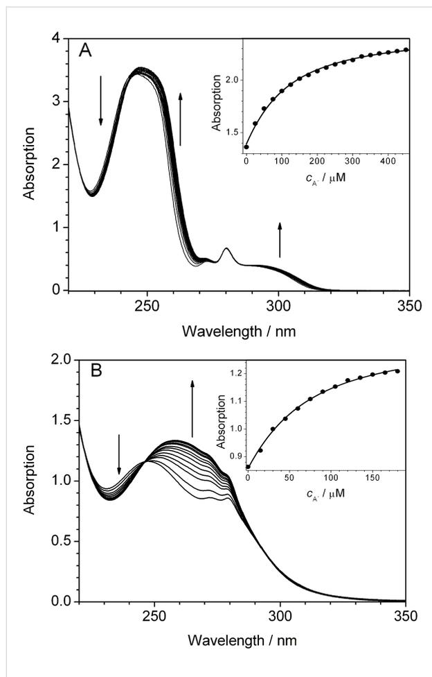
**Figure 1:** Photometric titration of A) tetrabutylammonium chloride (TBAC) to **1h** ( $c_{1h} = 50 \mu\text{M}$ ) and of B) tetrabutylammonium (10*S*)-camphorsulfonate (**SCS**) to **1i** ( $c_{1i} = 30 \mu\text{M}$ ). Arrows indicate the changes of the absorption with increasing concentration of the salt. Inset: Plot of the absorbance at 260 nm vs  $c_{\text{TBAC}}$  (A) and at 272 nm vs  $c_{\text{SCS}}$  (B); straight line represents the fit of the isotherm to a 1:1 stoichiometry.
