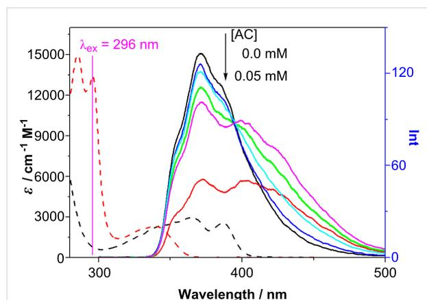
**Figure 4:** UV–vis spectra of AC (black dashed line) and **7** (red dashed line) and fluorescence spectra of **7** (0.02 mM) in the presence of 0.0, 0.0041, 0.0125, 0.025, 0.0375 and 0.05 mM AC in pH 9 phosphate buffer at 20 °C.  $\lambda_{\text{ex}} = 296 \text{ nm}$ .
