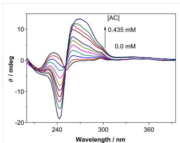
**Figure 3:** Circular dichroism spectra of **6** (0.2 mM) in the presence of 0, 0.0083, 0.025, 0.048, 0.071, 0.093, 0.11, 0.15, 0.18, 0.21 and 0.26 mM AC in pH 9 phosphate buffer at 20 °C.
