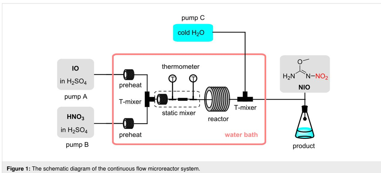
**Figure 1:** The schematic diagram of the continuous flow microreactor system.
