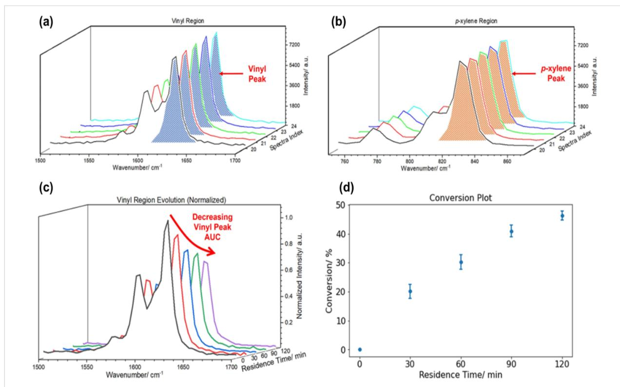
**Figure 8:** Overlay of several Raman spectra of a single condition featuring the styrene vinyl region (a) and the *p*-xylene region (b). (c) Waterfall plot depicting the decrease in the vinyl peak AUC over time. (d) A representative conversion plot shows an increasing conversion with residence time. Figure 8 is adapted from [53]. Figure 8 was reprinted with permission from [53], Copyright 2023 American Chemical Society.
