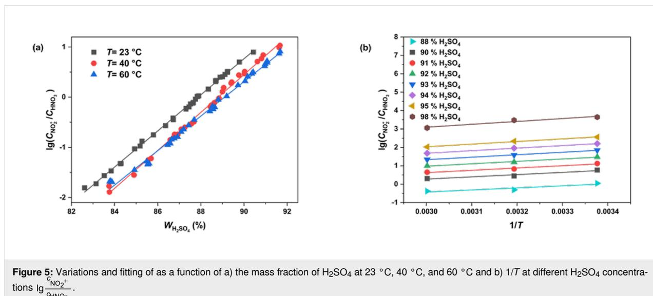
**Figure 5:** Variations and fitting of as a function of a) the mass fraction of  $\text{H}_2\text{SO}_4$  at 23 °C, 40 °C, and 60 °C and b)  $1/T$  at different  $\text{H}_2\text{SO}_4$  concentrations  $\lg\left(\frac{c_{\text{NO}_2^+}}{c_{\text{HNO}_3}}\right)$ .
