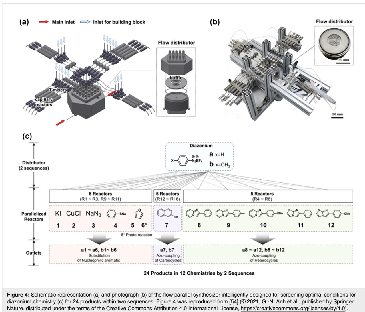
**Figure 4:** Schematic representation (a) and photograph (b) of the flow parallel synthesizer intelligently designed for screening optimal conditions for diazonium chemistry (c) for 24 products within two sequences. Figure 4 was reproduced from [54] (© 2021, G.-N. Anh et al., published by Springer Nature, distributed under the terms of the Creative Commons Attribution 4.0 International License, <https://creativecommons.org/licenses/by/4.0>).
