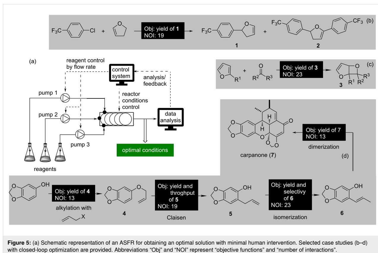
**Figure 5:** (a) Schematic representation of an ASFR for obtaining an optimal solution with minimal human intervention. Selected case studies (b–d) with closed-loop optimization are provided. Abbreviations "Obj" and "NOI" represent "objective functions" and "number of interactions".
