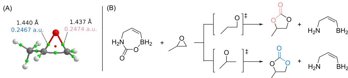
**Figure 2:** (A) Structure of PO annotated with the C–O bond distances and electron densities at the BCPs. BCPs are indicated by green spheres and the ring critical point by a red sphere. (B) Schematic representation of the two possible ring-opening reactions of PO in the presence of activated CO<sub>2</sub>.
