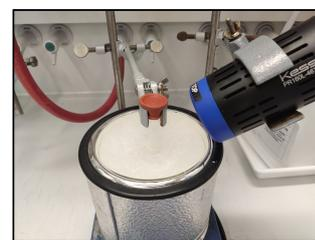
set-up with ice/NaCl bath
