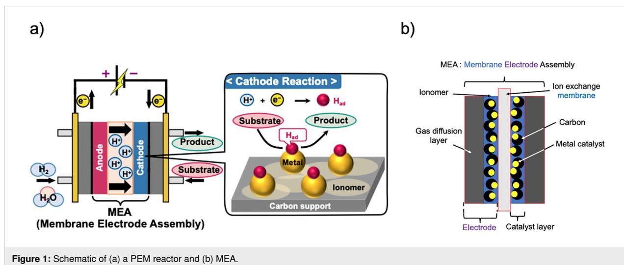
Figure 1: Schematic of (a) a PEM reactor and (b) MEA.
