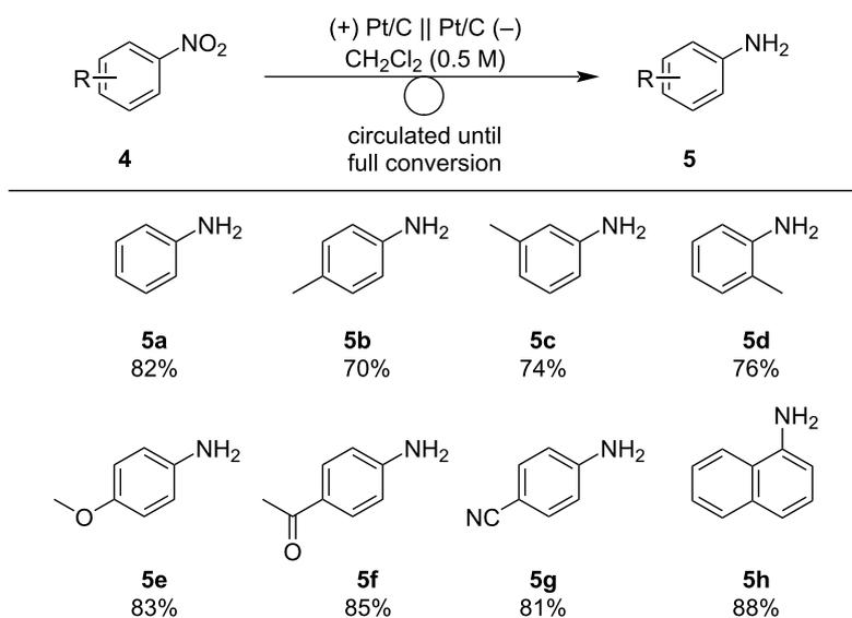
**Scheme 3:** Scope of the electrochemical reduction of nitroarenes. Reaction conditions: anode catalyst, Pt/C; cathode catalyst, Pt/C; **4**, 2.25 mmol; solvent,  $\text{CH}_2\text{Cl}_2$  (0.5 M); flow rate of the solution of **4**,  $0.75 \text{ mL min}^{-1}$ ; flow rate of  $\text{H}_2$  gas,  $100 \text{ mL min}^{-1}$ ; reaction temperature, room temperature; current density,  $50 \text{ mA cm}^{-2}$ . The solution was circulated until the full conversion of **4**. Isolated yield.
