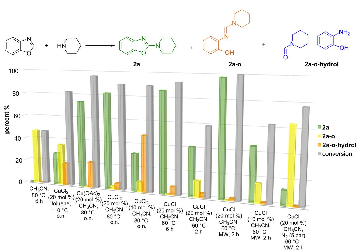
**Figure 1:** Reaction of benzimidazole with piperidine. a) Reaction scheme including intermaidates and b) conversion and selectivity plot of the C2-amination of benzoxazole with piperidine. Reaction conditions: benzoxazole (0.1 mmol), piperidine (0.15 mmol), copper catalyst, solvent (1.0 mL). Conversion was measured by NMR spectroscopy (see Figure S1 in Supporting Information File 1 for an example).
