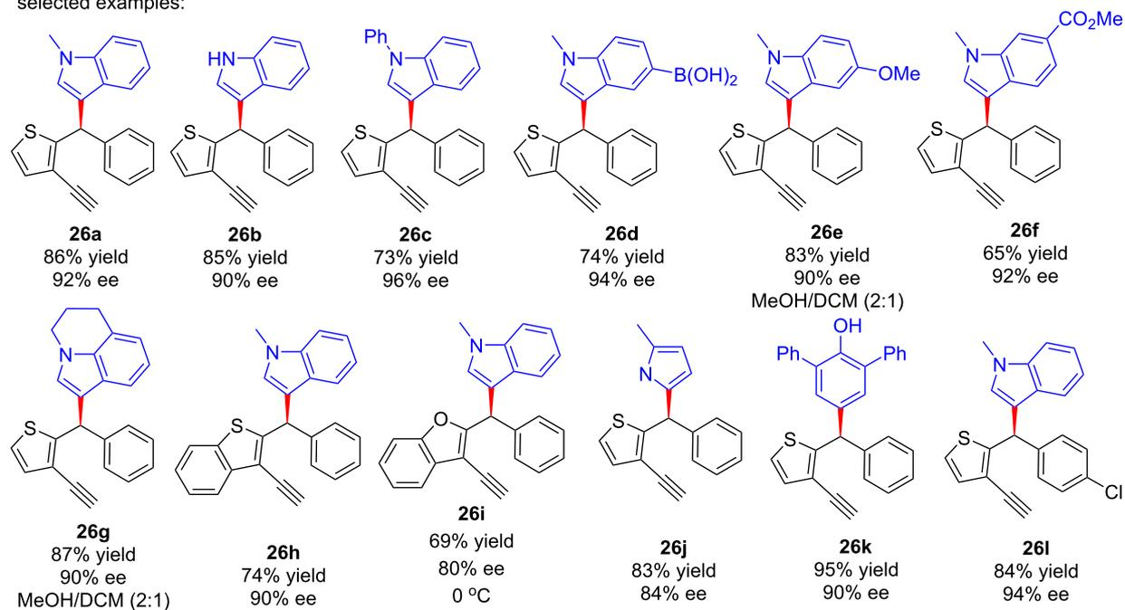
Scheme 25: Arylation by alkynylcopper driven dearomatization and rearomatization.
