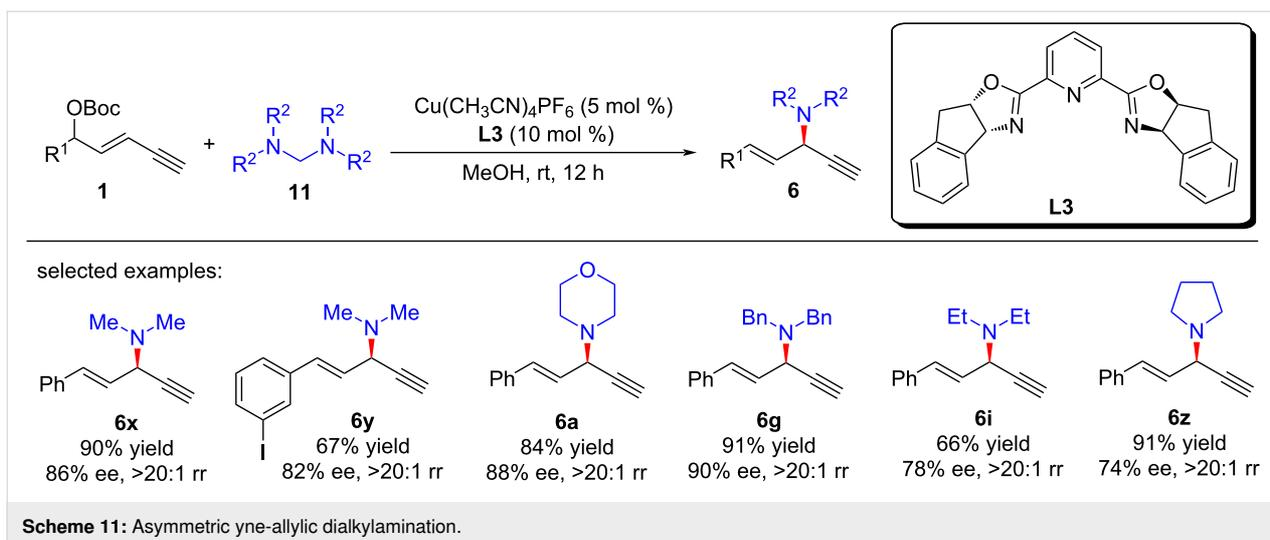
and enantioselectivities (Scheme 11, **6a**, **6g**, **6i** and **6z**). Further control experiments and DFT calculations show that during the catalytic process, tertiary amine directly participates as a nucleophilic reagent to give the ammonium salt, which then releases dimethylaminium to provide the final product (Scheme 12).
