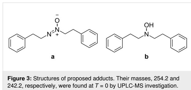
An attempt to identify the higher molecular masses observed by MS was made, and two intermediate structures are proposed in Figure 3. Together with **(a)**, *N,N*-diphenethylhydroxylamine **(b)** as second product is proposed. The latter may be produced from the reaction of 2-phenylacetaldehyde **(e)** and the reduced amino product **d** via reductive alkylation [38-40] (Scheme 3).
