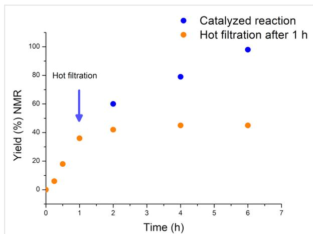
**Figure 4:** Hot filtration test for the Si-MonoAm-Cu(I)-catalysed C2-amination of benzoxazole with piperidine in acetonitrile at 80 °C. Si-MonoAm-Cu(I) was filtered off after 60 min using a hot filter.
