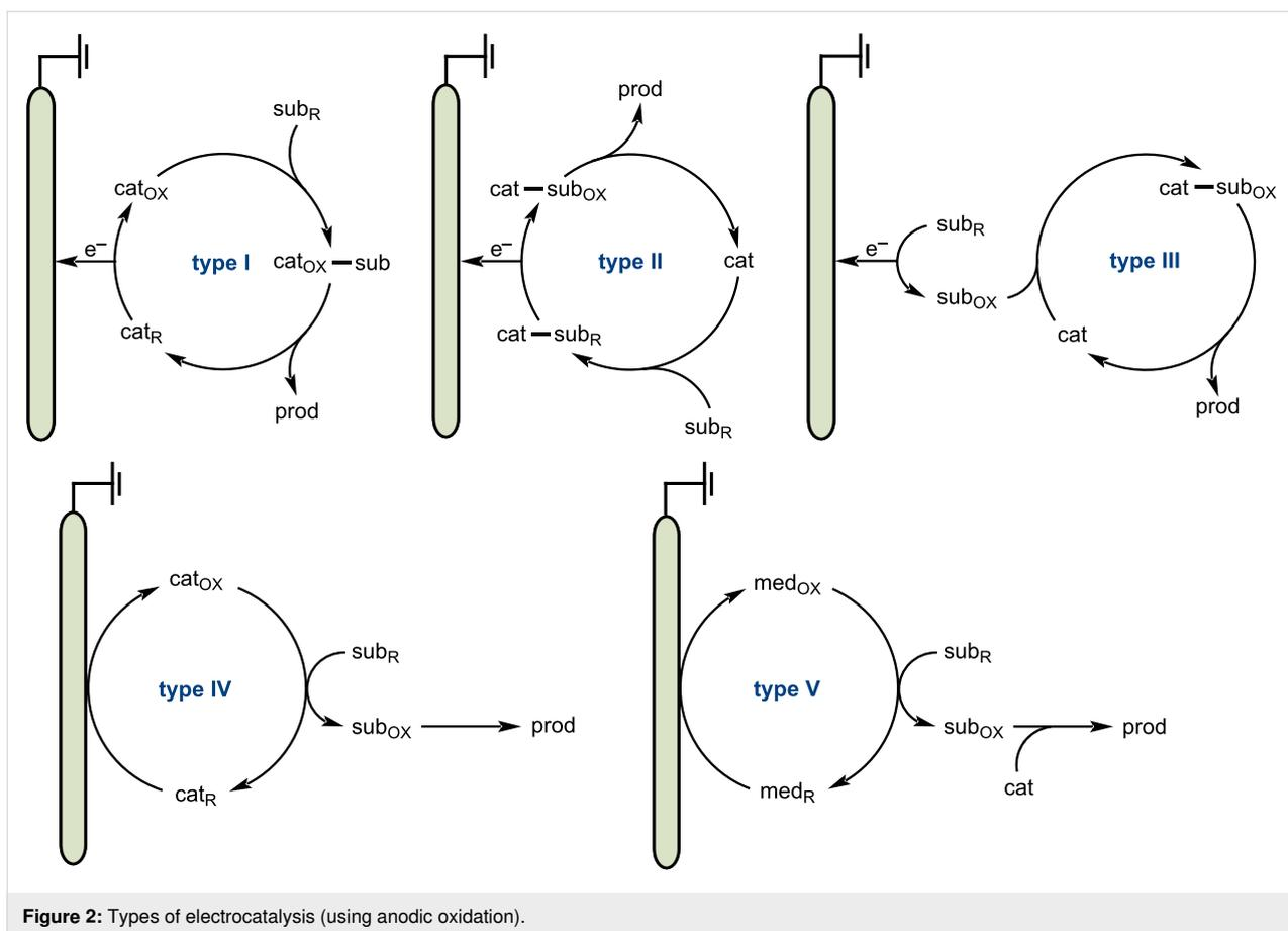
**Figure 2:** Types of electrocatalysis (using anodic oxidation).
