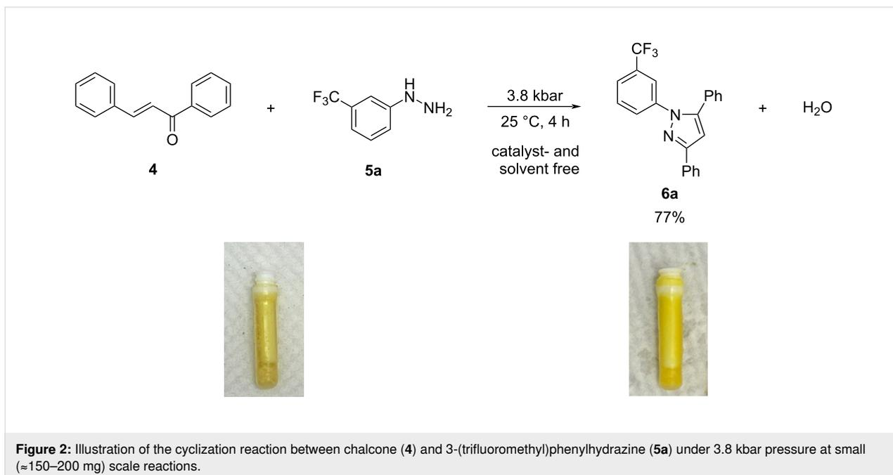
**Figure 2:** Illustration of the cyclization reaction between chalcone (**4**) and 3-(trifluoromethyl)phenylhydrazine (**5a**) under 3.8 kbar pressure at small ( $\approx 150$ – $200$  mg) scale reactions.
