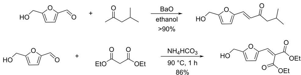
**Scheme 115:** Base-catalyzed aldol condensation/dehydration sequences from HMF.
