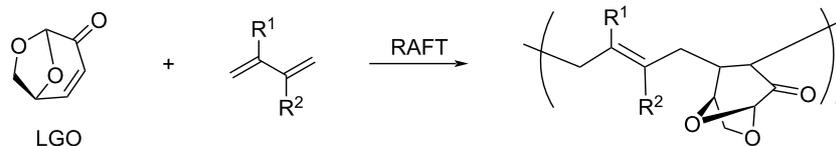
**Scheme 152:** RAFT co-polymerization of LGO and butadienes.
