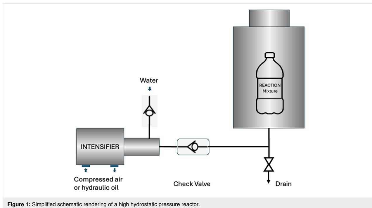
**Figure 1:** Simplified schematic rendering of a high hydrostatic pressure reactor.
