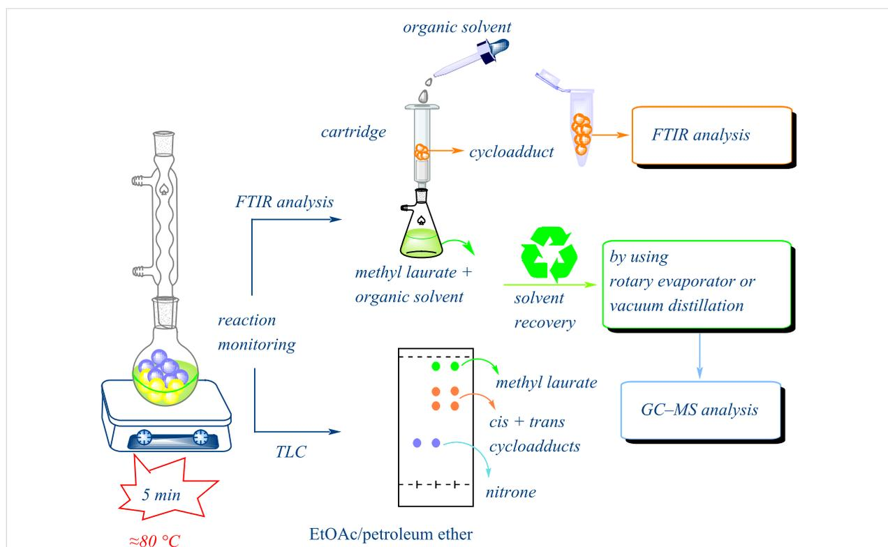
**Figure 12:** Simplified scheme describing the reaction monitoring and solvent recovery.
