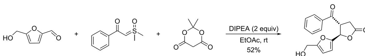
**Scheme 105:** Synthesis of HMF derived disubstituted  $\gamma$ -butyrolactone.
