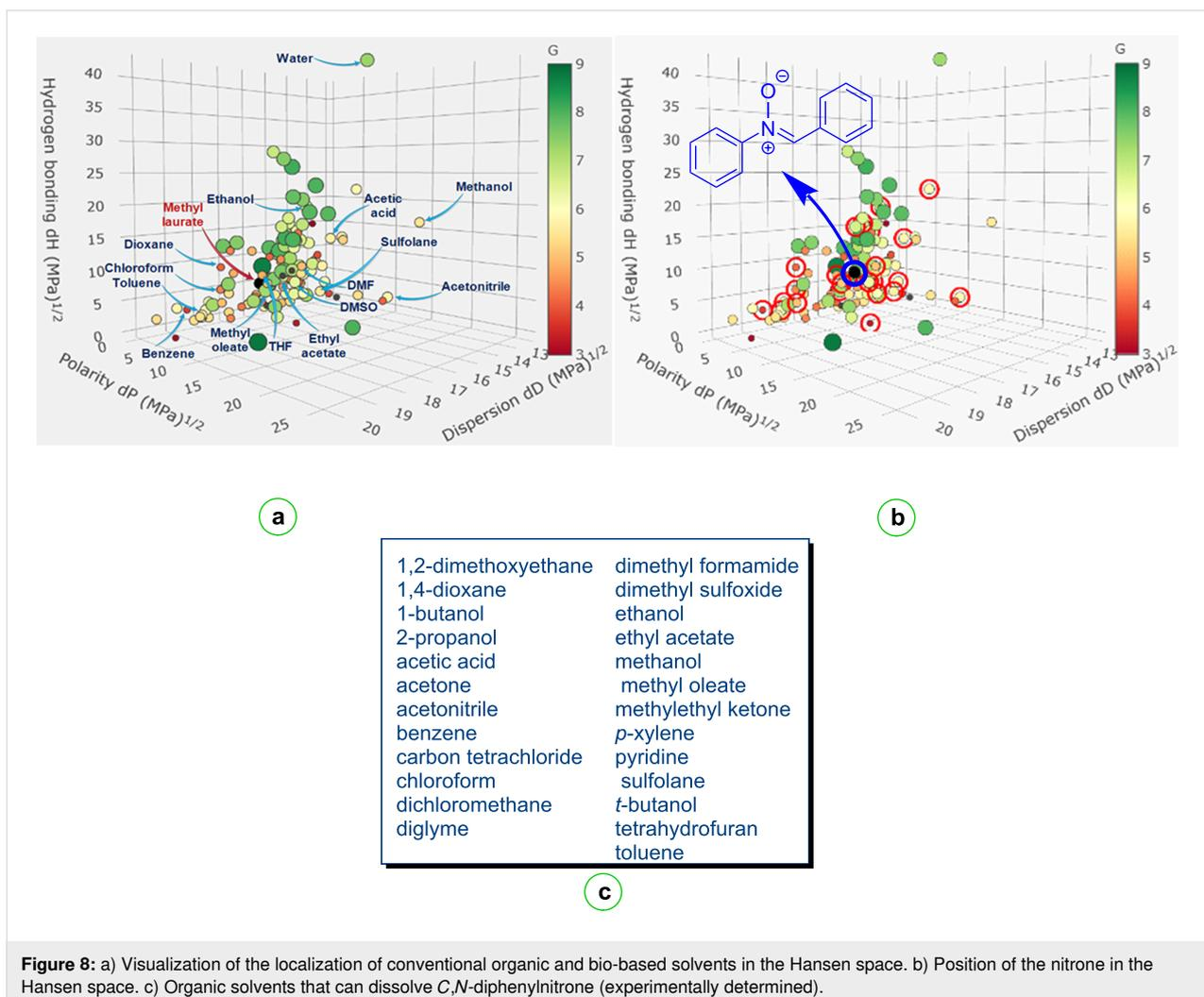
**Figure 8:** a) Visualization of the localization of conventional organic and bio-based solvents in the Hansen space. b) Position of the nitron in the Hansen space. c) Organic solvents that can dissolve *C,N*-diphenylnitron (experimentally determined).
