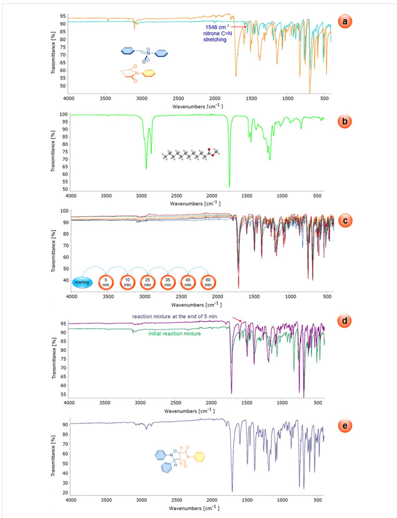
**Figure 13:** a) The superimposed spectra of *C,N*-diphenylnitron and *N*-phenylmaleimide. b) The spectrum of methyl laurate. c) The spectrum of the reaction mixture, collected from the reaction medium after one hour had elapsed since the beginning of the reaction. d) The spectrum of the initial reaction mixture and the mixture collected from the reaction medium after five minutes. e) The spectrum of the isolated product **3a**.
