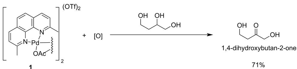
**Scheme 30:** Conversion of polyols by  $[\text{neocuproinePd}(\text{OAc})_2(\text{OTf})_2]_2$  to  $\alpha$ -hydroxy ketones.
