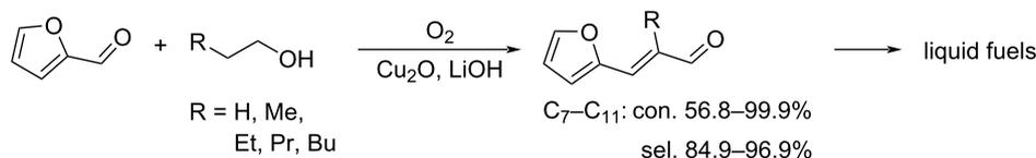
**Scheme 51:** The aerobic oxidative condensation of biomass-derived furfural and linear alcohols.
