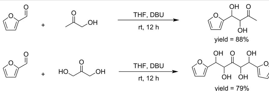
**Scheme 26:** C–C-bond-formation reactions of a biomass-based feedstock aromatic aldehyde (C<sub>5</sub>) and hydroxyacetone (C<sub>3</sub>).
