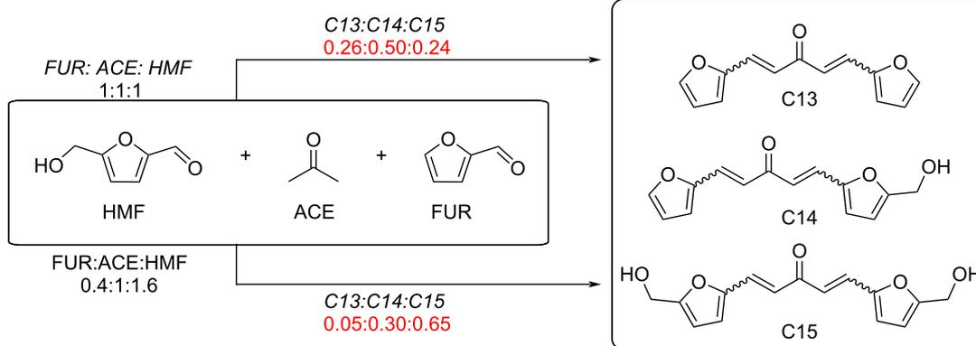
**Scheme 114:** Cross-condensation of furfural, acetone and HMF into C<sub>13</sub>, C<sub>14</sub> and C<sub>15</sub> products.
