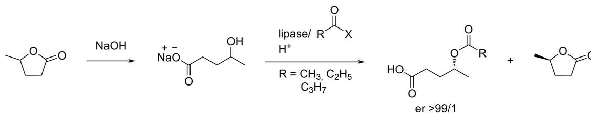
**Scheme 93:** Construction of 4-acyloxypentanoic acids from GVL.
