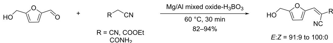
**Scheme 116:** Condensation of HMF and active methylene nitrile.
