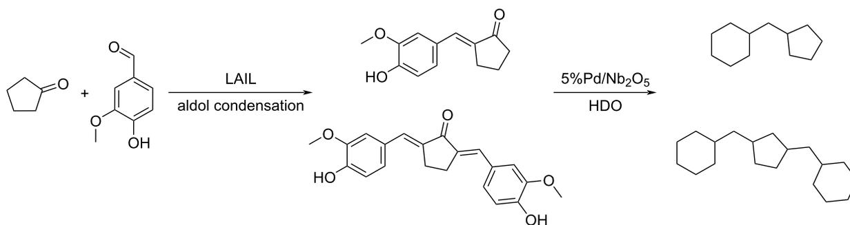
**Scheme 66:** Synthesis of jet fuels range cycloalkanes from CPN and lignin-derived vanillin.
