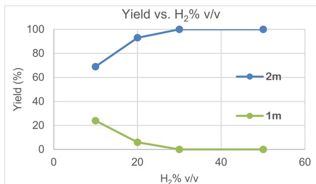
**Figure 3:** Continuous-flow hydrogenation of benzaldehyde **1m** by varying the H<sub>2</sub>/N<sub>2</sub> v/v ratio. Conditions: solution of **1m** in EtOAc (0.06 M) with decane as an internal standard; substrate flow rate, 10 mL h<sup>-1</sup>; H<sub>2</sub> + N<sub>2</sub> mixed-gas flow rate, 20 mL min<sup>-1</sup>; amount of Pt in the column, 0.032 mmol; reaction temperature, room temperature.
