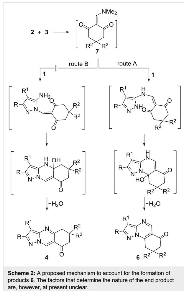
**Scheme 2:** A proposed mechanism to account for the formation of products **6**. The factors that determine the nature of the end product are, however, at present unclear.
