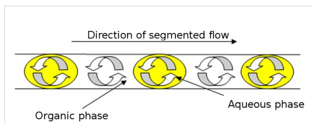
**Figure 9:** Schematic illustrating the mixing of immiscible reagent streams in a microfluidic channel, whereby the continuous phase composition depends on the ratio of organic and aqueous reactants employed.
