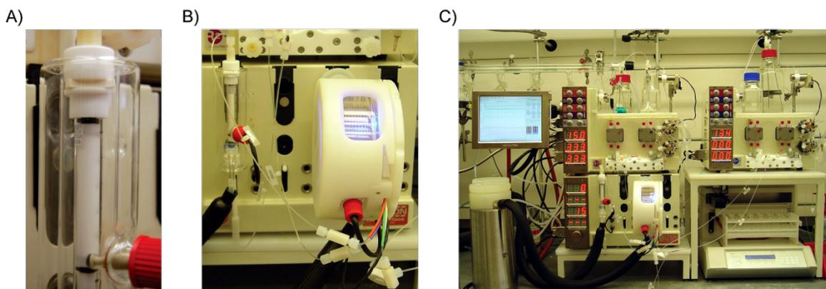
**Figure 2:** General reactor setup. A) A glass Omnifit column is packed with 1 g of proline. B) The column is then placed in-line with a 10 mL PFA coil-tube reactor. C) The components are connected to HPLC pumps for solvent and reagent inputs. The reactor is controlled by a computer in order to program the timing of the reagent and solvent inputs and fraction collection.
