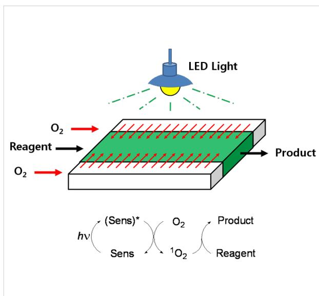
**Figure 3:** Photosensitized oxygenation in the triple-channel microreactor.
