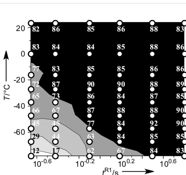
**Figure 2:** Effects of the temperature ( $T$ ) and the residence time in **R1** ( $t^{\text{R1}}$ ) on the yield of anisole in the Br–Li exchange reaction of *p*-bromoanisole followed by reaction with methanol in the flow microreactor system. The contour plot with scatter overlay shows the yields of anisole (%), which are indicated by small circles.
