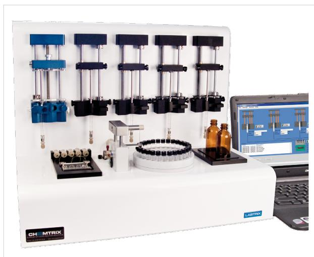
**Figure 2:** Photograph illustrating Labtrix<sup>®</sup> S1, the automated micro-reactor development apparatus from Chemtrix BV (NL), used for the evaluation described herein.
