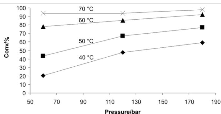
**Figure 5:** Nucleophilic aromatic substitution reaction of 1-fluoro-4-nitrobenzene (**15**) with pyrrolidine (**16**) in THF (Scheme 5) at different temperatures and three different pressures performed in a 8 mL stainless steel coil at a flow rate of 1 mL/min.
