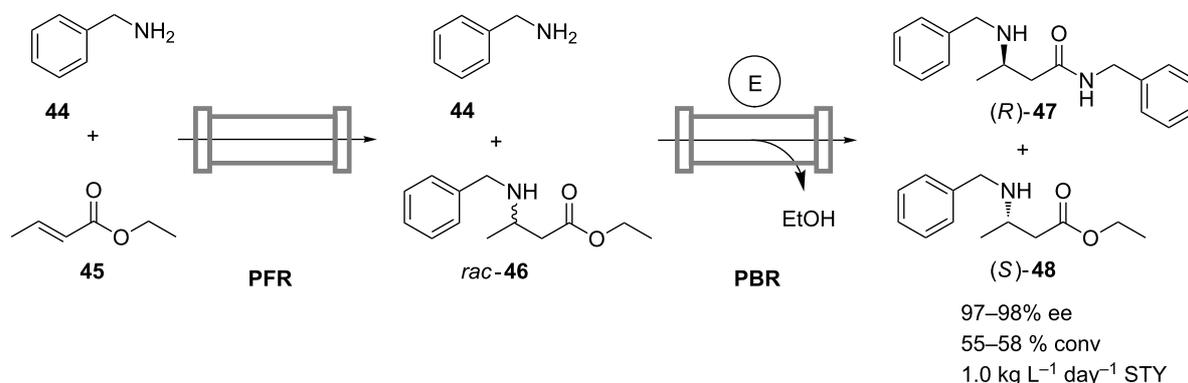
**Scheme 14:** Continuous solvent-free chemo-enzymatic synthesis of ethyl (*S*)-3-(benzylamino)butanoate (**48**) in a sequence of a plug-flow reactor (PFR) and a packed-bed reactor containing Novozym 435 (E) [38].
