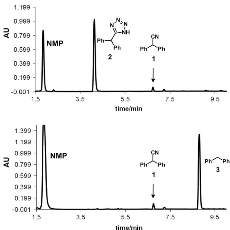
**Figure 1:** HPLC-UV chromatograms (215 nm) of crude reaction mixtures from the cycloaddition of diphenylacetonitrile (**1**) with NaN<sub>3</sub> (Scheme 1) comparing microwave batch (top) and continuous flow conditions (bottom). Reaction parameters: 220 °C, ≈16 min, 2.5 equiv NaN<sub>3</sub>, NMP/AcOH/H<sub>2</sub>O 5:3:2.
