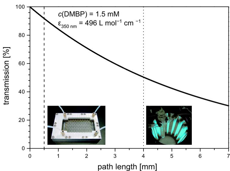
**Figure 3:** Light-penetration profile for a 1.5 mM solution of DMBP at 350 nm. The vertical lines represent the path length in the dwell device (vertical dashed line) versus the effective path length in the Schlenk flask (vertical dotted line).
