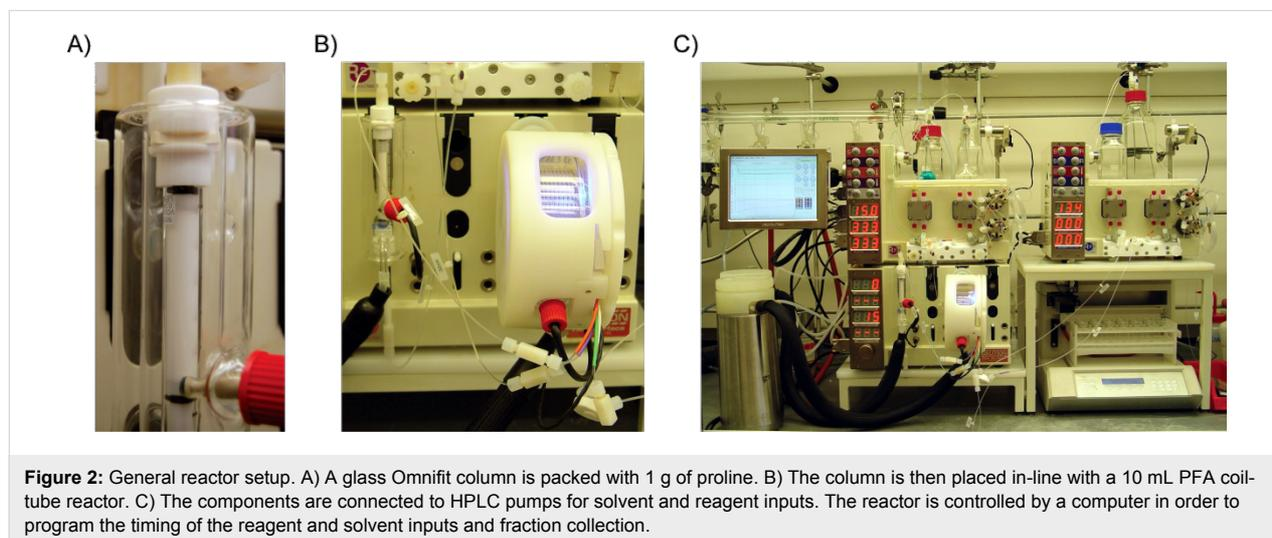
**Figure 2:** General reactor setup. A) A glass Omnifit column is packed with 1 g of proline. B) The column is then placed in-line with a 10 mL PFA coil-tube reactor. C) The components are connected to HPLC pumps for solvent and reagent inputs. The reactor is controlled by a computer in order to program the timing of the reagent and solvent inputs and fraction collection.
