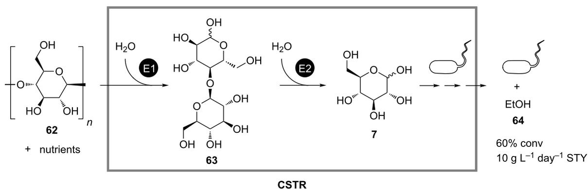
**Scheme 19:** Continuous fermentative production of ethanol (**64**) from hardwood lignocellulose (**62**) in a stirred-tank reactor (CSTR) containing yeast cells, cellulase (E1) and  $\beta$ -glucosidase (E2) [45].
