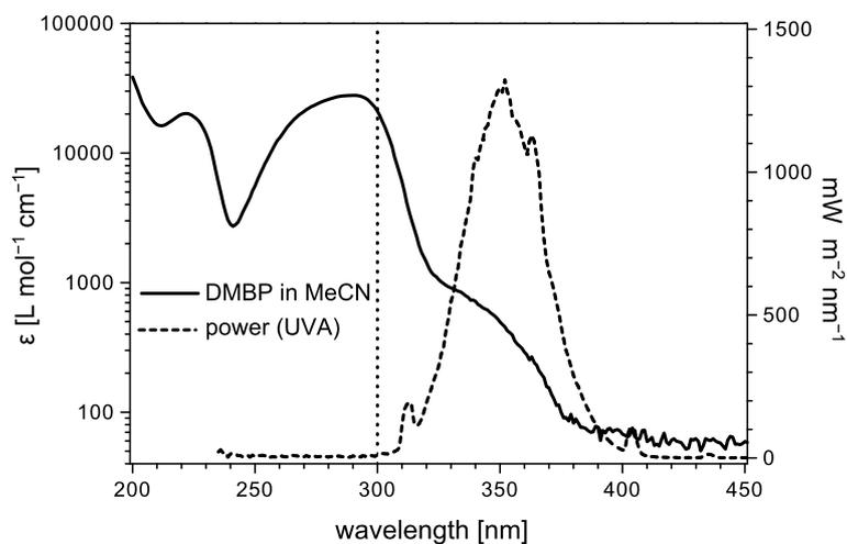
**Figure 2:** UV-spectrum of DMBP (in MeCN) versus emission spectrum of the UVA lamp. The vertical dotted line represents the cut-off wavelength of Foturan™ and Pyrex at 300 nm (approx. 30% transmission).
