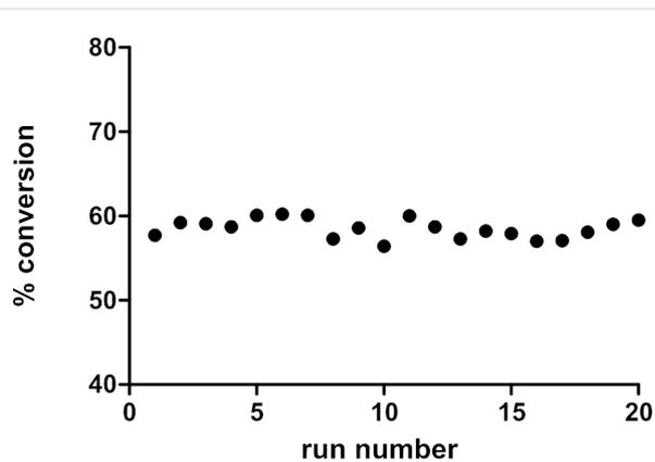
**Figure 4:** Conversion of styrene to ethylbenzene over 20 reactions in sequence through a single 30 mm 10% Pd/C CatCart<sup>®</sup>. All reactions were carried out with a 10% Pd/C 30 mm CatCart<sup>®</sup>, with 2.0 M in MeOH, at a flow rate of 1.0 mL/min, at 30 °C, with 1.9 mL per injection, and 10 mL product solution collected. The conversion was determined by GC–MS analysis with decane as an internal standard.
