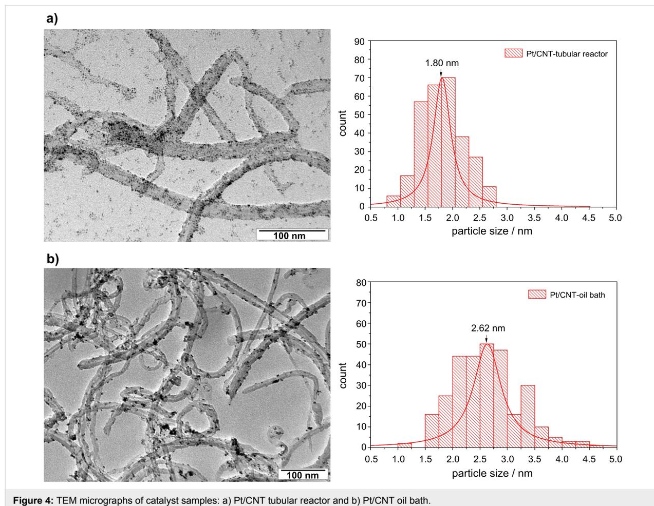
Figure 4: TEM micrographs of catalyst samples: a) Pt/CNT tubular reactor and b) Pt/CNT oil bath.
