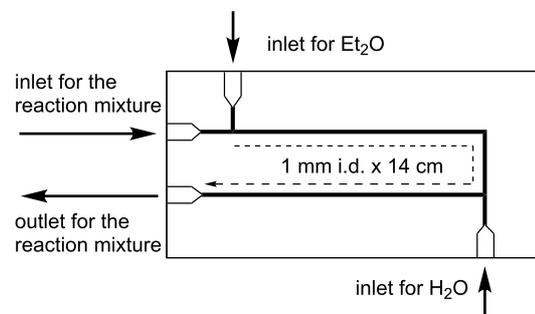
Figure 2: Hastelloy-made microextraction unit.
