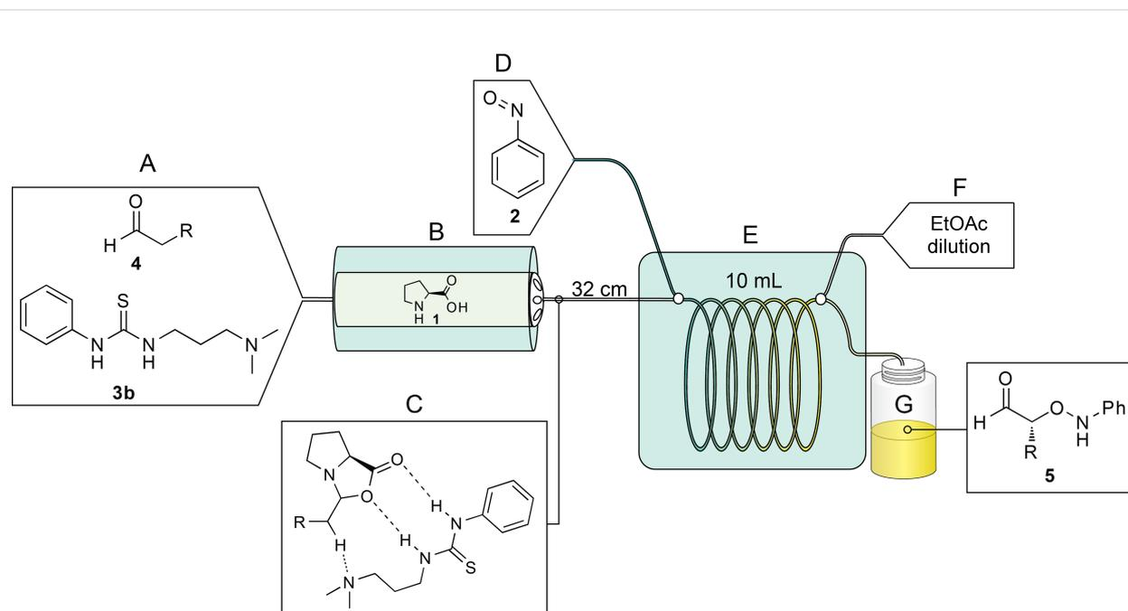
**Figure 3:** Schematic of the reactor setup. As the starting aldehyde and thiourea 3b (A) enter the proline packed-bed (B) an oxazolidinone intermediate is formed, drawing the proline into the solution (C). Upon precooling in a reactor coil (E) the intermediate is mixed with nitrosobenzene (D). Prior to exiting, ethyl acetate is added to dilute the reaction (F) and product is collected into vials (G) for further reduction, work-up, and isolation.
