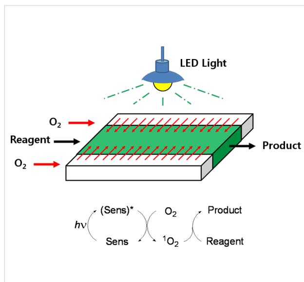
**Figure 3:** Photosensitized oxygenation in the triple-channel microreactor.
