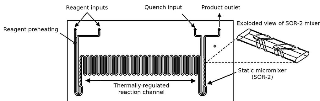
**Figure 3:** Schematic illustrating the  $10 \mu\text{L}$  reactor manifold used for the  $\text{S}_{\text{N}}\text{Ar}$  reactions described herein (3223; Chemtrix BV, NL), with the important features highlighted.
