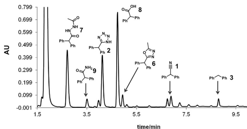
**Figure 2:** HPLC-UV chromatogram (215 nm) showing the decomposition of tetrazole **2** in NMP/AcOH/H<sub>2</sub>O 5:3:2 (0.125 M) after heating in a stainless steel flow coil at 180 °C for 5.3 min.
