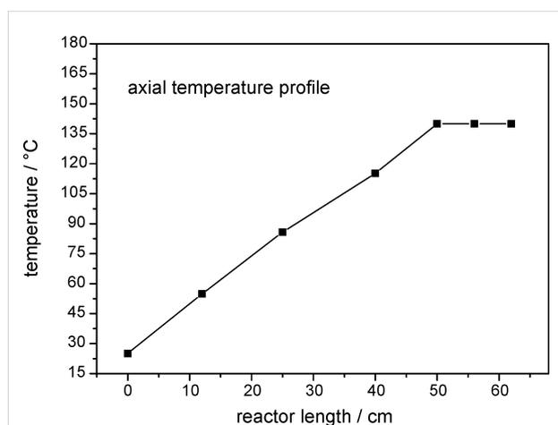
**Figure 2:** Measured temperature profile along the tubular reactor.
