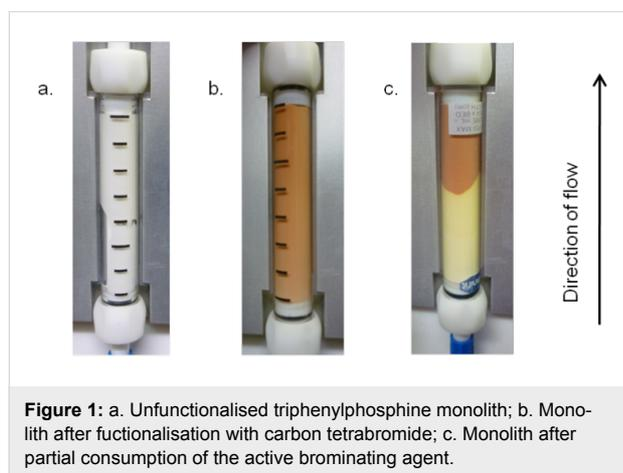
**Figure 1:** a. Unfunctionalised triphenylphosphine monolith; b. Monolith after functionalisation with carbon tetrabromide; c. Monolith after partial consumption of the active brominating agent.
