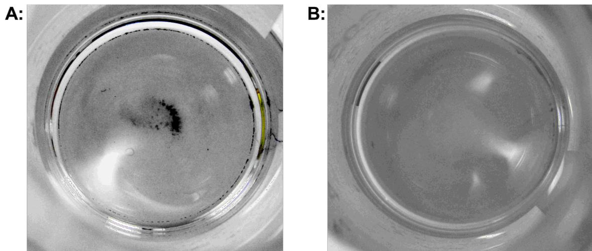
**Figure 7:** Leached catalyst from 30 mm 10% Pd/C CatCart<sup>®</sup>. First 10 mL wash aliquot (A) compared to second 10 mL wash aliquot (B). Photographs were taken from above, with the samples in 20 mL scintillation vials.
