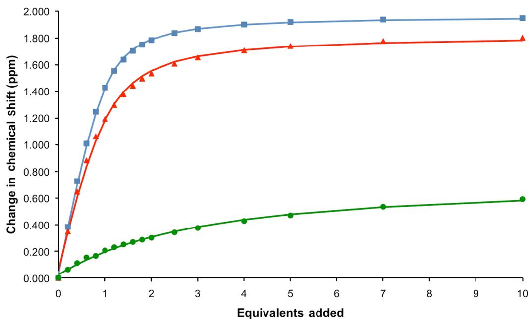
**Figure 3:** Titration data (solid points) and fitted binding isotherms (curves) monitoring the triazolium proton, d, for titration of benzoate, chloride and iodide into a solution of  $5\text{-}2\text{PF}_6$  (500 MHz, 293 K,  $\text{CD}_3\text{CN}$ ).
