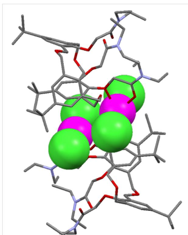
**Figure 23:** X-ray crystal structure of [**17a**·HgCl<sub>2</sub>]<sub>2</sub> (CCDC ID 168653) [69].
