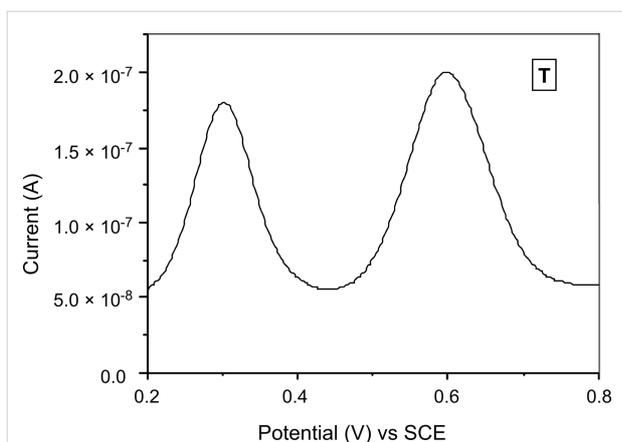
**Figure 4:** Differential pulse voltammogram of **T** in acetonitrile (0.1 M *n*-Bu<sub>4</sub>NPF<sub>6</sub> as electrolyte, Ag wire as a quasi-reference electrode, 1,1'-dimethylferrocene as internal standard, scan rate = 20 mV s<sup>-1</sup> and a pulse height of 2 mV).
