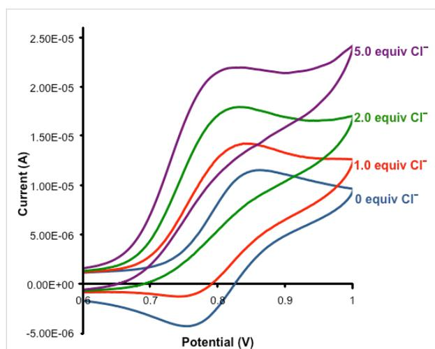
**Figure 4:** CV of **5·2PF<sub>6</sub>** upon the addition of TBA·Cl (electrolyte: 0.1 M TBA·PF<sub>6</sub>/CH<sub>3</sub>CN, [**5·2PF<sub>6</sub>**] = 0.50 mM, 293 K. Potential vs. Ag/AgCl reference).
