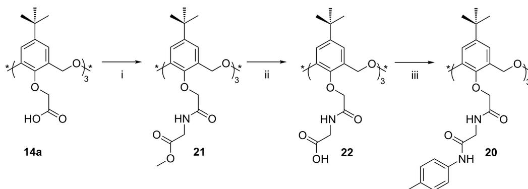
**Scheme 12:** Extending the lower rim: (i) Glycine methyl ester, HOBt, dicyclohexylcarbodiimide (DCC), CH<sub>2</sub>Cl<sub>2</sub>; (ii) NaOH, H<sub>2</sub>O/1,4-dioxane; (iii) *p*-toluidine, HOBt, DCC, CH<sub>2</sub>Cl<sub>2</sub> [37].
