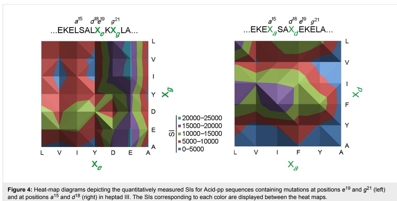
**Figure 4:** Heat-map diagrams depicting the quantitatively measured SIs for Acid-pp sequences containing mutations at positions  $e^{19}$  and  $g^{21}$  (left) and at positions  $a^{15}$  and  $d^{18}$  (right) in heptad III. The SIs corresponding to each color are displayed between the heat maps.
