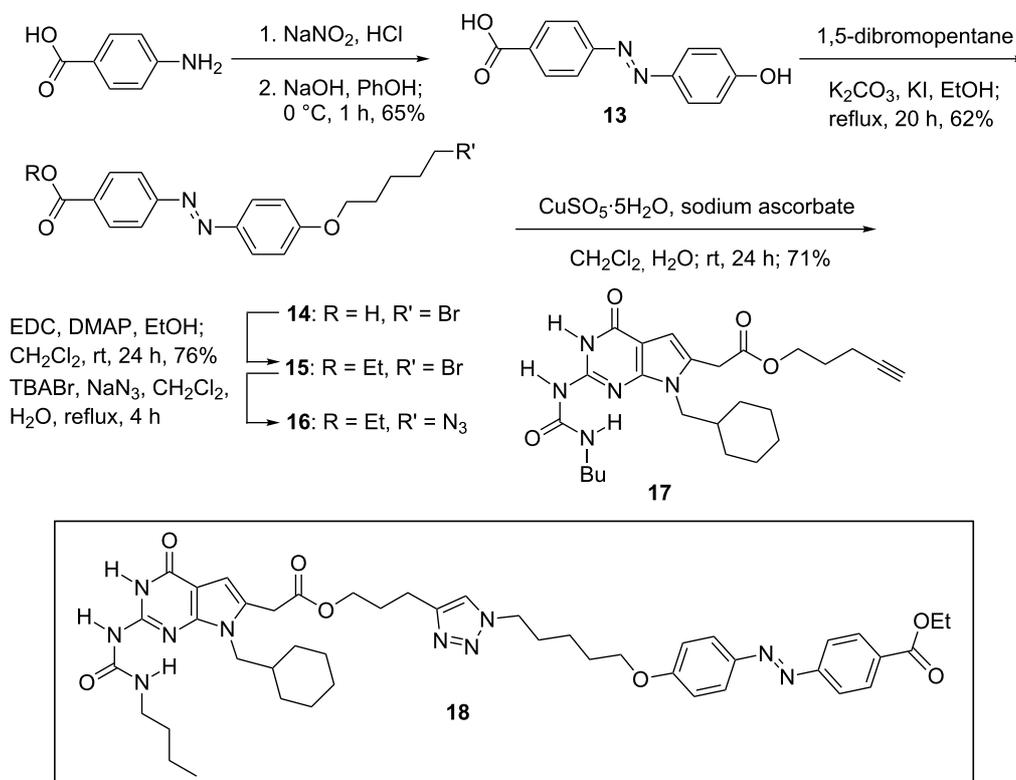
**Scheme 4:** Synthesis of azobenzene dye-coupled DeUG **18**.
