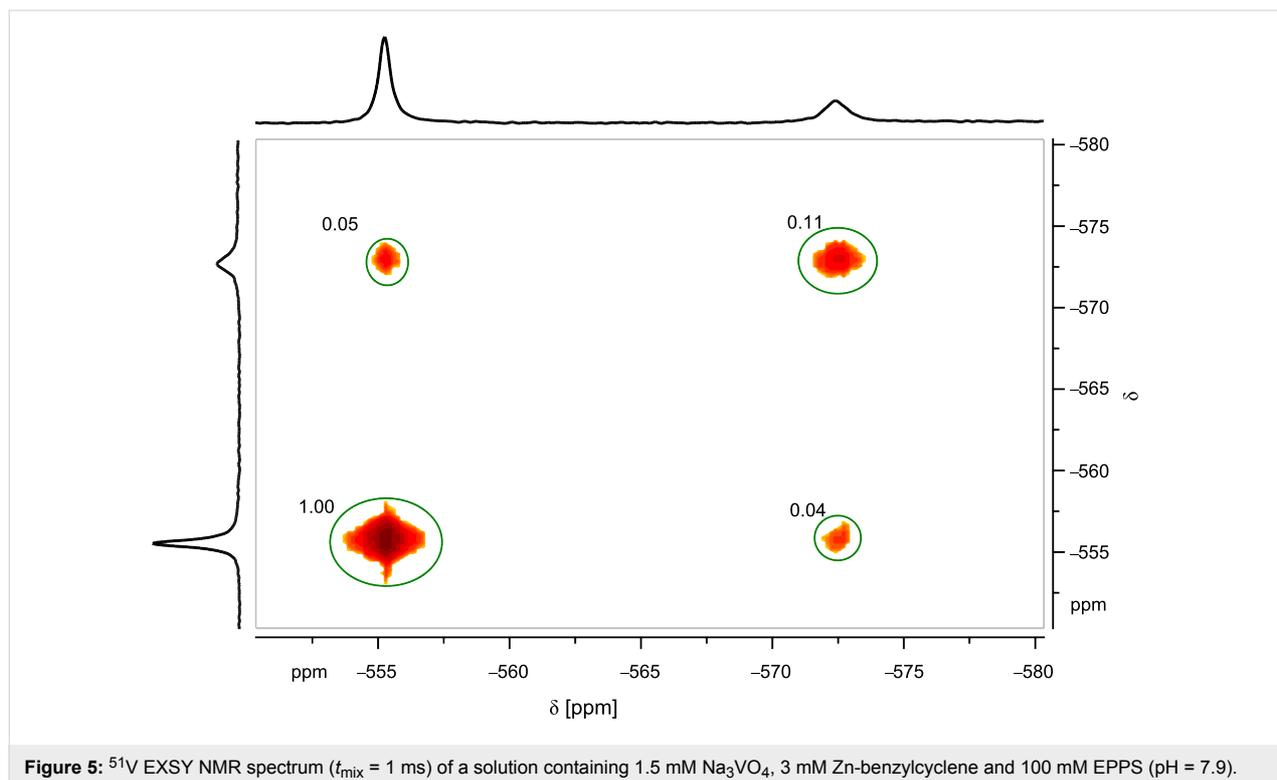
**Figure 5:**  $^{51}\text{V}$  EXSY NMR spectrum ( $t_{\text{mix}} = 1 \text{ ms}$ ) of a solution containing 1.5 mM  $\text{Na}_3\text{VO}_4$ , 3 mM Zn-benzylcyclene and 100 mM EPPS (pH = 7.9).
