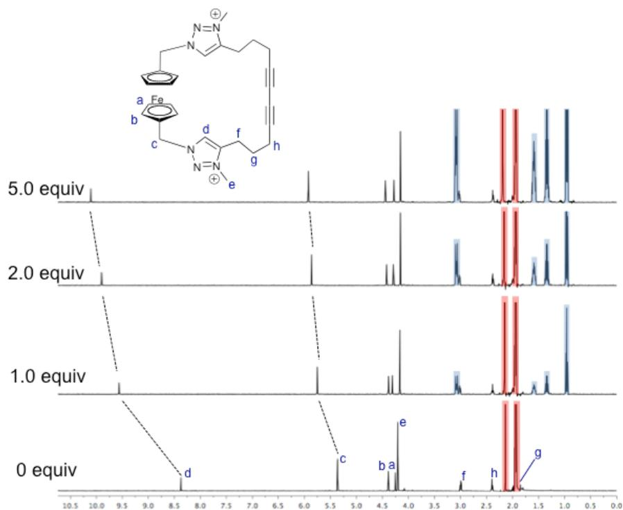
**Figure 2:**  $^1\text{H}$  NMR spectra of  $5\text{-}2\text{PF}_6$  after the addition of 0, 1.0, 2.0 and 5.0 equiv of TBA-Cl (500 MHz, 293 K,  $\text{CD}_3\text{CN}$ ). Red-shaded peaks correspond to solvent signals ( $\text{H}_2\text{O}$  and  $\text{CH}_3\text{CN}$ ); blue-shaded peaks correspond to signals from TBA cations.
