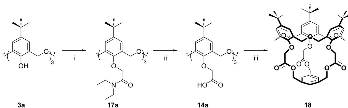
**Scheme 11:** Capping the lower rim: (i) *N,N*-Diethylchloroacetamide, NaH, THF; (ii) NaOH, H<sub>2</sub>O/1,4-dioxane; (iii) 1,3,5-tris(bromomethyl)benzene, Na<sub>2</sub>CO<sub>3</sub>, DMF [33].
