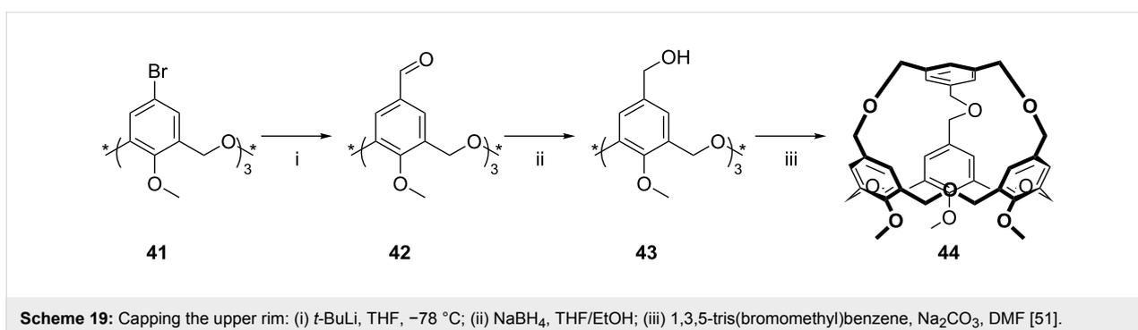
**Scheme 19:** Capping the upper rim: (i) *t*-BuLi, THF, –78 °C; (ii) NaBH<sub>4</sub>, THF/EtOH; (iii) 1,3,5-tris(bromomethyl)benzene, Na<sub>2</sub>CO<sub>3</sub>, DMF [51].
