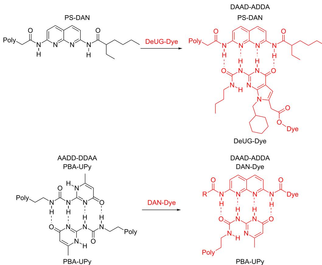
**Figure 2:** Illustration of the use of DeUG-Dye and DAN-Dye as colorimetric indicators for supramolecular interactions through specific quadruply hydrogen-bonding interactions. Top: DeUG-Dye interacts with DAN modified polystyrene (PS). Bottom: DAN-Dye interacts with UPy modified polybutyl acrylate (PBA).
