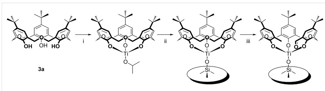
**Scheme 20:** Effect of Ti(IV)/SiO<sub>2</sub> on **3a**: (i) Ti(OiPr)<sub>4</sub>, toluene; (ii) triphenylsilanol, toluene; (iii) partially dehydroxylated silica gel, toluene [58].
