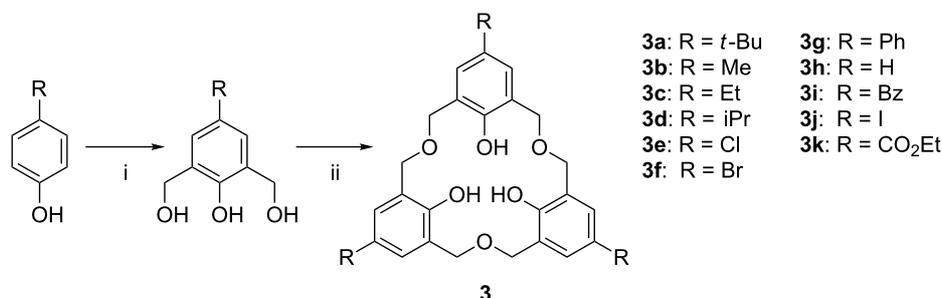
**Scheme 1:** Synthesis of oxacalix[3]arenes: (i) Formaldehyde (37% aq), NaOH (aq), 1,4-dioxane; glacial acetic acid, acetone; (ii) refluxing *o*-xylene [14] or Na<sub>2</sub>SO<sub>4</sub>, MsOH, in refluxing DME [15].
