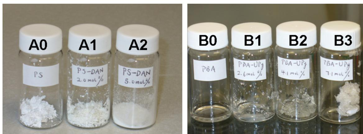
**Figure 5:** Physical appearance of DAN-modified PS and UPy-modified PBA. Left: A0 = PS, A1 = PS-DAN 2.0 mol %, A2 = PS-DAN 5.0 mol %. Right: B0 = PBA, B1 = PBA-UPy 2.6 mol %, B2 = PBA-UPy 4.1 mol %, B3 = PBA-UPy 7.1 mol %.
