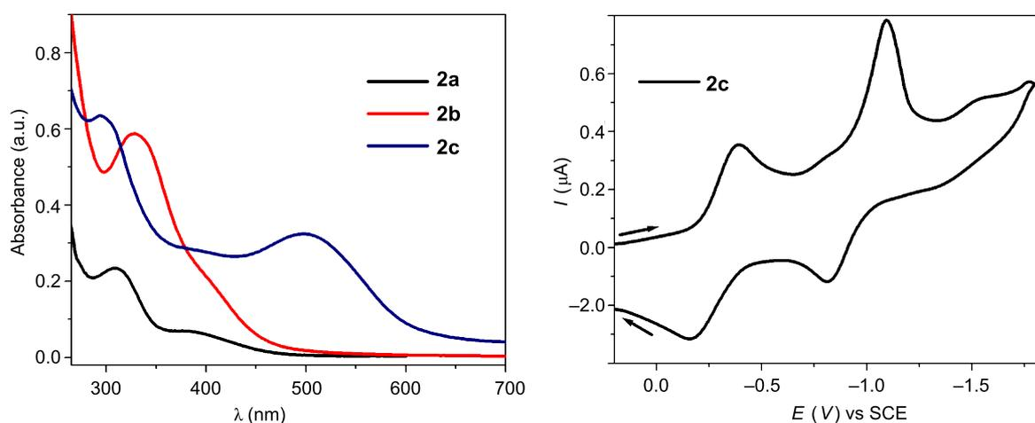
**Figure 6:** UV–vis absorption spectrum (left) of macrocycles (**2a–2c**) recorded in CH<sub>3</sub>CN at 298 K, and cyclic voltammogram of **2c** (right) performed in CH<sub>2</sub>Cl<sub>2</sub>/0.1 M (*n*-Bu)<sub>4</sub>NPF<sub>6</sub> with a scan rate of 100 mV s<sup>-1</sup> versus SCE at 298 K.
