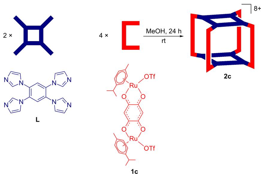
**Scheme 3:** Formation of an octanuclear macrocycle **2c** upon reaction of Ru(II)<sub>2</sub>-based acceptors **1c** with imidazole-based tetratopic donor **L** in methanol at room temperature.
