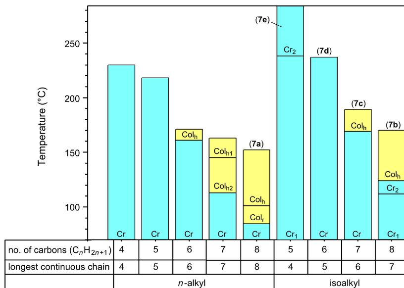
**Figure 1:** Comparison of the phase behaviours of the  $\alpha$ -substituted phthalocyanines with *n*-alkyl [25] and isoalkyl side chains. The stable ranges for the crystal phases are shown in blue and those of the columnar liquid-crystalline phases in yellow.
