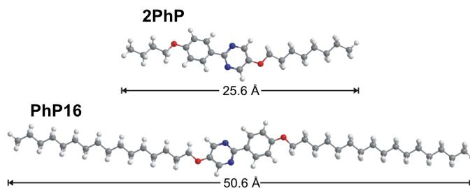
**Figure 2:** Molecular structures and molecular lengths of **2PhP** and **PhP16**. The longer mesogen **PhP16** is approximately twice the length of the shorter mesogen **2PhP**. The energy of each molecular structure was minimized by molecular modelling with the semiempirical method MOPAC/AM1 for the most extended conformers.
