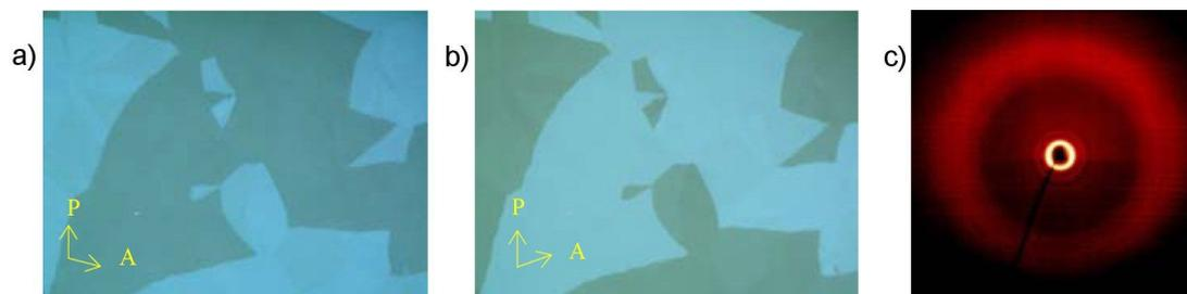
**Figure 19:** Compound **OH 5d**: Optical photomicrographs of chiral domains at 122 °C; polariser and analyser are uncrossed by about a)  $-8^\circ$  and b)  $+8^\circ$  from the  $90^\circ$  position; c) X-ray pattern of a powderlike sample at 110 °C.
