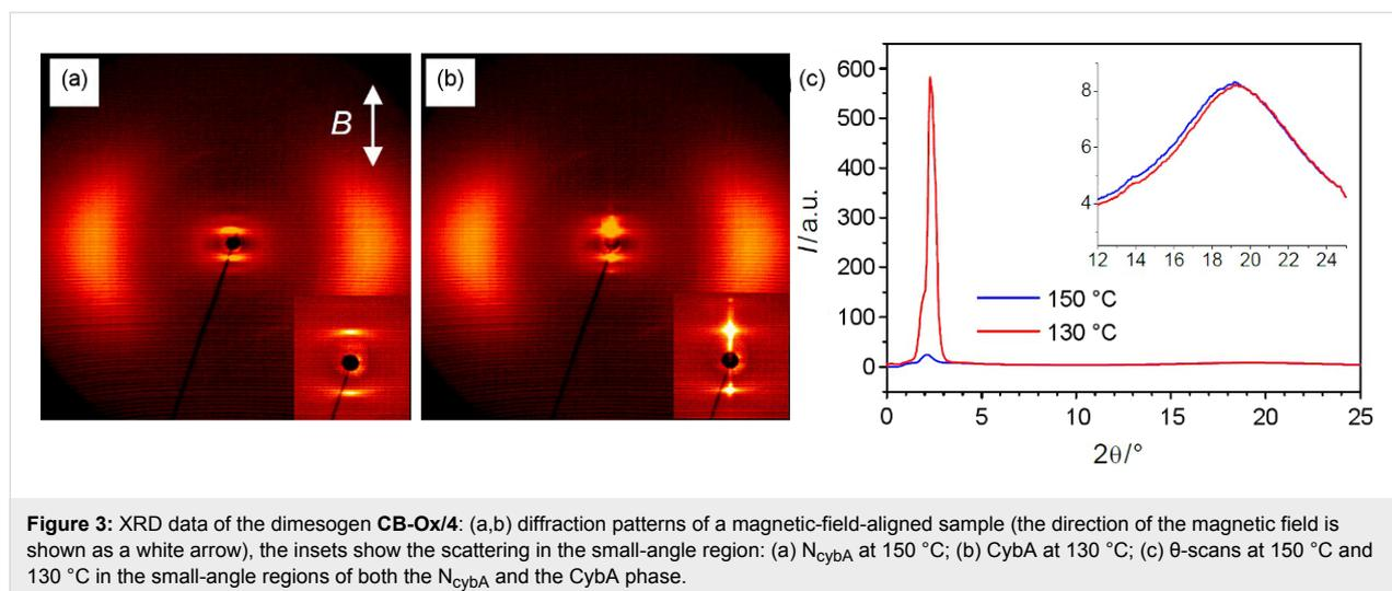
**Figure 3:** XRD data of the dimesogen **CB-Ox/4**: (a,b) diffraction patterns of a magnetic-field-aligned sample (the direction of the magnetic field is shown as a white arrow), the insets show the scattering in the small-angle region: (a)  $N_{\text{cybA}}$  at 150 °C; (b)  $\text{CybA}$  at 130 °C; (c)  $\theta$ -scans at 150 °C and 130 °C in the small-angle regions of both the  $N_{\text{cybA}}$  and the  $\text{CybA}$  phase.
