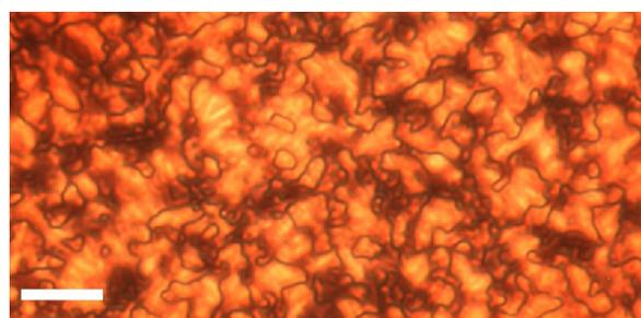
**Figure 15:** Threaded nematic texture of **Au@C<sub>12</sub>/13** as observed by POM at RT. Scale bar = 10 μm. Reprinted with permission from [65]. Copyright 2009 Wiley-VCH Publishers.
