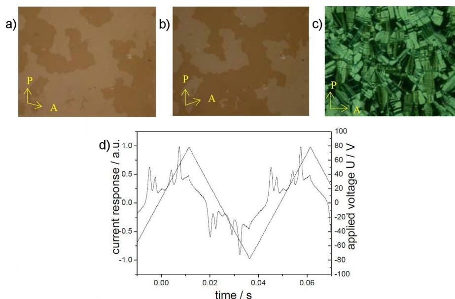
**Figure 20:** Compound **OH 5b**: a), b) Chiral domains at 175 °C, 0 V, polarisers uncrossed by about  $\pm 8^\circ$  from the  $90^\circ$  position; c) birefringent texture formed under an electric field ( $U = 100 \text{ V}_{A.C.}$ ); d) current response ( $U = 158 \text{ V}_{pp}$ ,  $f = 20 \text{ Hz}$ ,  $T = 174 \text{ }^\circ\text{C}$ ,  $d_{\text{cell}} = 6 \text{ }\mu\text{m}$ ).
