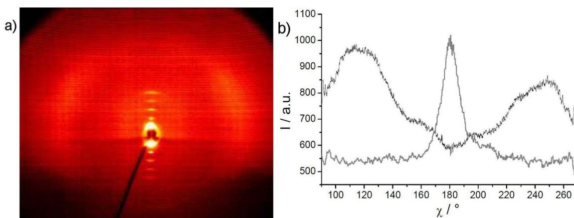
**Figure 11:** a) 2D X-ray pattern of a surface-aligned sample of compound **OH 3b** at 160 °C (lower part of the pattern shadowed by the heating stage); b)  $\chi$ -scan for the diffuse scattering (black line), compared to the position of the layer reflections on the meridian (grey line).
