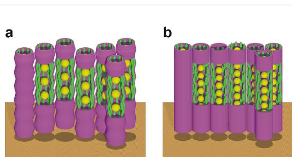
**Figure 16:** Schematic representation of the gold NP columnar structures. (a) Rhombohedral phase in **Au@C<sub>12</sub>/13** and (b) hexagonal columnar phase in **Au@C<sub>6</sub>/13**. Gold NPs = yellow, ligands = green. Reprinted with permission from [65]. Copyright 2009 Wiley-VCH Publishers.
