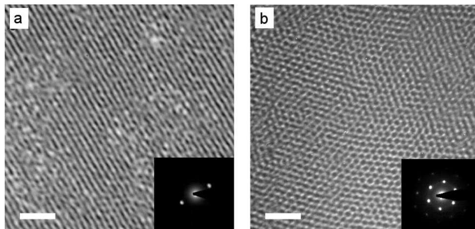
**Figure 17:** TEM images of thin films of the  $R\bar{3}m$  phase of **Au@C<sub>12/13</sub>** recorded with the beam (a) parallel to the  $(1\bar{1}1)$  plane and (b) parallel to the  $[001]$  axis. Scale bar = 20 nm. Insets show the corresponding electron-diffraction patterns. Reprinted with permission from [65]. Copyright 2009 Wiley-VCH Publishers.
