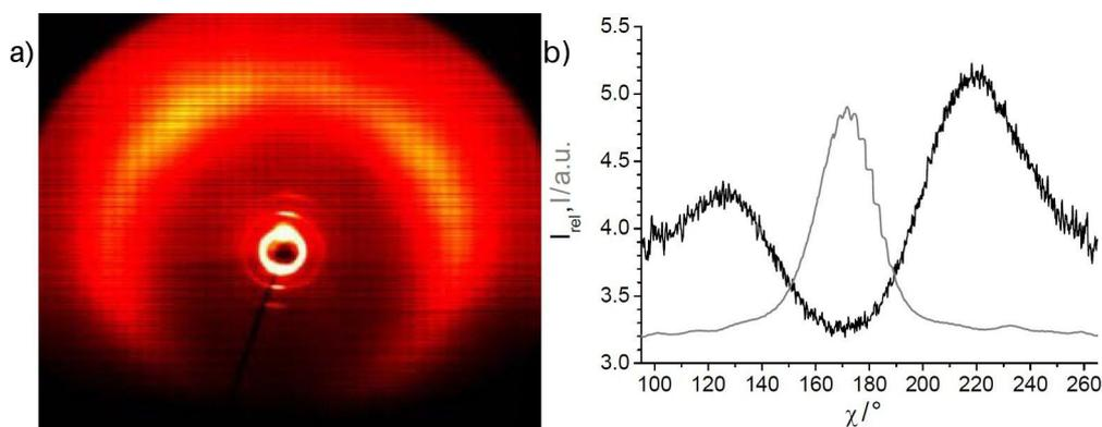
**Figure 6:** a) 2D X-ray pattern of a surface-aligned sample of compound **OH 2a** at 128 °C (lower part of the pattern shadowed by the heating stage); b)  $\chi$  scan for the outer diffuse scattering with maxima at  $\chi \approx 125$  and  $220^\circ$  [ $I_{\text{rel}} = I(128^\circ)/I(140^\circ)$ , isotropic liquid], and the position of the layer reflections for comparison (gray line).
