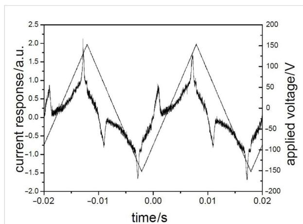
**Figure 23:** Current response of compound **OH 6b** exhibiting two repolarisation peaks proving an antiferroelectric switching ( $U_{A.C.} = 15$  V/  $\mu\text{m}$ ,  $f = 50$  Hz,  $T = 174$  °C,  $d_{\text{cell}} = 6$   $\mu\text{m}$ ).
