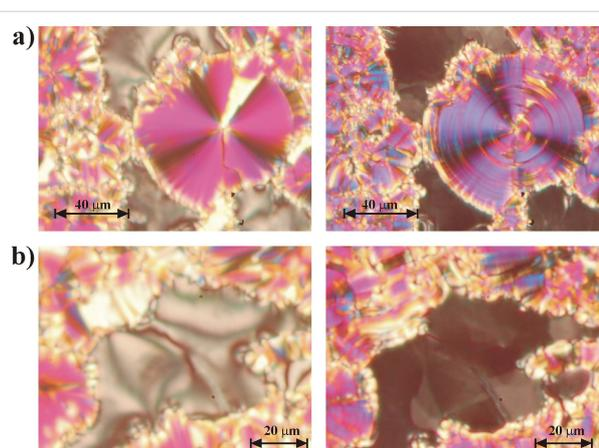
**Figure 8:** Textures of the pure compound **PhP16** on cooling. Left: SmC phase at 96.8 °C Right: same positions in the SmF phase at 82.7 °C. (a) In the upper part a fan-shaped texture is shown, while (b) in the lower part a homeotropic texture can be seen.
