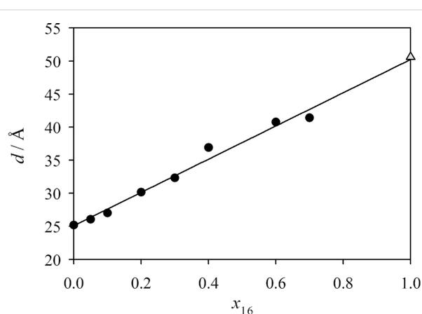
**Figure 4:** The layer spacing obtained by SAXS-measurements in the SmA phase at  $T = T_c$  is plotted against the mole fraction  $x_{16}$  (closed circles) as well as the molecular length for pure **PhP16** calculated by molecular modelling (grey triangle).
