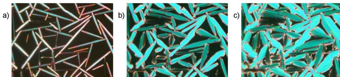
**Figure 10:** Growth of a fan-shaped texture from lancetlike filaments upon cooling of the isotropic liquid of compound **OH 3b**.
