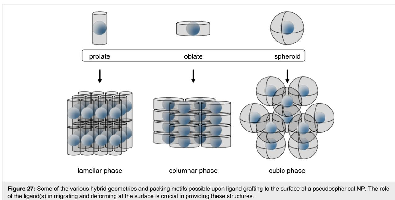
**Figure 27:** Some of the various hybrid geometries and packing motifs possible upon ligand grafting to the surface of a pseudospherical NP. The role of the ligand(s) in migrating and deforming at the surface is crucial in providing these structures.
