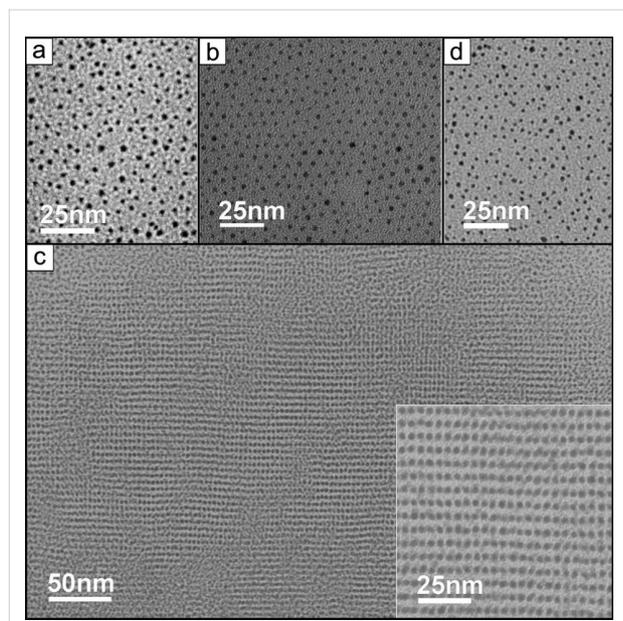
**Figure 26:** TEM images of Au@**23<sub>5,12</sub>** prepared from aged solutions stood for 10 days in solutions of (a) 1:1 MeOH/toluene (disordered), (b) 2:1 MeOH/toluene (hcp), (c) 3:1 MeOH/toluene (stripelike; inset is an expansion), (d) 4:1 MeOH/toluene (disordered). Reprinted with permission from [94]. Copyright 2007 American Chemical Society.
