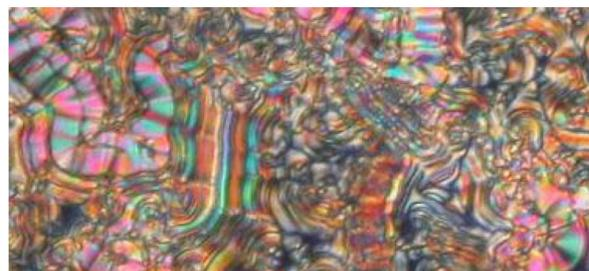
**Figure 5:** Compound **OH 2a**: Texture of the SmCP phase at 126 °C.
