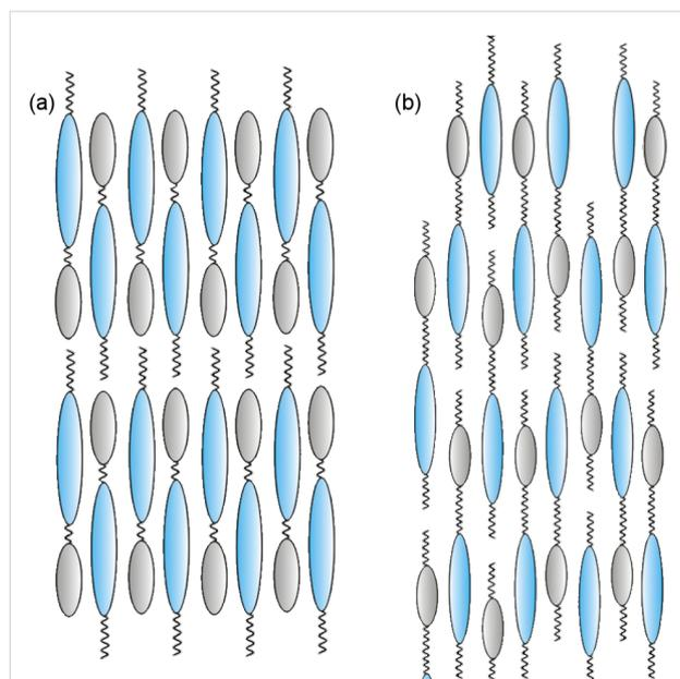
**Figure 4:** Models showing the suggested organizations of dimesogens in the smectic phases and in the preferred local structure in the cybotactic clusters of the related nematic phases: (a) monolayer structure ( $d \sim L$ ); (b) intercalated structure ( $d \sim \frac{1}{2}L$ ). The molecular tilt and the bent-shape of the mesogenic units are not considered.
