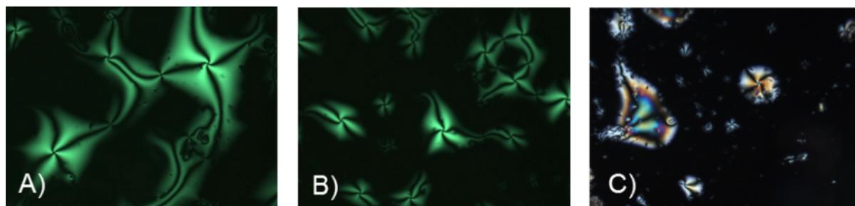
**Figure 4:** Schlieren textures of **13a** and **13b** under crossed polarizers upon cooling (cooling rate 5 K/min) from the isotropic liquid (magnification 200×): (A) **13b** (61 °C), (B) **13b** at 61 °C, different section, (C) **13a** (46 °C).
