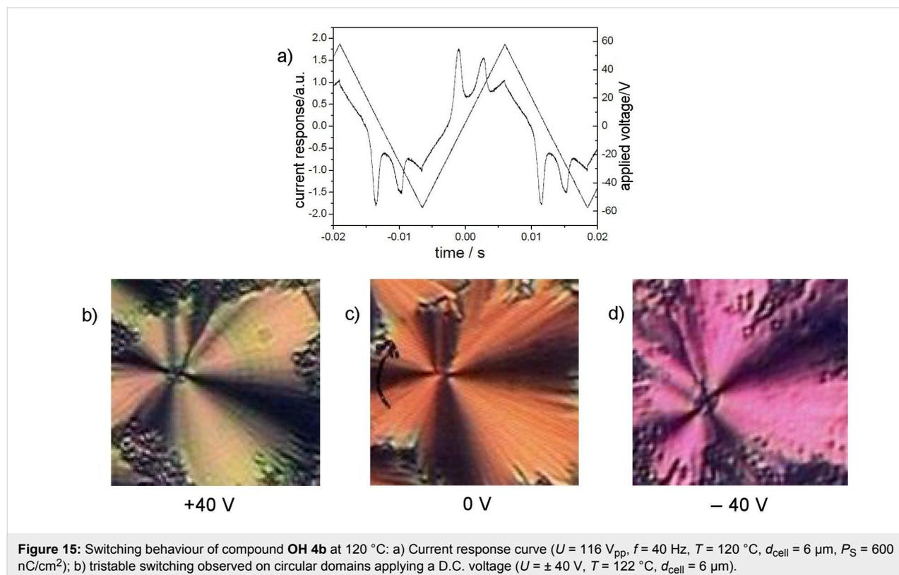
**Figure 15:** Switching behaviour of compound **OH 4b** at  $120$  °C: a) Current response curve ( $U = 116$  V<sub>pp</sub>,  $f = 40$  Hz,  $T = 120$  °C,  $d_{\text{cell}} = 6$  μm,  $P_S = 600$  nC/cm<sup>2</sup>); b) tristable switching observed on circular domains applying a D.C. voltage ( $U = \pm 40$  V,  $T = 122$  °C,  $d_{\text{cell}} = 6$  μm).
