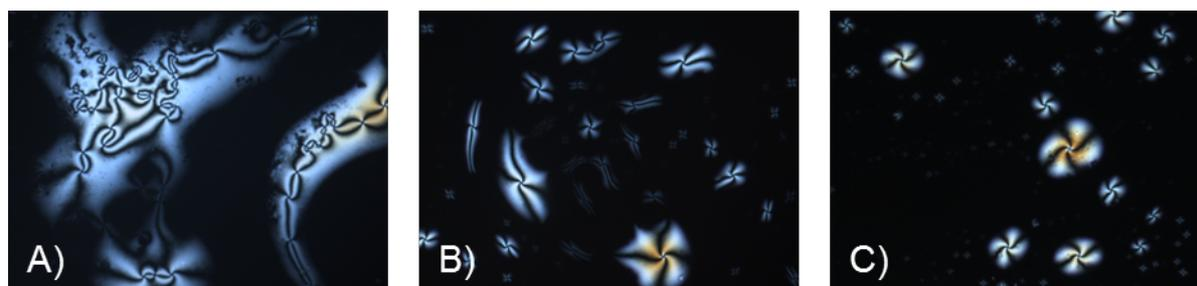
**Figure 3:** Schlieren textures of **11a** and **11b** under crossed polarizers, upon cooling (cooling rate 5 K/min) from the isotropic liquid (magnification 200×): (A) **11a** (20 °C), (B) **11a** (14 °C), (C) **11b** (29 °C).
