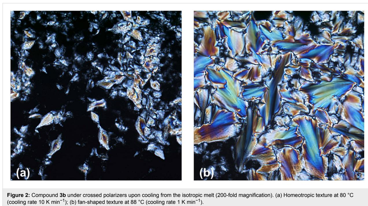
Figure 2: Compound **3b** under crossed polarizers upon cooling from the isotropic melt (200-fold magnification). (a) Homeotropic texture at  $80 \text{ }^\circ\text{C}$  (cooling rate  $10 \text{ K min}^{-1}$ ); (b) fan-shaped texture at  $88 \text{ }^\circ\text{C}$  (cooling rate  $1 \text{ K min}^{-1}$ ).
