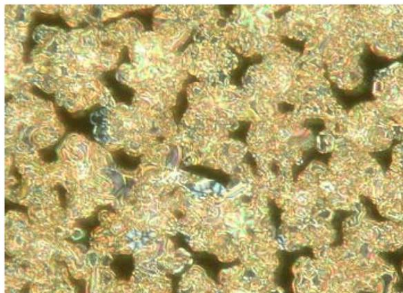
**Figure 24:** On cooling the isotropic liquid phase of compound **OH 6c**; a Schlieren texture together with fringe pattern appears characteristic for SmCP<sub>A</sub> phases.
