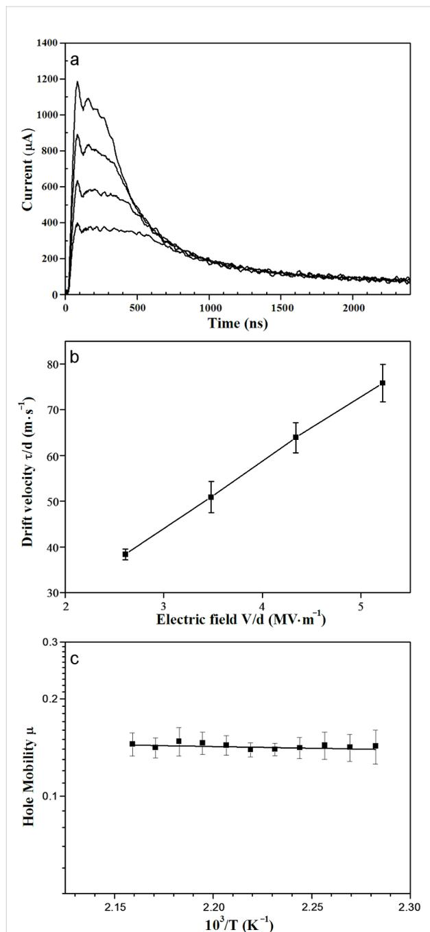
**Figure 3:** (a) Time-of-flight hole transients for an ITO/7c/ITO cell with the liquid crystal in its Col<sub>h</sub> phase at 185 °C. Applied voltages 60 V (top trace), 80 V, 100 V, 120 V (bottom trace). (b) Drift velocity as a function of electric field (185 °C). (c) Temperature-dependence of the hole mobility within the Col<sub>h</sub> phase. The error bars represent 2σ.
