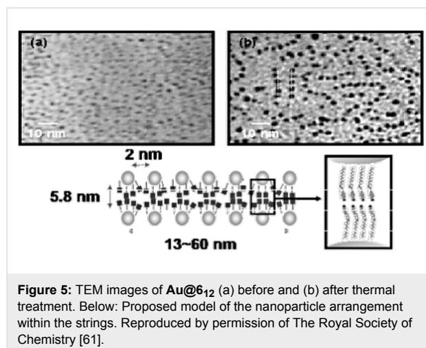
**Figure 5:** TEM images of Au@6<sub>12</sub> (a) before and (b) after thermal treatment. Below: Proposed model of the nanoparticle arrangement within the strings. Reproduced by permission of The Royal Society of Chemistry [61].
