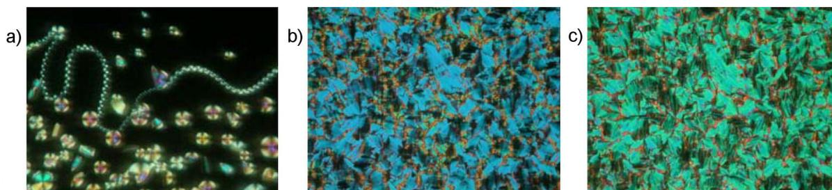
**Figure 8:** Optical photomicrographs of compound **OH 3a**: a) On cooling of the isotropic liquid; c)  $U = 0$  V; b)  $U_{D.C.} = \pm 67$  V,  $T = 172$  °C,  $d_{cell} = 6$   $\mu\text{m}$ .
