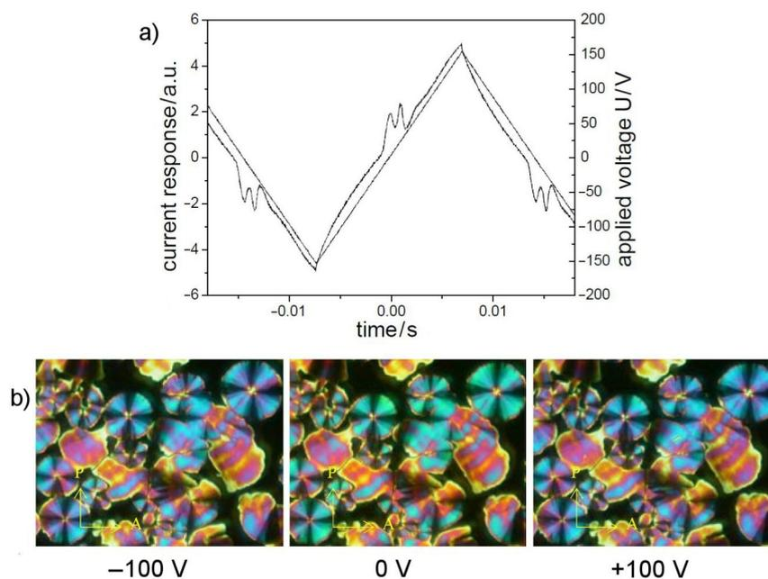
**Figure 9:** Electro-optical behaviour of compound **OH 3a**: a) Current response curve ( $U = 308$  V<sub>pp</sub>,  $f = 35$  Hz,  $T = 172$  °C,  $d_{cell} = 6$   $\mu\text{m}$ ,  $P_S = 370$  nC/cm<sup>2</sup>); b) texture of the  $\text{SmCP}_A$  phase depending on the polarity of the applied field.
