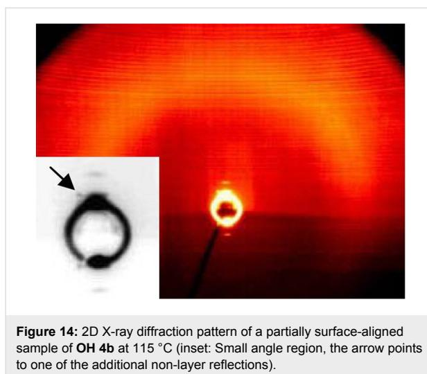
**Figure 14:** 2D X-ray diffraction pattern of a partially surface-aligned sample of **OH 4b** at  $115$  °C (inset: Small angle region, the arrow points to one of the additional non-layer reflections).
