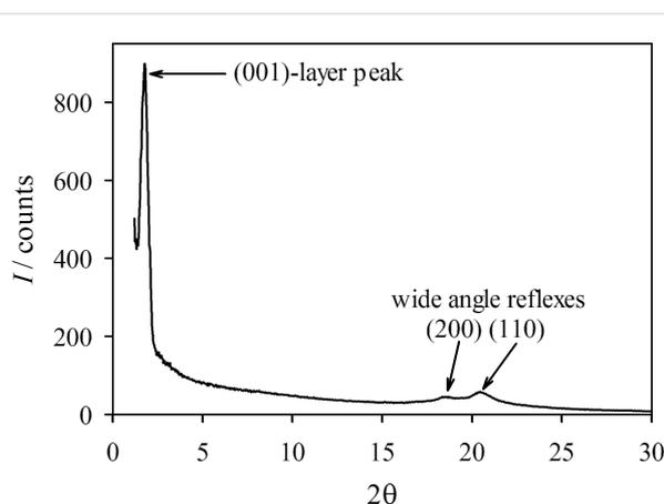
**Figure 9:** Integrated intensity profile of an unoriented sample of **PhP16** at  $T = 82.5$  °C in the SmF phase.
