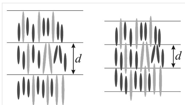
**Figure 1:** Smectic A phase of a mixture of two mesogens differing strongly in molecular length. Left: The layer spacing corresponds to the length of the long mesogen; no out-of-layer fluctuations occur. This leads to a lot of unfavorable free volume. Right: By reducing the smectic translational order the molecules are now densely packed. This leads to extensive out-of-layer fluctuations. Reproduced after [1].
