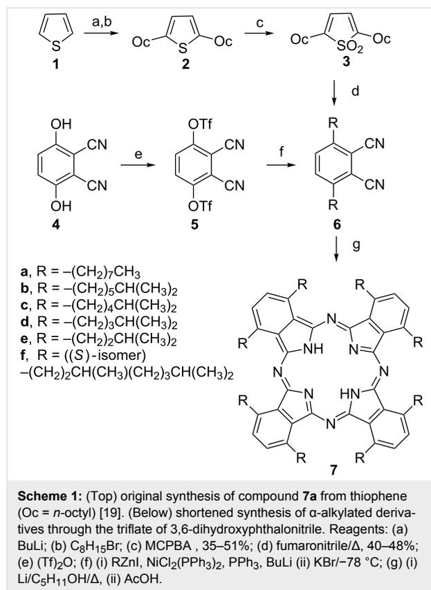
**Scheme 1:** (Top) original synthesis of compound **7a** from thiophene (Oc = *n*-octyl) [19]. (Below) shortened synthesis of  $\alpha$ -alkylated derivatives through the triflate of 3,6-dihydroxyphthalonitrile. Reagents: (a) BuLi; (b)  $C_8H_{15}Br$ ; (c) MCPBA, 35–51%; (d) fumaronitrile/ $\Delta$ , 40–48%; (e)  $(Tf)_2O$ ; (f) (i) RZnI,  $NiCl_2(PPh_3)_2$ ,  $PPh_3$ , BuLi (ii) KBr/ $-78^\circ C$ ; (g) (i)  $Li/C_5H_{11}OH/\Delta$ , (ii) AcOH.
