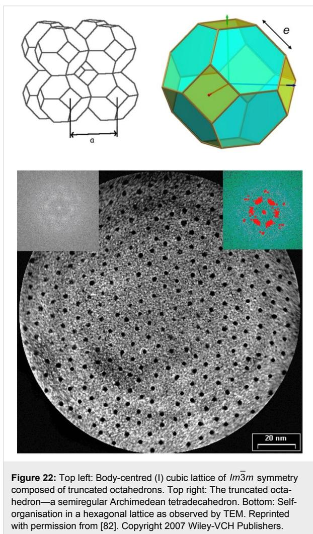
The dendronised nanoparticles spontaneously self-assembled into a hexagonal lattice on the TEM grid: The mean distances between first and second neighbours were about 7.6 and 13.7 nm, respectively, in very good agreement with the NP diameter and the dendritic shell (Figure 22). This system also
