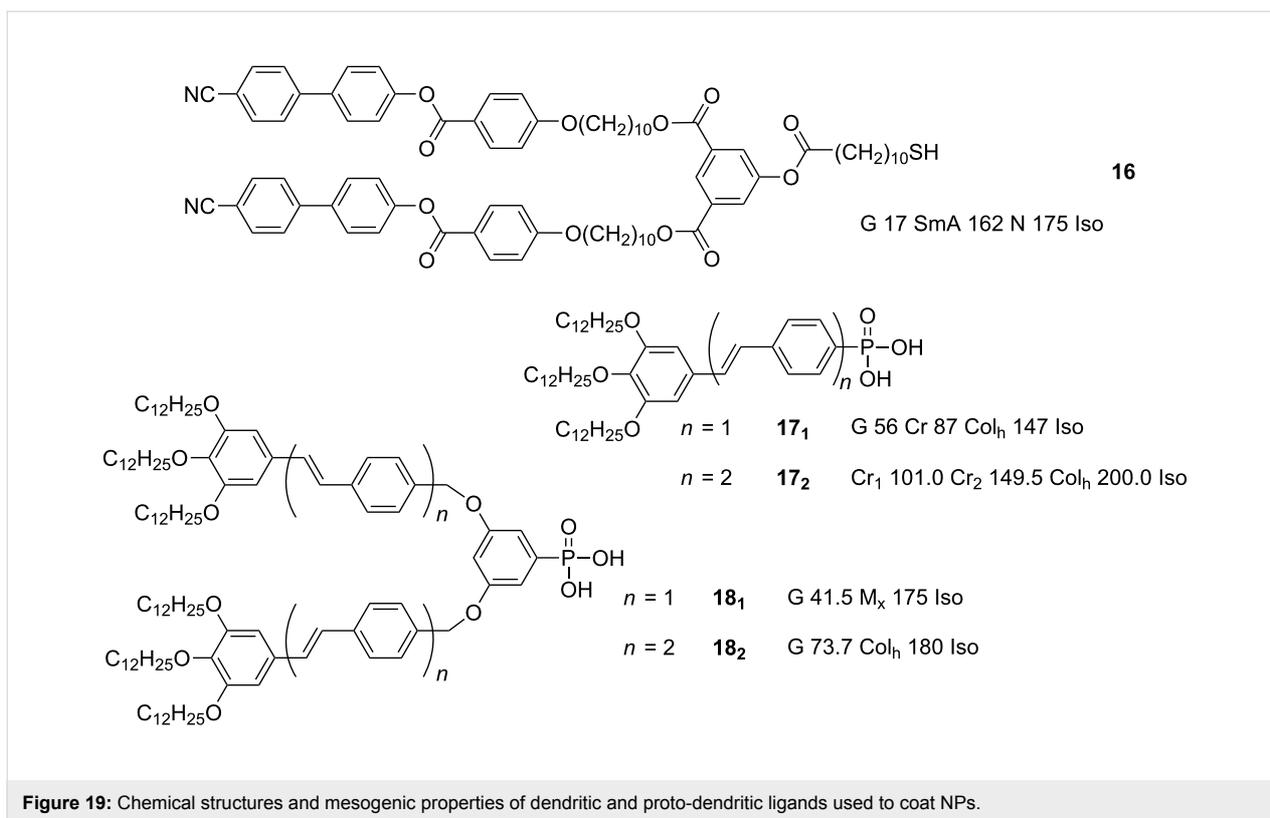
**Figure 19:** Chemical structures and mesogenic properties of dendritic and proto-dendritic ligands used to coat NPs.
