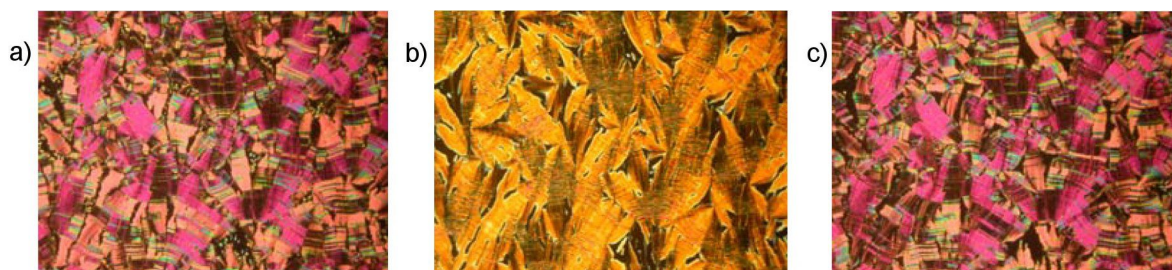
Figure 17: Electro-optical behaviour observed on the fan-shaped texture of compound OH 4d ; U_{\text{D.C.}} = 47 \text{ V} ; T = 123^\circ\text{C} ; a) -47 \text{ V} ; b) 0 \text{ V} ; c) +47 \text{ V} .
