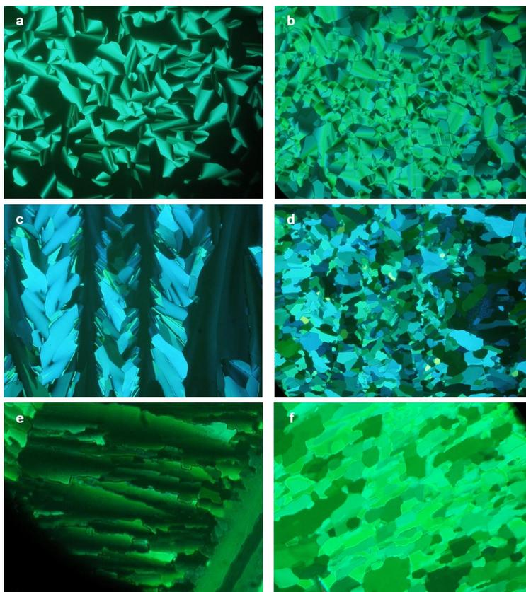
**Figure 2:** Optical micrographs taken with crossed polarisers and at a magnification of  $\times 20$ . (a) *n*-Octyl derivative **7a** in the  $Col_h$  phase at 145 °C. (b) **7a** in the  $Col_r$  phase at 100 °C. (c) Isooctyl derivative **7b** in the  $Col_h$  phase at 170 °C. (d) **7b** in the unknown (but probably Cr) phase at 120 °C. (e) Isoheptyl derivative **7c** in the  $Col_h$  phase at 170 °C. (f) **7c** in the Cr phase at 155 °C.
