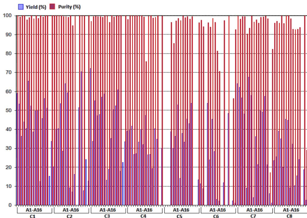
**Figure 3:** Results for the synthesis of a 128-member library of aminated coumarins by using the Chemspeed SLT100 automated synthesizer. Purified by an automated preparative reverse-phase HPLC (Waters 2767 Mass Directed Fractionation) detected by UV (270 nm). Purity was determined by reverse-phase HPLC (Waters Alliance 2795 system) with peak area (UV) at 214 nm.
