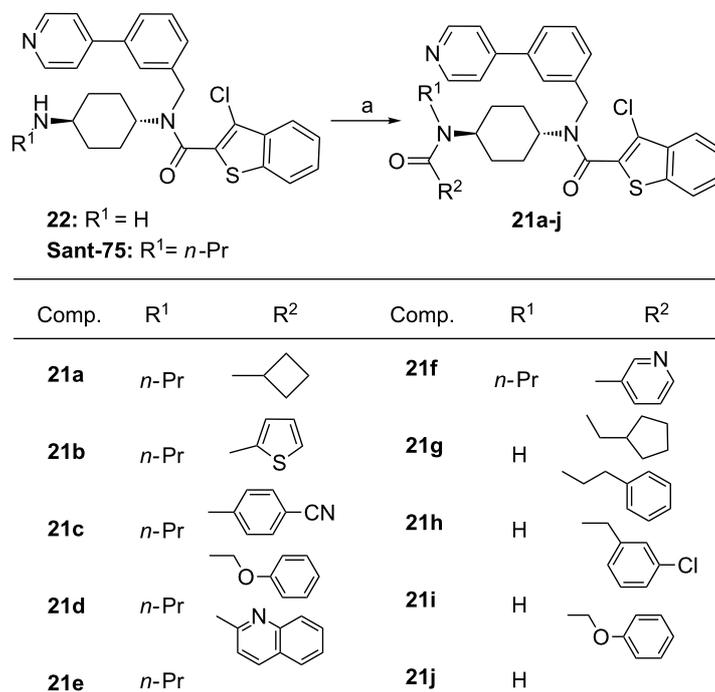
**Scheme 7:** Chemical modifications on the motif D. Reagents and conditions: (a) R<sup>2</sup>COCl, CH<sub>2</sub>Cl<sub>2</sub>.
