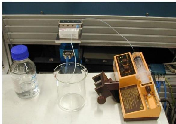
**Figure 5:** Test setup with continuously operating, miniaturized photoreactor.
