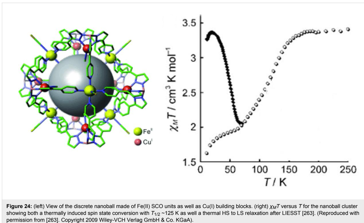
**Figure 24:** (left) View of the discrete nanoball made of  $\text{Fe}(\text{II})$  SCO units as well as  $\text{Cu}(\text{I})$  building blocks. (right)  $\chi_M T$  versus  $T$  for the nanoball cluster showing both a thermally induced spin state conversion with  $T_{1/2} \sim 125$  K as well as a thermal HS to LS relaxation after LIESST [263]. (Reproduced with permission from [263]. Copyright 2009 Wiley-VCH Verlag GmbH & Co. KGaA).
