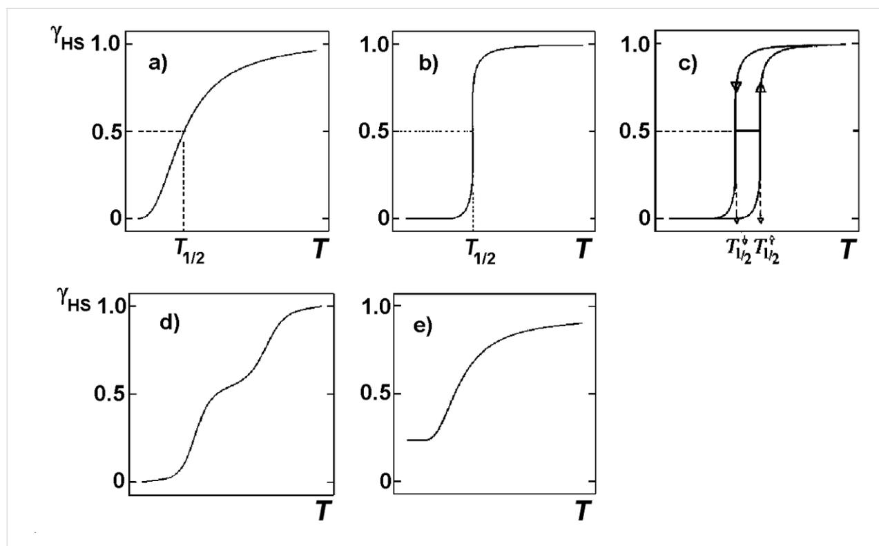
**Figure 2:** Types of spin transition curves in terms of the molar fraction of HS molecules,  $\gamma_{\text{HS}}(T)$ , as a function of temperature [23]. (Reproduced with permission from [27]. Copyright 2003 Wiley-VCH Verlag GmbH & Co. KGaA).
