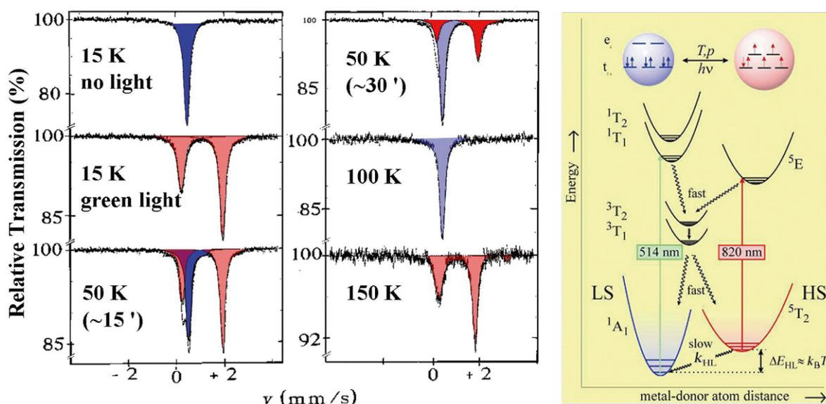
**Figure 6:** (left) Demonstration of light-induced spin state trapping (LIESST) in  $[\text{Fe}(\text{ptz})_6]\text{BF}_4)_2$  with  $^{57}\text{Fe}$  Mössbauer spectroscopy (for details see text). (right) Jablonski diagram showing the photophysical processes of the LIESST and reverse-LIESST effects [23]; details are described in the text (Reproduced with permission from [36]. Copyright 2012 Wiley-VCH Verlag GmbH & Co. KGaA).
