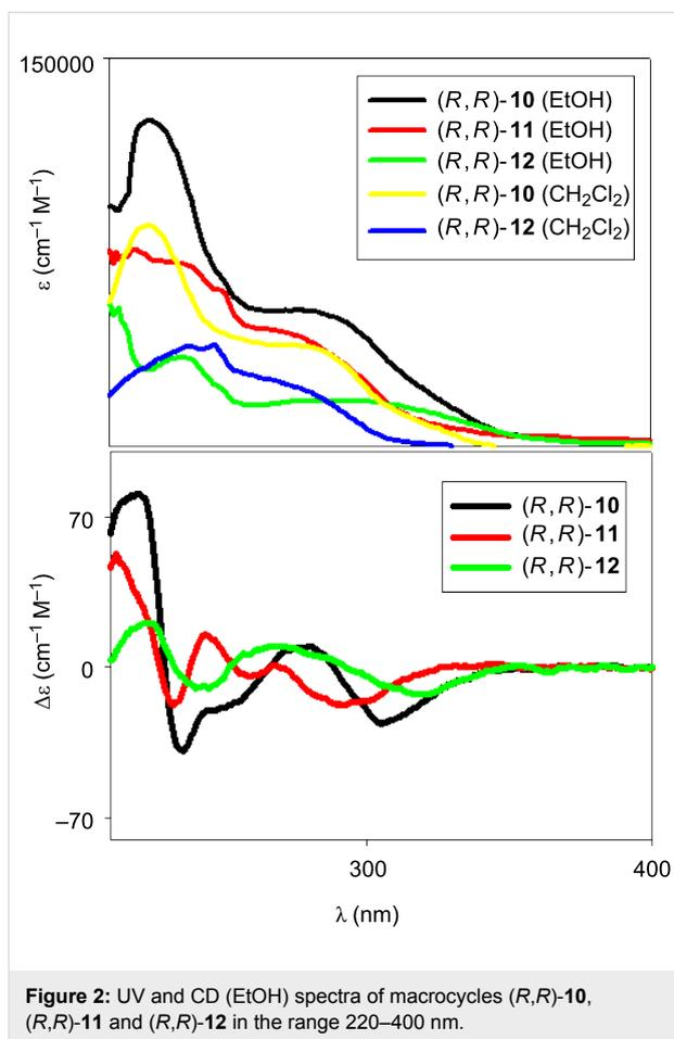
**Figure 2:** UV and CD (EtOH) spectra of macrocycles (*R,R*)-**10**, (*R,R*)-**11** and (*R,R*)-**12** in the range 220–400 nm.
