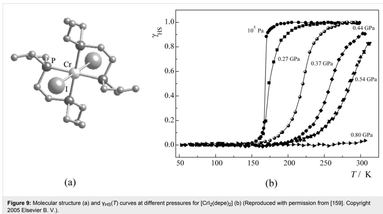
**Figure 9:** Molecular structure (a) and  $\gamma_{\text{HS}}(T)$  curves at different pressures for  $[\text{Cr}_2(\text{depe})_2]$  (b) (Reproduced with permission from [159]. Copyright 2005 Elsevier B. V.).
