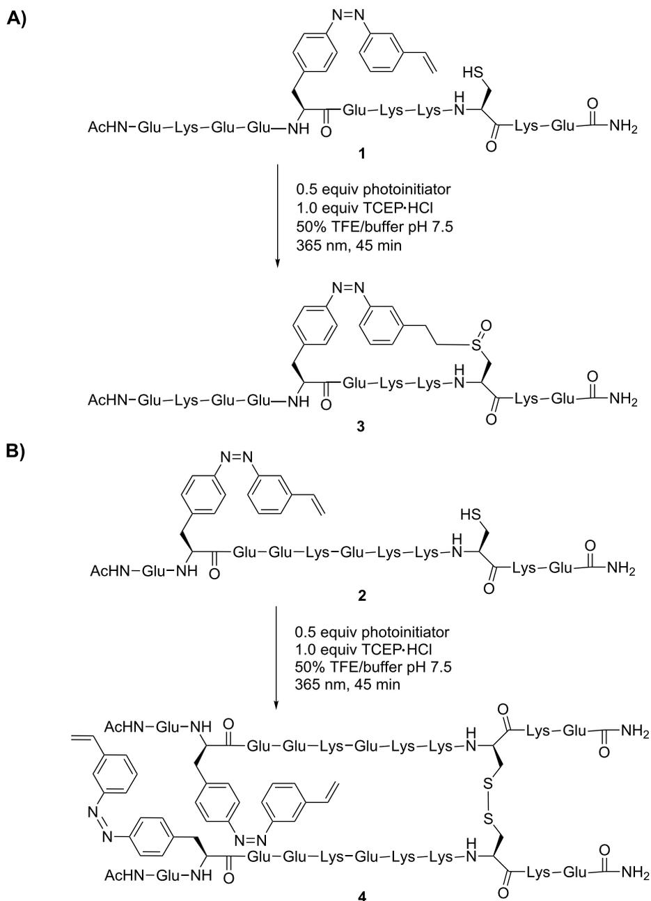
**Scheme 2:** Thiol–ene click reaction of PSCaa with cysteine within the helical model peptides **1** ( $i,i+4$ ) and **2** ( $i,i+7$ ) under structure-inducing conditions in the presence of trifluoroethanol (50%).
