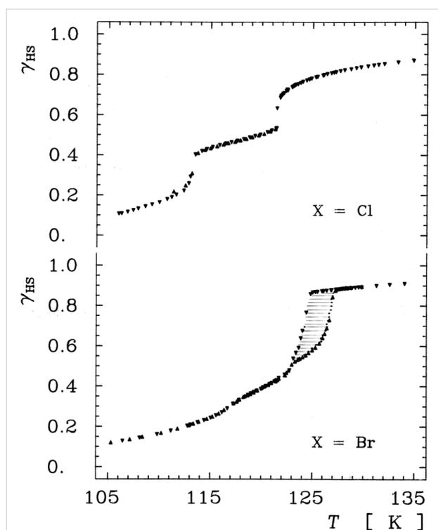
**Figure 13:** Influence of the noncoordinated anion on the spin transition curve  $\gamma_{\text{HS}}(T)$  near the transition temperature  $T_{1/2}$  in  $[\text{Fe}(\text{II})(2\text{-pic})_3]\text{X}_2 \cdot \text{EtOH}$  ( $\text{X} = \text{Cl}, \text{Br}$ ). (Reproduced with permission from [27]. Copyright 2003 Wiley-VCH Verlag GmbH & Co. KGaA).
