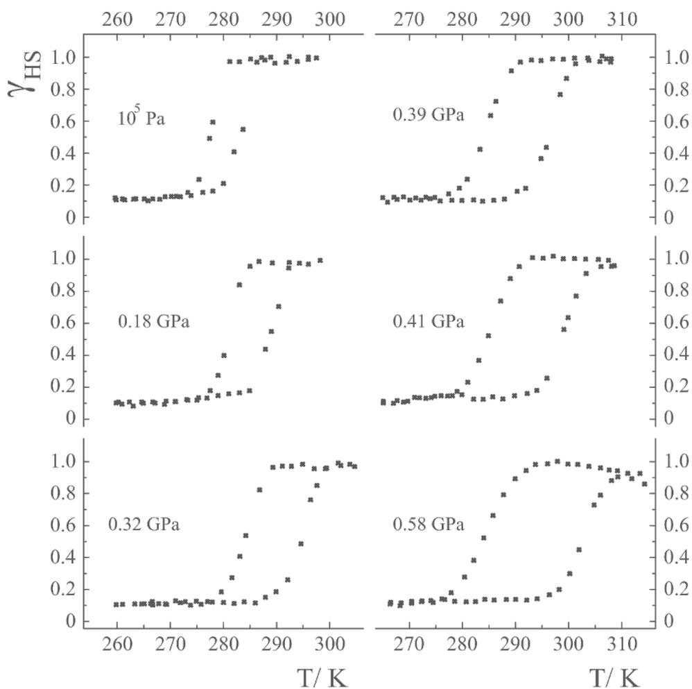
**Figure 10:** HS molar fraction  $\gamma_{\text{HS}}$  versus  $T$  at different pressures for  $[\text{Fe}(\text{phy})_2](\text{BF}_4)_2$ . The hysteresis loop broadens with increasing pressure. (Reproduced with permission from [167]. Copyright 1999 Elsevier B. V.).
