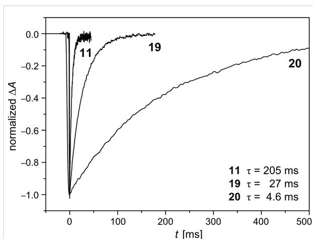
**Figure 20:** Transient absorptions generated by UV irradiation ( $\lambda = 355$  nm) of azo-dyes **11** (*type-II*), **19** (*type-III*) and **20** (*type-III*) in ethanol at 298 K ( $[AZO] = 20 \mu\text{M}$ ,  $\lambda_{\text{obs}} = 370$  nm). From [63] – Reproduced by permission of the Royal Society of Chemistry.
