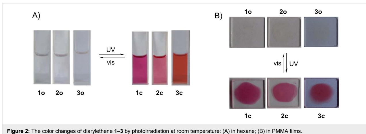
**Figure 2:** The color changes of diarylethene **1–3** by photoirradiation at room temperature: (A) in hexane; (B) in PMMA films.
