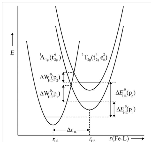
**Figure 7:** Schematic representation of the pressure influence ( $p_2 > p_1$ ) on the LS and HS potential wells of an Fe(II) spin crossover compound (Reproduced with permission from [159]. Copyright 2005 Elsevier B. V.).
