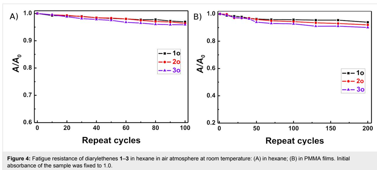
**Figure 4:** Fatigue resistance of diarylethenes **1–3** in hexane in air atmosphere at room temperature: (A) in hexane; (B) in PMMA films. Initial absorbance of the sample was fixed to 1.0.
