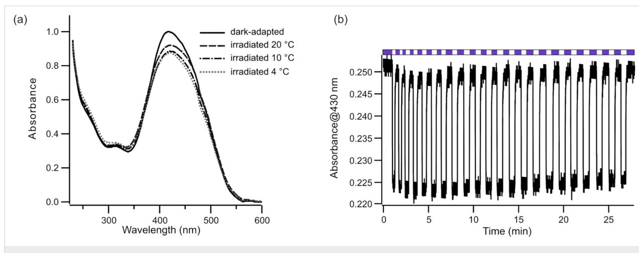
**Figure 3:** (a) Photoswitching of **2** with violet light (407–410 nm) at different temperatures (4, 10 and 20  $^{\circ}$ C) in 25 mM sodium phosphate buffer at pH 8. (b) Multiple rounds of photoswitching of **2** with alternating violet light (violet bars) and dark adaption (white bars) in 25 mM phosphate buffer, pH 8, at 10  $^{\circ}$ C.
