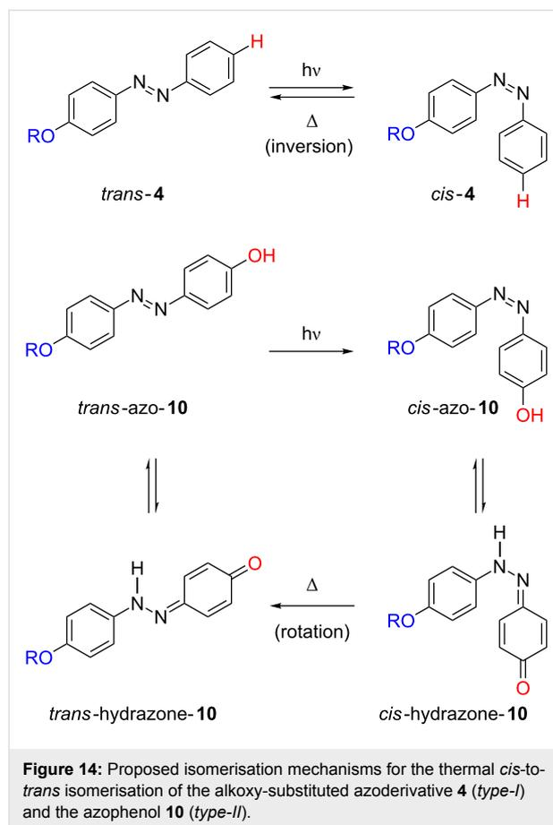
**Figure 14:** Proposed isomerisation mechanisms for the thermal *cis*-to-*trans* isomerisation of the alkoxy-substituted azoderivative **4** (*type-I*) and the azophenol **10** (*type-II*).
