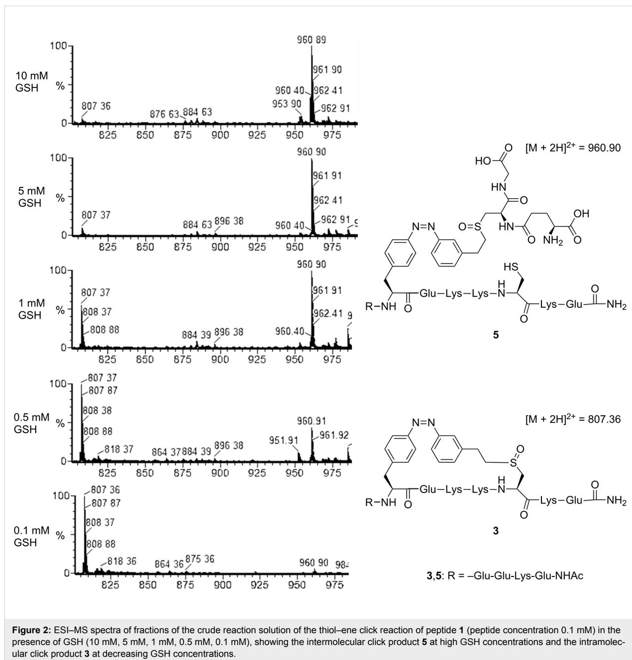
**Figure 2:** ESI-MS spectra of fractions of the crude reaction solution of the thiol–ene click reaction of peptide **1** (peptide concentration 0.1 mM) in the presence of GSH (10 mM, 5 mM, 1 mM, 0.5 mM, 0.1 mM), showing the intermolecular click product **5** at high GSH concentrations and the intramolecular click product **3** at decreasing GSH concentrations.
