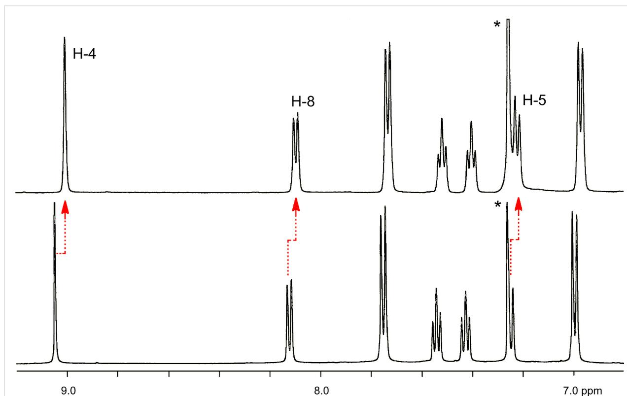
**Figure 4:** Aromatic region of the  $^1\text{H}$  NMR ( $\text{CDCl}_3$ , 500 MHz, 25 °C) spectra of macrocycle (*R,R*)-**12** (2.8 mM, bottom) and at the end of the titration with tetrabutylammonium succinate ( $[(R)-\mathbf{7}] = 2.8$  mM,  $[(\text{CH}_2\text{CO}_2)_2(\text{Bu}_4\text{N})_2] = 28$  mM, top). Asterisks indicate the residual solvent peaks.
