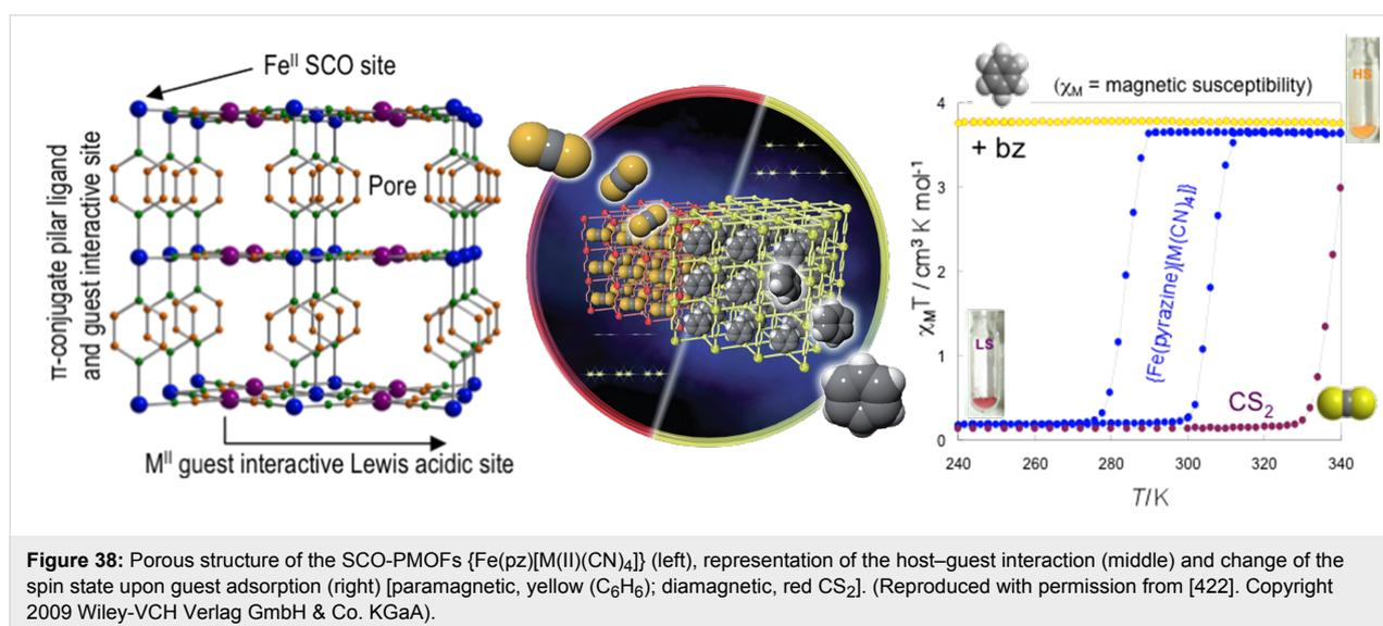
**Figure 38:** Porous structure of the SCO-PMOFs  $\{\text{Fe}(\text{pz})[\text{M}(\text{II})(\text{CN})_4]\}$  (left), representation of the host-guest interaction (middle) and change of the spin state upon guest adsorption (right) [paramagnetic, yellow ( $\text{C}_6\text{H}_6$ ); diamagnetic, red  $\text{CS}_2$ ]. (Reproduced with permission from [422]. Copyright 2009 Wiley-VCH Verlag GmbH & Co. KGaA).
