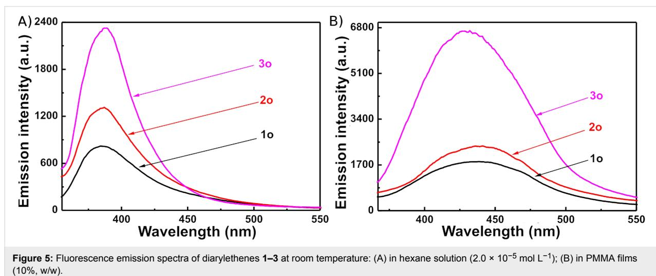
**Figure 5:** Fluorescence emission spectra of diarylethenes **1–3** at room temperature: (A) in hexane solution ( $2.0 \times 10^{-5}$  mol L<sup>-1</sup>); (B) in PMMA films (10%, w/w).
