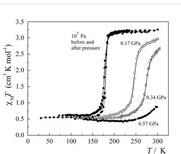
**Figure 8:**  $\chi_{\text{M}}T$  versus  $T$  curves at different pressures for  $[\text{Fe}(\text{phen})_2(\text{NCS})_2]$ , polymorph II. (Reproduced with permission from [159]. Copyright 2005 Elsevier B. V.).
