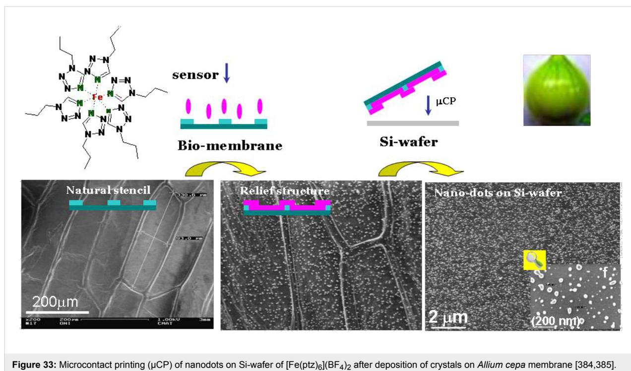
**Figure 33:** Microcontact printing ( $\mu\text{CP}$ ) of nanodots on Si-wafer of  $[\text{Fe}(\text{ptz})_6](\text{BF}_4)_2$  after deposition of crystals on *Allium cepa* membrane [384,385].
