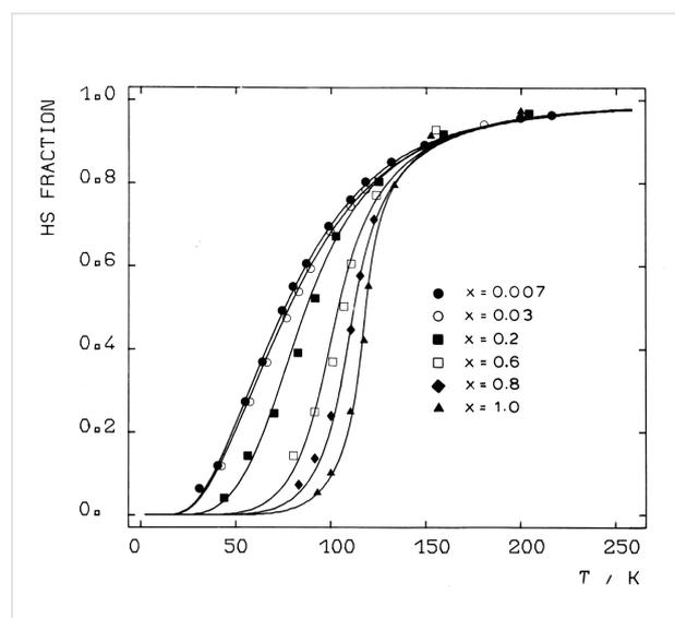
**Figure 12:** Temperature dependence of the HS fraction  $\gamma_{\text{HS}}(T)$ , determined from Mössbauer spectra of  $[\text{Fe}(\text{II})_x\text{Zn}_{1-x}(2\text{-pic})_3]\text{Cl}_2\cdot\text{EtOH}$  for different iron concentrations  $x$ . The ST curves become more gradual with increasing  $x$  due to weakening of the strength of the cooperative interactions. (Reproduced with permission from [27]. Copyright 2003 Wiley-VCH Verlag GmbH & Co. KGaA).
