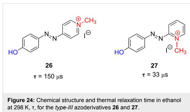
Because of their very fast thermal isomerisation rate, **26** and **27** are the best candidates to be applied as fast information-transmitting photochromic switches. Figure 25 shows the information-transmission capability of azo-dye **26** with time. The repeatability of the different optical oscillators was tested by submitting them to consecutive UV-irradiation–dark cycles. The optical photochromic switches reported show no fatigue (Figure 25).
