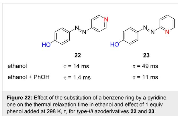
**Figure 22:** Effect of the substitution of a benzene ring by a pyridine one on the thermal relaxation time in ethanol and effect of 1 equiv phenol added at 298 K,  $\tau$ , for *type-III* azoderivatives **22** and **23**.
