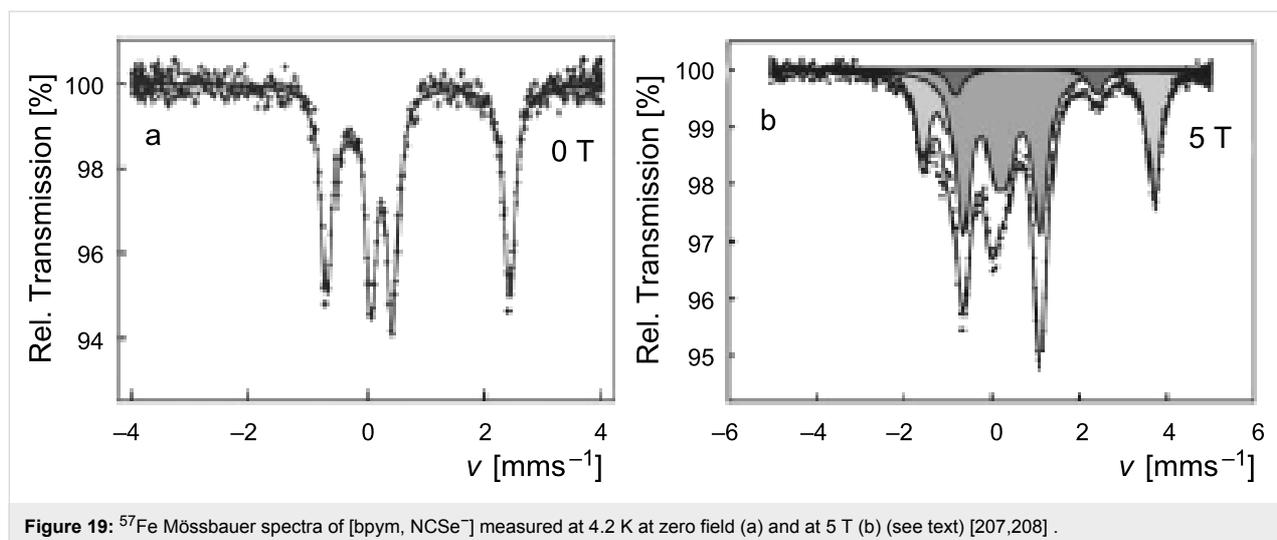
**Figure 19:**  $^{57}\text{Fe}$  Mössbauer spectra of [bpym,  $\text{NCS}^-$ ] measured at 4.2 K at zero field (a) and at 5 T (b) (see text) [207,208].
