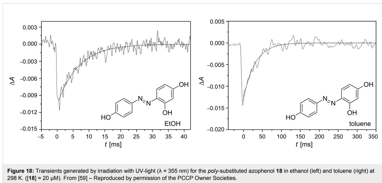
tions at 298 K, respectively (see Figure 8). As mentioned above, the relaxation time of *type-II* azophenols ranged from 400 ms to 6 ms in ethanol, depending on the position of the phenol groups within the azobenzene core. However, both types of azoderivatives are still too slow for use as light-driven real-time information-transmitting systems or photo-driven optical oscillators.
