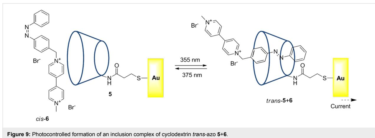
the translation of the optical signals recorded by the bipyridinium azobenzene **6** via a  $\beta$ -cyclodextrin single phase prepared on a gold electrode [109].
