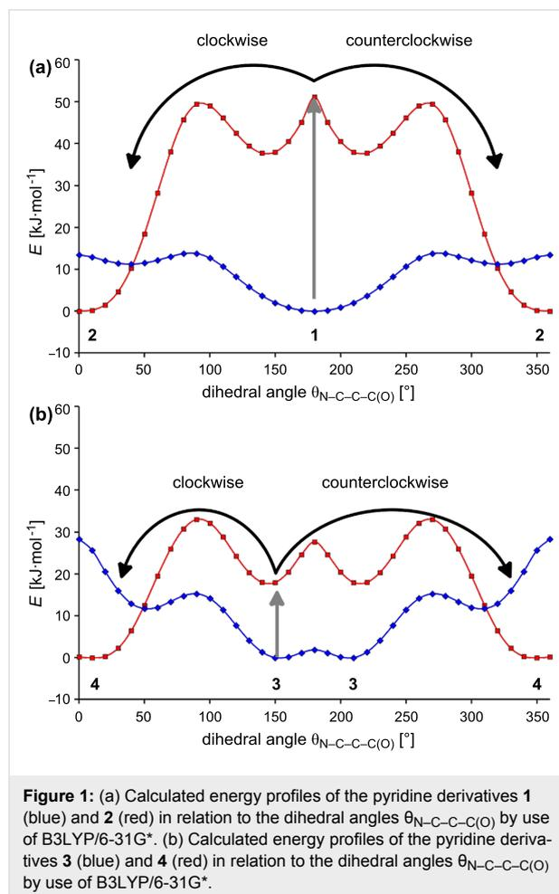
**Figure 1:** (a) Calculated energy profiles of the pyridine derivatives **1** (blue) and **2** (red) in relation to the dihedral angles  $\theta_{\text{N-C-C(O)}}$  by use of B3LYP/6-31G\*. (b) Calculated energy profiles of the pyridine derivatives **3** (blue) and **4** (red) in relation to the dihedral angles  $\theta_{\text{N-C-C(O)}}$  by use of B3LYP/6-31G\*.
