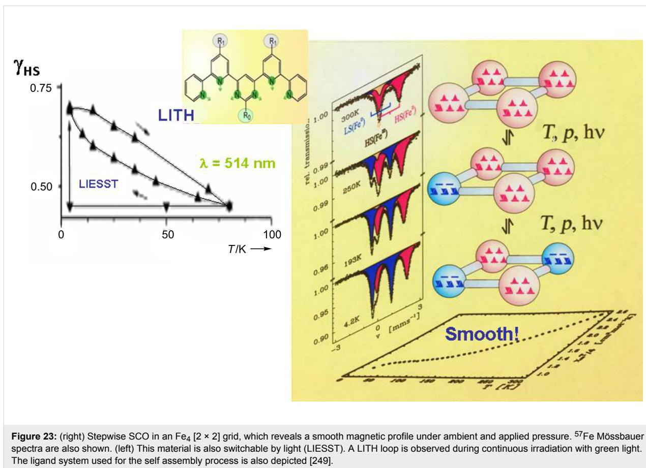
**Figure 23:** (right) Stepwise SCO in an  $\text{Fe}_4 [2 \times 2]$  grid, which reveals a smooth magnetic profile under ambient and applied pressure.  $^{57}\text{Fe}$  Mössbauer spectra are also shown. (left) This material is also switchable by light (LIESST). A LITH loop is observed during continuous irradiation with green light. The ligand system used for the self assembly process is also depicted [249].
