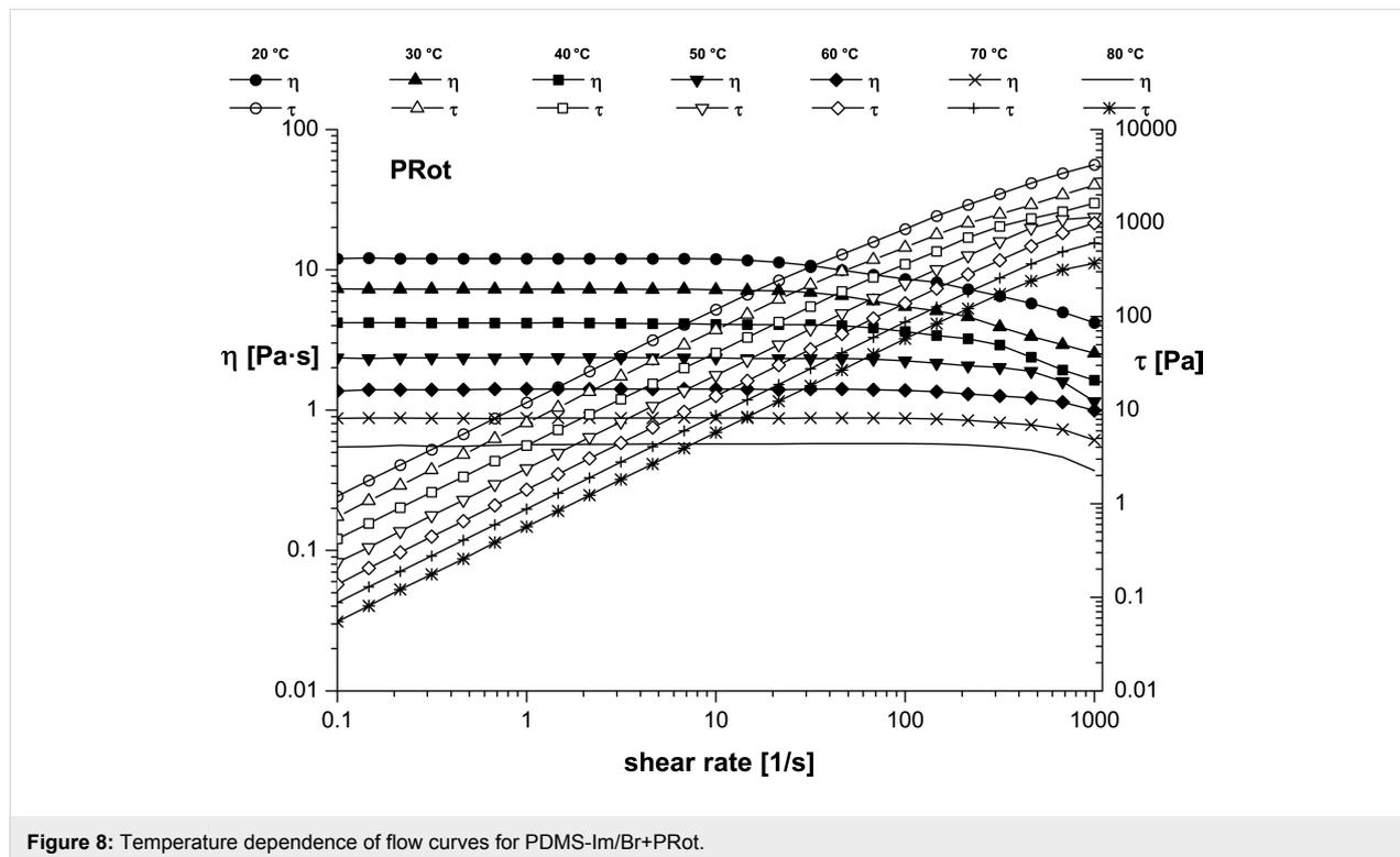
Figure 8: Temperature dependence of flow curves for PDMS-Im/Br+PRot.
