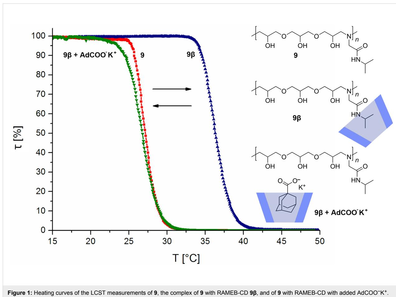
**Figure 1:** Heating curves of the LCST measurements of **9**, the complex of **9** with RAMEB-CD **9β**, and of **9** with RAMEB-CD with added  $\text{AdCOO}^- \text{K}^+$ .
