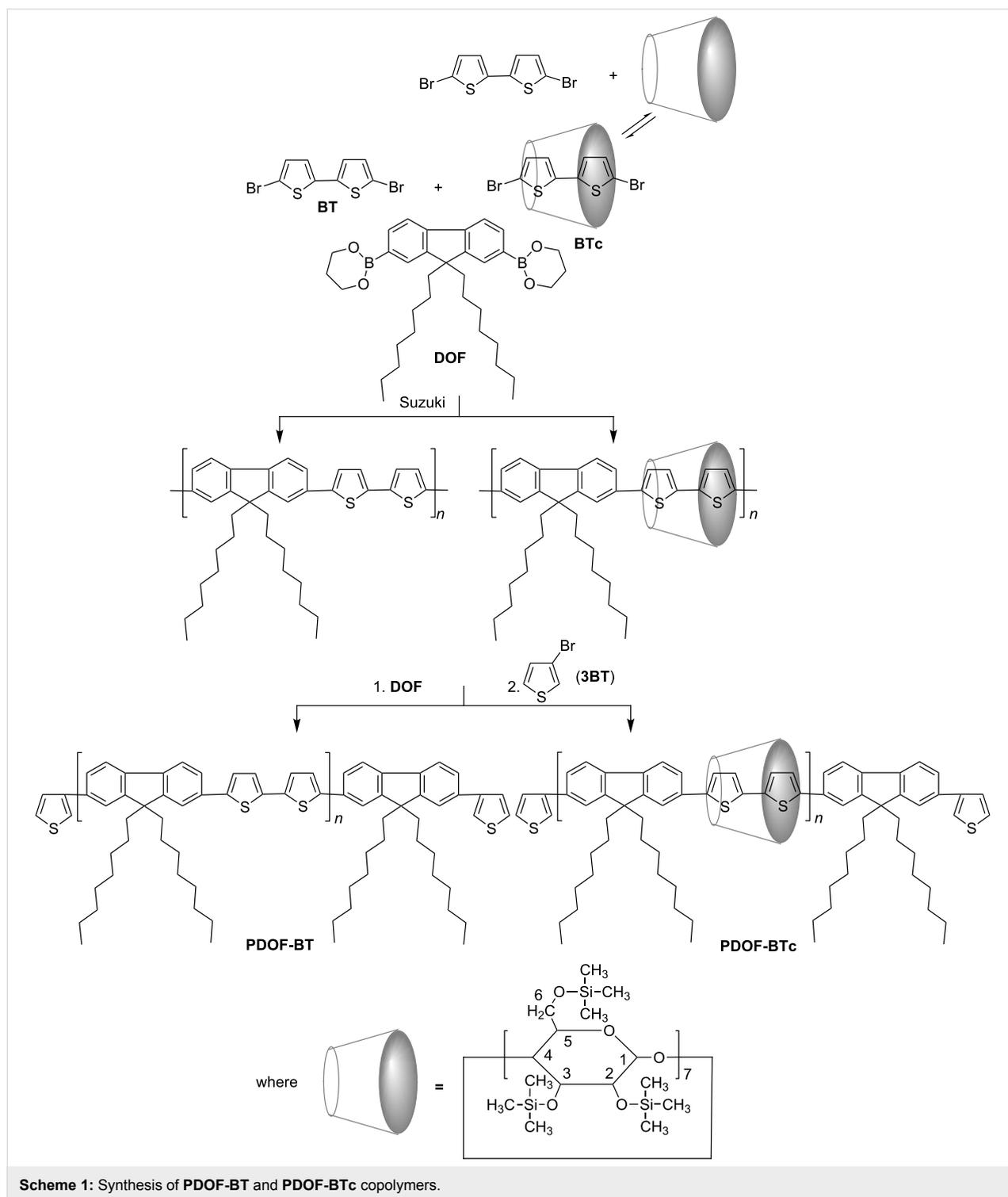
The chemical structure of **PDOF-BTc** (insoluble part in petroleum ether) and **PDOF-BT** copolymers was proved by  $^1\text{H}$  NMR and FTIR analysis. The infrared spectrum of the **PDOF-BTc** (Figure 2B) shows all the characteristic bands of **PDOF-BT** and additional bands located in the  $748\text{--}1251\text{ cm}^{-1}$  region. Note that the peaks at
