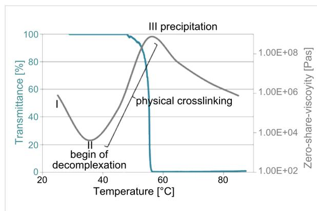
**Figure 3:** Transmittance [%] and zero-shear-viscosity [Pas] as a function of temperature for a 50 wt % solution of polymer **8**. (I → II: Viscosity decreases with higher temperature; II → III: Gradual decomplexation of the polymer, RAMEB-CD molecules slip off from the polymer side chain, aggregates are formed; III: Precipitation of the polymer).
