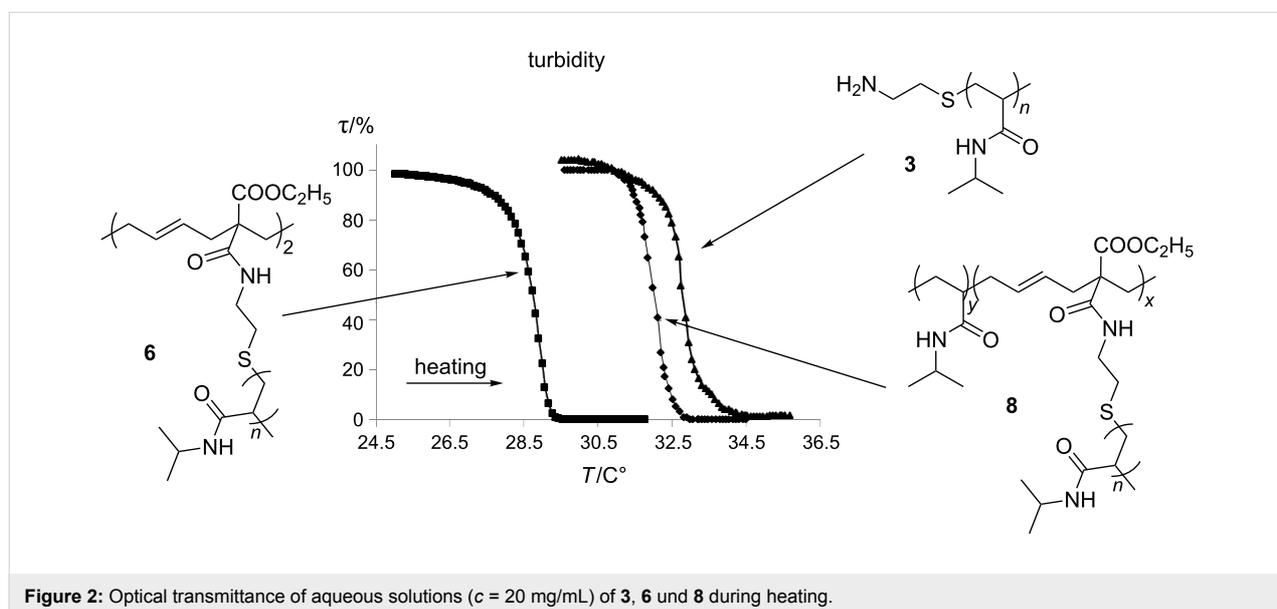
Figure 2: Optical transmittance of aqueous solutions ( $c = 20\text{ mg/mL}$ ) of **3**, **6** and **8** during heating.
