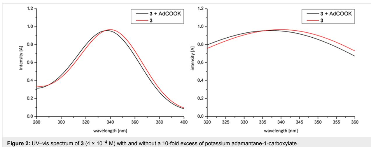
**Figure 2:** UV-vis spectrum of **3** ( $4 \times 10^{-4}$  M) with and without a 10-fold excess of potassium adamantane-1-carboxylate.
