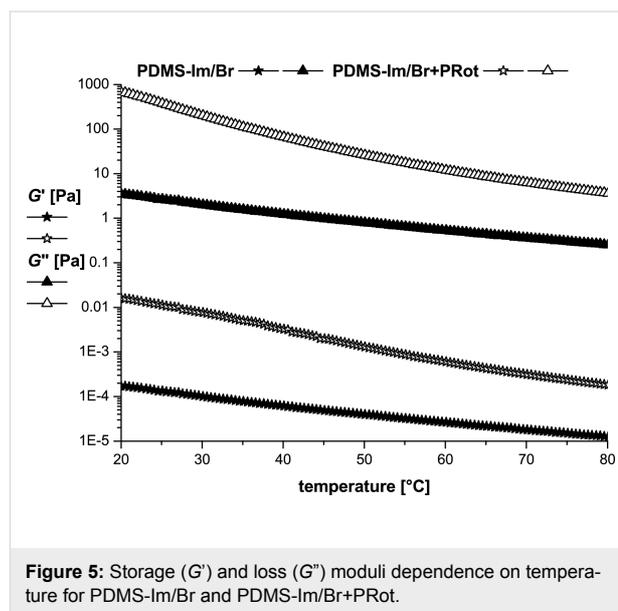
**Figure 5:** Storage ( $G'$ ) and loss ( $G''$ ) moduli dependence on temperature for PDMS-Im/Br and PDMS-Im/Br+PRot.
