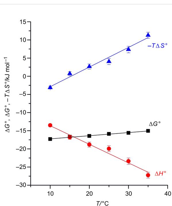
**Figure 2:** Temperature dependence of  $-T\Delta S^\circ$ ,  $\Delta H^\circ$  and  $\Delta G^\circ$  for the inclusion of 1-adamantane carboxylate in heptakis-2,3,6-tri-*O*-methyl- $\beta$ -CD (**3**) measured by ITC.
