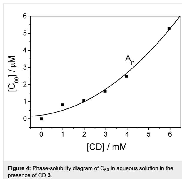
**Figure 4:** Phase-solubility diagram of  $C_{60}$  in aqueous solution in the presence of CD 3.
