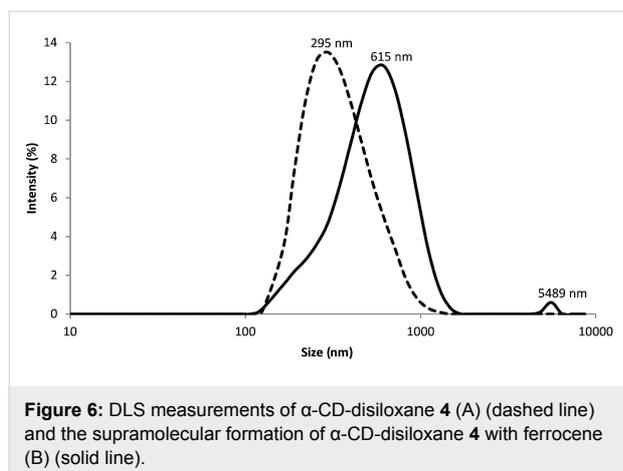
**Figure 6:** DLS measurements of  $\alpha$ -CD-disiloxane **4** (A) (dashed line) and the supramolecular formation of  $\alpha$ -CD-disiloxane **4** with ferrocene (B) (solid line).
