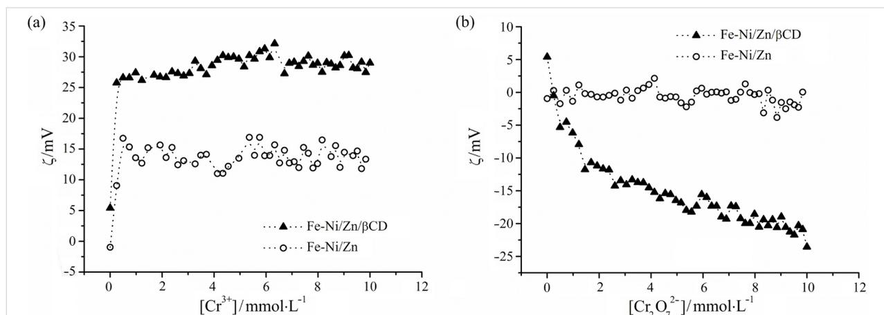
**Figure 8:** Adsorption curves of (a)  $\text{Cr}^{3+}$  and (b)  $\text{Cr}_2\text{O}_7^{2-}$  ions using Fe-Ni/Zn and Fe-Ni/Zn/ $\beta$ CD aqueous suspensions.
