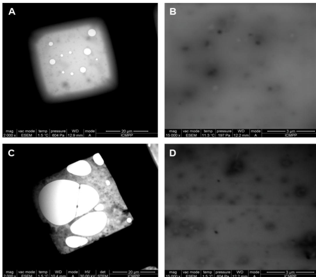
**Figure 2:** Wet-STEM images at 30 kV in bright field mode of: PDMS-Im/Br ionic liquid (A,B) and mixture of PDMS-Im/Br with PRot (C,D).
