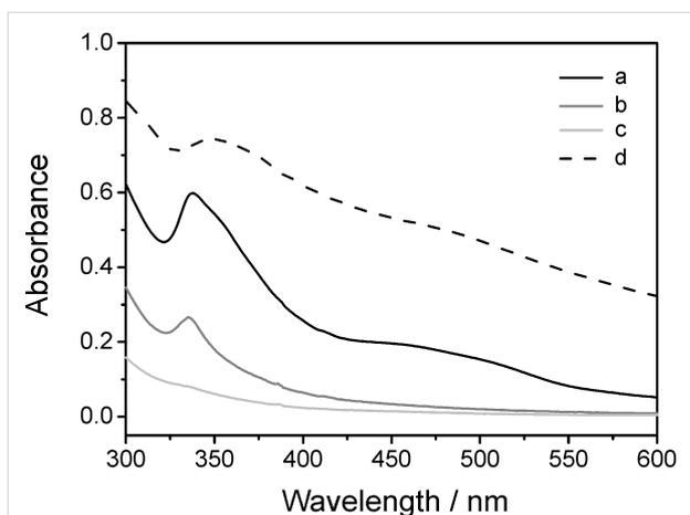
**Figure 5:** UV–vis spectra of the water solution of C<sub>60</sub> produced by stirring C<sub>60</sub> in 6mM  $\gamma$ -CD solution in DMF/toluene (v/v 1:1) at rt for 7 d, followed by dissolution of the resulting complex in water after evaporation of the solvents (procedure **c**): (a) before filtration, (b) after filtration, and (c) after centrifugation; (d) *n*C<sub>60</sub> made from THF [43] before filtration.
