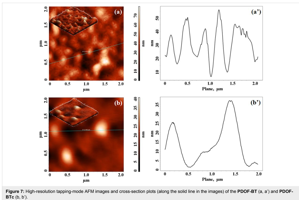
**Figure 7:** High-resolution tapping-mode AFM images and cross-section plots (along the solid line in the images) of the **PDOF-BT** (a, a') and **PDOF-BTc** (b, b').
