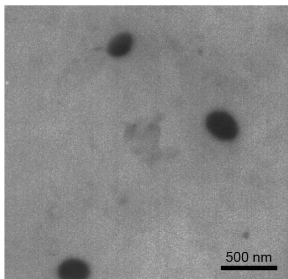
**Figure 2:** TEM microphotograph of cyclodextrin carbonate nanosponge (magnification 46,000×).
