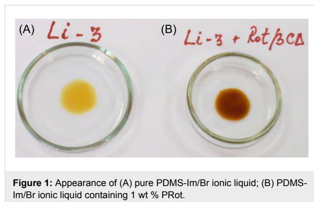
**Figure 1:** Appearance of (A) pure PDMS-Im/Br ionic liquid; (B) PDMS-Im/Br ionic liquid containing 1 wt % PRot.
