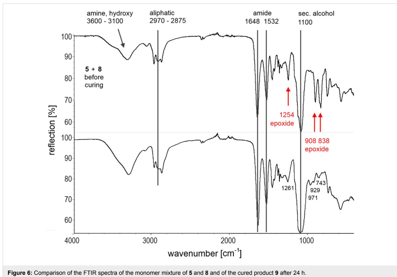
**Figure 6:** Comparison of the FTIR spectra of the monomer mixture of **5** and **8** and of the cured product **9** after 24 h.
