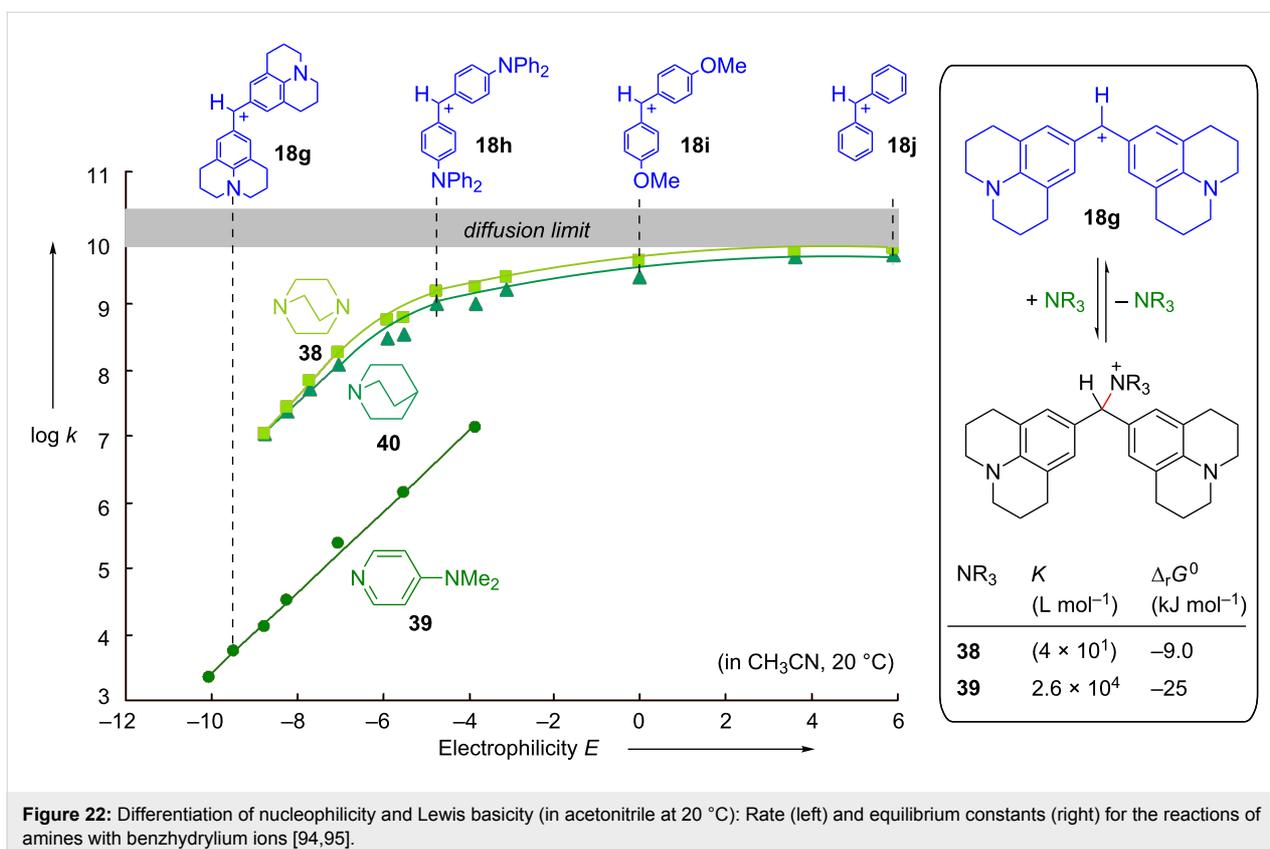
**Figure 22:** Differentiation of nucleophilicity and Lewis basicity (in acetonitrile at 20 °C): Rate (left) and equilibrium constants (right) for the reactions of amines with benzhydrylium ions [94,95].
