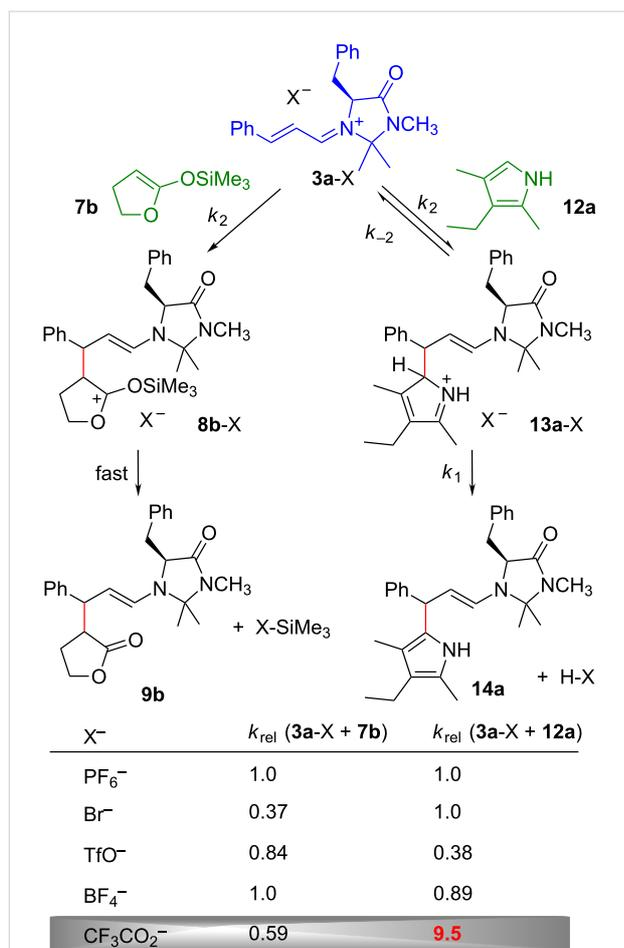
**Figure 8:** Counterion effects in electrophilic reactions of iminium ions **3a-X** (at 20 °C, silyl ketene acetal **7b** in dichloromethane with *c*(**3a-CF<sub>3</sub>CO<sub>2</sub>**) = (1.7–2.5) × 10<sup>-5</sup> M, kryptopyrrole **12a** in acetonitrile with *c*(**3a-CF<sub>3</sub>CO<sub>2</sub>**) = 5.0 × 10<sup>-5</sup> M).
