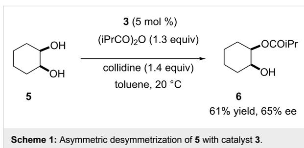
Scheme 1: Asymmetric desymmetrization of **5** with catalyst **3**.
