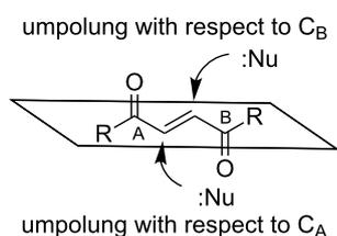
**Figure 1:** The conjugated addition to unsaturated 1,4-diketone 1.
