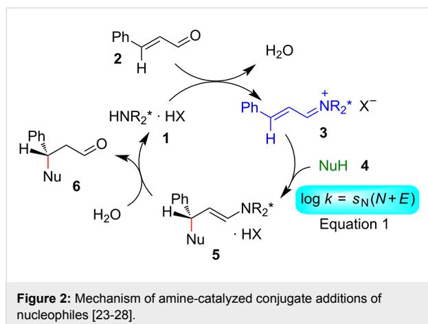
the precursor carbonyl compounds (e.g., **2**), it was necessary to determine the reactivity parameters  $N$  and  $s_N$  of potential nucleophilic substrates **4** and the electrophilicity parameters  $E$  of iminium ions **3**.
