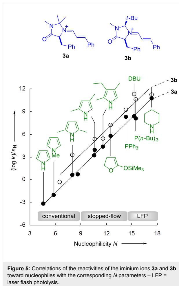
Figure 5: Correlations of the reactivities of the iminium ions 3a and 3b toward nucleophiles with the corresponding  $N$  parameters – LFP = laser flash photolysis.
