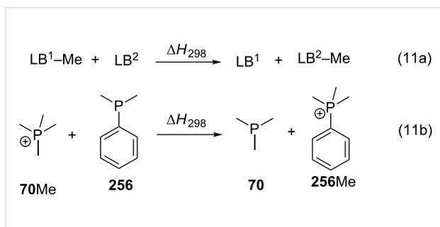
**Scheme 11:** (a) General definition for a methyl cation transfer reaction between Lewis bases  $LB^1$  and  $LB^2$ , and (b) methyl cation exchange between trimethylphosphane (**70**) and dimethylphenylphosphane (**256**).
