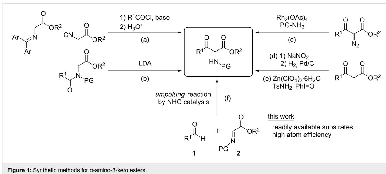
these esters are still needed. We envisioned that highly atom-efficient synthesis of  $\alpha$ -amino- $\beta$ -keto esters could be achieved by a novel umpolung approach including C–C bond construction, that is, formal addition of acyl anion equivalents generated from aldehydes **1** with NHCs, to  $\alpha$ -imino esters **2** (Figure 1, (f)).
