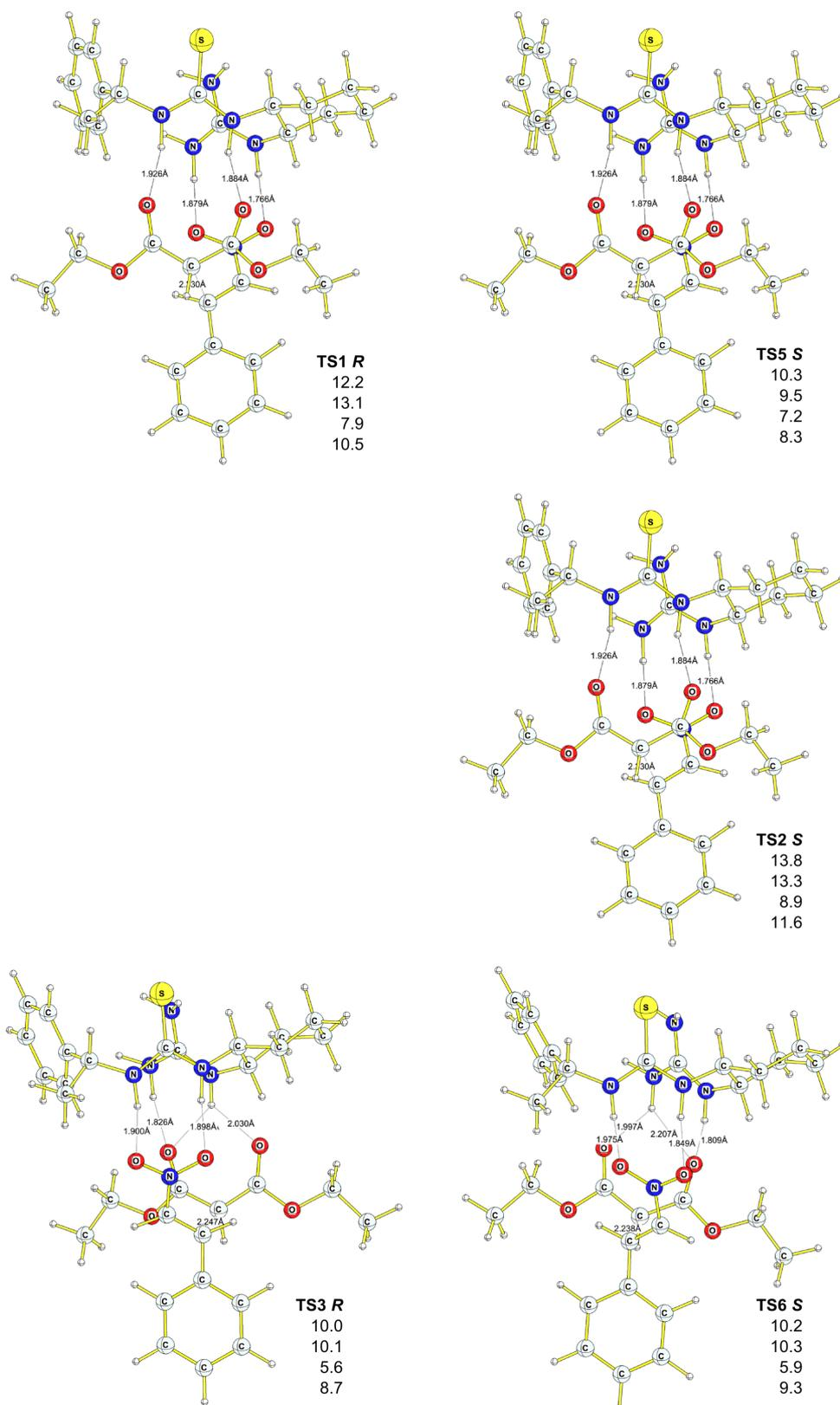
**Figure 3:** Geometries of transition states for *R* and *S* products. Relative energies (with respect to *Init10*) are in kcal·mol<sup>-1</sup>, B3PW91/6–31G(d) (first entry), DFT-PCM (second entry), MP2/6–311++ G(d,p)//B3PW91/6–31G(d) (third entry), DFT-D (fourth entry). Bond lengths are in Å.
