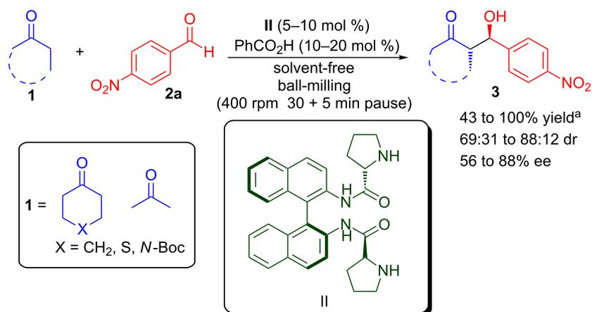
**Scheme 3:** (*S*)-Binam-L-prolinamide catalysed asymmetric aldol reaction by using a ball-mill. <sup>a</sup>Conversion.
