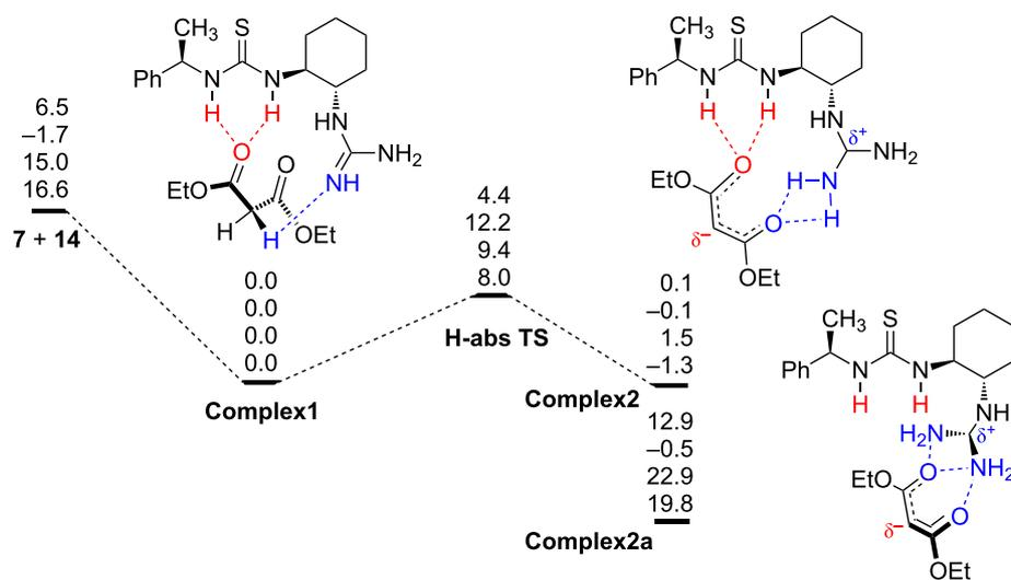
**Scheme 4:** Energy profile for the first step of the reaction between catalyst 7 and malonate 14. Energies are in kcal·mol<sup>-1</sup>, B3PW91/6–31G(d) (first entry), DFT-PCM (second entry), MP2/6–311++G(d,p)//B3PW91/6–31G(d) (third entry), DFT-D (fourth entry).
