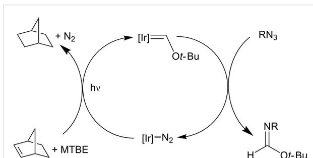
**Scheme 15:** Catalytic oxidation of MTBE by multiple C–H activations and nitrene-group transfer to a  $\text{M}^{\delta-}=\text{E}^{\delta+}$  FLP [18,78].
