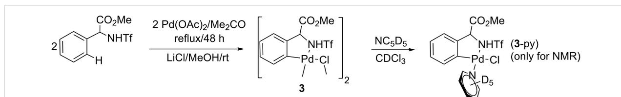
**Scheme 2:** Synthesis and NMR characterization of orthometallated complex **3**.
