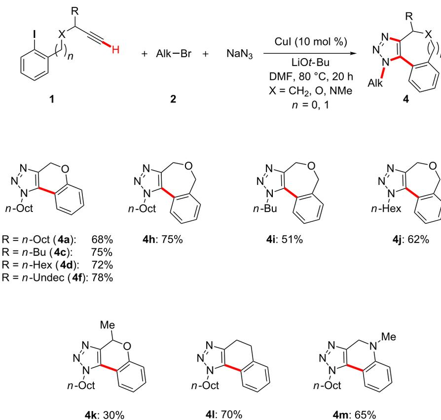
**Scheme 4:** Nonsequential cascade synthesis of fully substituted triazoles **4**. General reaction conditions: **1** (1.00 mmol), **2** (1.00 mmol), NaN<sub>3</sub> (1.05 mmol), CuI (10 mol %) DMF (3.0 mL), LiOt-Bu (2.00 mmol); yields of isolated product.
