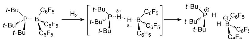
**Scheme 1:** Heterolytic cleavage of  $H_2$  by a phosphine/borane FLP by  $H_2$  polarization in the P–B cavity [5,11].
