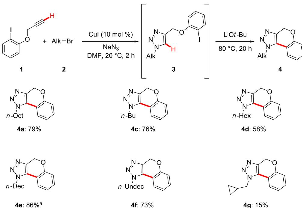
**Scheme 3:** Copper-catalyzed reaction sequence using alkyl bromides **2**. General reaction conditions: **1** (1.00 mmol), **2** (1.00 mmol), NaN<sub>3</sub> (1.05 mmol), CuI (10 mol %), DMF (3.0 mL), LiOt-Bu (2.00 mmol); yields of isolated product. <sup>a</sup>60 °C in the first step.
