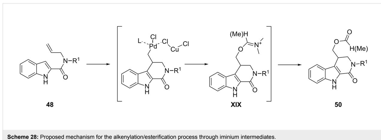
oxidation or the generation of hetero-bimetallic palladium/copper intermediates, which may undergo nucleophilic attack by the solvent on the exocyclic carbon to give the iminium intermediates **XIX** (Scheme 28). Finally, the latter may be converted into the esters **50** by hydrolysis.
