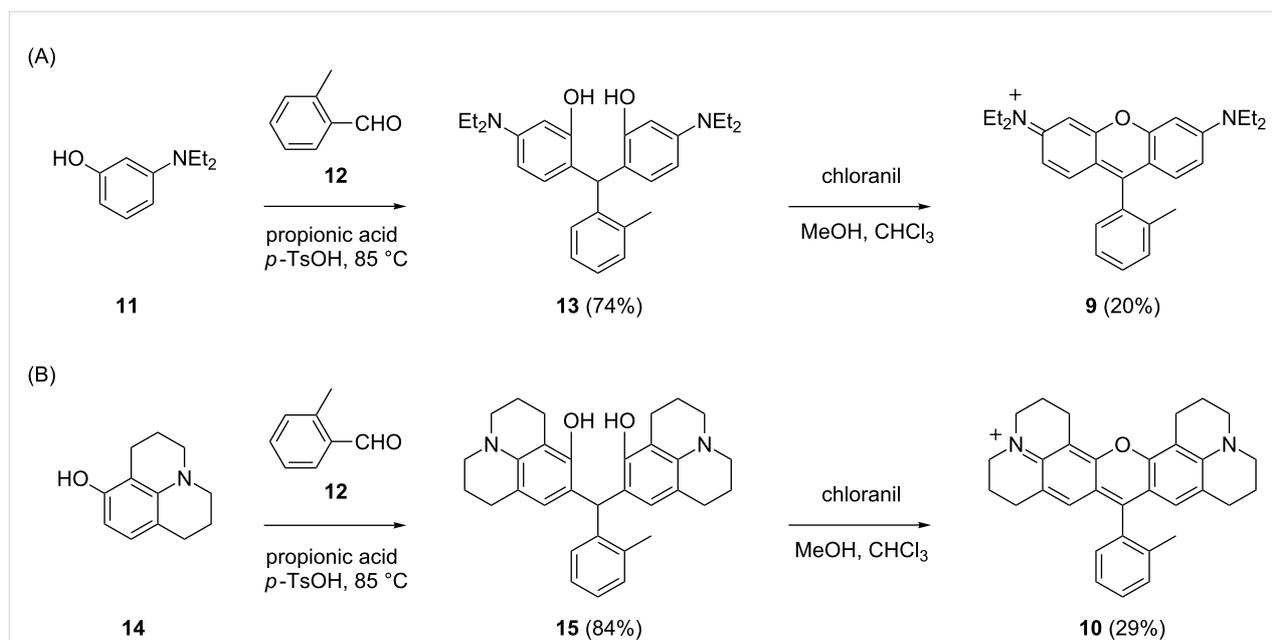
**Scheme 1:** Synthesis of the HRB **9** and HR101 **10** fluorophores.
