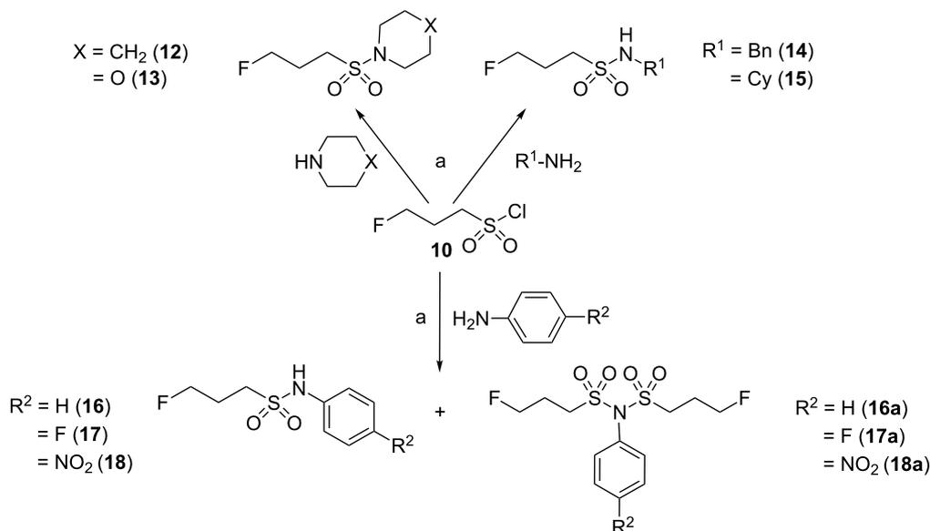
**Scheme 3:** Synthesis of 3-fluoropropanesulfonamides **12–18**. Reagents and conditions: (a) triethylamine (TEA), CH<sub>2</sub>Cl<sub>2</sub>, reflux (for **12–17**) or pyridine, CH<sub>2</sub>Cl<sub>2</sub>, rt (for **18**).
