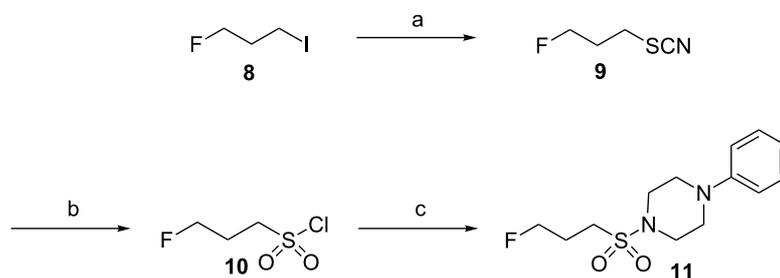
**Scheme 2:** Synthesis of 3-fluoropropanesulfonamide **11** via intermediary 3-fluoropropanesulfonyl chloride (**10**). Reagents and conditions: (a) KSCN, CH<sub>3</sub>OH, reflux; (b) Cl<sub>2</sub>, H<sub>2</sub>O/AcOH, rt; (c) *N*-phenylpiperazine, triethylamine (TEA), CH<sub>2</sub>Cl<sub>2</sub>, reflux.
