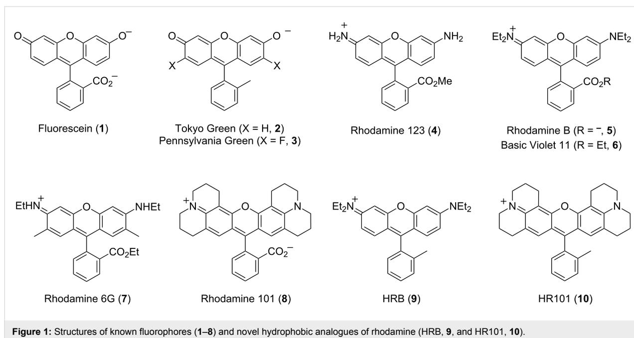
**Figure 1:** Structures of known fluorophores (**1–8**) and novel hydrophobic analogues of rhodamine (HRB, **9**, and HR101, **10**).
