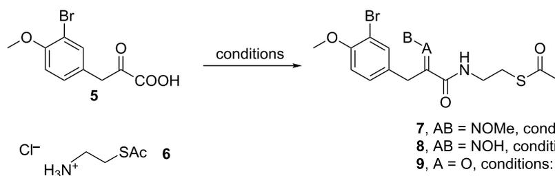
**Scheme 2:** Synthesis of **7–9**. Conditions: (i)  $\text{HCl} \cdot \text{H}_2\text{NOMe}$ , pyridine, rt, 12 h; (ii) EDC, NHS, dioxane, rt, 3 h; (iii) **6**,  $\text{Et}_3\text{N}$ , dioxane/MeOH, rt; (iv)  $\text{HCl} \cdot \text{H}_2\text{NOH}$ , pyridine, rt, 12 h; (v) DCC, NOHP, **6**,  $\text{Et}_3\text{N}$ , dioxane, rt, 24 h.
