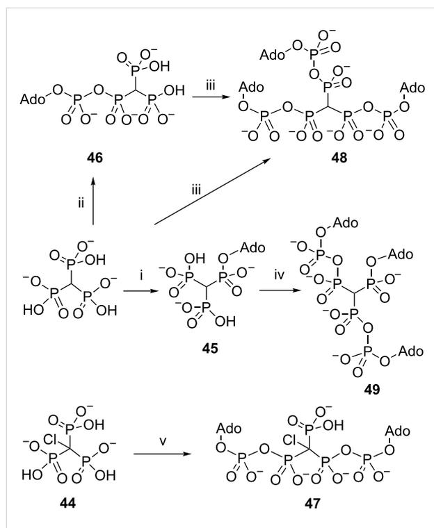
**Scheme 24:** Synthesis of trisphosphonate modified nucleotides. Reagents: i, 5'-O-tosyl adenosine, MeCN; ii, AMP-morpholidate (0.8 equiv), tetrazole, pyridine; iii, AMP-morpholidate (5 equiv), tetrazole, pyridine; iv, excess AMP-morpholidate, pyridine; v, AMP-morpholidate (2.2 equiv), tetrazole, pyridine. All counterions are tri-*n*-butylammonium. Ado = 5'-adenosyl.
