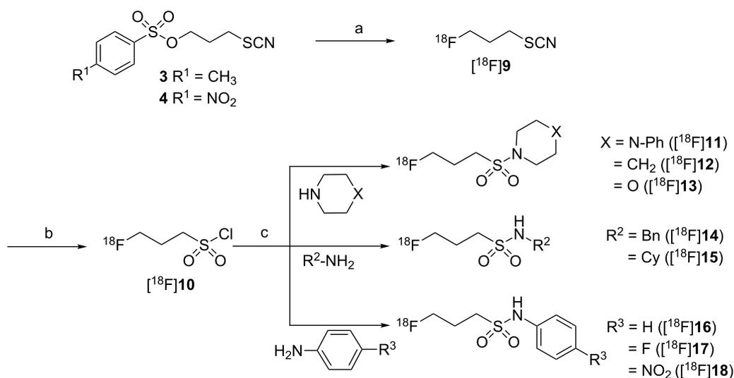
**Scheme 4:** Radiosynthesis of 3- $^{18}\text{F}$ fluoropropanesulfonamides  $^{18}\text{F}$ 11– $^{18}\text{F}$ 18. Reagents and conditions: (a)  $^{18}\text{F}$ F<sup>-</sup>, Kryptofix<sub>222</sub>, K<sub>2</sub>CO<sub>3</sub>, CH<sub>3</sub>CN, 82 °C; (b) Cl<sub>2</sub>/H<sub>2</sub>O, C<sub>18</sub>-modified silica gel; (c) auxiliary base as specified in Table 2, CH<sub>2</sub>Cl<sub>2</sub>, rt.
