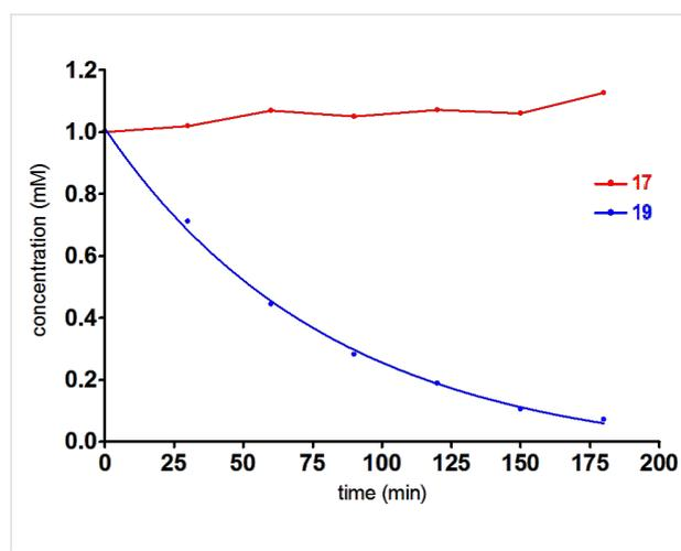
**Figure 6:** Time course of the carboxylesterase-catalysed degradation of 3-fluoropropanesulfonamide **17** (red) and fluoroacetamide **19** (blue). The pseudo first-order rate constant for the decay of **19** was (0.012 ± 0.001) min<sup>-1</sup> corresponding to a half-life of 57.8 min. Data points represent average values from two measurements originating from two independent experiments with SEM values less than 10% of the mean values.
