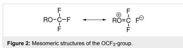
**Figure 2:** Mesomeric structures of the OCF<sub>3</sub>-group.
