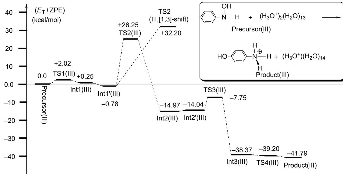
**Figure 5:** Energy changes (in kcal/mol) of model III. The corresponding geometries are shown in Figure 4. The apparent small reversal of energies of Int3(III) and TS4(III) comes from the splicing method, B3LYP/6-311+G(d,p) SCRF = PCM//B3LYP/6-31G(d), Et(B3LYP/6-31G(d)) of Int3(III) = -1509.9900126 Hartree and Et(B3LYP/6-31G(d)) of TS4(III) = -1509.9895045 Hartree.
