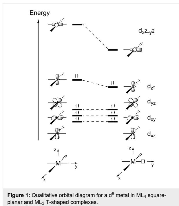
**Figure 1:** Qualitative orbital diagram for a  $d^8$  metal in  $\text{ML}_4$  square-planar and  $\text{ML}_3$  T-shaped complexes.
