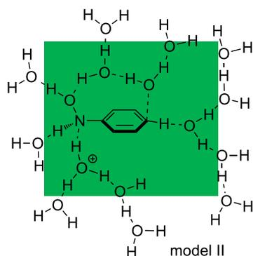
**Figure 2:** An assumed reaction system composed of Ph-NHOH and  $\text{H}_3\text{O}^+(\text{H}_2\text{O})_{14}$ . The green area represents the reaction region of TS2. To protons of  $\text{H}_3\text{O}^+$  and  $\text{H}_2\text{O}$  in the area, catalytic water molecules are linked in the  $\text{O}-\text{H}\cdots\text{OH}_2$  hydrogen-bond pattern.
