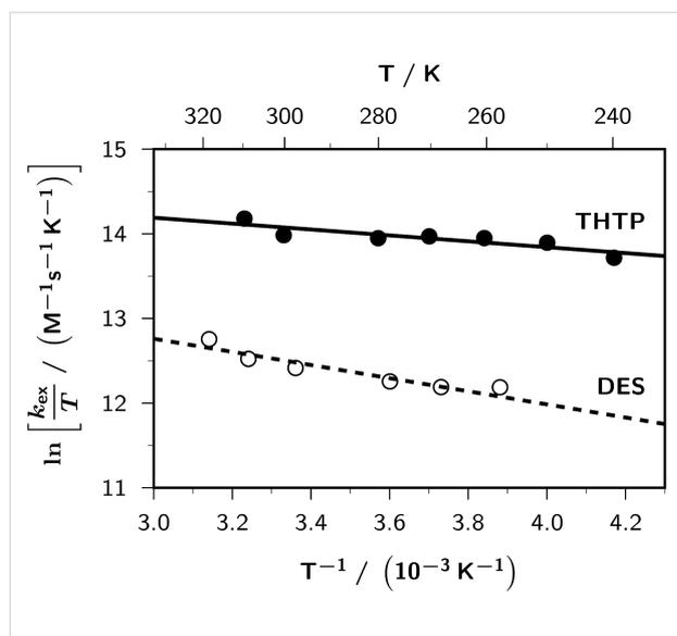
**Figure 2:** Eyring plots of the self-exchange rate constants  $k_{\text{ex}}$  for **DES** (open circles and broken line; linear regression,  $15.08 - 775/T$ ,  $r^2 = 0.94$ ) and **THTP** (filled circles and solid line; linear regression,  $15.24 - 349/T$ ,  $r^2 = 0.88$ ) in acetonitrile- $d_3$ ; sensitizer **TTP**<sup>+</sup>. For all other experimental parameters and further explanation, see Figure 1 and text.
