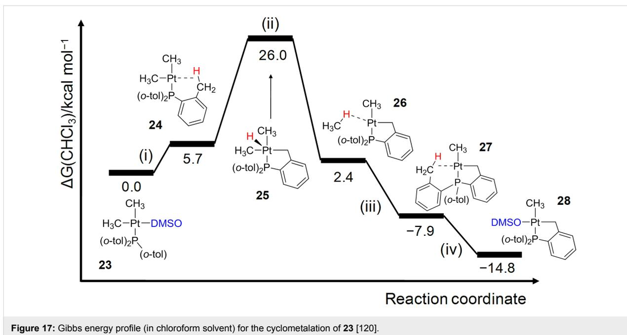
Figure 17: Gibbs energy profile (in chloroform solvent) for the cyclometalation of 23 [120].
