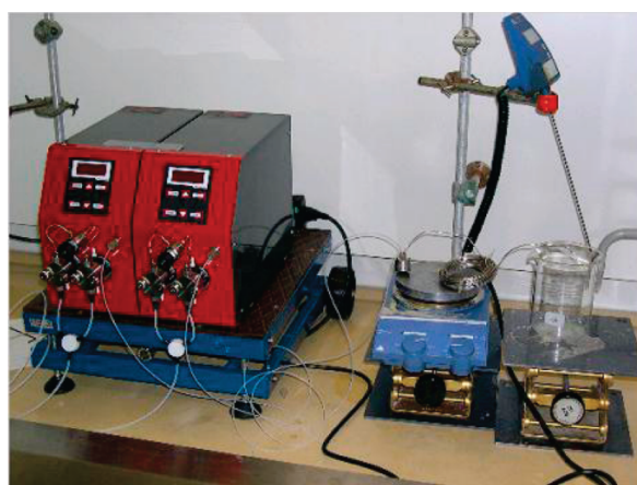
Figure 4: Photograph of the experimental setup for the synthesis of alkyl-nitropyrazoles. IMM's SIMM-V2 micromixer was used to ensure better mixing at the cost of pressure drop. Reproduced with permission from [31]. Copyright 2009 The American Chemical Society.
