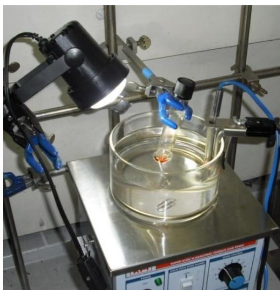
**Figure 3:** Experimental setup for the photopolymerization using the LED.
