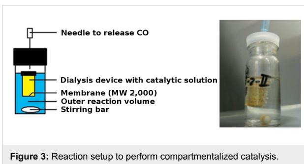
Figure 3: Reaction setup to perform compartmentalized catalysis.
