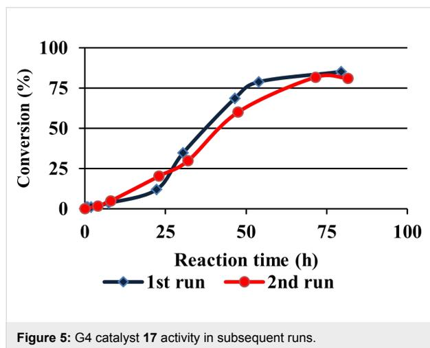
Figure 5: G4 catalyst **17** activity in subsequent runs.
