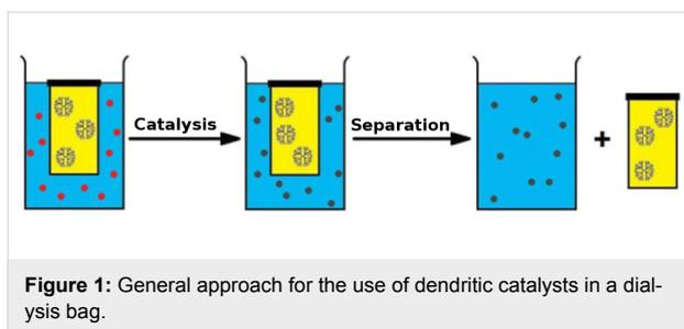
**Figure 1:** General approach for the use of dendritic catalysts in a dialysis bag.
