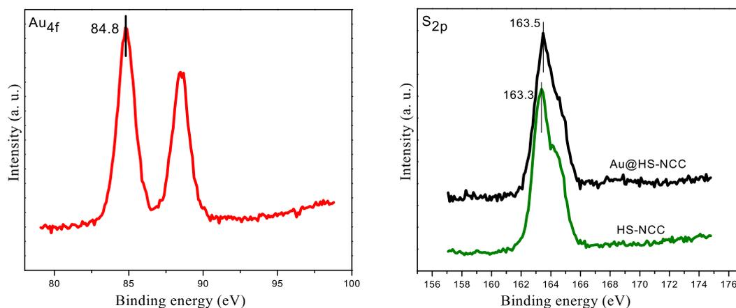
**Figure 1:** Au<sub>4f</sub> and S<sub>2p</sub> XPS spectra of the Au@HS-CNC (4.4 mol %) catalyst.
