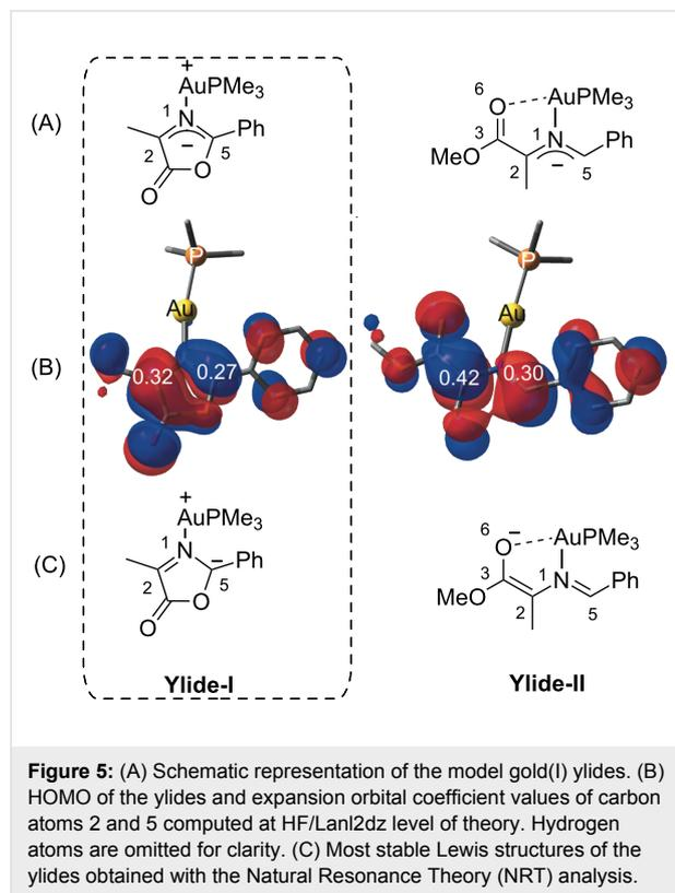
**Figure 5:** (A) Schematic representation of the model gold(I) ylides. (B) HOMO of the ylides and expansion orbital coefficient values of carbon atoms 2 and 5 computed at HF/LanL2dz level of theory. Hydrogen atoms are omitted for clarity. (C) Most stable Lewis structures of the ylides obtained with the Natural Resonance Theory (NRT) analysis.
