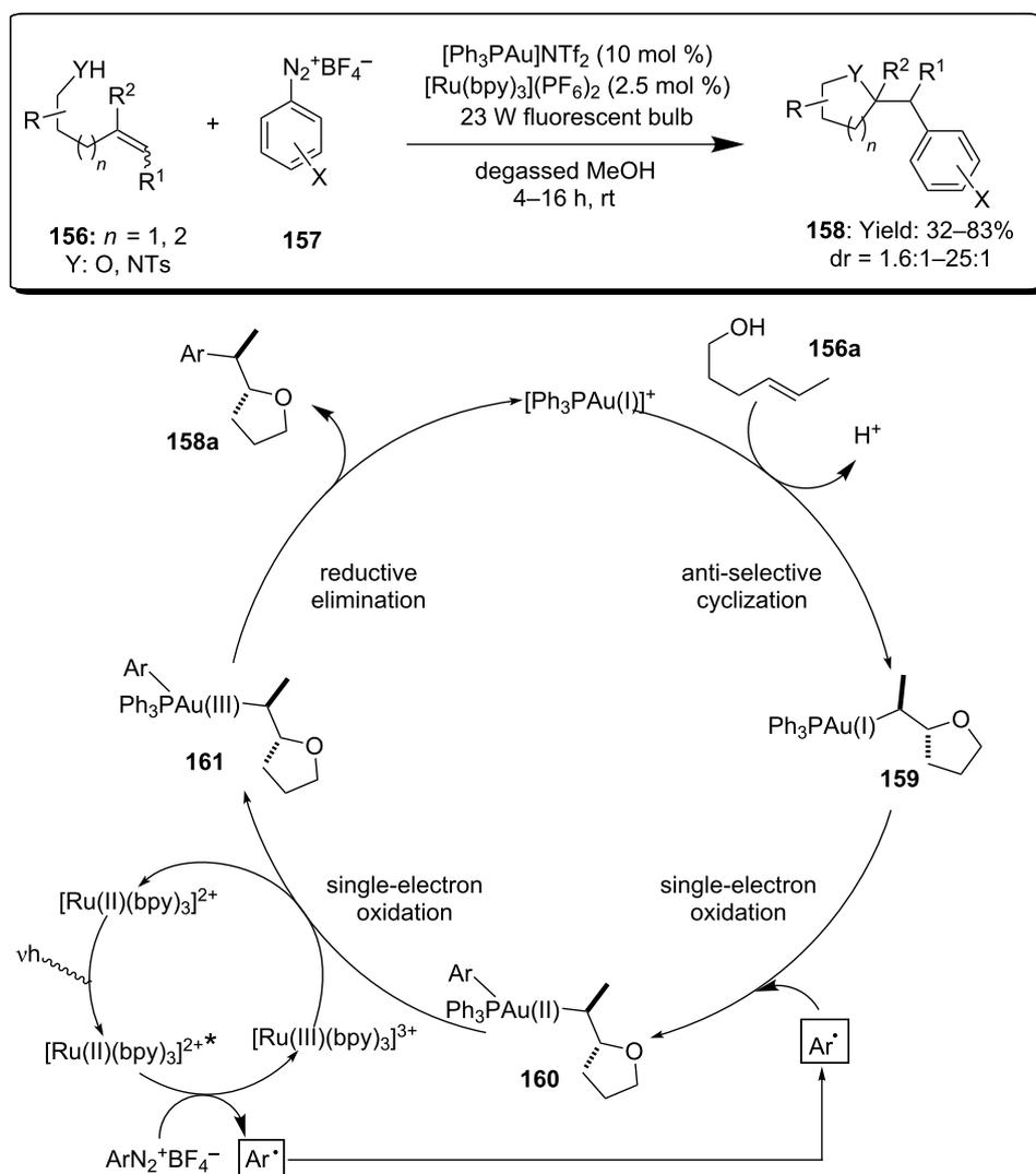
**Scheme 40:** Oxy- and amino-arylation of alkenes by [Au(I)]/[Au(III)] photoredox catalysis.
