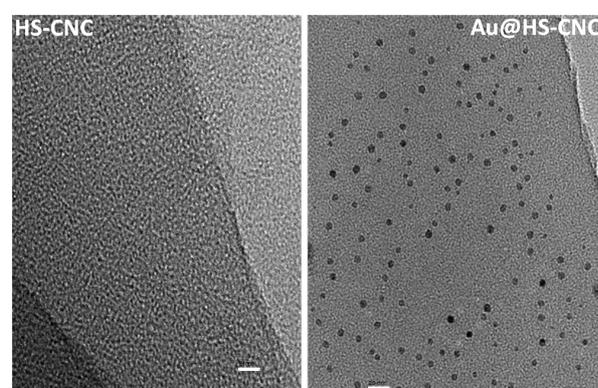
**Figure 2:** TEM pictures of the HS-CNC and Au@HS-CNC (4.4 mol %) catalyst (scale bar: 5 nm).
