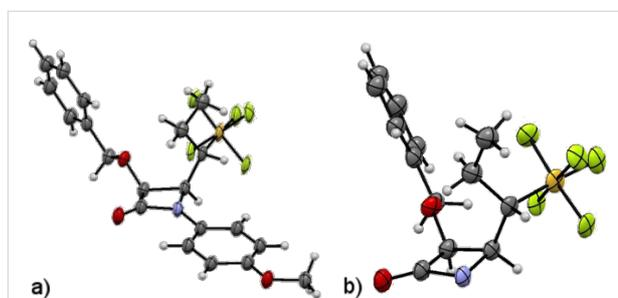
**Figure 2:** The stereochemistry of **7c**, 1,2-*lk, lk* (*Si, Si-S*), as determined by single crystal X-ray diffraction studies. Thermal ellipsoids are set at 50% probability. (a) Complete structure of **7c**. (b) PMP protecting group hidden for clarity.
