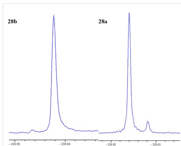
**Figure 5:** Partial  $^{19}\text{F}\{^1\text{H}\}$  NMR (400 MHz, L-(+)-DIPT/ $\text{CDCl}_3$ , 300 K) spectra of **28b** and **28a** using optimised conditions: SW 40; AQ = 0.8; O1P -230; d1 = 5; 32 or 64 scans.
