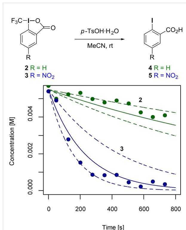
**Figure 6:** Sample kinetic traces for the decomposition of **2** (green) and **3** (blue) to **4** and **5**, respectively, upon reaction with *p*-TsOH in MeCN. Solid lines represent the average decay ( $k_{\text{decomp}}$ ) based on 6 individual measurements and dashed lines are decays based on  $k_{\text{decomp}} \pm \sigma$ .
