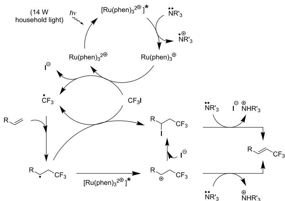
**Figure 17:** Proposed mechanism for the trifluoromethylation of alkenes with trifluoromethyl iodide under Ru-based photoredox catalysis (E. J. Cho et al.) [106].**Table 33:** Trifluoromethylation of indoles with trifluoromethyl iodide under Ru-based photoredox catalysis [107].
