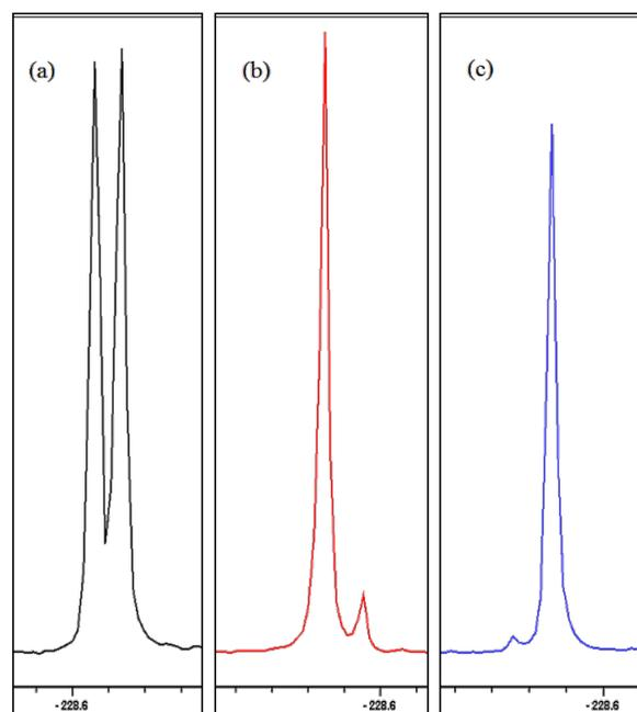
**Figure 4:** Partial  $^{19}\text{F}\{^1\text{H}\}$  NMR spectra (376 MHz, L-(+)-DIPT/ $\text{CDCl}_3$ , 300 K) spectra of (a) racemate **28c**, (b) diol **28b** and (c) **28a** under standard acquisition parameters revealing the partial enantiomer overlap.
