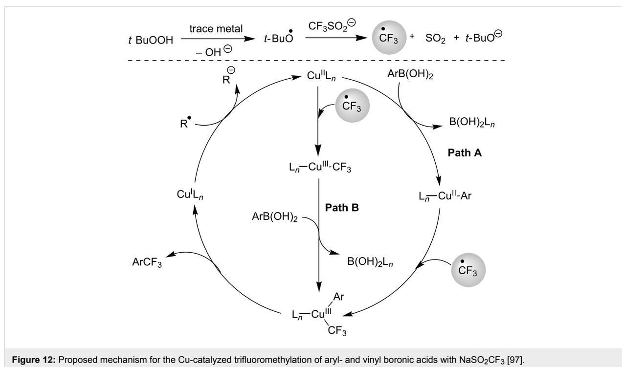
**Figure 12:** Proposed mechanism for the Cu-catalyzed trifluoromethylation of aryl- and vinyl boronic acids with NaSO<sub>2</sub>CF<sub>3</sub> [97].
