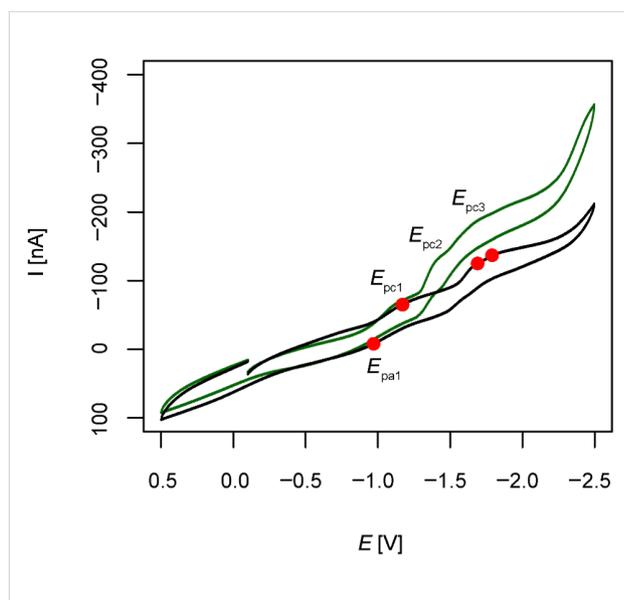
**Figure 5:** Cyclic voltammetry of **3** (1 mM, black) and of a mixture of **3** (1 mM) and methyl 2-iodo-5-nitrobenzoate (1 mM, green) in anhydrous MeCN + 0.1 M Bu<sub>4</sub>NBF<sub>4</sub>, platinum electrode, scan rate = 0.1 V/s.
