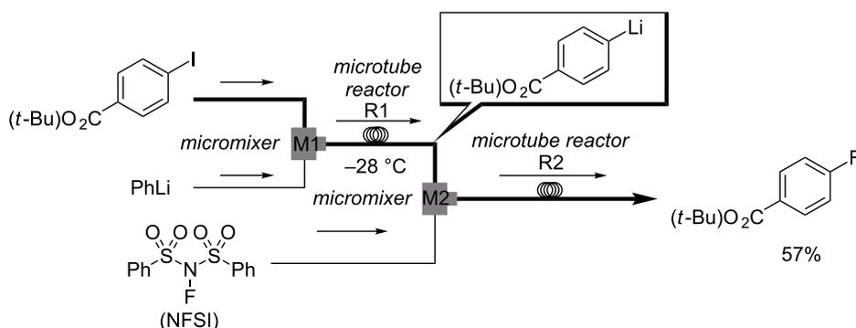
**Scheme 6:** Continuous-flow reactor for electrophilic aromatic fluorination.
