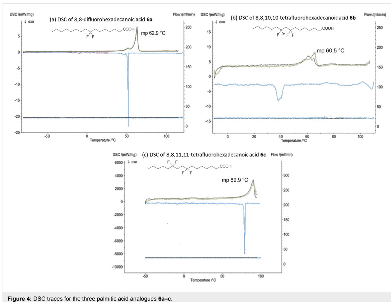
Figure 4: DSC traces for the three palmitic acid analogues **6a–c**.
