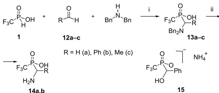
**Scheme 3:** Three-component synthesis of CF<sub>3</sub> containing α-aminophosphinic acids **14a,b**. Reagents and conditions: i) An equimolar mixture of acid **1**, dibenzylamine, HCl and two fold excess of aldehyde, H<sub>2</sub>O, 80 °C, 3 h; isolated yields: **13a** (52%), **13b** (28%); yields, determined by <sup>31</sup>P and <sup>19</sup>F NMR: **13c** (<10%). ii) H<sub>2</sub>, ethanol, catalysis 10% Pd/C, rt, normal pressure, yields: **14a** (95%), **14b** (90%).
