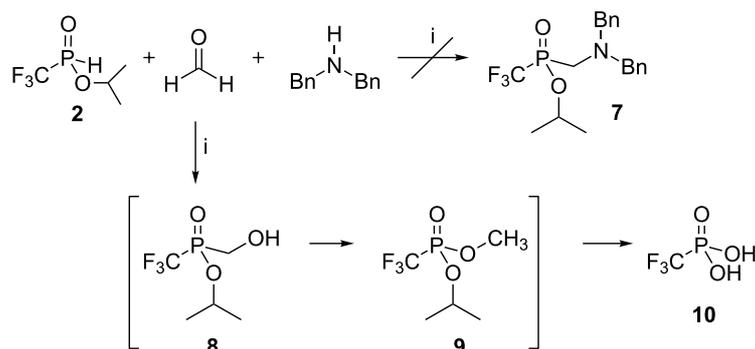
**Scheme 2:** Three-component Kabachnik–Fields reaction of CF<sub>3</sub>(H)P(O)(OiPr) (**2**) with formaldehyde and dibenzylamine. Reagents and conditions: i) an equimolar mixture of reagents, H<sub>2</sub>O, 80 °C, 3 h, argon atmosphere, yield **10** ~80% or an equimolar mixture of reagents, dioxane, 100 °C, 3 h, argon atmosphere, yield **10** ~90%.
