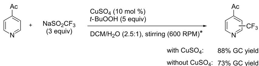
**Scheme 7:** Trifluoromethylation of 4-acetylpyridine with Langlois's reagent by P. S. Baran et al. (\* Stiring had a strong influence on the reaction efficiency; see the original article for details) [89].
