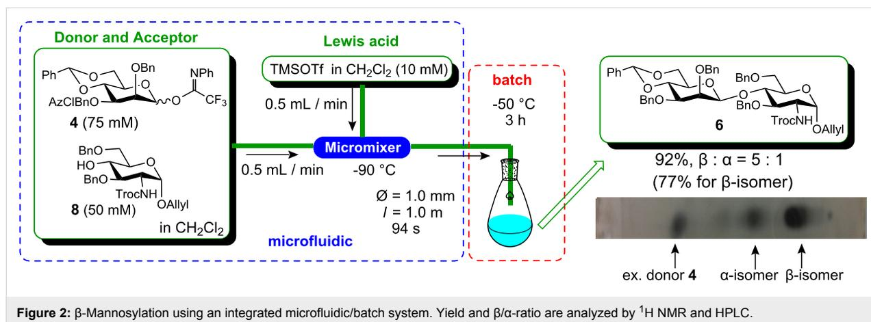
**Figure 2:**  $\beta$ -Mannosylation using an integrated microfluidic/batch system. Yield and  $\beta/\alpha$ -ratio are analyzed by  $^1\text{H}$  NMR and HPLC.
