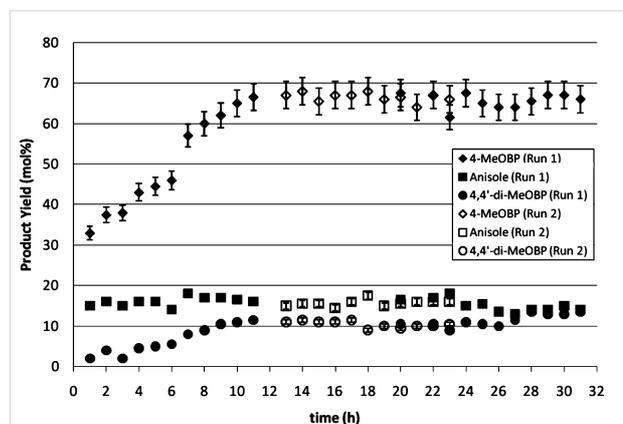
**Figure 6:** Kumada reaction carried out in a parallel channel meso reactor over a 31-hour period at a flow rate of 95 ml h<sup>-1</sup> to show catalyst stability and lifetime.
