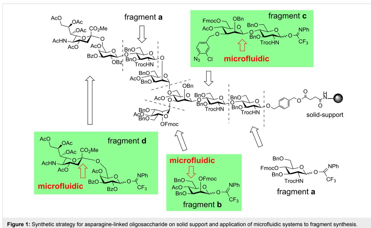
**Figure 1:** Synthetic strategy for asparagine-linked oligosaccharide on solid support and application of microfluidic systems to fragment synthesis.
