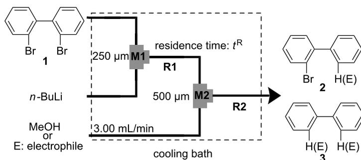
**Figure 1:** Microflow system for Br-Li exchange reaction of 2,2'-dibromobiphenyl (**1**). T-shaped micromixer: **M1** ( $\phi = 250 \mu\text{m}$ ) and **M2** ( $\phi = 500 \mu\text{m}$ ), microtube reactor: **R1** and **R2** ( $\phi = 1000 \mu\text{m}$ ,  $l = 50 \text{ cm}$ ), a solution of 2,2'-dibromobiphenyl (**1**): 0.10 M in THF, a solution of *n*-BuLi: 0.50 M in hexane, a solution of electrophile: 0.30 M in THF.
