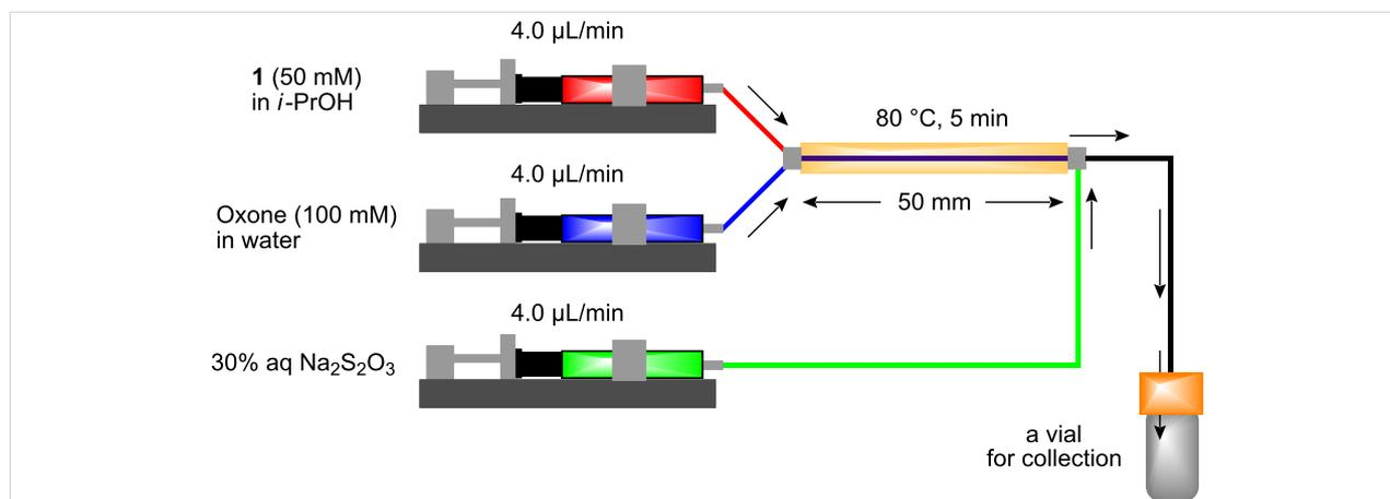
**Figure 1:** Miniflow reaction system of oxidative cyclization.
