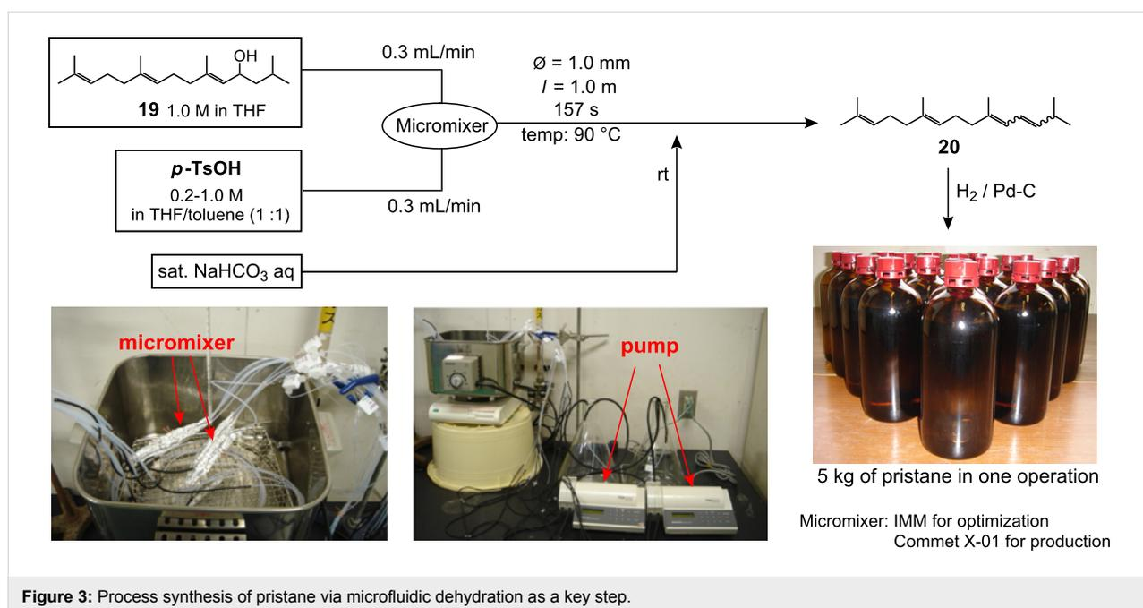
Figure 3: Process synthesis of pristane via microfluidic dehydration as a key step.
