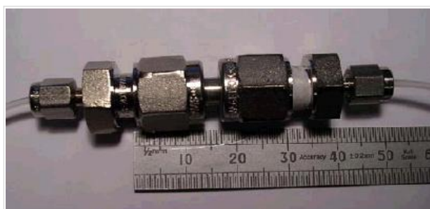
Figure 1: Stainless steel single column flow reactor for discovery scale synthesis.
