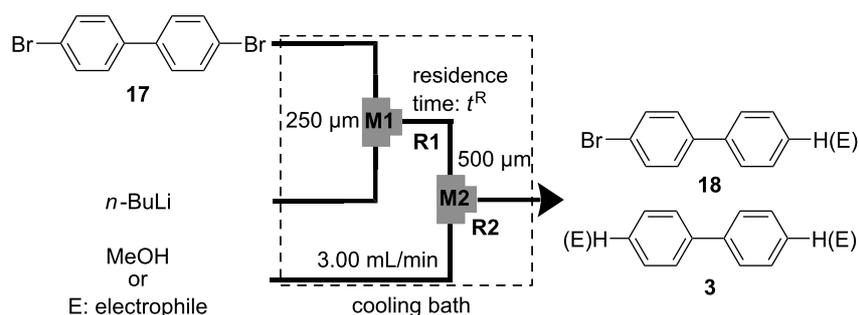
**Figure 4:** Microflow system for Br-Li exchange reaction of 4,4'-dibromobiphenyl (**17**). T-shaped micromixer: **M1** ( $\phi = 250 \mu\text{m}$ ) and **M2** ( $\phi = 500 \mu\text{m}$ ), microtube reactor: **R1** and **R2** ( $\phi = 1000 \mu\text{m}$ ,  $l = 50 \text{ cm}$ ), a solution of 4,4'-dibromobiphenyl (**17**): 0.10 M in THF, a solution of *n*-BuLi: 0.50 M in hexane, a solution of an electrophile: 0.30 M in THF.
