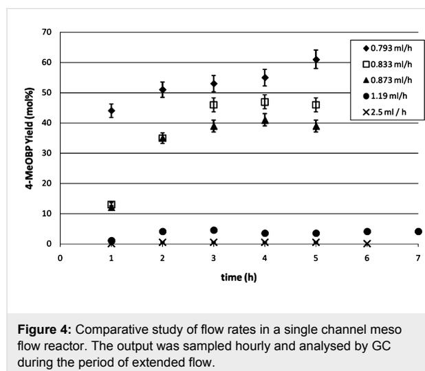
**Figure 4:** Comparative study of flow rates in a single channel meso flow reactor. The output was sampled hourly and analysed by GC during the period of extended flow.
