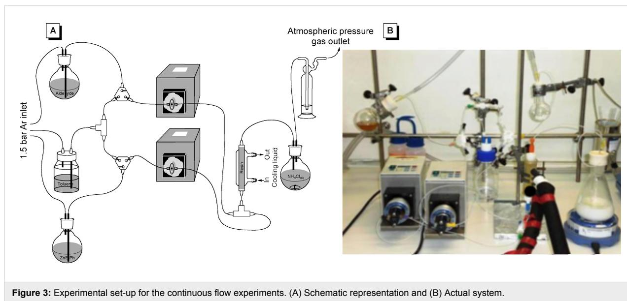
**Figure 3:** Experimental set-up for the continuous flow experiments. (A) Schematic representation and (B) Actual system.
