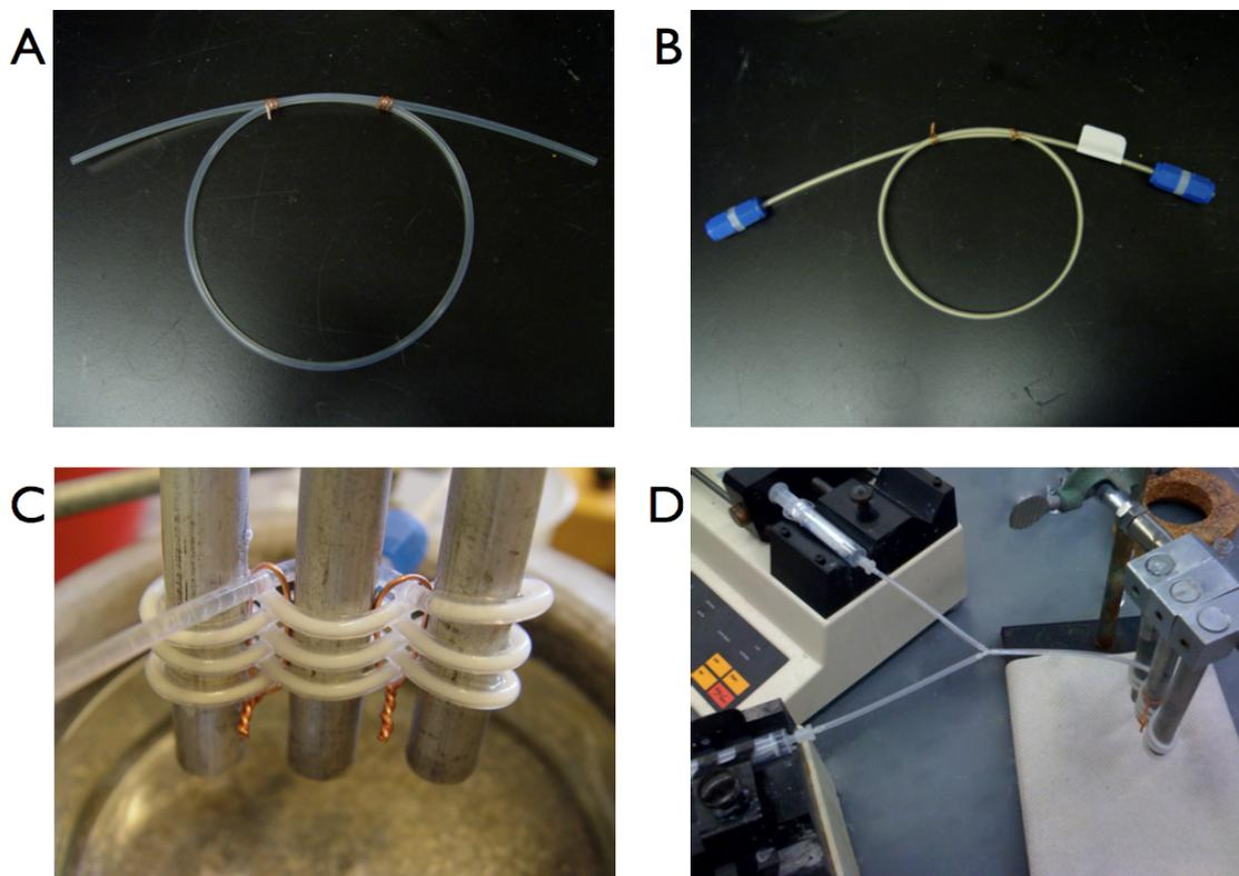
**Figure 1:** The simplified microreactor setup. Empty tubing (A) is packed with functionalized AO resin and attached to caps (B). The packed bed is woven between metal bars (C) and connected to syringe pumps (D).
