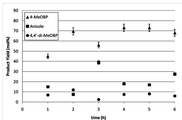
**Figure 5:** Kumada reaction carried out in a parallel channel meso reactor at a flow rate of 95 ml h<sup>-1</sup>.
