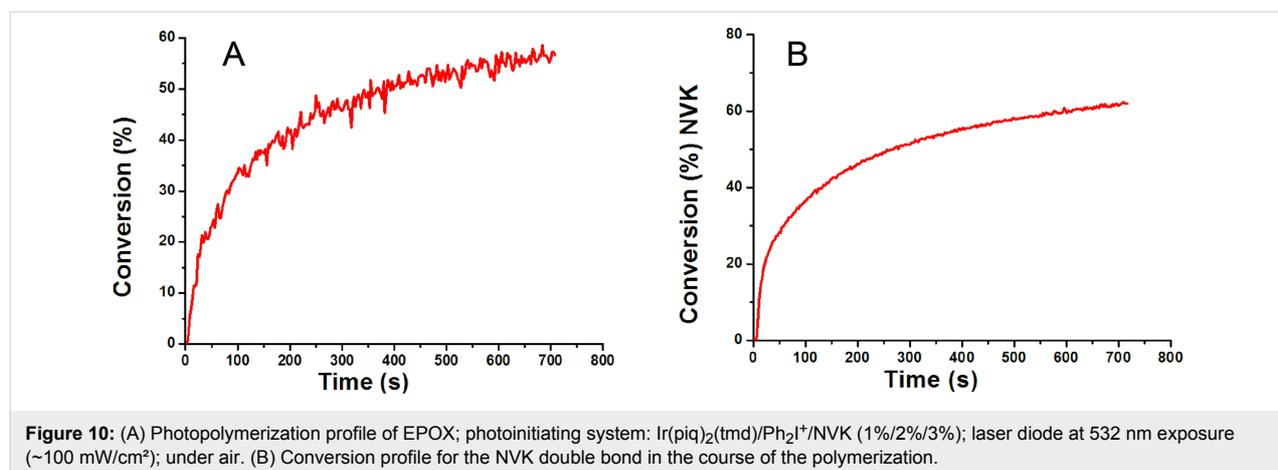
**Figure 10:** (A) Photopolymerization profile of EPOX; photoinitiating system:  $\text{Ir}(\text{piq})_2(\text{tmd})/\text{Ph}_2\text{I}^+/\text{NVK}$  (1%/2%/3%); laser diode at 532 nm exposure ( $\sim 100$  mW/cm $^2$ ); under air. (B) Conversion profile for the NVK double bond in the course of the polymerization.
