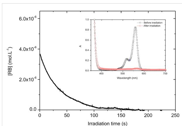
**Figure 1:** Evolution of RB concentration as a function of irradiation time ( $\lambda = 532 \text{ nm}$ ,  $9 \text{ mW}\cdot\text{cm}^{-3}$ ); insert: absorption spectra obtained before and after irradiation.
