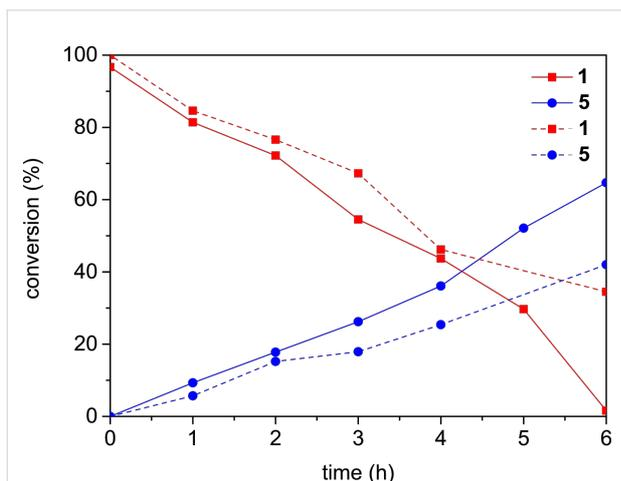
**Figure 1:** Conversion of substrate **1** and formation of product **5** observed during photocatalysis with PDI in the presence of 0.4 equiv (dashed lines) and 1.0 equiv (solid lines) of Ph-SH as additive; reaction conditions: **1** (20 mM), Ph-SH (20 mM), PDI (0.5 mM), in CH<sub>2</sub>Cl<sub>2</sub>/MeOH 3:1 (4 mL), argon atmosphere, 30 °C, 250 mW LED, λ = 530 nm, **1** and **5** identified and quantified by GC-MS.
