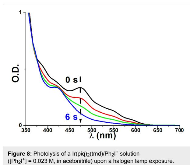
**Figure 8:** Photolysis of a  $\text{Ir}(\text{piq})_2(\text{tmd})/\text{Ph}_2\text{I}^+$  solution ( $[\text{Ph}_2\text{I}^+] = 0.023$  M, in acetonitrile) upon a halogen lamp exposure.
