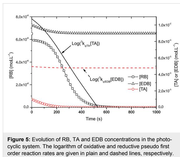
**Figure 5:** Evolution of RB, TA and EDB concentrations in the photocyclic system. The logarithm of oxidative and reductive pseudo first order reaction rates are given in plain and dashed lines, respectively.
