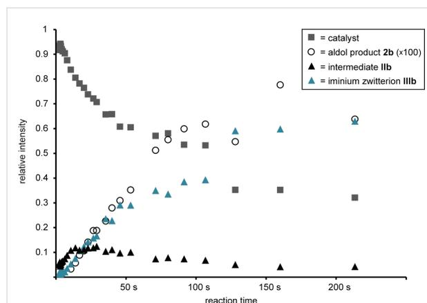
**Figure 6:** Normalized relative intensities in ESI spectra recorded for the inverse aldol reaction of butyraldehyde, diethyl ketomalonate and charge-tagged catalyst **1** at different time stages using the continuous-flow setup with two microreactors shown in Figure 3.
