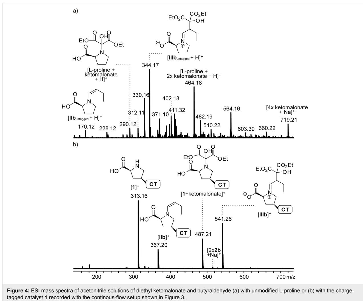
**Figure 4:** ESI mass spectra of acetoneitrile solutions of diethyl ketomalonate and butyraldehyde (a) with unmodified L-proline or (b) with the charge-tagged catalyst **1** recorded with the continuous-flow setup shown in Figure 3.
