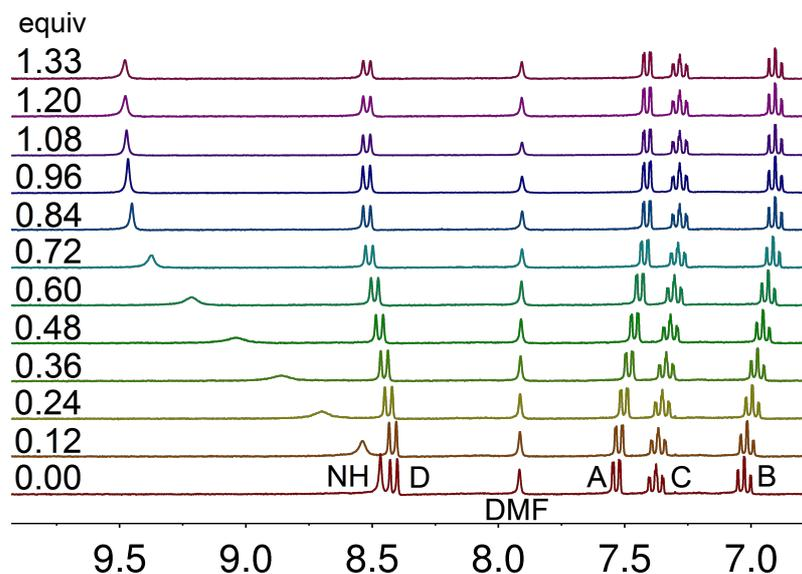
**Figure 4:**  $^1\text{H}$  NMR spectra of **2** in  $\text{THF-}d_8$  after addition of increasing molar equivalents of tetrabutylammonium nitrate. The N–H proton resonance shows a distinct downfield shift depending on the concentration of the anion. The small invariant DMF signal originates from the solvent of recrystallization used to purify the sample for the NMR experiments.
