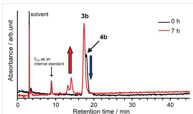
**Figure 7:** HPLC profiles of the reaction mixture of **3b** and **4b**, (black) before and (red) after heating in refluxing toluene. Conditions: column, Buckyprep ( $\varnothing$  4.6 mm  $\times$  250 mm); eluent, toluene; flow rate, 1.0 mL/min; wavelength, 330 nm; rt.
