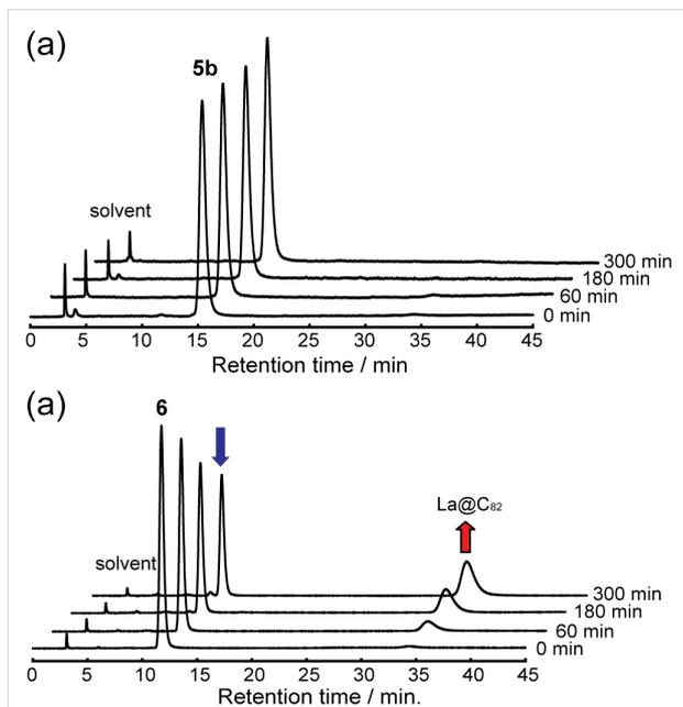
**Figure 15:** HPLC profiles for comparison of the thermal stabilities of (a) **5b** and (b) **6** at 30 °C. Conditions: column, Buckyprep ( $\varnothing$  4.6 mm  $\times$  250 mm); temperature, 40 °C.
