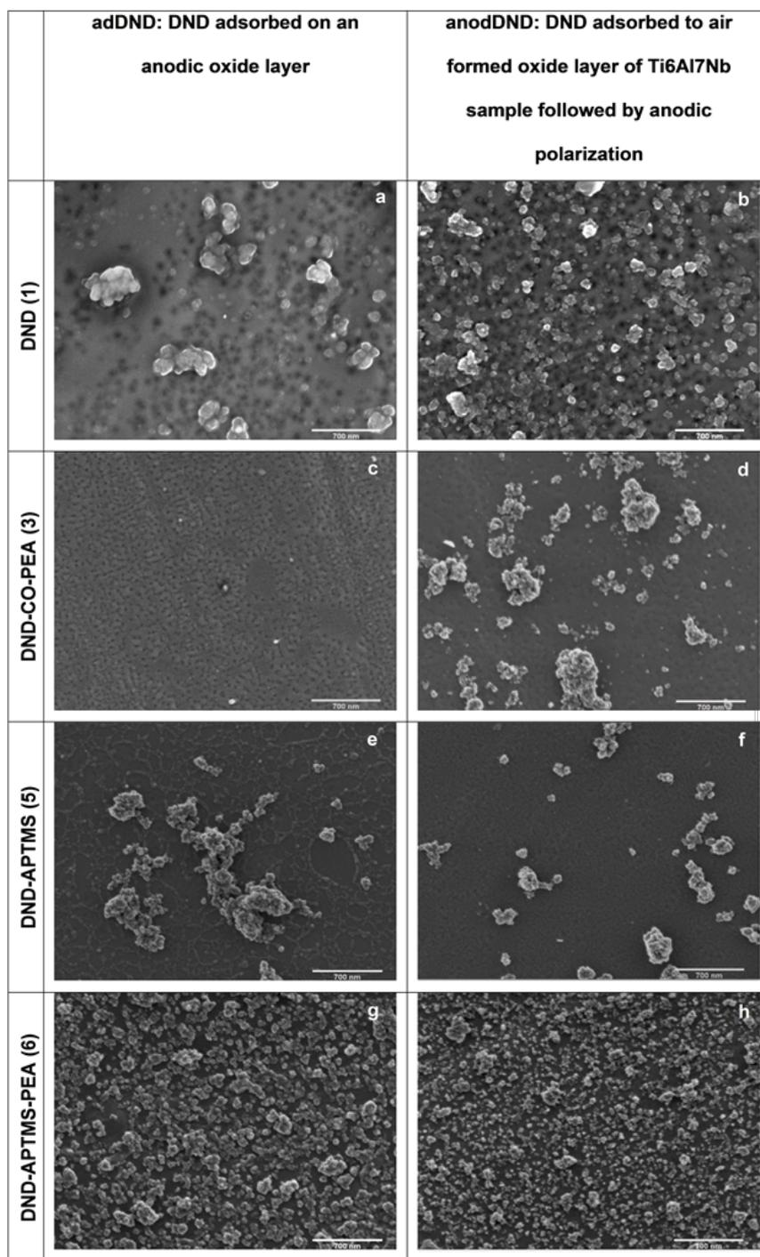
**Figure 4:** SEM images of titanium anodic oxide surface with: (a,b) unmodified DND; (c,d) DND-COOH functionalized with O-PEA (3); (e,f) silanized nanodiamonds with APTMS 5 and (g,h) silanized nanodiamonds functionalized with O-PEA 6. Left column – adDND. DND adsorbed on an anodic oxide layer and right column – anodDND with adsorption of DND on air formed oxide layer of Ti sample followed by anodic polarization. Anodic polarization was consistently carried out at 60 V and 50 mA/cm<sup>2</sup>.
