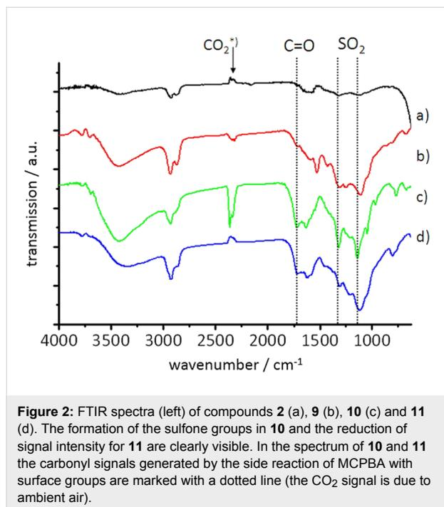
**Figure 2:** FTIR spectra (left) of compounds **2** (a), **9** (b), **10** (c) and **11** (d). The formation of the sulfone groups in **10** and the reduction of signal intensity for **11** are clearly visible. In the spectrum of **10** and **11** the carbonyl signals generated by the side reaction of MCPBA with surface groups are marked with a dotted line (the  $\text{CO}_2$  signal is due to ambient air).
