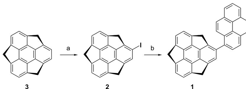
**Scheme 1:** Synthesis of pyrenylsumanene (**1**): (a)  $\text{Sc}(\text{OTf})_3$  (5 mol %), DIH (100 mol %),  $\text{CH}_2\text{Cl}_2$ , rt, 2.5 h, yield 80%; (b) palladium (II) acetate (20 mol %), 1-pyreneboronic acid (150 mol %), acetone/water 4:1, 40 °C, 12 h, yield 84%.
