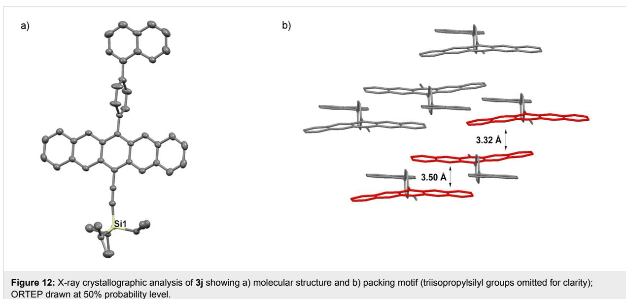
while the intervening benzene ring is nearly perpendicular to both the pentacene skeleton ( $\sim 90^\circ$ ) and the naphthyl group ( $\sim 86^\circ$ ). Compound **3j** arranges in a 1D slipped stack arrangement along the crystallographic *b*-axis with two different interplanar distances of  $\sim 3.50$  Å and 3.32 Å.
