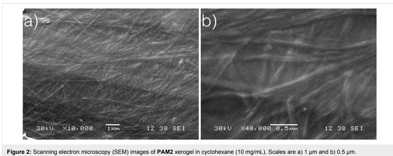
**Figure 2:** Scanning electron microscopy (SEM) images of **PAM2** xerogel in cyclohexane (10 mg/mL). Scales are a) 1  $\mu\text{m}$  and b) 0.5  $\mu\text{m}$ .
