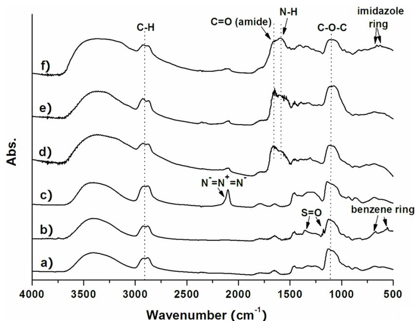
**Figure 1:** FTIR spectra of a) ND50-PG, b) ND-PG-OTs, c) ND-PG-N<sub>3</sub>, d) ND-PG-Arg<sub>8</sub>, e) ND-PG-Lys<sub>8</sub>, and f) ND-PG-His<sub>8</sub>. Arrows indicate new absorption bands in each step.
