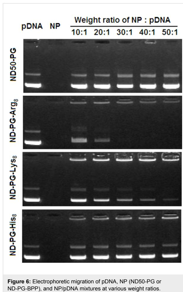
**Figure 6:** Electrophoretic migration of pDNA, NP (ND50-PG or ND-PG-BPP), and NP/pDNA mixtures at various weight ratios.
