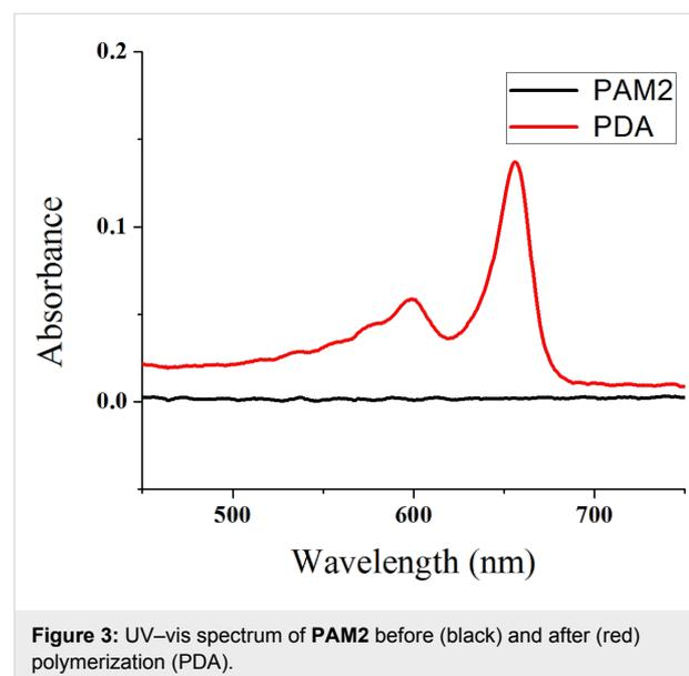
**Figure 3:** UV-vis spectrum of **PAM2** before (black) and after (red) polymerization (PDA).
