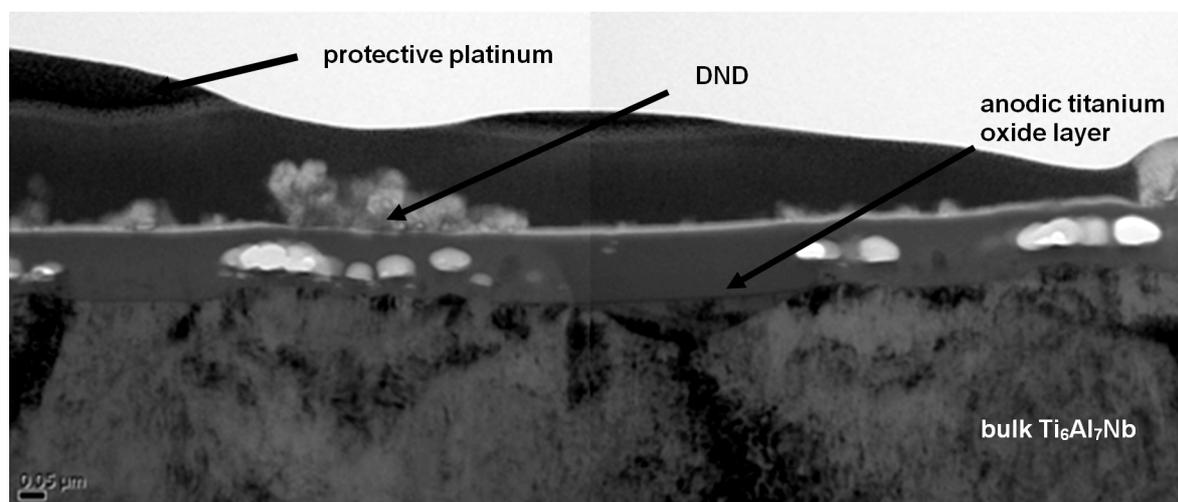
**Figure 5:** STEM image of immobilized aminosilanzed DND **6** adsorbed to the air-formed passive layer of  $\text{Ti}_6\text{Al}_7\text{Nb}$  sample followed by anodic polarization (60 V, 50  $\text{mA}/\text{cm}^2$ ).
