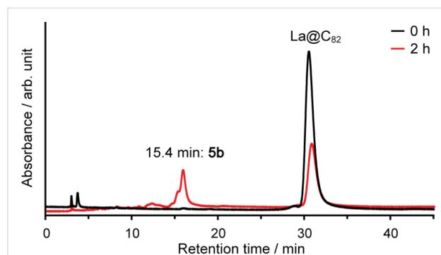
**Figure 10:** HPLC profiles of the reaction mixture for **5b**. Conditions: column, Buckyprep ( $\varnothing$  4.6 mm  $\times$  250 mm); eluent, toluene; flow rate, 1.0 mL/min; wavelength: 330 nm; 40  $^\circ\text{C}$ .
