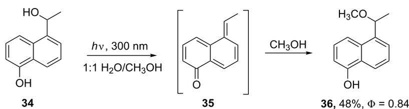
**Scheme 8:** Photodehydration and substitution of 5-(1-hydroxyethyl)-1-naphthol **34** [19].
