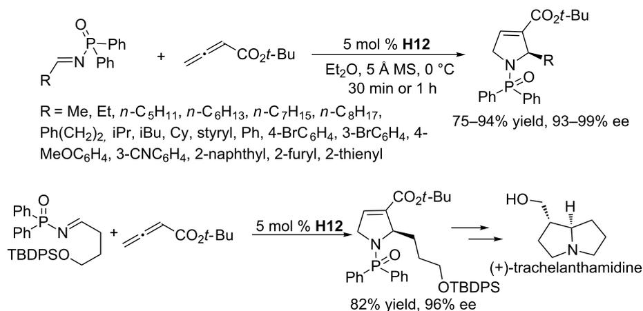
**Scheme 34:** Asymmetric [3 + 2] annulation of *N*-diphenylphosphinoylimines with allenates, catalyzed by the chiral phosphine **H12**, and its application in the formal synthesis of (+)-trachelanthamidine.
