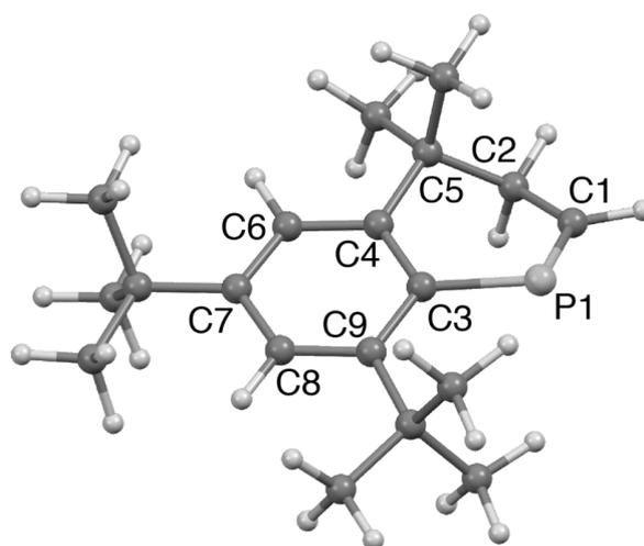
**Figure 4:** Optimized structure of **2** [MP2(full)/6-31G(d)]. Bond distances (Å): P1–C1 1.678, C1–C2 1.491, P1–C3 1.840, C2–C5 1.534, C3–C4 1.424, C4–C5 1.530, C4–C6 1.396, C6–C7 1.394, C7–C8 1.393, C8–C9 1.403, C3–C9 1.427. Bond angle and dihedral angles (°): C3–P1–C1 101.7, C1–P1–C3–C4 22.9, C1–P1–C3–C9 160.1.
