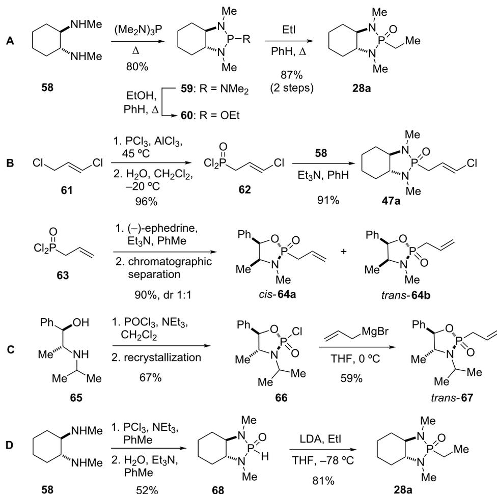
**Scheme 9:** Synthesis of phosphonamides by (A) Arbusov reaction, (B) condensation of diamines with phosphonic acid dichlorides, (C) nucleophilic displacement, (D) alkylation of phosphorus acid diamides [1,5,6,28,30,51,69].
