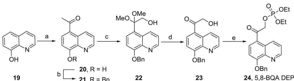
**Scheme 2:** Synthesis of diethyl 8-(benzyloxy)quinolin-5-yl-2-oxoethyl phosphate (5,8-BQA DEP, **24**). Reagents and conditions: (a) CH<sub>3</sub>COCl, AlCl<sub>3</sub>, nitrobenzene, 14 h, 40%; (b) PhCH<sub>2</sub>Br, K<sub>2</sub>CO<sub>3</sub>, DMF, rt, 24 h, 100%; (c) PhI(OAc)<sub>2</sub>, MeOH, KOH, 0 °C to rt, 24 h, 90%; (d) 50% CH<sub>3</sub>COOH, rt, 12 h, 98%; (e) P(O)Cl(OEt)<sub>2</sub>, pyridine, –5 °C to rt, 24 h, 30%.
