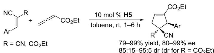
**Scheme 22:** Asymmetric [3 + 2] annulations of arylidenemalononitriles and analogues with an allenolate, catalyzed by the chiral phosphine **H5**.
