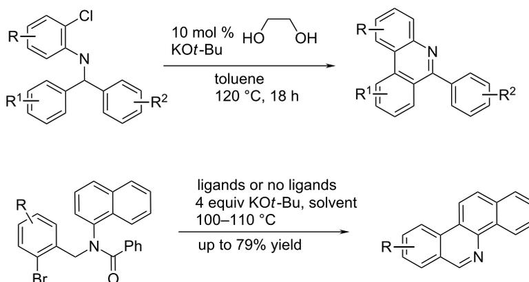
**Scheme 17:** C–H arylation with aryl chloride in the presence of a simple diol complex with KO*t*-Bu (top) [39]; for some cases it worked also in the absence of diol (bottom) [40].
