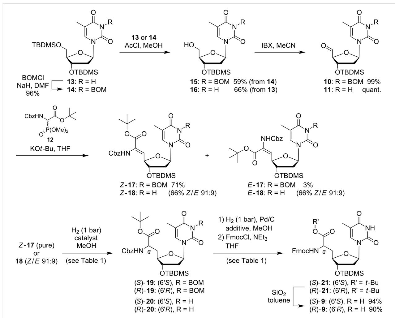
**Scheme 2:** Synthesis of *N*-Fmoc-protected thymidine-derived nucleosyl amino acids (*S*)-**9** and (*R*)-**9**; details on the reactions from **17** and **18** to **21** (asymmetric hydrogenation and subsequent protecting group manipulations) are given in Table 1.
