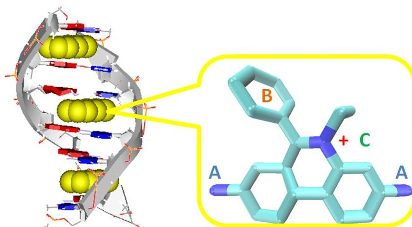
**Figure 1:** Schematic presentation of the intercalative binding mode by the neighbour exclusion principle and important structural features of ethidium bromide: A) amino substituents responsible for fluorescence increase upon DNA intercalation; B) phenyl substituent for steric control and also impact on fluorimetric properties; C) permanent positive charge for aqueous solubility and electrostatic attraction to the DNA or RNA phosphate backbone.
