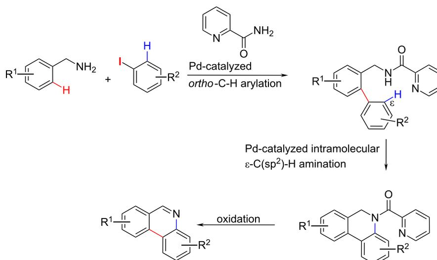
**Scheme 11:** The common Pd-catalyst for the biphenyl conjugation results simultaneously in picolinamide-directed cyclisation; obtained *N*-picolinamide dihydrophenanthridine is easily converted to phenanthridine [32].
