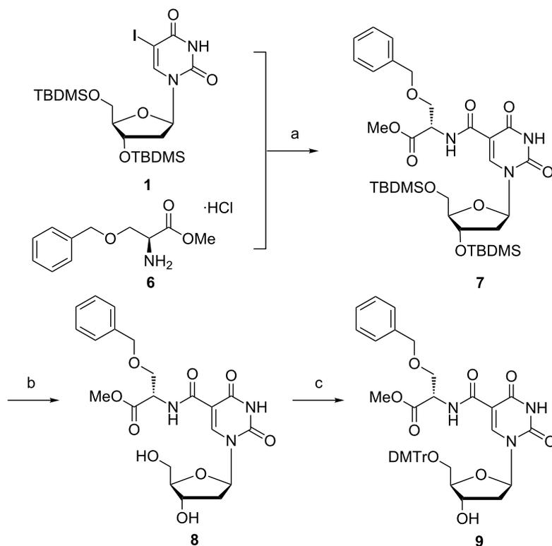
**Scheme 2:** Reagents and conditions: a)  $Et_3N$ ,  $Pd(PPh_3)_4$ , THF, CO (4 bar), 48 h, 70 °C (68%); b)  $Et_3N \cdot 3HF$ ,  $Et_3N$ , THF, overnight, rt (86%); c) DMTr-Cl, pyridine, DCM, overnight, rt (82%).
