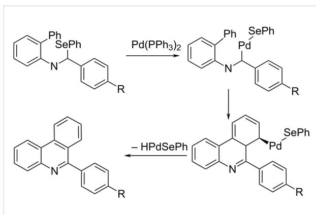
**Scheme 12:** Pd(0)-mediated cyclisation of imidoyl-selenides forming 6-arylphenanthridine derivatives [16]. The insertion of the Pd(0) species into the carbon selenium bond followed by fast rearomatization to phenanthridine is involved with the loss of HPdSePh.
