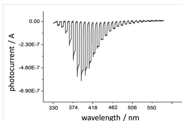
**Figure 6:** Photocurrent generated at the  $[\text{CrF}_5(\text{H}_2\text{O})]^{2-}$ @ $\text{TiO}_2$  electrode as a function of the wavelength of the incident light, recorded at constant potential of 500 mV vs Ag/AgCl. The spikes originate from the opening and closing of the shutter.
