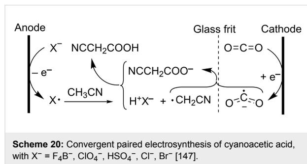
The electrocarboxylation of acetonitrile to cyanoacetic acid is an example of a convergent paired electrosynthesis, meaning that two different substrates undergo either oxidation or reduction to afford products that react among themselves to generate
