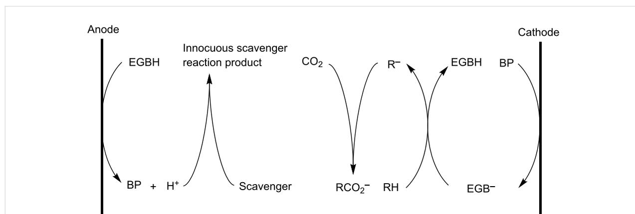
**Scheme 21:** General scheme of carboxylation of weak acidic hydrocarbons with electrogenerated bases. RH: weakly acidic hydrocarbon; BP: base precursor; EGB<sup>-</sup>: electrogenerated base; EGBH: conjugate acid of electrogenerated base [151].
