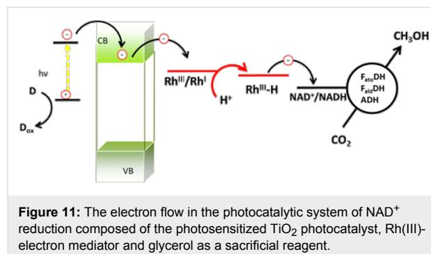
**Figure 11:** The electron flow in the photocatalytic system of  $\text{NAD}^+$  reduction composed of the photosensitized  $\text{TiO}_2$  photocatalyst,  $\text{Rh}(\text{III})$ -electron mediator and glycerol as a sacrificial reagent.
