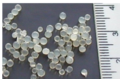
Figure 12: Beads produced from Ca-alginate and TEOS containing co-encapsulated F_{\text{ate}}\text{DH} , F_{\text{ald}}\text{DH} and ADH.
