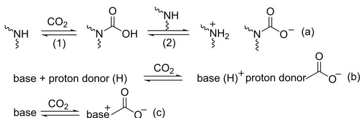
**Scheme 1:** Reactions of CO<sub>2</sub> with amino-group containing absorbents (a), base/proton donor binary system (b) or strong organic base (c).
