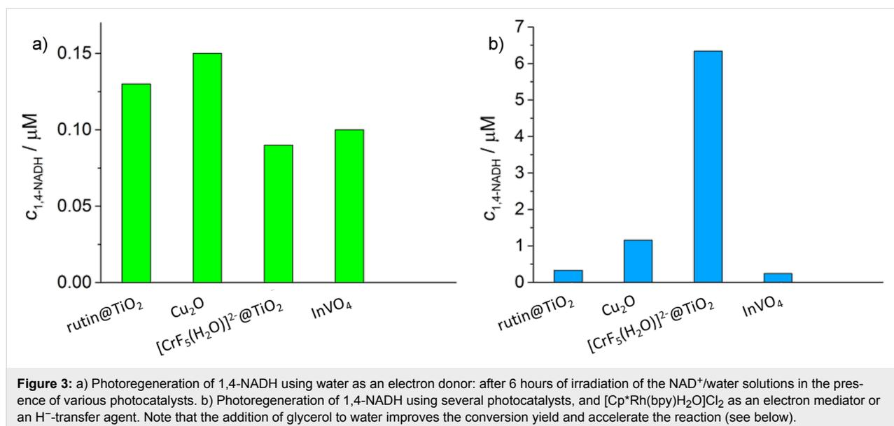
**Figure 3:** a) Photoregeneration of 1,4-NADH using water as an electron donor: after 6 hours of irradiation of the NAD<sup>+</sup>/water solutions in the presence of various photocatalysts. b) Photoregeneration of 1,4-NADH using several photocatalysts, and [Cp<sup>\*</sup>Rh(bpy)H<sub>2</sub>O]Cl<sub>2</sub> as an electron mediator or an H<sup>+</sup>-transfer agent. Note that the addition of glycerol to water improves the conversion yield and accelerate the reaction (see below).
