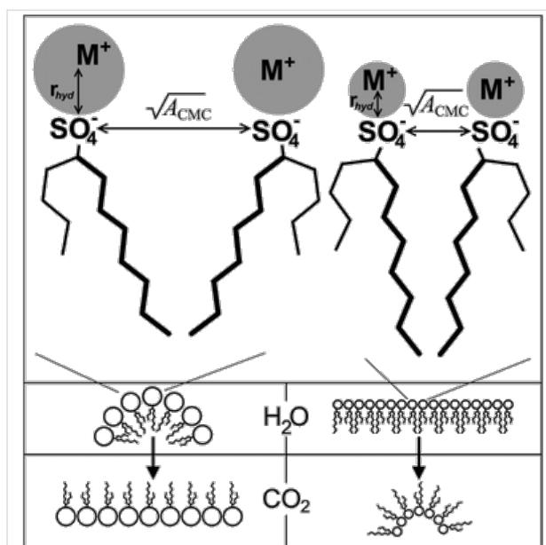
**Figure 6:** Schematic showing how hydrated cation radius ( $r_{\text{hyd}}$ ) mediates surfactant headgroup repulsions by controlling limiting headgroup area at critical micelle concentration ( $A_{\text{cmc}}$ ). Changes in  $A_{\text{cmc}}$  and  $r_{\text{hyd}}$  affect preferred curvature and therefore aggregate morphology in water and scCO<sub>2</sub>. Reprinted with permission from [32]. Copyright 2012 American Chemical Society.
