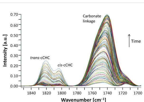
**Figure 3:** Carbonate region of the time-resolved IR spectra recorded during the copolymerisation of CO<sub>2</sub> and cyclohexene with catalyst **2**.
