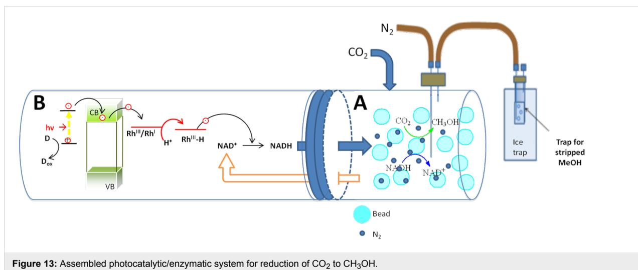
**Figure 13:** Assembled photocatalytic/enzymatic system for reduction of  $\text{CO}_2$  to  $\text{CH}_3\text{OH}$ .
