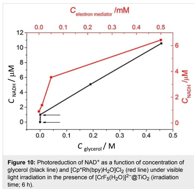
**Figure 10:** Photoreduction of  $\text{NAD}^+$  as a function of concentration of glycerol (black line) and  $[\text{Cp}^*\text{Rh}(\text{bpy})\text{H}_2\text{O}]\text{Cl}_2$  (red line) under visible light irradiation in the presence of  $[\text{CrF}_5(\text{H}_2\text{O})]^{2-}@\text{TiO}_2$  (irradiation time; 6 h).
