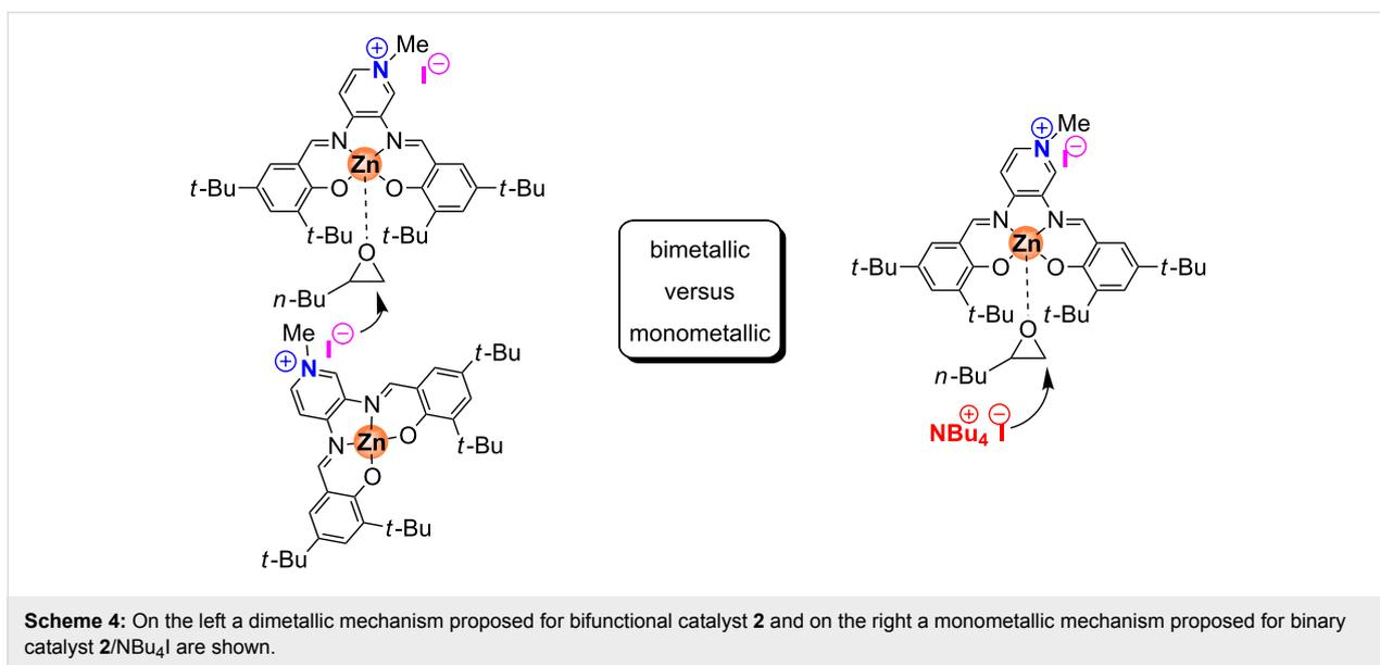
bifunctional Zn complex **2** (0.1–0.4 mol %). These experiments were carried out at 40 °C, a minimal reaction temperature required for the bifunctional catalyst to provide a sufficiently disaggregated state and thus the required Lewis acid centers for catalytic turnover when combined with NBu<sub>4</sub>I (Figure 9).
