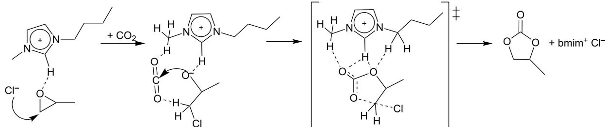
**Scheme 5:** Two-step pathway for the cycloaddition of propylene oxide and CO<sub>2</sub> in the ionic liquid 1-butyl-3-methylimidazolium chloride (bmim<sup>+</sup> Cl<sup>−</sup>).
