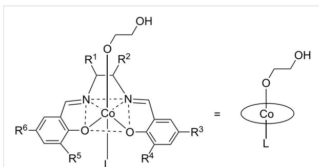
**Figure 2:** The [(2-hydroxyethoxy)Co<sup>III</sup>(salen)(L)] complex chosen as catalyst model for the calculations; **1:** R<sup>1–6</sup> = H; **1a:** R<sup>1–2</sup> = -C<sub>4</sub>H<sub>9</sub>, R<sup>3–6</sup> = H; **1b:** R<sup>1–2</sup> = -C<sub>4</sub>H<sub>8</sub>, R<sup>3–6</sup> = *t*-Bu.
