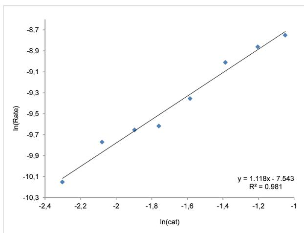
**Figure 6:** Double logarithmic plot to determine the order with respect to the binary system  $\text{NBu}_4\text{I}/\text{Zn}$  complex **1**. Conditions: 1,2-epoxyhexane (10 mmol) as substrate, 30 °C, 1 MPa of  $\text{CO}_2$ , 2 h,  $[\text{Zn}] = [\text{NBu}_4\text{I}] = 0.10\text{--}0.35$  mol %. For the steady state domain using two different concentrations of binary catalyst please refer to Supporting Information File 1, Figure S5.
