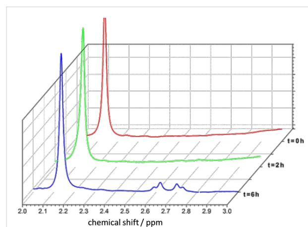
**Figure 4:**  $^1\text{H}$  NMR spectra recorded at  $t = 0$ , after 2 and 6 h of irradiation in water. The selected range, 2–3 ppm, is diagnostic for NADH H-signals. The signal at 2.1 ppm results from the ribose hydrogen in the cofactor molecule and is taken as a reference peak. The concentration of the rhodium complex is 0.5 mM, with  $c_{\text{glycerol}} = 0.05 \text{ M}$ .
