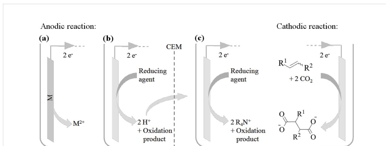
**Scheme 6:** Overview of electrocarboxylation setups using (a) a sacrificial anode, (b) an inert anode, generating protons, with a cation exchange membrane (CEM) and (c) an inert anode, releasing tetraalkylammonium cations.
