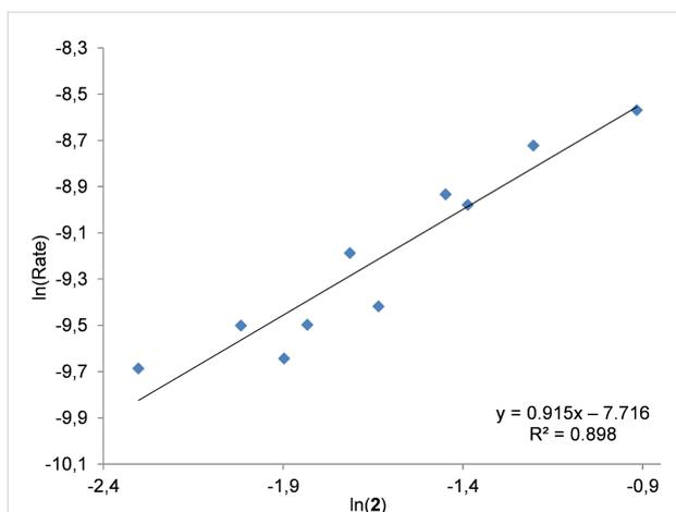
**Figure 9:** Double logarithmic plot to determine the order with respect to the bifunctional Zn complex **2** in the presence of NBu<sub>4</sub>I. Conditions: 1,2-epoxyhexane (10 mmol) as substrate, 40 °C, 1 MPa of CO<sub>2</sub>, 2 h; [2] = 0.1–0.4 mol %, [NBu<sub>4</sub>I] = 0.6 mol % [48].
