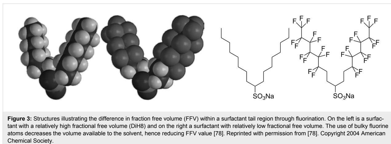
**Figure 3:** Structures illustrating the difference in fraction free volume (FFV) within a surfactant tail region through fluorination. On the left is a surfactant with a relatively high fractional free volume (DiH8) and on the right a surfactant with relatively low fractional free volume. The use of bulky fluorine atoms decreases the volume available to the solvent, hence reducing FFV value [78]. Reprinted with permission from [78]. Copyright 2004 American Chemical Society.
