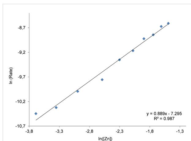
**Figure 4:** Double logarithmic plot to determine the order in binary catalyst Zn(salphen) **1**/NBu<sub>4</sub>I in the presence of a (small) excess of NBu<sub>4</sub>I. Conditions: 1,2-epoxyhexane (10 mmol) as substrate, 30 °C, 1 MPa of CO<sub>2</sub>, 2 h, [Zn] = 0.025–0.225 mol % and [NBu<sub>4</sub>I] = 0.4 mol %. For the steady state domain using two different concentrations of binary catalyst please refer to Supporting Information File 1, Figure S5.
