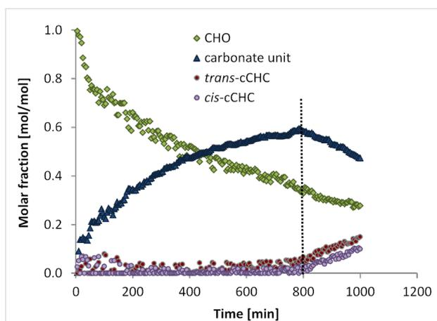
**Figure 4:** Time–concentration profile of the copolymerisation of CO<sub>2</sub> and CHO in the presence of catalytic amounts of complex **2**.
