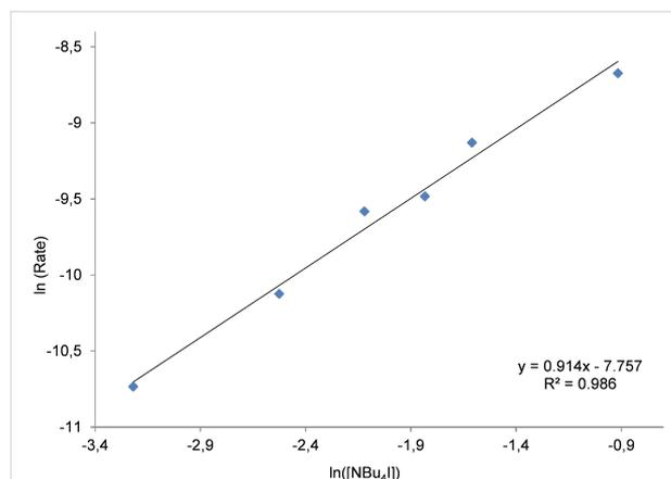
**Figure 5:** Double logarithmic plot to determine the order in binary catalyst Zn(salphen) **1**/NBu<sub>4</sub>I in the presence of (a small excess of) Zn(salphen) complex **1**. Conditions: 1,2-epoxyhexane (10 mmol) as substrate, 30 °C, 1 MPa of CO<sub>2</sub>, 2 h; [Zn] = 0.2 mol %, [NBu<sub>4</sub>I] = 0.04–0.4 mol %. For the steady state domain using two different concentrations of binary catalyst please refer to Supporting Information File 1, Figure S5.
