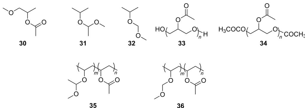
**Figure 4:** Structures of three CO<sub>2</sub>-philic candidates: (**30**) MIA, (**31**) 2MEP and (**32**) 2MMP and the respective polymer candidates they produce: (**33**) -OH terminated oligo(3-acetoxy acetate), OAO, based on MIA; (**34**) -OCOCH<sub>3</sub> terminated OAO, also based on MIA; (**35**) PVMEE, poly(vinyl 1-methoxyethyl ether-co-acetate), based on 2MEP and finally (**36**) PVMME, poly(vinyl methoxymethyl ether-co-acetate), based on 2MMP.
