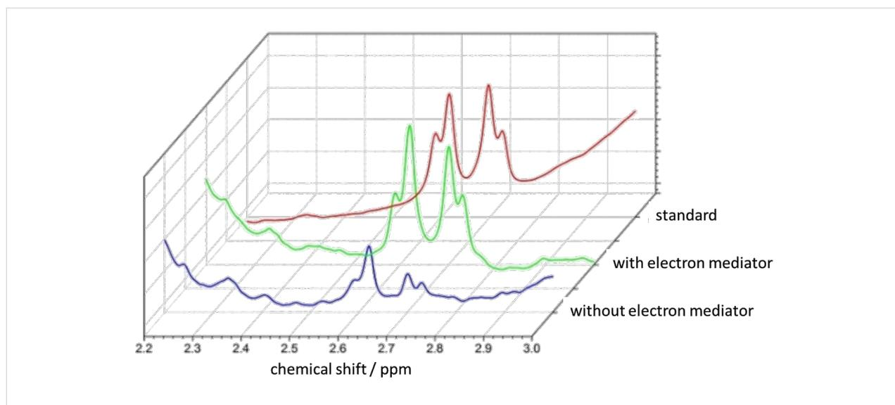
**Figure 5:**  $^1\text{H}$  NMR spectrum of a standard 1,4-NADH (red line), and of 1,4-NADH formed from  $\text{NAD}^+$  upon photocatalysis in the absence (blue) and the presence (green) of the Rh-complex as a mediator and  $[\text{CrF}_5(\text{H}_2\text{O})]^{2-}@\text{TiO}_2$  as a photocatalyst.
