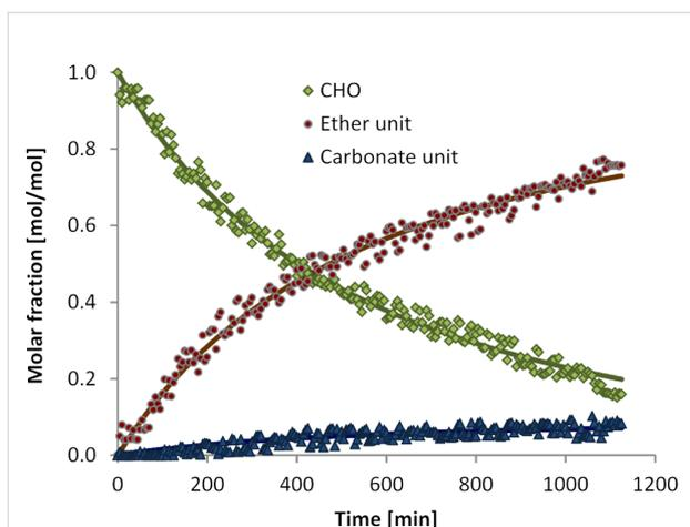
**Figure 2:** Time–concentration profile of the copolymerisation of CO<sub>2</sub> and CHO in the presence of catalytic amounts of complex **1** and fit according to a first order kinetic in CO<sub>2</sub> and in epoxide.
