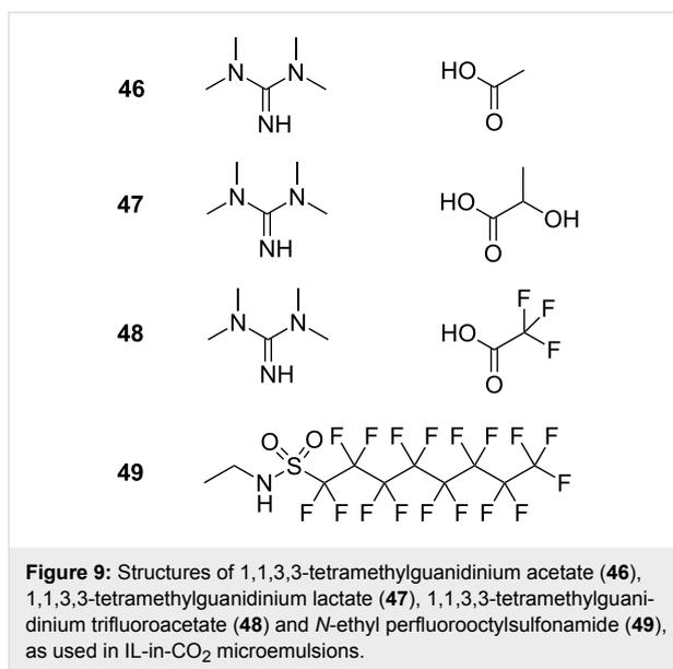
**Figure 9:** Structures of 1,1,3,3-tetramethylguanidinium acetate (**46**), 1,1,3,3-tetramethylguanidinium lactate (**47**), 1,1,3,3-tetramethylguanidinium trifluoroacetate (**48**) and *N*-ethyl perfluorooctylsulfonamide (**49**), as used in IL-in-CO<sub>2</sub> microemulsions.
