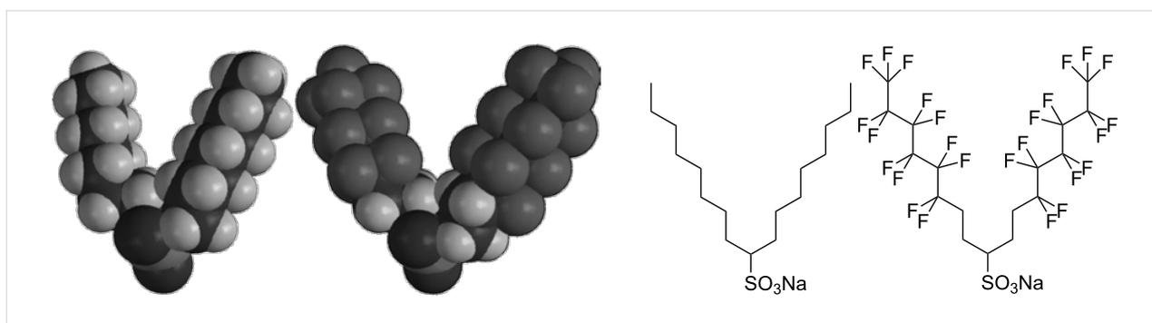
**Figure 3:** Structures illustrating the difference in fraction free volume (FFV) within a surfactant tail region through fluorination. On the left is a surfactant with a relatively high fractional free volume (DiH8) and on the right a surfactant with relatively low fractional free volume. The use of bulky fluorine atoms decreases the volume available to the solvent, hence reducing FFV value [78]. Reprinted with permission from [78]. Copyright 2004 American Chemical Society.
