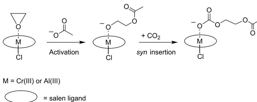
**Scheme 2:** Epoxide and CO<sub>2</sub> copolymerisation by homogeneous Cr(III)- and Al(III)-salen complexes.
