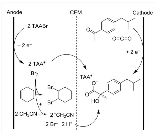
**Scheme 15:** Electrocarboxylation of *p*-isobutylacetophenone with stable electrodes [94,95].
