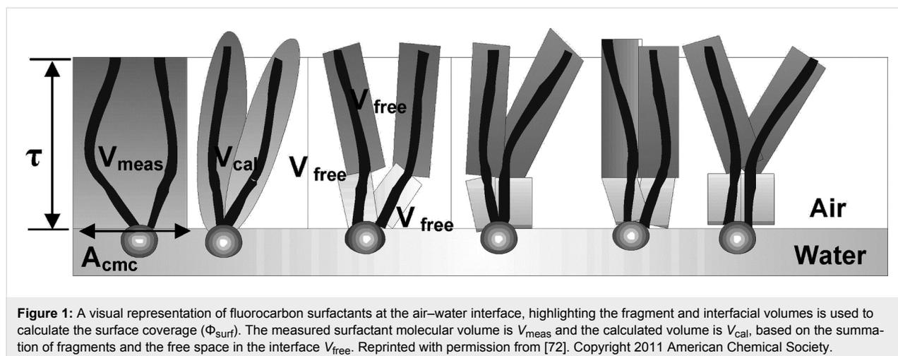
**Figure 1:** A visual representation of fluorocarbon surfactants at the air–water interface, highlighting the fragment and interfacial volumes is used to calculate the surface coverage ( $\Phi_{\text{surf}}$ ). The measured surfactant molecular volume is  $V_{\text{meas}}$  and the calculated volume is  $V_{\text{cal}}$ , based on the summation of fragments and the free space in the interface  $V_{\text{free}}$ . Reprinted with permission from [72]. Copyright 2011 American Chemical Society.
