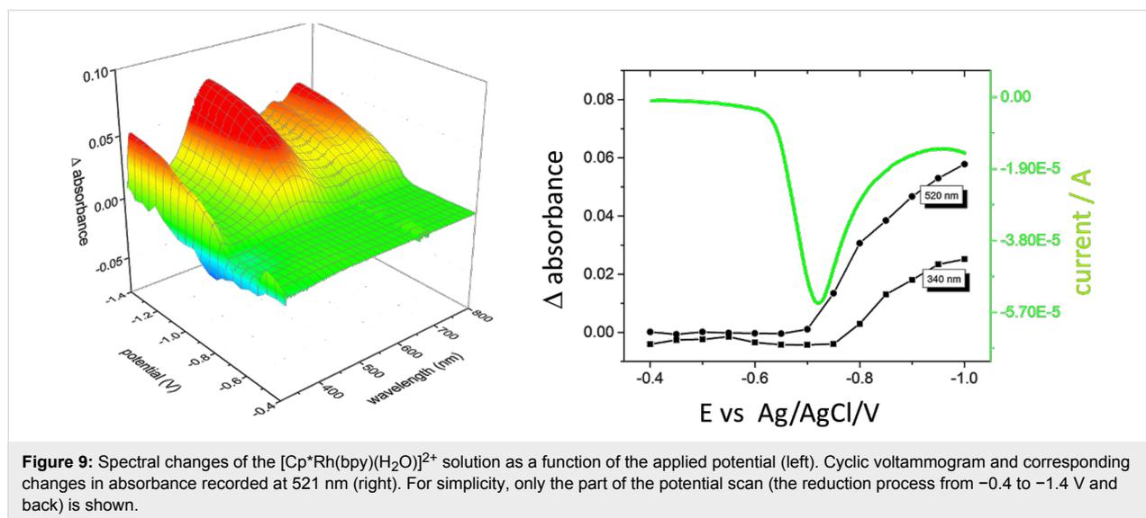
**Figure 9:** Spectral changes of the  $[\text{Cp}^*\text{Rh}(\text{bpy})(\text{H}_2\text{O})]^{2+}$  solution as a function of the applied potential (left). Cyclic voltammogram and corresponding changes in absorbance recorded at 521 nm (right). For simplicity, only the part of the potential scan (the reduction process from  $-0.4$  to  $-1.4$  V and back) is shown.
