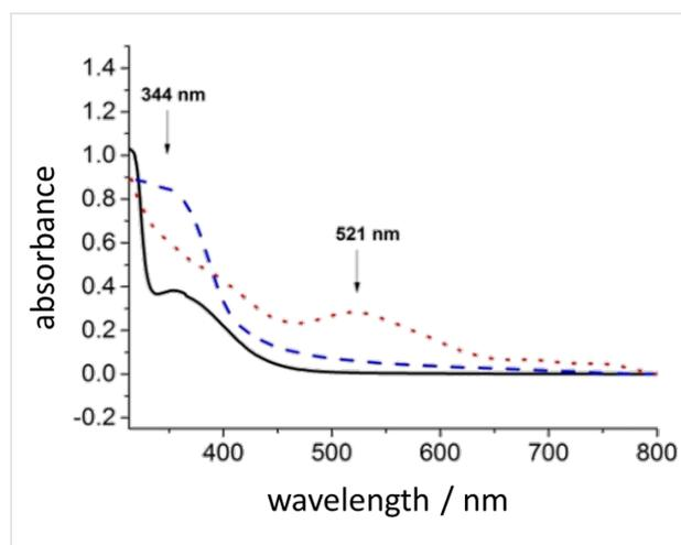
**Figure 8:** UV–vis absorption spectra of an aqueous solution of  $[\text{Cp}^*\text{Rh}(\text{bpy})(\text{H}_2\text{O})]^{2+}$ . Continuous black line: spectrum of the starting rhodium complex in water. Dotted red line: spectrum of the rhodium complex after treatment with hydrogen. Dashed blue line: spectrum of the rhodium-hydride complex after addition of  $\text{NAD}^+$ : the band at 521 nm disappears and the band at 344 nm attributed to  $\text{NADH}$  appears.
