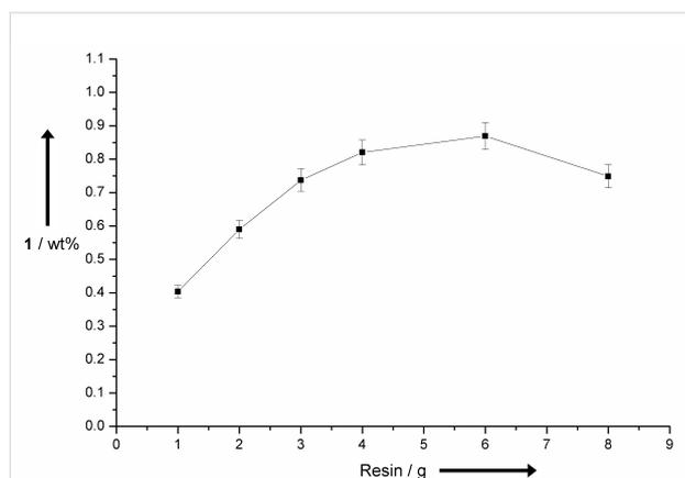
**Figure 8:** Recovery of vanillin (**1**) by adsorption from lignin containing reaction solutions after electrochemical treatment at Ni foam electrodes. Different amounts of resin were applied in a batch process. Desorption was performed treating the loaded resins with an acidic solution (EtOAc/AcOH, 8:2) in a batch process.
