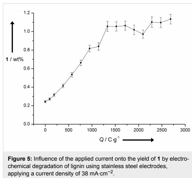
**Figure 5:** Influence of the applied current onto the yield of **1** by electrochemical degradation of lignin using stainless steel electrodes, applying a current density of 38 mA·cm<sup>-2</sup>.
