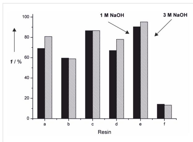
**Figure 6:** Amount of vanillin (**1**) removed by adsorption in a batch process at different strongly basic anion exchange resins. Experiments were performed at two different NaOH concentrations and desorption was realized by acidic treatment of the loaded resins.
