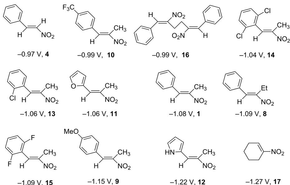
**Scheme 4:** Reduction potentials ( $E_{p,c}$  in Volt) of nitroolefins. Conditions: amalgamated gold wire,  $v = 0.1$  V/s, 0.2 M TEA-*p*Tos in DMF, accuracy of  $E_{p,c} = \pm 0.02$  V vs SCE, measured against the Marple electrode and converted to SCE.
