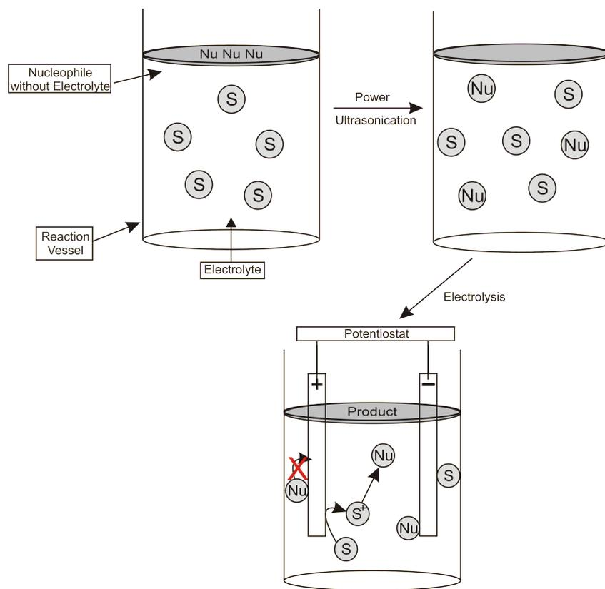
**Figure 4:** Schematic illustration of the anodic substitution reaction system using acoustic emulsification. Figure redrawn from reference [45].
