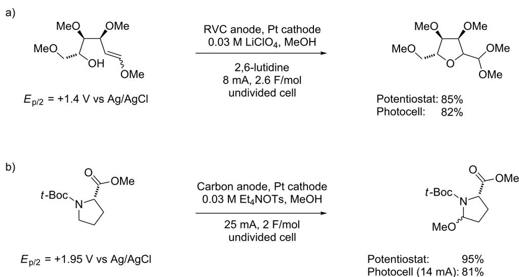
**Scheme 2:** Examples of solar-driven direct electrochemical oxidations.
