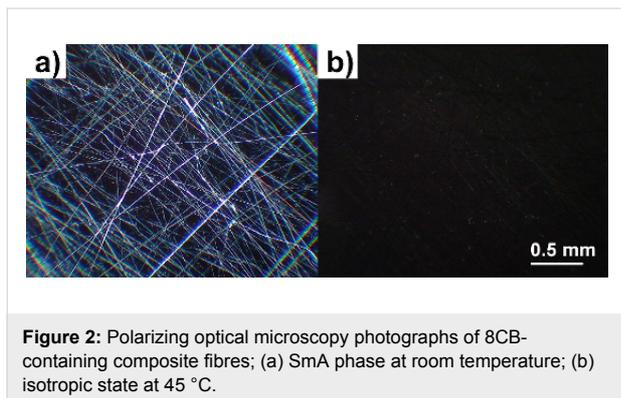
**Figure 2:** Polarizing optical microscopy photographs of 8CB-containing composite fibres; (a) SmA phase at room temperature; (b) isotropic state at 45 °C.
