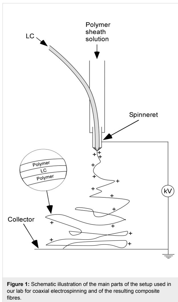
**Figure 1:** Schematic illustration of the main parts of the setup used in our lab for coaxial electrospinning and of the resulting composite fibres.
