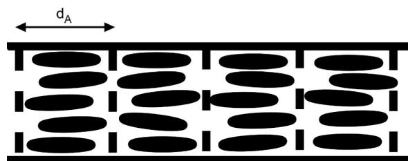
**Figure 10:** Schematic sketch of the arrangement of LC molecules and the smectic layers in an electrospun fibre.
