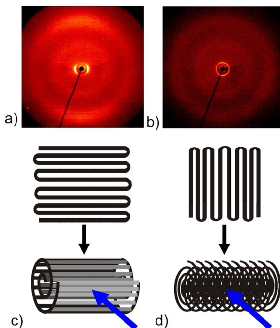
**Figure 8:** a), b): 2D X-ray diffraction pattern of oriented fibres at two perpendicular roll-up directions schematically sketched in c) and d), respectively. The incident X-ray beam is represented by the blue arrow. These scattering patterns from the composite fibres should be compared to those from unfilled PVP fibres and bulk 8CB, respectively, shown in Figure 9.
