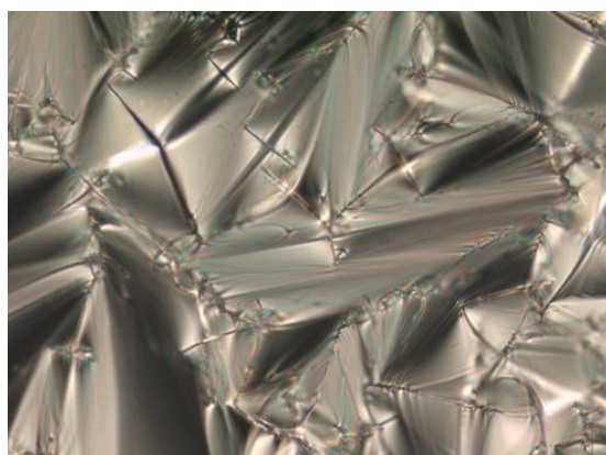
Figure 6: Fan-shaped texture of compound 6e at 45 °C upon cooling from the isotropic liquid (cooling rate 10 K/min) (magnification 200×).
