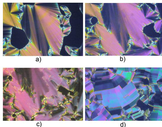
Figure 4: Optical textures of **16D[6]** obtained for the same region of the sample upon cooling: (a) SmA growing from isotropic (251 °C), (b) focal-conic texture of SmC (242 °C), (c) SmI (229 °C), and (d) broken focal-conic texture of SmF (211 °C). Magnification  $\times 60$ .
