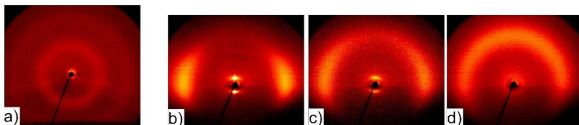
**Figure 9:** X-ray diffraction patterns of PVP fibres without LC (a) and of surface-aligned samples of bulk 8CB in the SmA, nematic and isotropic phase, respectively (b to d).
