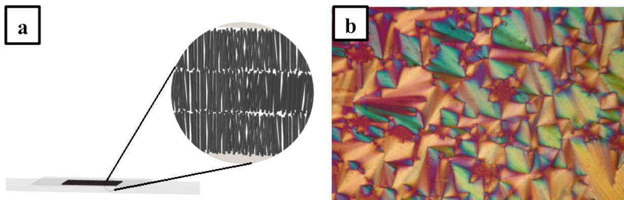
**Figure 5:** (a) Illustration of a single homeotropic monodomain, which is observed as a black isotropic texture under POM, (b) focal conic texture observed at 80 °C with **1<sub>8</sub>** (spacer Mylar foil 100  $\mu\text{m}$ ).
