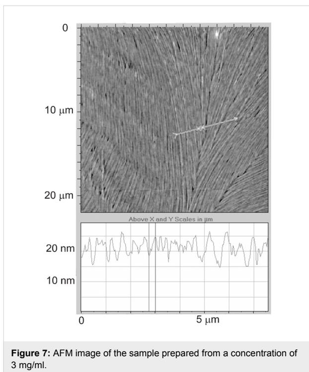
packed together. They appear quite thick even although the section of the surface given by the AFM identifies also some thinner features, suggesting that the thick structures may be thin fibers aggregating into superstructures.
