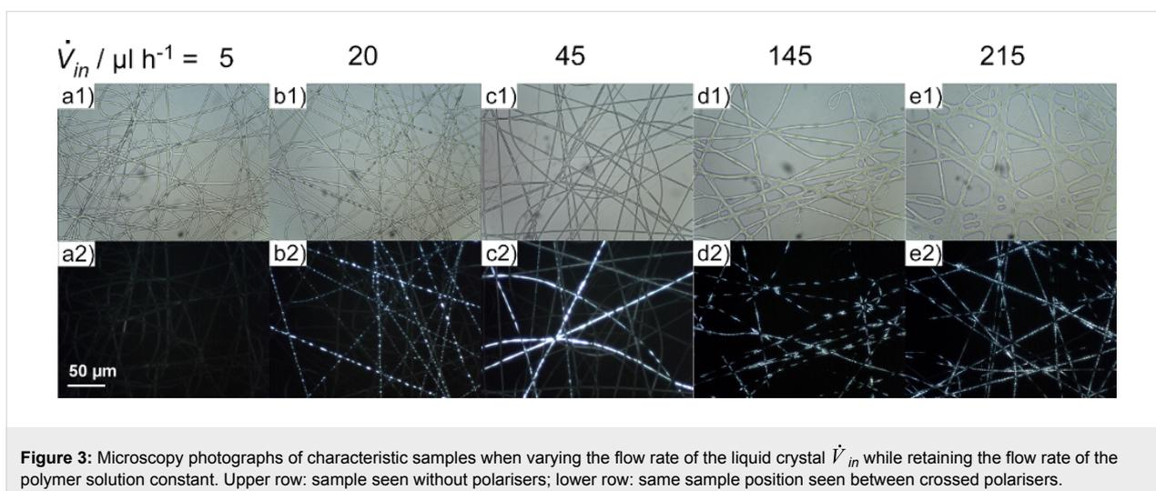
**Figure 3:** Microscopy photographs of characteristic samples when varying the flow rate of the liquid crystal  $\dot{V}_{in}$  while retaining the flow rate of the polymer solution constant. Upper row: sample seen without polarisers; lower row: same sample position seen between crossed polarisers.
