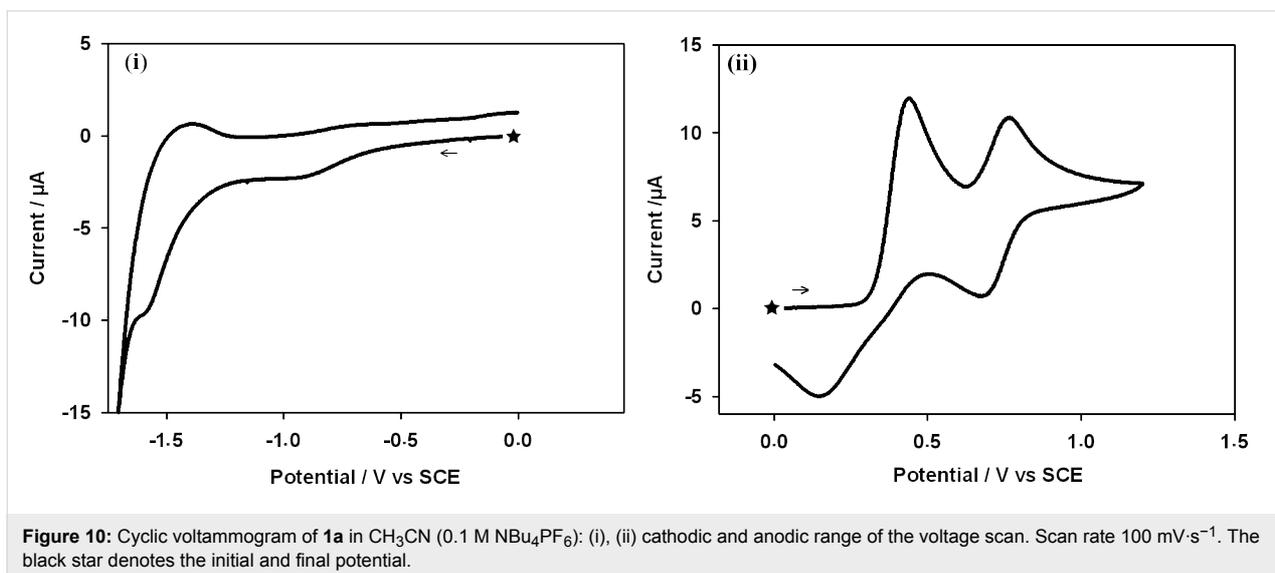
**Figure 10:** Cyclic voltammogram of **1a** in  $\text{CH}_3\text{CN}$  (0.1 M  $\text{NBU}_4\text{PF}_6$ ): (i), (ii) cathodic and anodic range of the voltage scan. Scan rate  $100 \text{ mV}\cdot\text{s}^{-1}$ . The black star denotes the initial and final potential.
