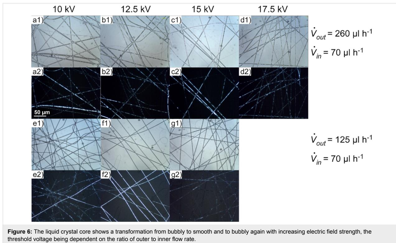
**Figure 6:** The liquid crystal core shows a transformation from bubbly to smooth and to bubbly again with increasing electric field strength, the threshold voltage being dependent on the ratio of outer to inner flow rate.
