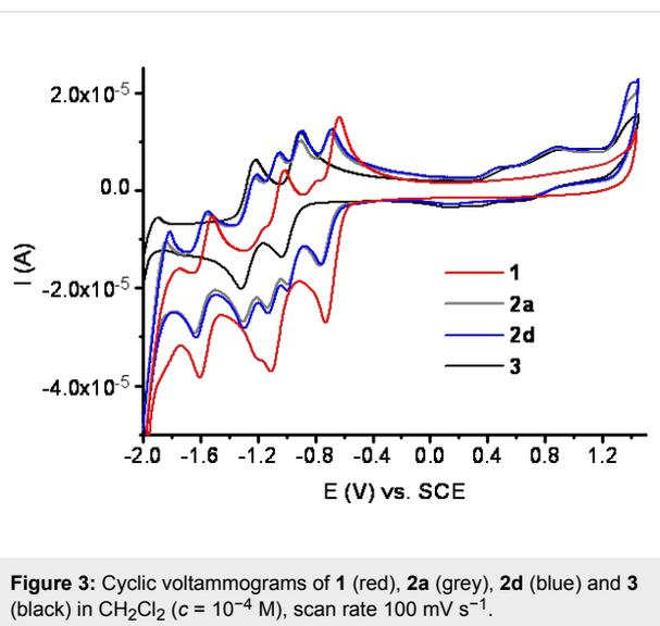
**Figure 3:** Cyclic voltammograms of **1** (red), **2a** (grey), **2d** (blue) and **3** (black) in  $\text{CH}_2\text{Cl}_2$  ( $c = 10^{-4}$  M), scan rate 100  $\text{mV s}^{-1}$ .
