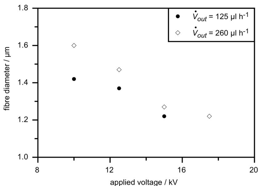
**Figure 7:** Influence of the applied voltage and the flow rate of the polymer solution on the mean fibre diameter.
