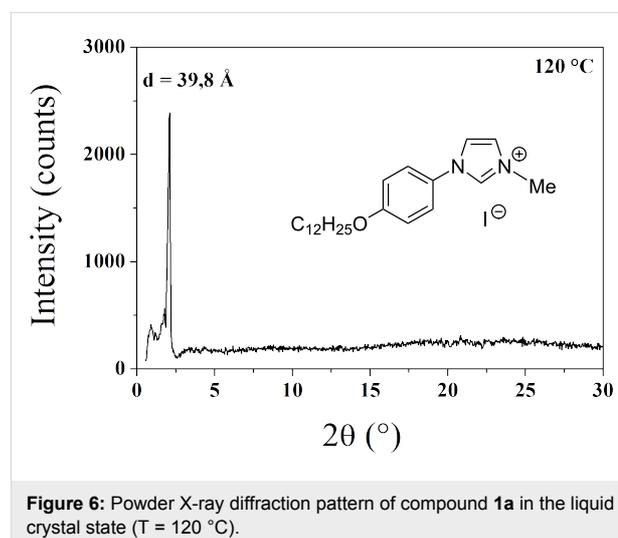
**Figure 6:** Powder X-ray diffraction pattern of compound **1a** in the liquid crystal state ( $T = 120 \text{ °C}$ ).
