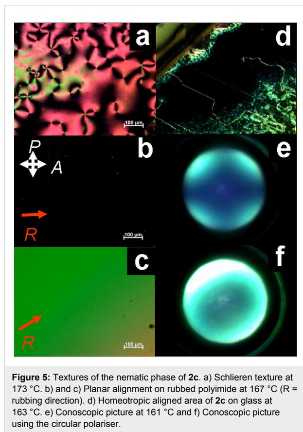
**Figure 5:** Textures of the nematic phase of **2c**. a) Schlieren texture at 173 °C. b) and c) Planar alignment on rubbed polyimide at 167 °C (R = rubbing direction). d) Homeotropically aligned area of **2c** on glass at 163 °C. e) Conoscopic picture at 161 °C and f) Conoscopic picture using the circular polariser.
