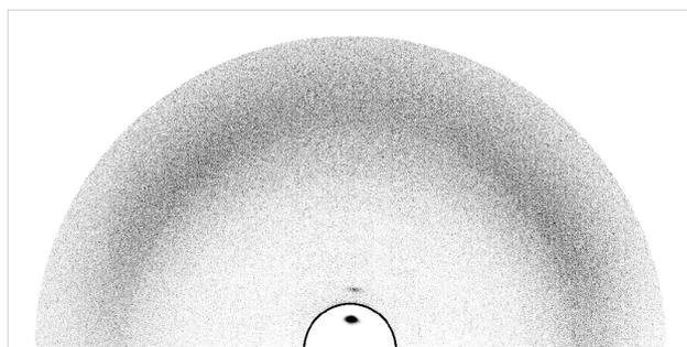
**Figure 8:** Grazing incidence X-ray pattern at 100 °C on the top of a 312 droplet, slowly cooled down from isotropic phase; for image contrast compatibility with the surrounding zone, intensities inside the zone, delimited by the black line and containing the first order reflection of the lamellar stacking, are divided by one hundred.
