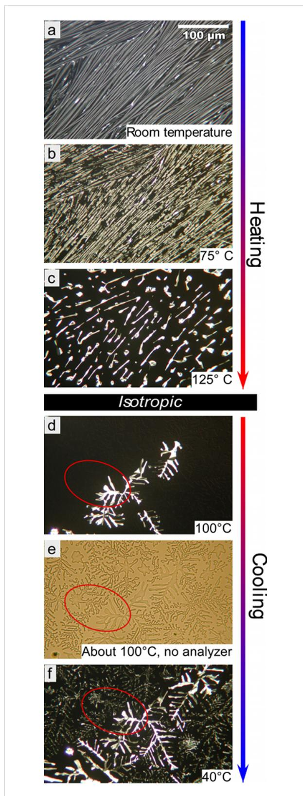
**Figure 1:** Optical microscopy textures of a film prepared by drop-casting on heating to the isotropic phase and subsequent cooling. All images were taken with crossed polarizers, except (e) which was taken with the analyzer removed.
