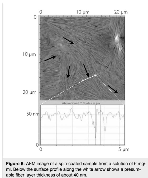
**Figure 6:** AFM image of a spin-coated sample from a solution of 6 mg/ml. Below the surface profile along the white arrow shows a presumable fiber layer thickness of about 40 nm.
