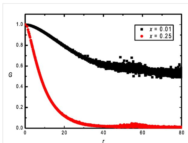
**Figure 1:** Nematic orientational correlation function  $G(r)$  for different values of  $x$  ( $x = 0.01$  and  $0.25$ ),  $N = 80 \times 80 \times 80$ ,  $J_{\text{LC-NP}} = -1$ ,  $J_{\text{LC-LC}} = J_{\text{NP-NP}} = 1$ .
