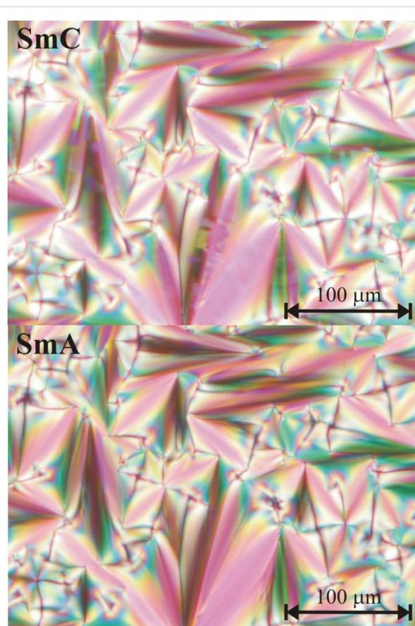
**Figure 6:** Textures of the mixture with 65% **PhP14** in **2PhP** as observed in the polarizing microscope. The upper part shows the broken fan-shaped texture of the SmC phase at  $T = 75$  °C. In the lower part the fan-shaped texture of SmA is observed at  $T = 86$  °C.
