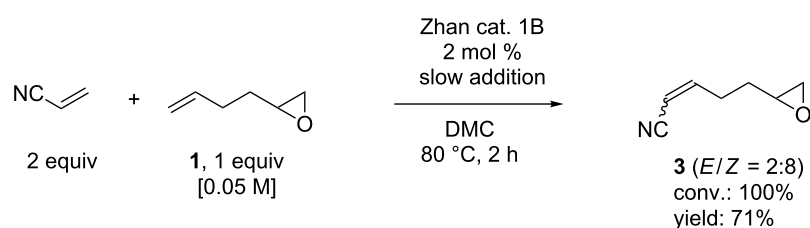
Scheme 2: Cross metathesis of 1 with acrylonitrile.
