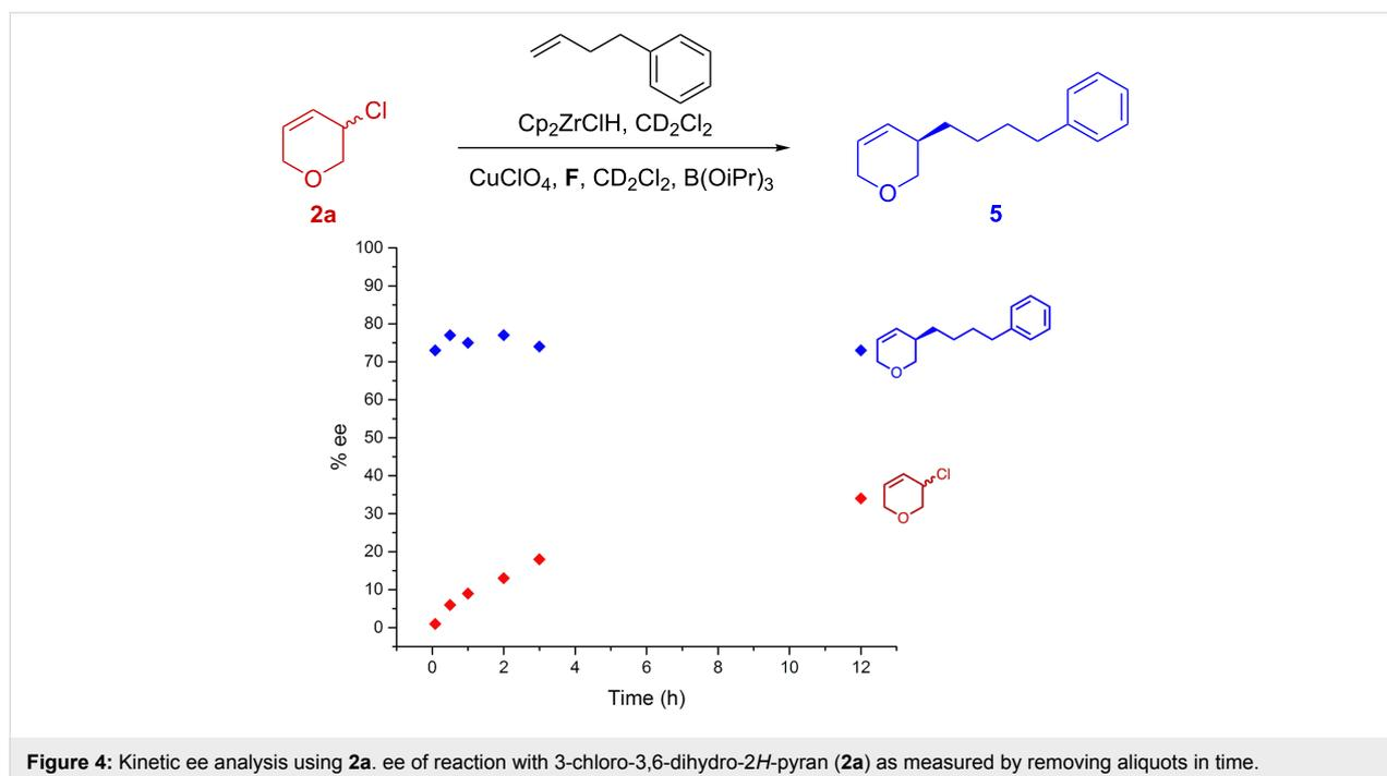
**Figure 4:** Kinetic ee analysis using **2a**. ee of reaction with 3-chloro-3,6-dihydro-2H-pyran (**2a**) as measured by removing aliquots in time.
