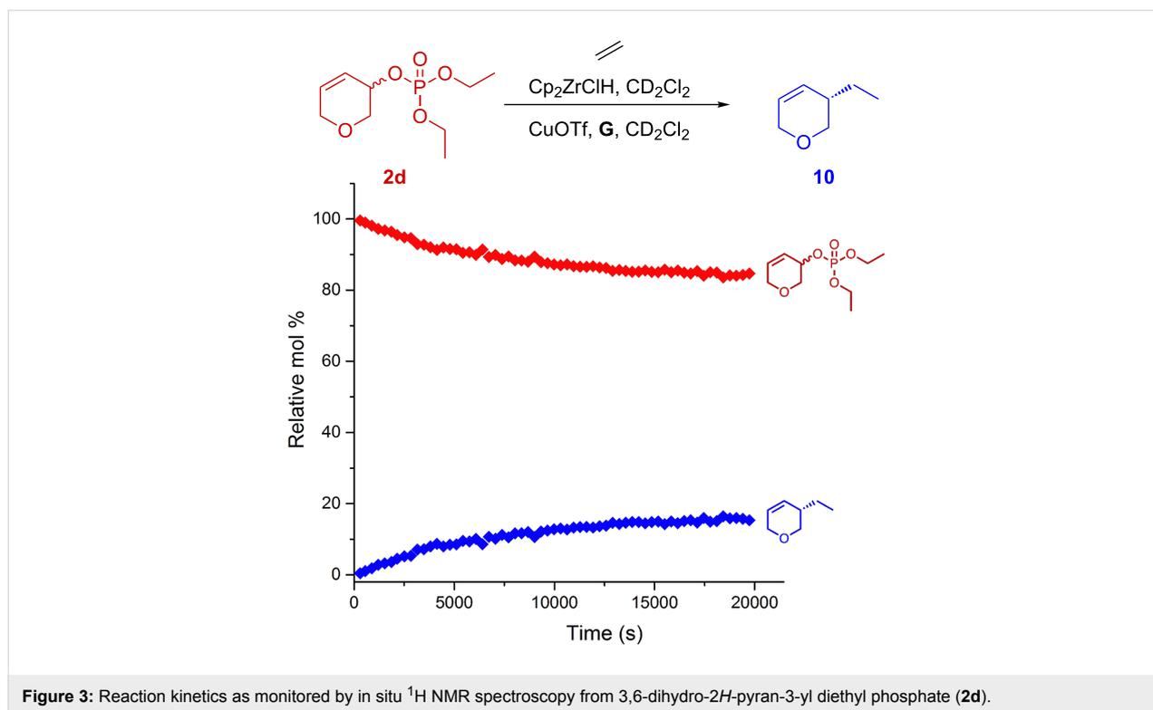
**Figure 3:** Reaction kinetics as monitored by in situ  $^1\text{H}$  NMR spectroscopy from 3,6-dihydro-2H-pyran-3-yl diethyl phosphate (**2d**).
