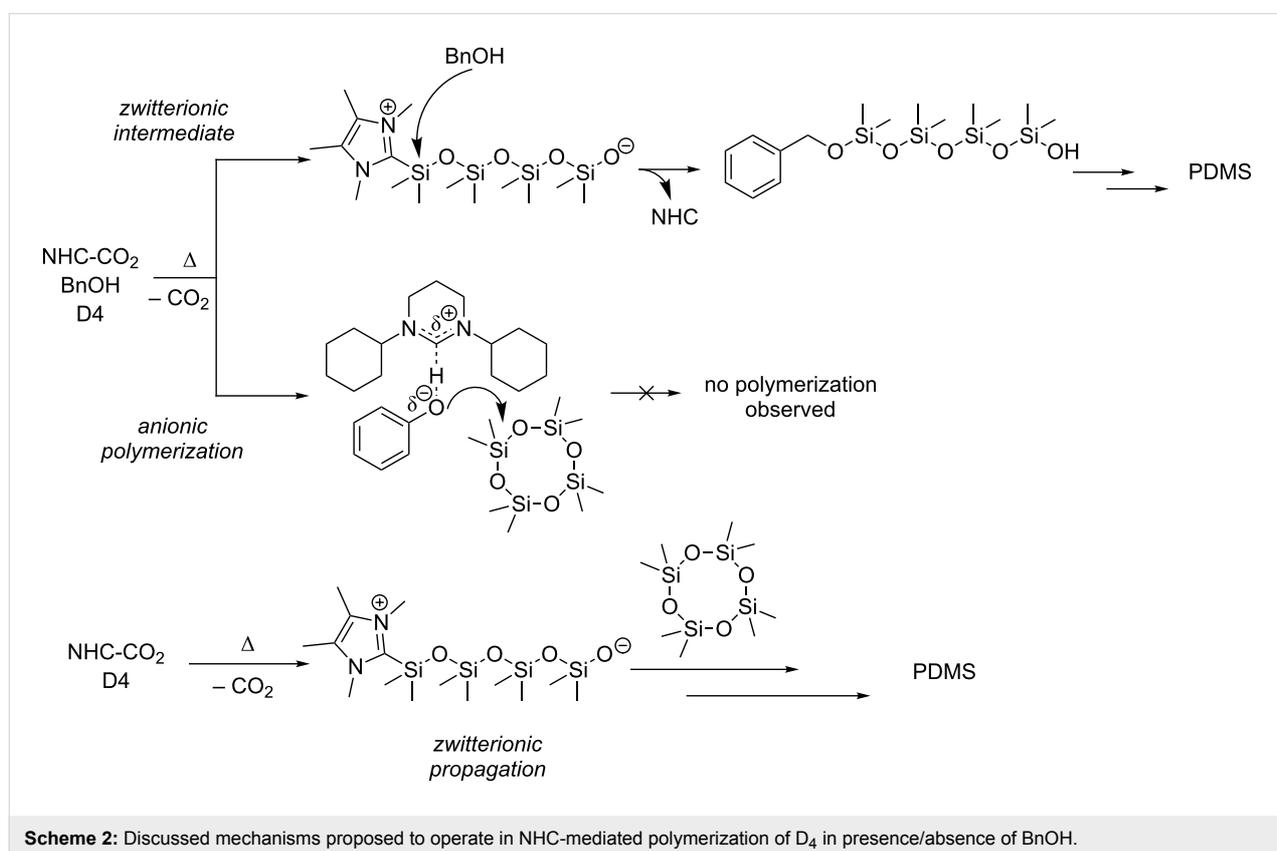
**Scheme 2:** Discussed mechanisms proposed to operate in NHC-mediated polymerization of D<sub>4</sub> in presence/absence of BnOH.
