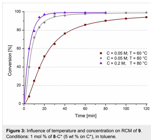
**Figure 3:** Influence of temperature and concentration on RCM of **9**. Conditions: 1 mol % of **8-C\*** (5 wt % on C\*), in toluene.
