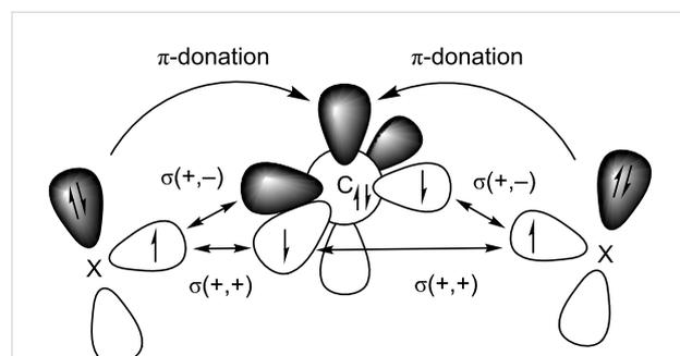
**Scheme 2:** Schematic view of the major orbital interactions between a carbon atom in the  $^3\text{P}$  electronic ground state with the configuration  $2s^2 2p_{\sigma}^1 2p_{\parallel}^1 2p_{\perp}^0$  and atoms  $X$  which possess a  $p(\pi)$  lone pair orbital. There are  $\sigma(+,+)$  and  $\sigma(+,-)$  interactions which give the two  $C_{\text{carb}}-X$   $\sigma$ -bonds and the  $\pi$ -donation  $X(\pi) \rightarrow C_{\text{carb}}$ .
