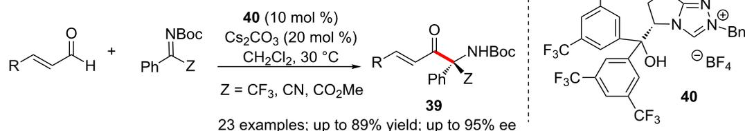
Scheme 25: Aza-benzoin reaction of enals with activated ketimines.
