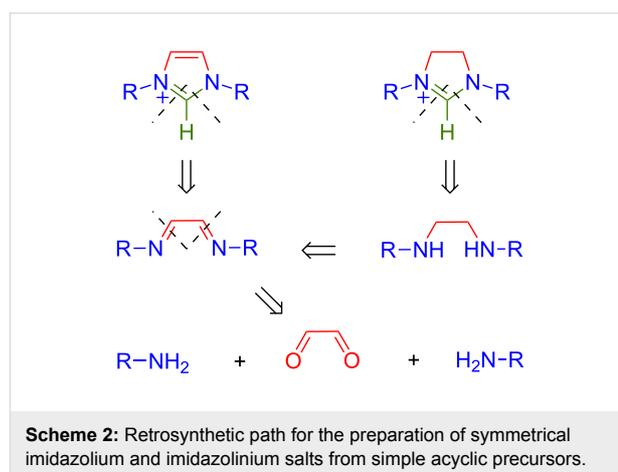
**Scheme 2:** Retrosynthetic path for the preparation of symmetrical imidazolium and imidazolinium salts from simple acyclic precursors.
