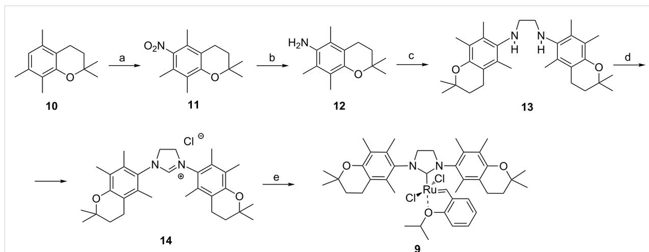
**Scheme 1:** Synthesis of the new NHC precursor. Reagents and conditions: a)  $\text{HNO}_3$ ,  $\text{CH}_2\text{Cl}_2$ ,  $0^\circ\text{C}$ , 58%; b)  $\text{HOCH}_2\text{SOONa}$ , Te, NaOH, dioxane,  $50^\circ\text{C}$ , 50%; c) 2,3-dihydroxy-1,4-dioxane, EtOH, HCOOH, rt, then  $\text{NaBH}_3\text{CN}$ , rt, 90%; d)  $\text{NH}_4\text{Cl}$ ,  $\text{HC}(\text{OMe})_3$ , reflux, 73%; e) I) *t*-AmOK, toluene, rt; II) Hoveyda–Grubbs 1<sup>st</sup> generation, toluene,  $65^\circ\text{C}$ , 68%.
