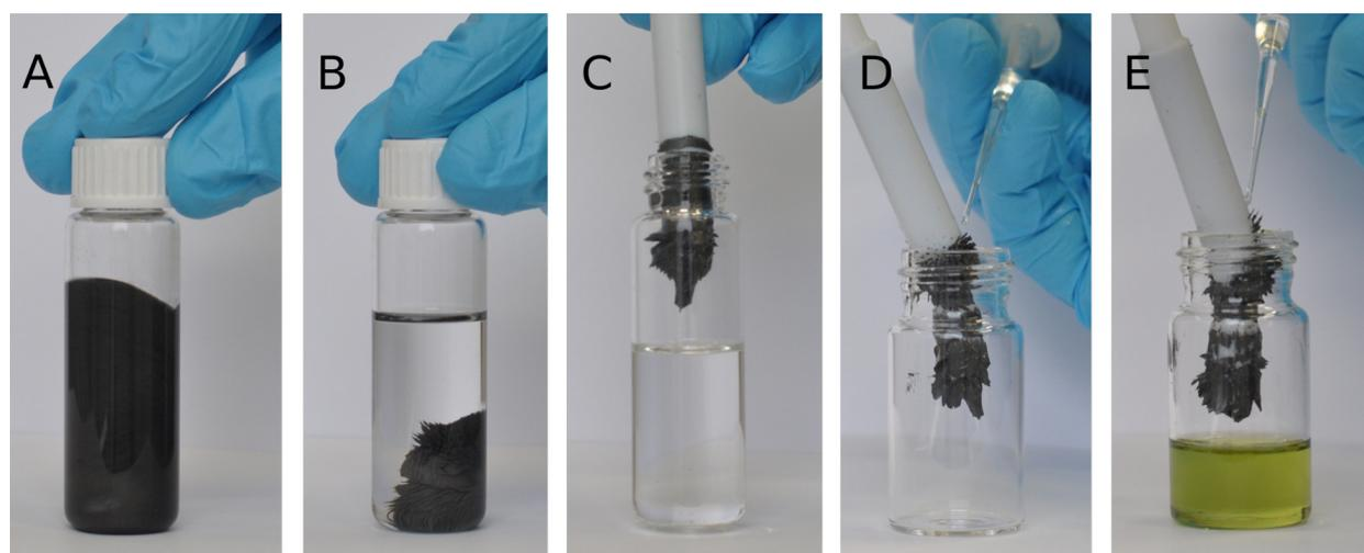
**Figure 9:** Removal of **8**-Fe and subsequent recovery of **8**. A: stirred reaction mixture containing **8**-Fe, B: the same reaction mixture after stirring ceased, C: catalysts **8**-Fe attached to the magnetic rod and removed, D: catalyst **8**-Fe being washed with CH<sub>2</sub>Cl<sub>2</sub>, E: CH<sub>2</sub>Cl<sub>2</sub> solution of catalyst **8** removed from Fe powder.
