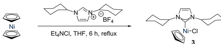
**Scheme 2:** Synthesis of [NiCl(Cp)(ICy)] using conventional heating.
