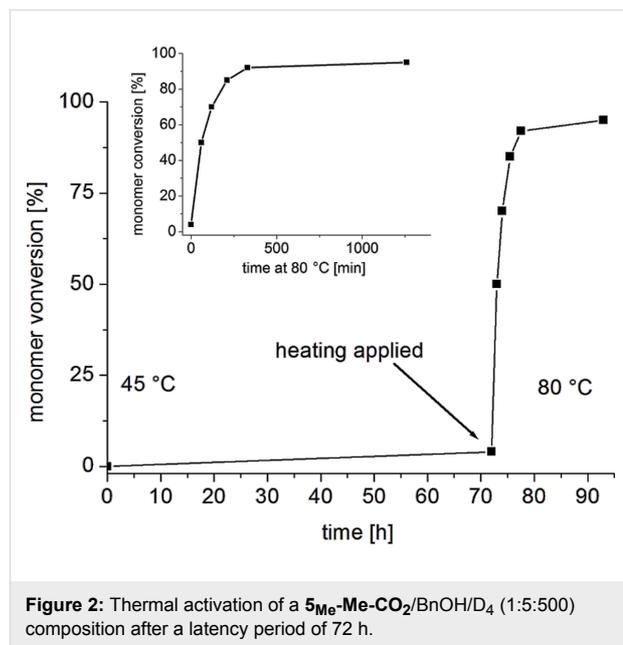
**Figure 2:** Thermal activation of a **5**<sub>Me</sub>-**Me**-**CO**<sub>2</sub>/BnOH/D<sub>4</sub> (1:5:500) composition after a latency period of 72 h.
