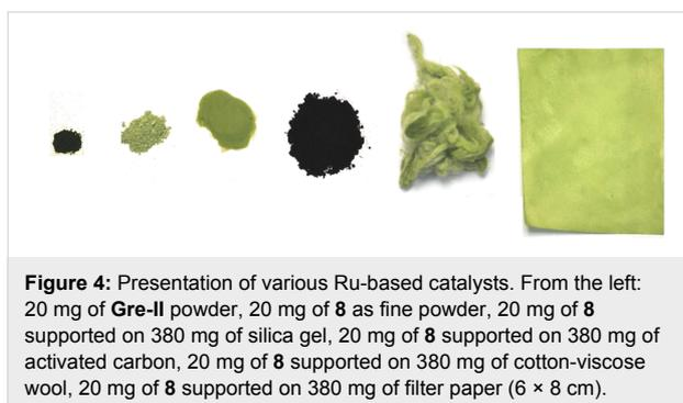
**Figure 4:** Presentation of various Ru-based catalysts. From the left: 20 mg of **Gre-II** powder, 20 mg of **8** as fine powder, 20 mg of **8** supported on 380 mg of silica gel, 20 mg of **8** supported on 380 mg of activated carbon, 20 mg of **8** supported on 380 mg of cotton-viscose wool, 20 mg of **8** supported on 380 mg of filter paper (6 × 8 cm).
