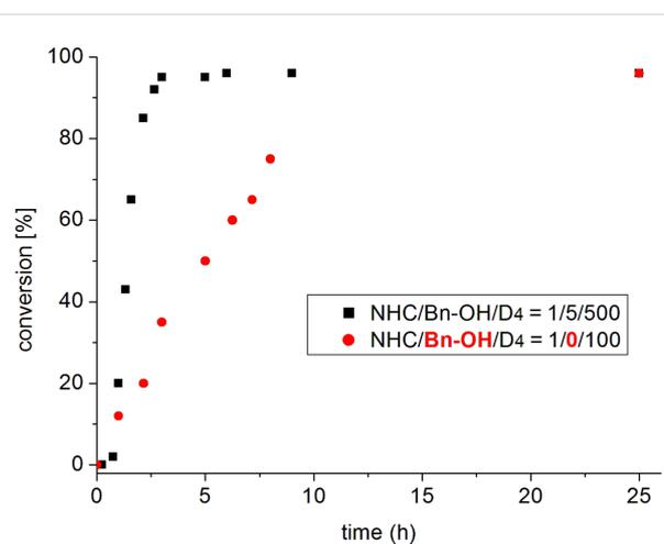
**Figure 1:** Comparison of conversion over time for D<sub>4</sub> polymerization (80 °C, bulk) using **5**<sub>Me</sub>-Me-CO<sub>2</sub>. Note that the fivefold monomer excess was used in case of BnOH being present.
