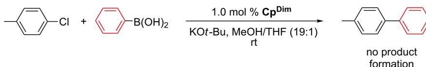
**Scheme 5:** **Cp<sup>Dim</sup>** is not an active precatalyst for a Suzuki–Miyaura reaction at room temperature.
