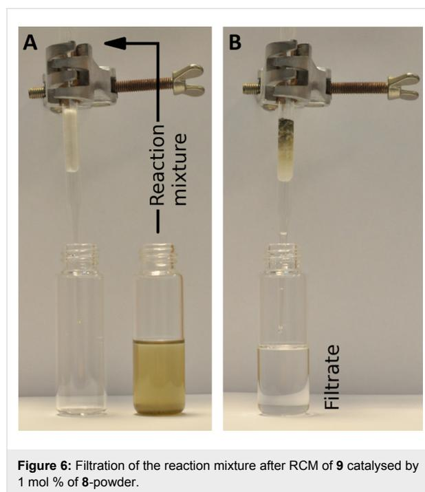
**Figure 6:** Filtration of the reaction mixture after RCM of **9** catalysed by 1 mol % of **8-powder**.
