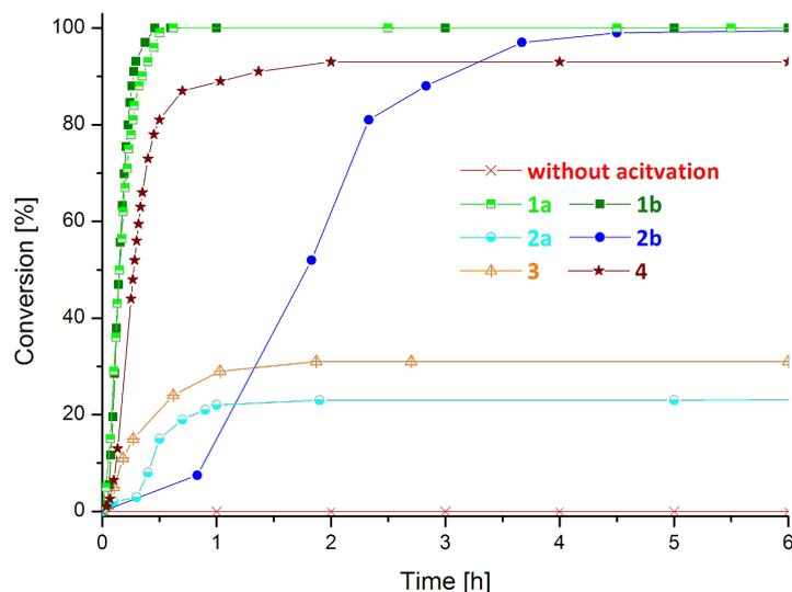
**Figure 2:** Time/conversion plot for the polymerization of **5** by preinitiators **1–4** in the presence of HCl ( $[\text{5}]:[\text{HCl}]:[\text{I}] = 50:25:1$ ;  $[\text{5}] = 0.1 \text{ mol/L}$ ; solvent:  $\text{CDCl}_3$ ).
