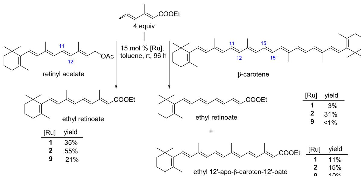
**Scheme 4:** CM reaction of  $\beta$ -carotene and retinyl acetate with ethyl (2*E*,4*Z/E*)-3-methylhexa-2,4-dienoate. Reaction conditions: diene (4 equiv, 0.325 M), alkene (1 equiv, 0.08 M). Yield was obtained by quantitative HPLC analysis. Yields were calculated in relation to polyene (retinyl acetate or  $\beta$ -carotene). In case of the  $\beta$ -carotene reaction, yields were divided by two due to the symmetry of the  $\beta$ -carotene molecule.
