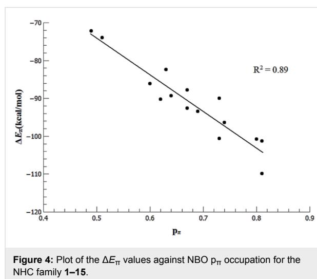
a reasonable correlation between the occupation of the  $p(\pi)$  AO at the  $C_{\text{carb}}$  atom and the energy which is associated with the  $X\rightarrow p(\pi)$   $\pi$ -donation.
